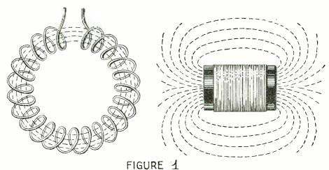
In this picture is shown how the magnetic field of the cylindrical coil sprays outward, while that of the toroid is confined within its windings.
