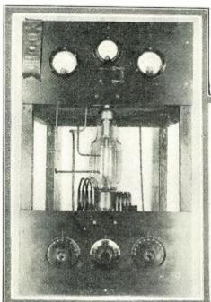
At the left are shown the panel and interior views of the receiver, which is of the Snell type, used at station FXI. The various inductance coils, which are shown on each side of the set, fit in the sockets provided for them in the upper left side of the receiver's baseboard.
