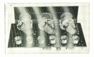
The diagram above shows in exaggerated fashion. the manner in which R.F. coils produce feed-back due to inter-stage coupling. At the left it is indicated how the radio waves, passing over the coils and wiring of the set as well as over the antenna, influence materially the operation of the receiver. The waves picked up by the second stage obviously are not amplified in the first stage. Moreover, this is a common source of interference from locals, when tuning in distant stations.
