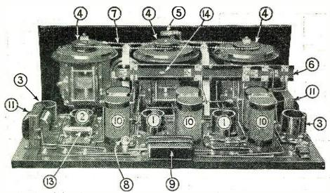
A receiver which employes beaded chains to move the three condensers in approximate synchronism, leaving the final adjustment to individual verniers. 1, R.F. Amplifier Sockets; 2, Detector Socket; 3, A.F. Amplifier Sockets; 4, Chain Gears; 5, Dial Light; 6, Automatic Wave-length Switch; 7, Beaded Chain Control Belt; 8, Pilot Light; 9, By-pass Condenser; 10, Binocular Coils; 11, A. F. Transformers; 13, Grid Leak-condenser; 14, Automatic Switch Lever.
