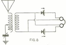
How a single pair of phones can be connected in the Duplex circuit to get full-wave rectification.
