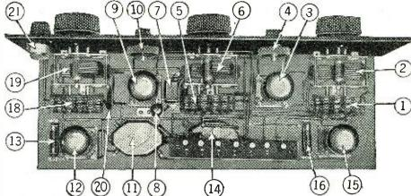
Fig. 3. 7 indicates the grid condenser, of .00025-µf. capacity; 8 is a standard type of variable grid leak; 12 is the first audio frequency amplifier tube; 13 is the amperite controlling the filament of tube 12; 14 is the second audio frequency amplifying transformer; 15 is the second audio frequency amplifier tube; and 16 is its filament control resistance.
