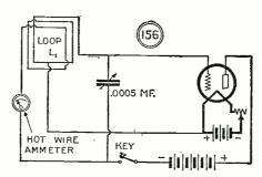
An extremely efficient and simple portable transmitter capable of signaling within the distance of 15 miles, using a loop in place of the conventional antenna.
