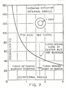
It is seen from this chart that the greatest inductance can be obtained in a toroid for a given coil diameter, when the internal diameter is small, or when the turns are bunched at the middle.
