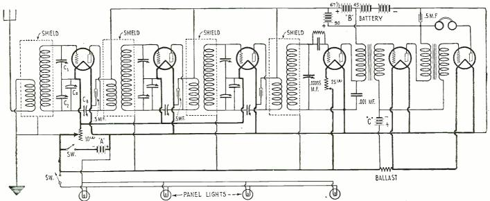
Wiring diagram of the receiver illustrated and described on the preceding page. Notice that the input and output circuits of each stage are kep at zero potential relation to each other by the Wheatstone's bridge arrangement of condensers. Cr compensates for the grid-filament tube capacitance and Cb for the grid-plate capacitance. A swith is provided to cut out the panel lights except when tuning, thus conserving the "A" battery
