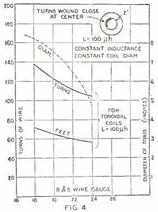
This graph shows the large number of turns and length of wire required in these toroids to give an inductance of 100 microhenries.
