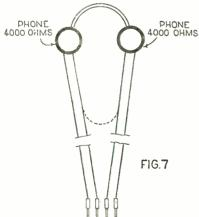
Method of connecting head set for use with Duplex system of crystal detection.
