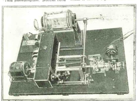
Photos in this article by courtesy of the Radio Corporation of America. Above is shown the transmitting apparatus for the broadcasting of photographs, maps, etc., by means of radio
