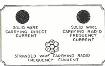
These cross-sections of wires illustrate how different currents behave in different wires.
