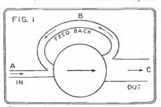
The above diagram shows how part of the output power is returned to the input, thus swelling the final volume of the output.
