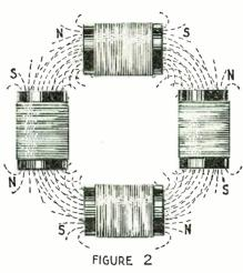
The nature of the toroid can be studied as an evolution from the cylindrical coil as shown by several of the latter arranged in a circle.
