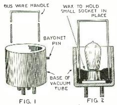
By using an old vacuum tube base, a miniature tamp and socket an efficient tube protector can be easily made.
