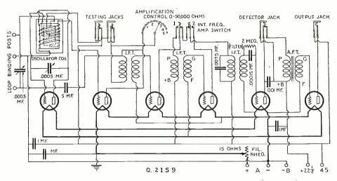
The original circuit used by the Western Electric Company in their type 6004-C radio receiving outfit. The oscillator coil design and connections are included in the diagram; the two 48-turn windings being placed on a 2-inch tube; the 40-turn winding on a 1-inch tube mounted within the 2-inch tube coil.
