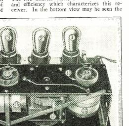
Bottom view of the receiver described on this page. Note that the tubes are mounted horizontally, when the set is in its normal position within the cabinet. The rheostat in the center of the sub-panel is on a common shaft with the tickler coil.
