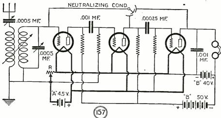
A novel receiving system in which resistance-coupled amplification and a neutralized stage of tuned radio frequency amplification are used, resulting in clear, undistorted signals that are very pleasing to the ear.
