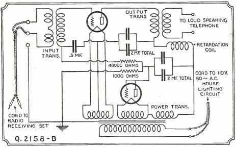
The Western Electric Type-B power amplifier unit which operates directly from an alternating current source, without any batteries required. The unit is very efficient.
