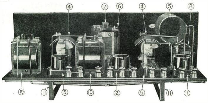
Photos courtesy of Samson Electric Co No. 1 is the R.F. tube socket; 2, the detector tube socket; 3, one of the A.F. amplifier sockets; 4, variable condensers; 5, antenna inductance: 6, R.F. transformer; 7, tickler coil; 8, rheostat; 9, neutralizing condenser; 10, A.F. transformers; 11, baseboard supports.
