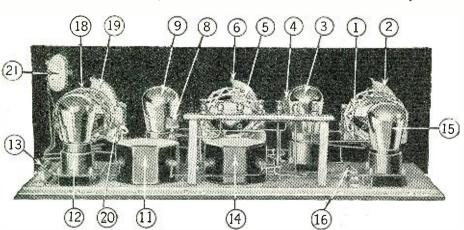
Fig. 4. 20 indicates the .00025-uf. fixed condenser, which is connected in series with the tuning condenser of one of the tuned radio frequency units, in order to reduce the effective capacity of the circuit; 21 is the 100- to 1,000-ohm variable resistance, used for controlling oscillation in the circuit of the detector tube.
