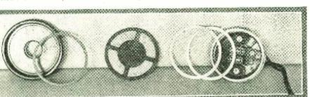
Fig. 2. This illustration shows the complete loud speaker unit disassembled. The metal-and-parchment diaphragm is suspended by means of several rings of fairly porous material, which allows maximum freedom of movement and further reduces any tendency vibration. Photo courtesy of Tower Manufacturing Corp.
