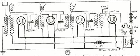
A new method of producing regeneration in, not only the detector stage, but the radio frequency stages as well. Regeneration is carried to such an extreme that unusual sensitivity, and thereby volume and distance, is obtained with this receiver. Cautious tuning is, however, required.
