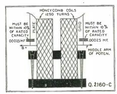
The design of the filter or in-put transformer. Although these coils may be wound similarly to ordinary transformers, ordinary honeycomb coils may be used with the same efficiency.
