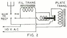
How the automatic switch may be connected in the power supply circuit of a vacuum tube transmitter.
