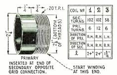
This illustration gives data on the construction of the "canned coils" of the receiver illustrated on page 1414.
