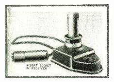
This compact instrument gives a quick, qualitative test of tube functions which would require half a dozen accurate meters to duplicate quantitatively.
