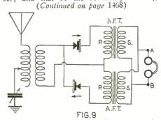
By using two low ratio transformers, a head set connected in the usual way (in series) may be used.
