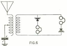
By employing two crystal detectors and two head-phone sets as shown in the above diagram both halves of an incoming radio wave are rectified.
