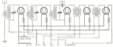
The circuit diagram of the Doughnut Five is shown above. The only adjustment, beside that of the three tuning condensers, is the rotentiometer, for regulating the grid bias on the R. F. tubes.
