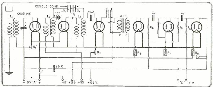
Above is shown the circuit diagram of this six-tube radio frequency receiver. The different values for the parts are given in the accompany-
