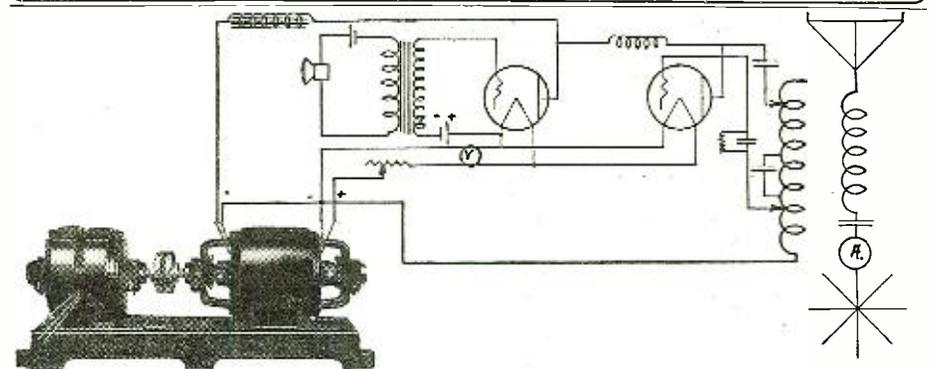
Item 37. 2 unit four bearing set, delivering 1000 volts, 600 watts for plate and 12 volts, 300 watts for filament. The "ESCO" Set is shown here furnishing Power Supply for 4-50 watters in a phone or telegraph set. This is the Item used by CB23 in pioneer achievement of the first two way amateur wireless communication between North and South America.
