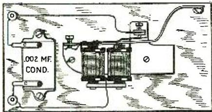
Details of the Vacuum Tube Safety Device.
