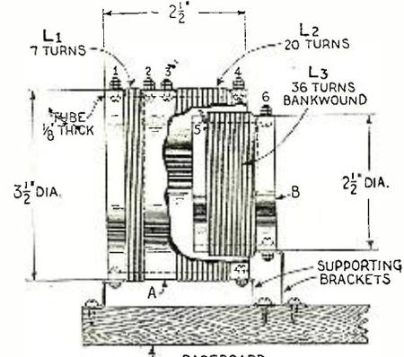
2176-B.—The design of an oscillator coil to operate in conjunction with a .001-mfd. variable condenser for a 10,000-meter type super-heterodyne receiver.
