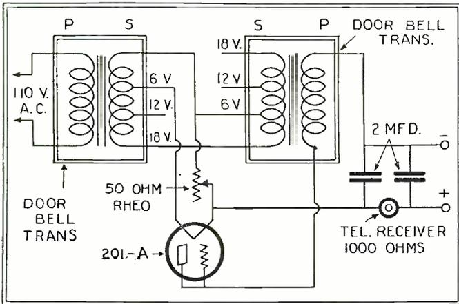
Right: Circuit diagram of one of the home made "B" eliminators. Note the single head-telephone employed as a choke coil.
