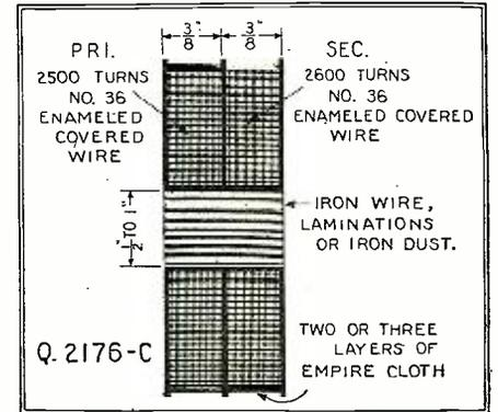
Design of an intermediate transformer which operates with maximum efficiency at 50 to 60 K.C. The correct amount of iron core must be determined experimentally.
