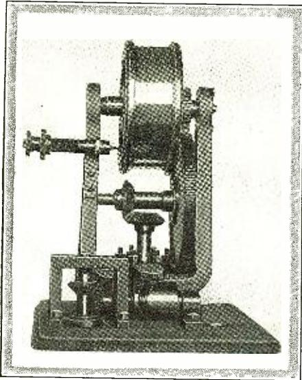
This is a front view of the cylinder or drum of mirrors. It is turned by an electric motor, and at the same time swung from side to side by the gear at its base.
