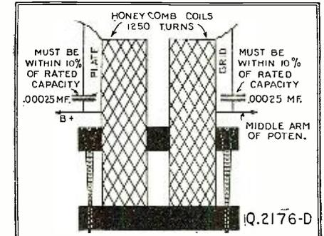
The design of the filter or input transformer. Although these coils may be wound similarly to ordinary transformers, ordinary honeycomb coils may be used with the same efficiency.
