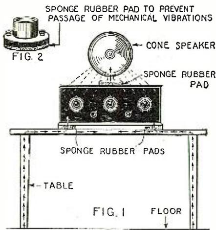
Vibrations from the floor, or from the loud speaker in operation, are often sufficient to affect the tubes and produce a ringing noise. The use of rubber pads will usually curb it.
