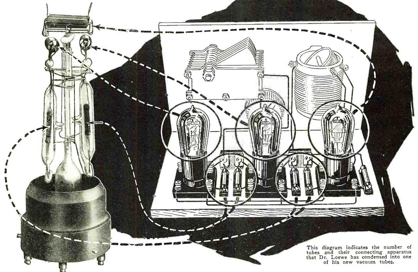
This diagram indicates the number of tubes and their connecting apparatus that Dr. Loewe has condensed into one of his new vacuum tubes.
