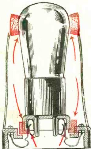
Showing double absorber for detector tube protection.
