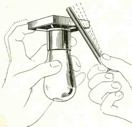
This experiment proves why B-T absorbers improve reception. Tap the base of the ordinary spring-suspended socket and feel the vibrations. Then touch the base with finger and feel them disappear. Vibrations never have a chance to start with the B-T method.
