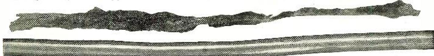
A photograph of two sections of solid aerial wire subjected to extreme climatic conditions. It is clear that the upper wire had no protective coating. One should not expect such damage under normal conditions; but it goes to show what corrosion the atmosphere can effect on metallic objects.
