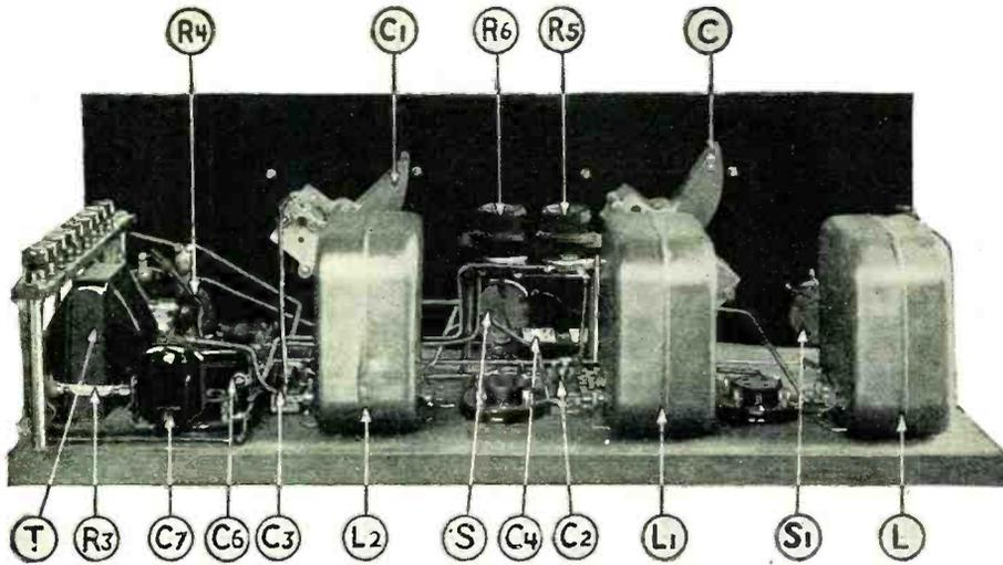
A rear view of the completed set. R5 and R6 are the rheostats controlling the detector tube and the three audio-frequency amplifier tubes. After being once correctly adjusted they need not be touched again. R3 and C7 are the grid leak and grid condenser, respectively. The detector tube socket is directly behind C7. C4 is a radio-frequency by-pass condenser.
