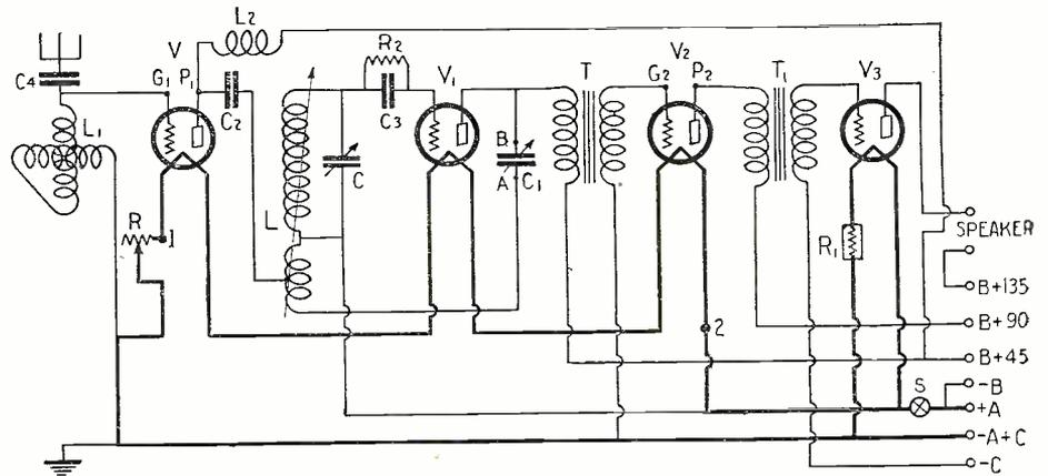
The schematic wiring diagram of the DX-2 receiver. V, V1 and V2 are contained in tube A, above illustrated. 1 and 2 mark the filament terminals.
