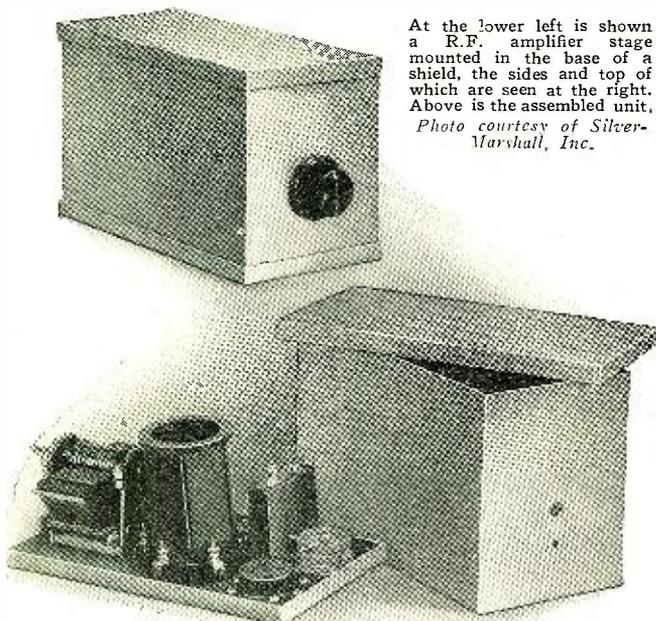
At the lower left is shown a R.F. amplifier stage mounted in the base of a shield, the sides and top of which are seen at the right. Above is the assembled unit. Photo courtesy of Silver-Marshall, Inc.
