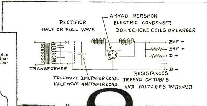
Circuit for building B eliminator using a Mershon Condenser as principle capacity.
