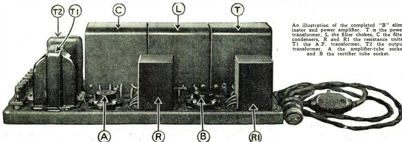
An illustration of the completed "B" eliminator and power amplifier. T is the power transformer, L the filter chokes, C the filter condensers, R and R1 the resistance units, T1 the A.F. transformer, T2 the output transformer. A the amplifier-tube socket and B the rectifier tube socket.
