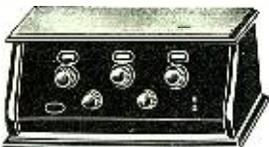
Mass., employs two stages of tuned radio frequency, detector and three of impedance-coupled audio; it tunes very sharp and the reproduction of speech and music is very efficient. It can be equipped for power operation.
