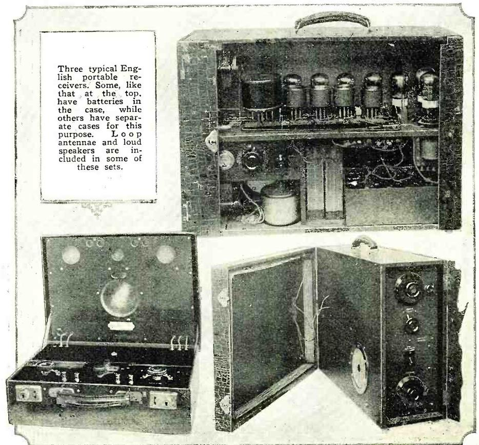
Three typical English portable receivers. Some, like that at the top, have batteries in the case, while others have separate cases for this purpose. Loop antennae and loud speakers are included in some of these sets.
