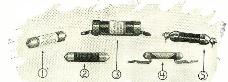
Fig. 10. A group of heavy-duty resistors which are employed principally as voltage adjusters in D.C. and A.C. "B" eliminators, but are useful also as current-by-pass and current-shunt units. Nos. 1 and 2 employ a carbon compound as the resistance; 3 is a lavite resistance unit. The resistance shown at 4 is made of carborundum; No. 5 is formed of a graphite compound which is fused into glass.
