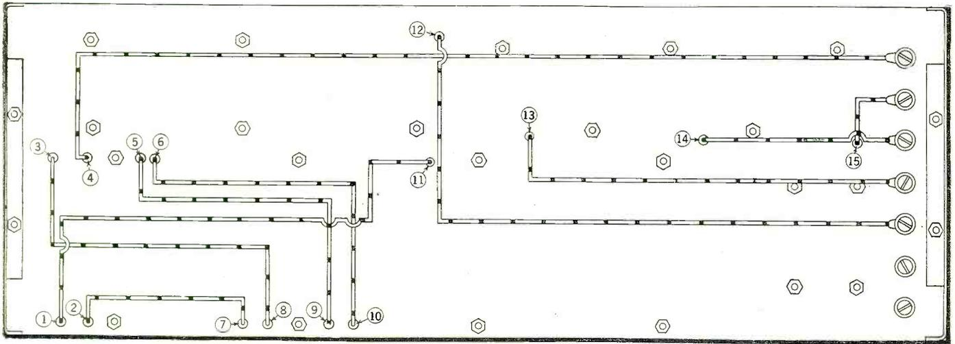
Below is shown the constructional layout of the panel for the receiver. All the necessary dimensions are given. The constructional layouts for both sub-bases, as well as the drilling layouts, are given on the opposite page. In all the illustrations and sketches the apparatus is similarly marked.
