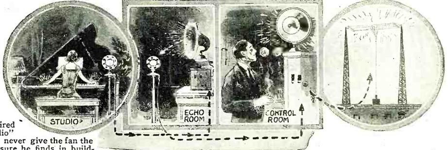
Station 2LO, London, has an "echo room," which is bare of the usual heavy studio drapery. Here a loud speaker reproduces the program, and a microphone collects the reverberations and adds them to the modulation of the music. This effect is never used with the voice of a speaker.
