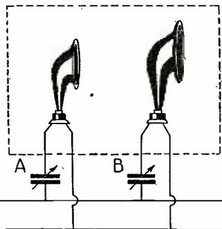
Better reproduction can be had by using two loud speakers, connected in parallel, and tuned by high-capacity condensers.
