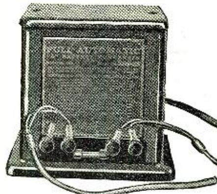
The complete automatic "A" battery charger. It is about seven inches high, five wide and four deep, and is made almost entirely of steel. Illustrations courtesy Apco Mfg. Co.
