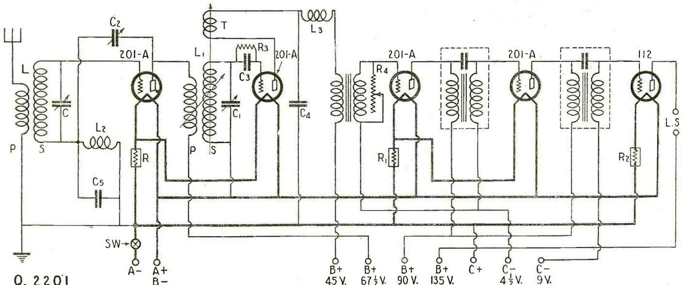
The circuit employed followed in the wiring of the Samson Dual T.C. receiver consists of a stage of neutralized R.F. amplification, a regenerative detector, one stage of transformer coupled audio frequency amplification and two stages of a new, improved type of audio amplifier.
