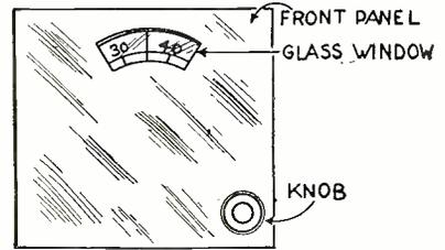
Details of the panel window showing location of vernier knob.
