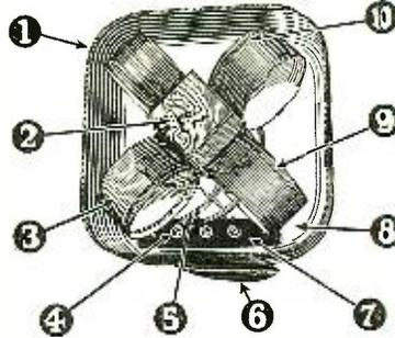
1. A scientifically designed shield against impact reception and electrostatic coupling. Heavy drawn copper, handsomely finished in natural copper lacquer, trimmed in gold.
