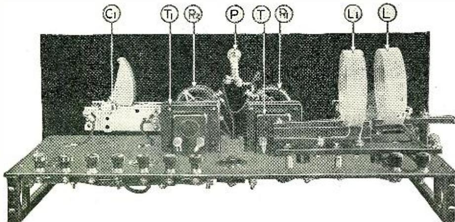
A rear view of the receiver. C1 is the condenser controlling regeneration; T and T1 are the A.F. transformers; R1 and R2, rheostats; P is the pilot light, and L and Li, the "wound-on-air" inductances, are the antenna coil, and secondary with fixed tickler, respectively.
