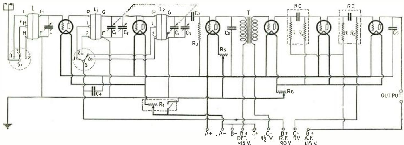
The complete schematic wiring diagram of the Quadraformer VI. Receiver. Note that the switch S controls both the R.F. transformers at once. Switch S1 controls the aerial coupler. The combination rheostat and filament switch is shown at R4.
