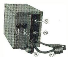
Front view of power unit: SW2, 110volt snap switch; H, fuse-block housing; A and B, plate-voltage rheostats.
