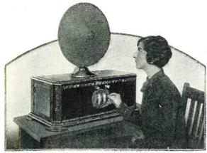
At the left is a view of the AC.-operated Ultradyne, mounted in an attractive walnut cabinet. The drum dial is the wavelength control, the knob at the left the volume control, and the other a sensitivity adjustment.
