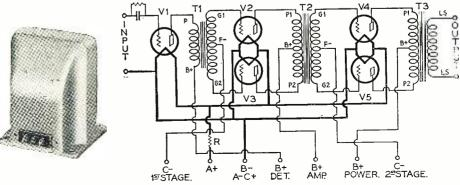
The unit illustrated on the left is a new-type push-pull transformer with center-tapped primary and secondary windings. It makes possible the use of the amplifier circuit shown.
