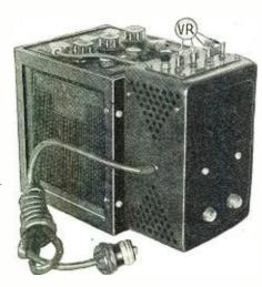
External appearance of the "A" power unit: the four posts marked VR are for regulating the rate of charge which the battery receives.
