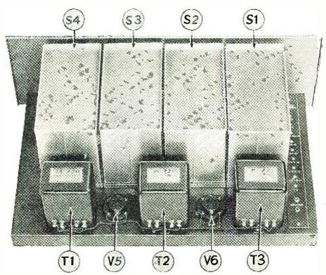
View of receiver with shielding compartments in place. S1, S2 and S3 are the first, second and third R.F. stages, respectively; S4, detector stage; T1 and T2, audio transformers; T3, output transformer; V5 and V6, audio-stage sockets.
