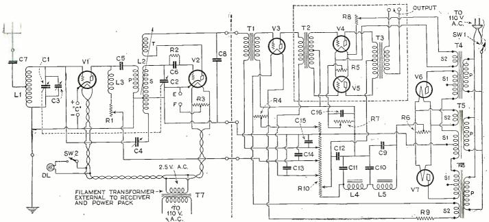
The complete schematic wiring diagram of the new two-tube Browning Drake receiver is shown at the left of the dotted line in the above illustration. The apparatus and wiring on the right of the dotted line is a power amplifier and plate-supply unit.
