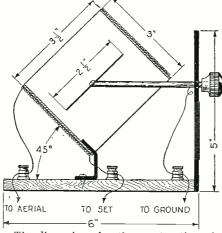
The dimensions for the construction of this home-made wave trap are given above.
