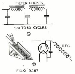
⑻ The purpose of a choke-coil-and-condenser system is to provide paths which offer different impedances to different frequencies, and therefore direct them almost entirely into different circuits. At A the choke is used to keep R.F. impulses from A.F. circuits, at B to separate the direct plate current from the A.F., at C to suppress the A.C. hum. In D a mechanical analogy to the electrical filter is shown.
