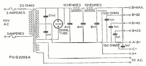
The circuit of an "A, B and C" power unit using a 350-milliampere tube is indicated here. The 500-ohm resistor between the "B" positive and "A" positive should be able to dissipate at least 250 milliamperes.
