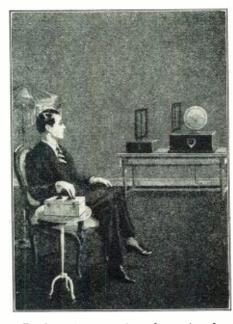
The loops in the station selector (on the small table) are concealed within the box; the left-hand cabinet on the table contains the band amplifier; and the fixed-frequency receiver is on the right.
