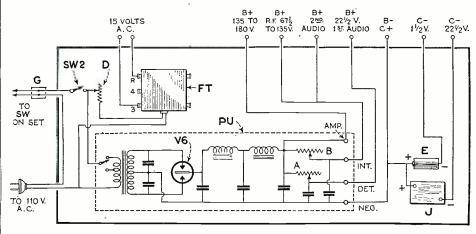
The schematic diagram of the power unit specially designed for use with the Electrified Peridyne.
