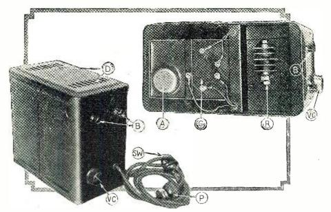
Two views of a new power unit which delivers 3 amperes at a potential of 6 volts. This device uses a dry electrolytic rectifier R, and an electrolytic condenser (C), and a heavy-duty choke as a filter.
