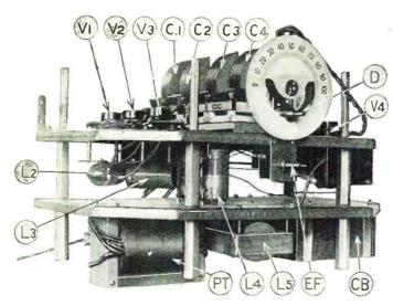
The four-gang condenser unit and the six tube sockets are the only parts mounted above the chassis.
