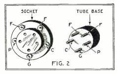
Diagram shows arrangement of terminals on a standard UY socket and tube base of the type used for a batterycable plug.
