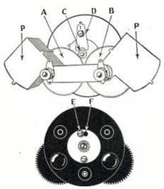
New twin rotor condenser, which may be adjusted for either a clockwise or a counter-clockwise reading.
