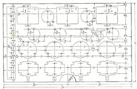
All holes required for mounting apparatus on the metal chassis of the receiver are shown with the correct measurements, in the above drawing. All holes required for passing wires through the chassis are also shown, and the position of the various parts is indicated in dotted lines.
