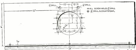
Above, details for drilling the front and sub-base panels of the receiver; the large hole for the drum dial may be cut by drilling around the circumference of the circle.
