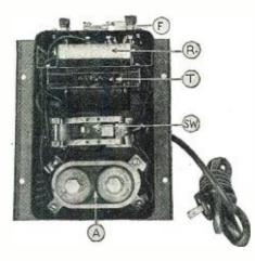
Arrangement of apparatus inside the power unit: A, rectifier unit; F, fuse; R, resistor; Sw, relay switch; T, transformer.
