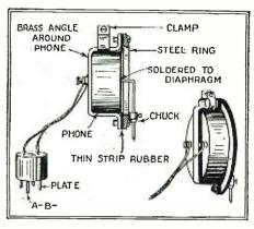
An electric phonograph pick-up unit may be made of an old sound box and a loud-speaker unit as shown.
