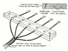
Complete details for building an inexpensive battery-cable separator are given in the above drawing.
