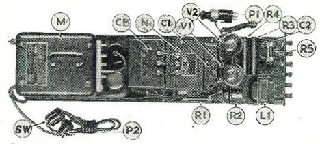
R1, 1,000-ohm resistor; R2, variable resistor; R3 and R4, 10,000-ohm resistors; R5, 100-ohm resistor; C2, 0.5-mf. by-pass condenser.
