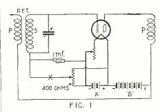
A potentiometer may be shunted across the "A" battery, with its arm connected to the grid, for preventing oscillations.
