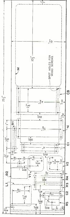
How the apparatus is located on the baseboard with drilling instructions given for a sub-panel if one is used.
