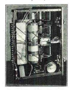
The rear view of the radio receiver, showing in the lower right corner the motor for driving the condensers.
