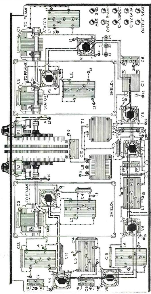
tracing on a piece of paper a full-size template, which later can be applied on the panel. The ready-made full-size drawings, which are available to set builders, may also be used. Each of the holes should be marked accurately with a center punch and drilled. Many of the holes in the drilling layout are for the wires which run from the various parts to the binding post under the sub-base panel. The position of all the parts is shown exactly in the drawings.
