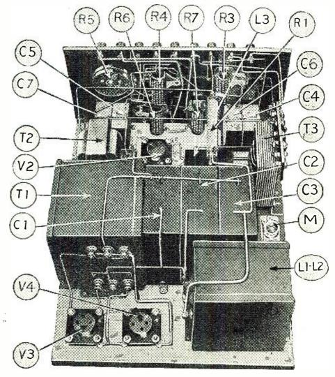
General view of power unit showing arrangement of apparatus on the baseboard. The letters correspond to those in the circuit diagram above and the list on page 965.
