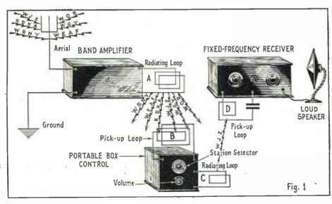
Signals from all stations within the receiver's range are amplified in the band amplifier, and the one to which it is desired to listen is tuned in by the station selector and transmitted on a new wavelength to the fixed-frequency receiver.
