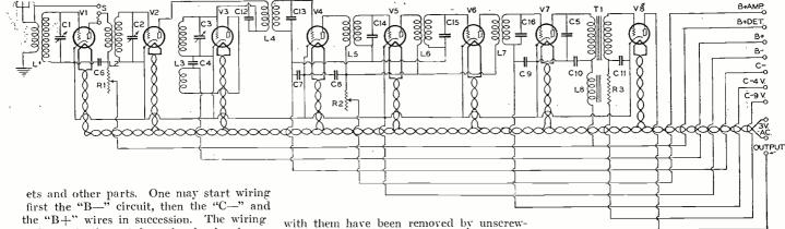
the "B+" wires in succession. The wiring underneath the sub-base is clearly shown and requires no further explanation. Needless to say, all the connections should be carefully soldered to make good contact and to avoid trouble in reception when the set is completed. This necessitates the use of a good soldering iron, some flux and good solder to make the proper connection. Rosin-core solder is recommended for this work.
