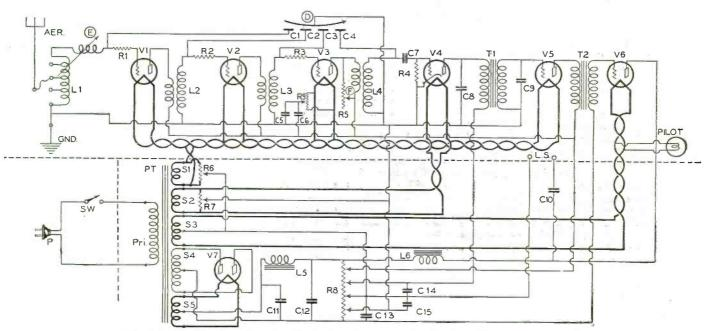
The complete circuit of the six-tube electrified receiver described on this page; parts and wiring shown below the line are in the power-supply circuit.
