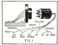
The method of mounting and wiring a home-made battery cable plug is clearly shown above.
