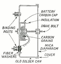
Fig. 1: Method of mounting the battery cap on the back of the can.
