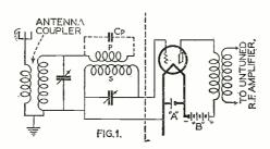
The fundamental tuning unit of the Somersalo system. The primary P is an open winding.
