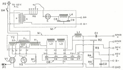
The circuit diagram of the socket-power unit and power amplifier, the components of which are named in the list of parts below.
