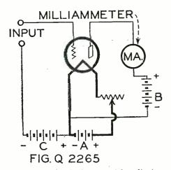
The circuit of a simple vacuum-tube voltmeter is shown. The milliammeter used should have a scale reading from 0 to  $1\frac{1}{2}$  milliamperes.
