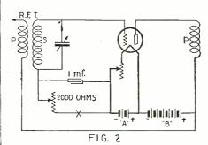
A variable high resistor may be substituted for the potentiometer with satisfactory results.
