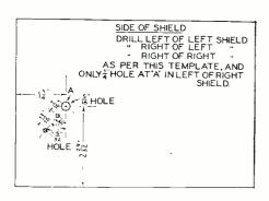
The above drawing shows the exact position for the condenser mounting holes in the shields.
