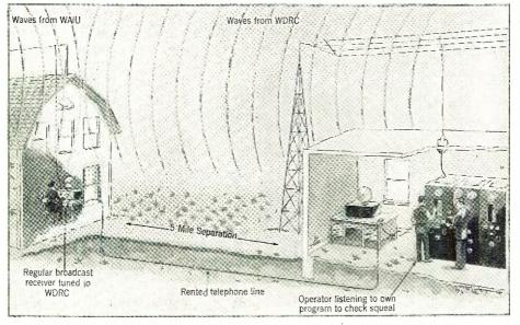
The operator at the broadcast station is thus enabled to determine if there is interference of his station's carrier with that of any other; and correct it accordingly.
