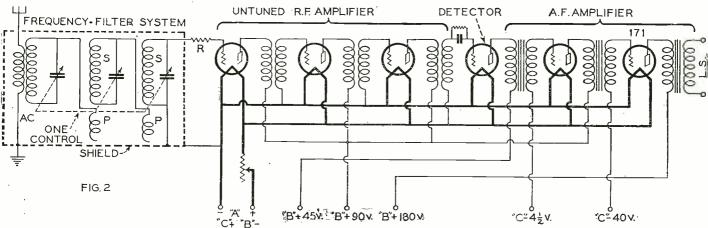
Schematic diagram of a receiver employing a Somersalo triple tuning unit; and untuned R.F. amplification. The open pri-
