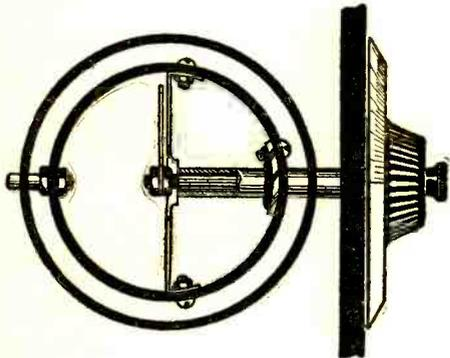
A clever arrangement in the way of Verniers. This can be mounted within the rotor of a vario-coupler or variometer.
