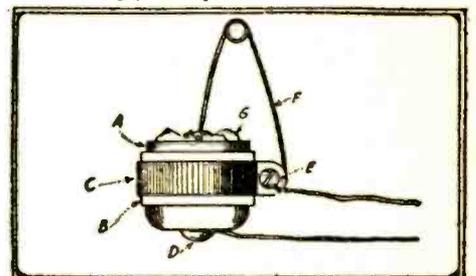
A real silicon detector, using a safety pin for simplicity.
