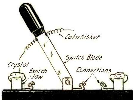
This is a clever idea. A single pole double throw switch is converted into a double crystal detector in the simple manner shown.
