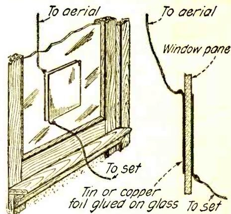
A clever stunt in the form of an aerial lead-in. The metal sheets to which the wires are connected act as a condenser.
