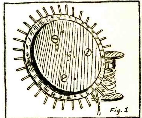
The two wooden discs grip the nails firmly while winding.
