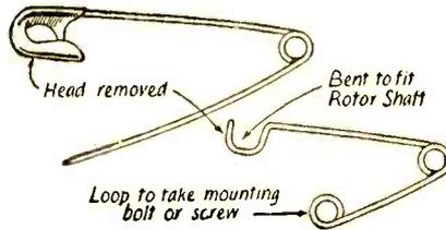
A variometer contact brush made from a safety pin. This affords a good wiping contact.
