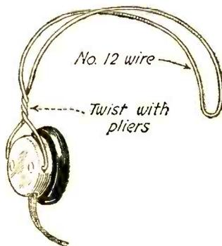
When an extra head-band is needed, it can be made in a few minutes with heavy wire.
