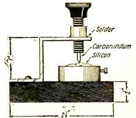
This combination of carborundum and silicon makes a very stable detector.
