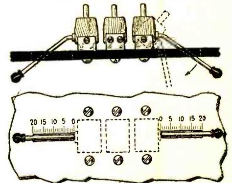
This illustrates the clever arrangement of the three-coil honeycomb mounting on the rear of a panel, with the controls on the front.
