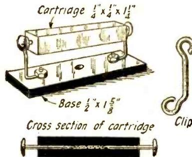
A cartridge form of fixed crystal detector especially adaptable to reflex receivers.
