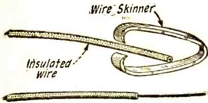
An excellent wire skinner made from a thick piece of spring brass.
