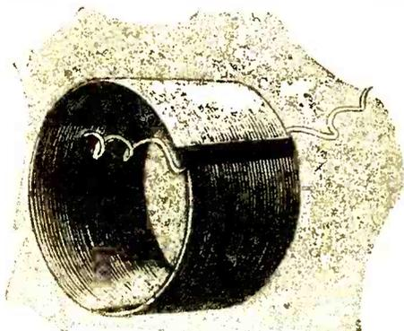
An efficient form of inductance. The coil is space wound and is self-supporting.
