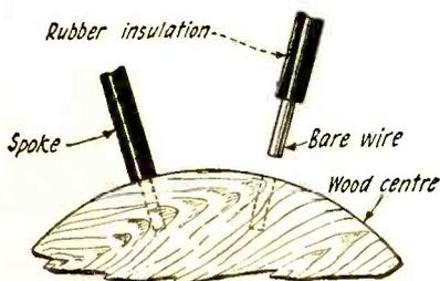
Rubber insulated wire is used for the spokes of this spider-web form.
