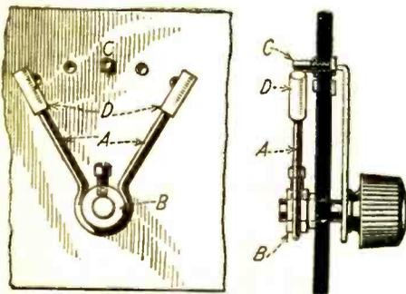
This switch stop is easily made from ordinary bus-bar.
