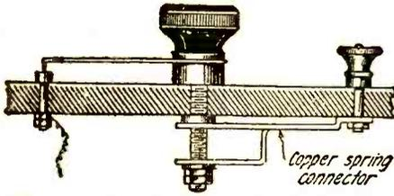
Permanent contact is maintained with this type of switch. The piece of bent copper connects the center of the switch to the binding post.
