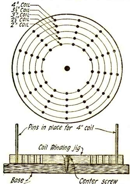
When holes are drilled, as indicated, and pins inserted in any set of holes, an excellent winding jig is produced.
