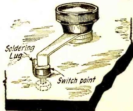
A simple switch stop made of a soldering lug fastened under the switch point.
