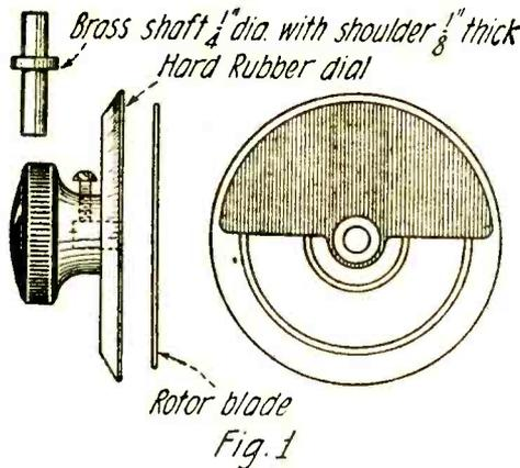
Showing the method of mounting the rotary plate on the dial. This is accomplished by a brass shaft with a shoulder.
