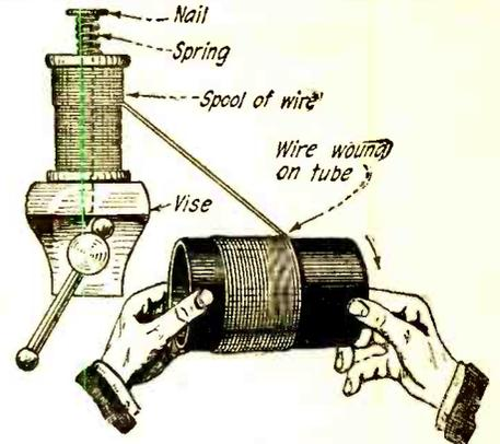
The spring and nail serve to keep the wire taut while winding a coil.
