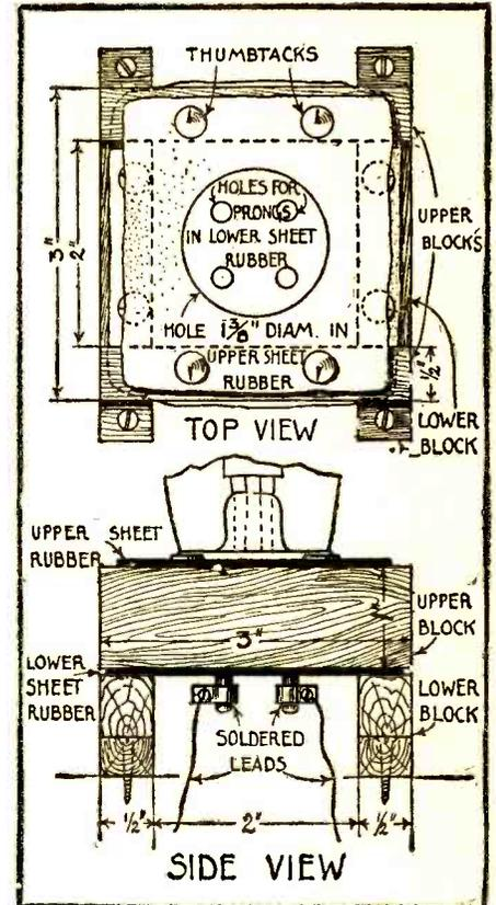
A vibrationless vacuum tube socket made from spare parts. To avoid losses, the connections are soldered directly to the tube prongs.
