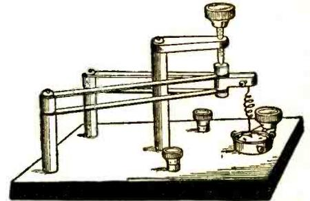
A very stable and serviceable type of crystal detector stand. The arrangement prevents the possible jarring out of a sensitive point.
