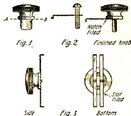
Another solution for the high cost of radio apparatus. We have found how to secure panels and B batteries from the old storage batteries. Now we can make knobs from the caps on the same battery.
