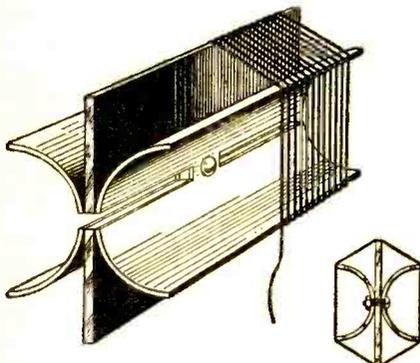
A low-loss coil form made from hard rubber tubing and a panel.
