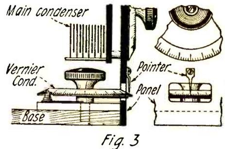
Method of mounting the novel vernier condenser. It is adjusted from the front of the panel by the thumb or forefinger.
