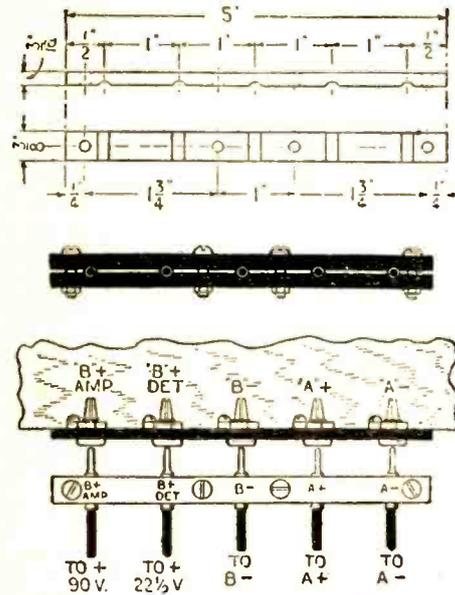
A battery connector that will save many minutes of sorting and connecting wires.
