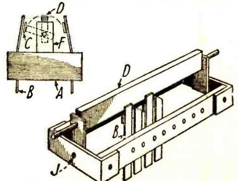
An easily constructed switch that will serve any number of purposes. It has the advantage of all contacts being stationary.
