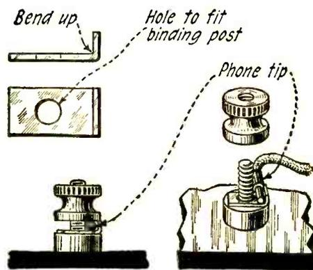
For loose binding post connections.
