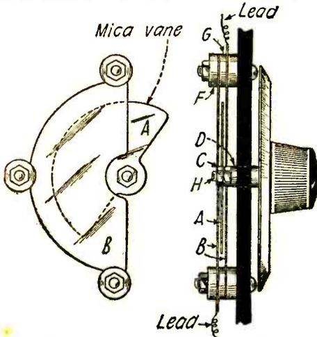
A rear and side view of the mica vane vernier condenser. The movable member changes the dielectric between the two stationary plates, thus increasing or decreasing the capacity very gradually.
