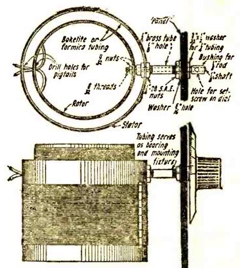
A neat method for mounting a variometer or variocoupler. Only one hole is drilled in the panel.
