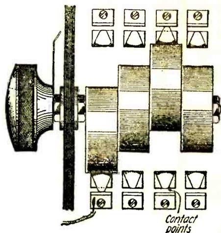
Here is an easily constructed panel switch that will serve many purposes. It is a good substitute for jacks.
