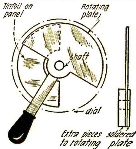
This vernier attachment is mounted directly behind the knob and dial and is adjusted by means of the insulating knob.
