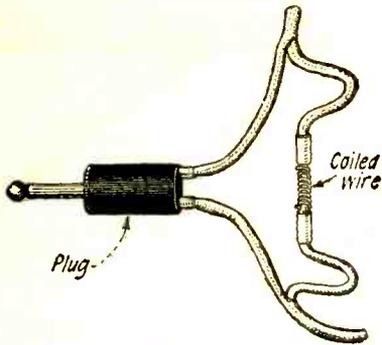
An emergency phone tip connector can be made from a piece of wire, coiled tightly.
