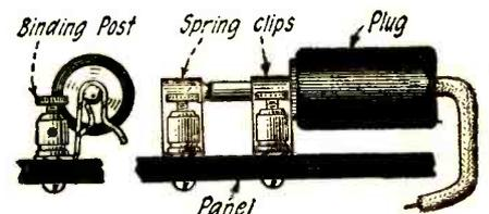
A simple jack made from two Fahnestock clips attached directly to the phone binding posts.
