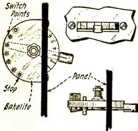
A switch of this type is a great space saver and has a pleasing appearance as well. The switch points are mounted underneath the piece of insulation so that dust cannot collect upon their surfaces.
