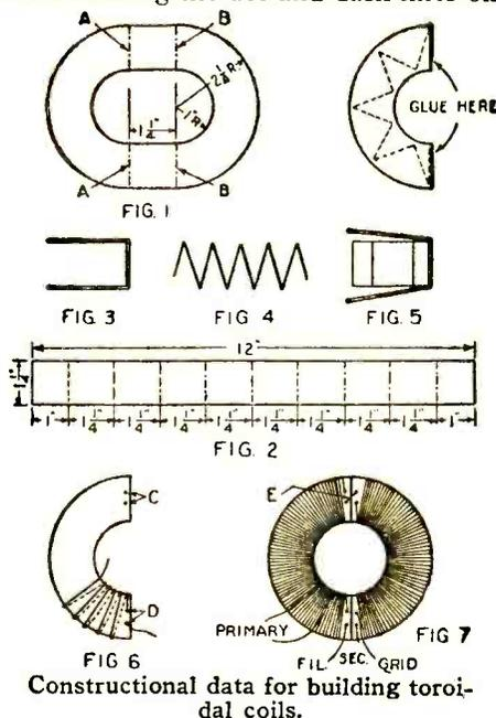
alternate sides and bent into the shape as shown at Fig. 4. Punch two small holes in one side of each end of each form, as shown at C and D, Fig. 5. These holes are used to retain the ends of the windings.
