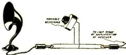
By the use of two plugs and jacks and a variable resistance connected, as shown above, in the output of a radio receiver, the volume of the signals received may be varied to any intensity desired by varying the amount of resistance.
