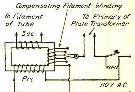
Use this scheme to prevent a drop in voltage on the filament when transmitting.
