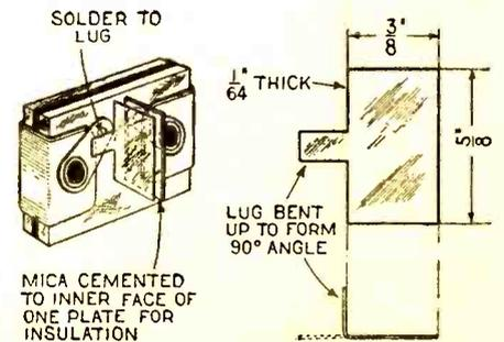
An auxiliary condenser useful for equalizing capacities.
