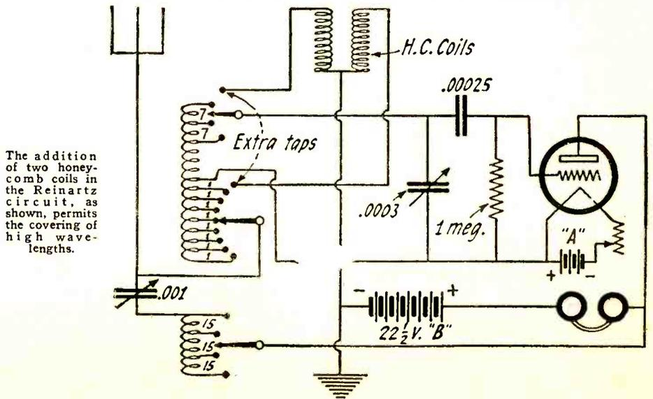
The addition of two honeycomb coils in the Reinartz circuit, as shown, permits the covering of high wavelengths.
