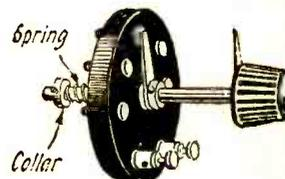
A clever design in back-of-panel switches. It is made from a discarded rheostat.
