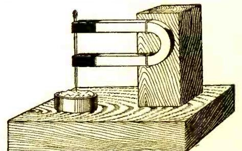
Here is a clever arrangement in the way of crystal detector. The horseshoe magnet holds the needle in any desired position.
