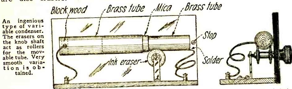
An ingenious type of variable condenser. The erasers on the knob shaft act as rollers for the movable tube. Very smooth variation is obtained.
