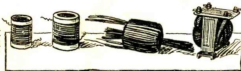
Insert a length of cardboard or fibre tubing in the core space as added protection to the primary winding.
