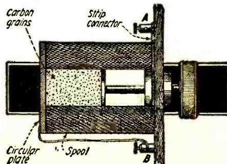
Here is a rheostat for that critical detector tube. It is not difficult to make.
