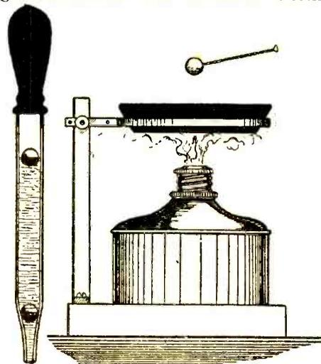
Small balls made of cork and sealing wax can be used for hydrometer floats.
