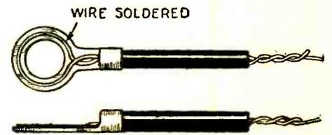
A strong connection can be made if the lugs are soldered to thin wires in this manner.
