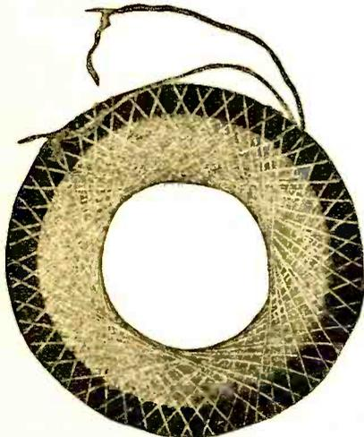
Showing the appearance of a complete short wave inductance coil. The wire is wound on a circular framework of insulating material.
