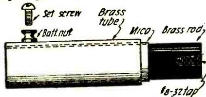
A very good idea in the way of variable grid condensers. The brass rod is threaded so that the condenser can be screwed directly onto the grid post on the tube socket.
