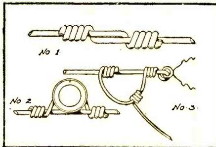
Showing three good ways of splicing wires.
