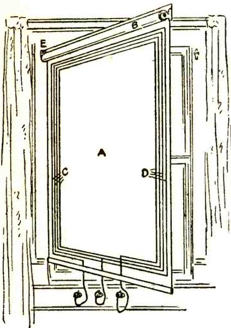
Wind your loop aerial on the shade and save space. It is easily done and if flexible wire is used the shade can be rolled up.
