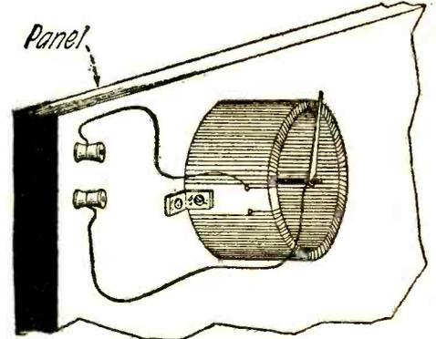
An easily constructed tuning coil for panel mounting. A switch arm replaces the usual slider.
