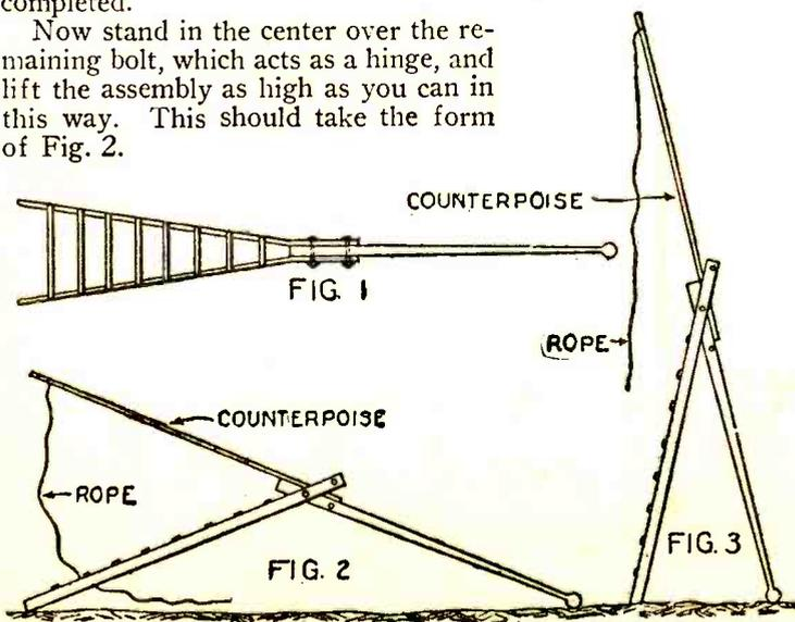
Now take the top of the mast, which is resting on the ground, and carry it toward the base until it is almost straight up. Place the end of the mast on the ground and guy the base with temporary stays in this position. You now have the top of the mast and the temporary counterpoise balanced as in Fig. 3.
