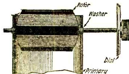
A snug fitting bearing is easily made by winding wire into a tight coil to fit the rotor shaft.
