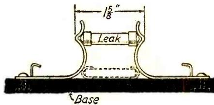
Spring connection clips are employed to make this grid leak and condenser holder.
