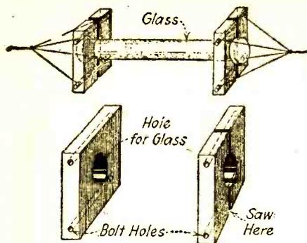
A good antenna insulator can be made with two blocks of wood and a glass towel rack.
