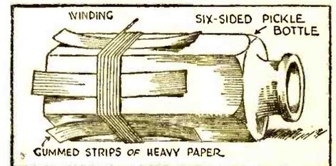
Method employed for winding the low-loss coil. The coil is secured by the gummed tape.
