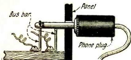
A simple single circuit jack made from bus bar wire.
