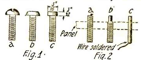
Various sizes and types of switch points can be made from ordinary round-head machine screws.
