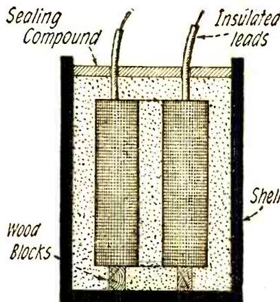
A transformer with a closed core composed of powdered iron. This helps to simplify the matter of construction.
