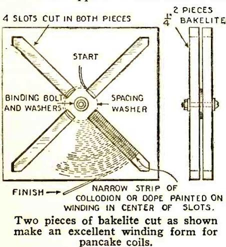
coil a thin coating of collodion or other "dope" for holding the turns in place. The result will be a coil that is wound on air and having as great an efficiency as many others that are much more difficult of construction.
