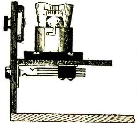
holes are drilled in the shelf. The jack may either be tapped or a bolt passed through. This not only adds to the compactness of the set but also simplifies the wiring somewhat. The sketch is practically self-explanatory, but only shows one jack. This process is repeated on the other two, forming a very firm mounting for the V.T. shelf.
