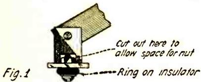
A simple method of improving the efficiency of a lightning switch.
