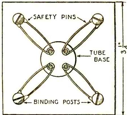
Four safety-pins, four bolts and a  $3\frac{1}{4}$ -inch square of bakelite make an efficient socket.
