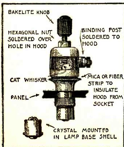
An excellent dust-proof crystal detector made from the parts of a cowl lamp.
