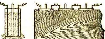
Single cell and complete battery of 22½ volts
