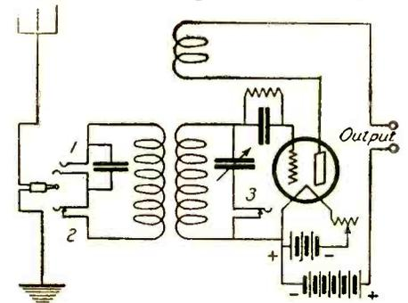
A clever jack arrangement for different circuits.
