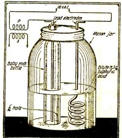
A Mason jar, a baby's milk bottle, a strip of lead and a diluted solution of sulfuric acid, and presto! You have an electrolytic interrupter. Be sure to bore an air vent on cover of jar.
