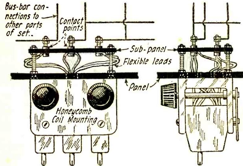
The constructional details of the honeycomb sub-panel are clearly shown here.
