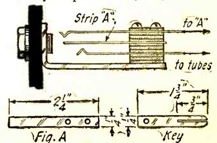
This filament switch requires a special key-plug to close the circuit. Other plugs will not fit the jack.
