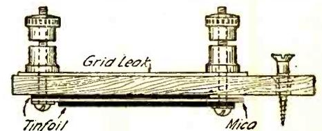
A grid condenser and grid leak are easily made in one unit.
