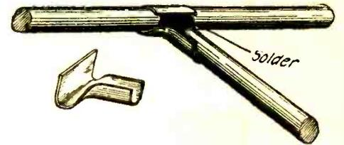
Connecting lugs made in the manner shown are very useful where difficult soldering jobs are encountered.
