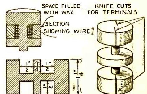
By placing the turns of a transformer on a candle cut as shown above, a simple and inexpensive coupling device will be constructed.
