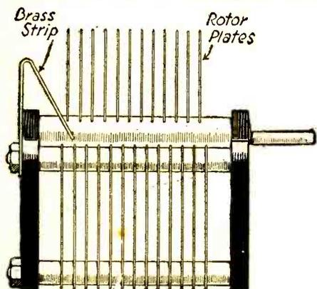
The condenser is shorted when the rotor plates come in contact with the brass strip.
