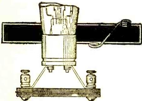
With four binding posts and some stiff wire a support may be made for the W. D. tubes as well as for the other types.
