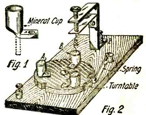
A three-cup crystal detector. The cups are made from wire lugs. The mounting table turns, thus affording selection.
