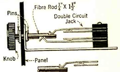
An easily constructed double pole quick acting switch.
