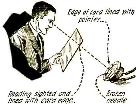
A good way of reading a meter that has a broken needle.
