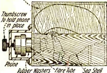
A very good loud speaker made out of a large sea shell. It is conveniently mounted in a cabinet.
