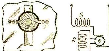
Fig. 2. A section of the commutator arrangement and the two brushes, showing how the coils are connected to it.
