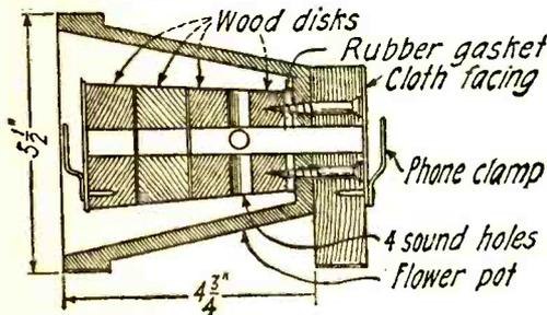
where shown. Assemble these. Glue a woolen cloth phone gasket at each end of speaker. Glue three pieces of cloth for the feet, where shown. Paint with auto enamel.
