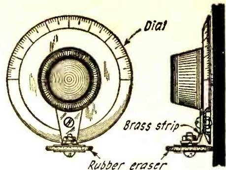
A sidewise movement of the thumb on the eraser affords a very fine adjustment of the position of the dial.
