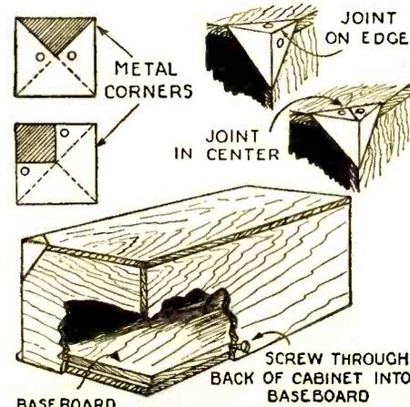
**The use of metal corners to hold panel to cabinet eliminates any need for screws.**
