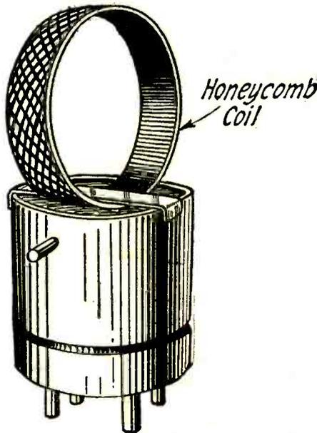
A changeable mounting can be easily made by mounting a coil on a discarded electron tube base.
