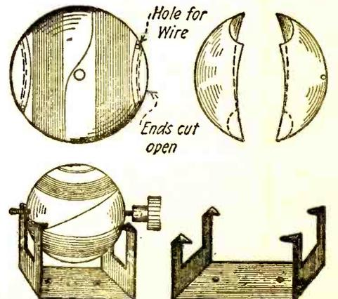
A simple variometer can be made from two paper toy balls. The total cost of this variometer is about twenty-five cents.
