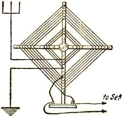
Here is a good stunt. The extra winding on the inside of the loop frame functions as an untuned antenna circuit.
