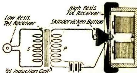
This amplifier is simple to make, it consists of a microphone button mounted on the diaphragm of a high resistance telephone receiver with a local circuit.
