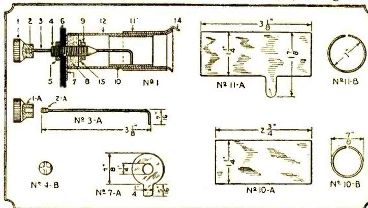
On the left is a detailed drawing of the parts for the vernier condenser that is described above. The glass tube, inside of which slides one of the tubular plates, is the dielectric of the condenser. Each figure is explained in the text.
