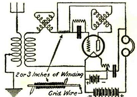
Two or three inches of winding on the grid wire will increase the wave-length.
