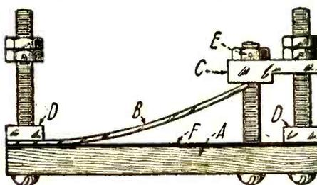
A variable grid leak that is free from wear. The spring strip "B" progressively shorts the high resistance "F" when pressed downward by the adjusting nut "E."
