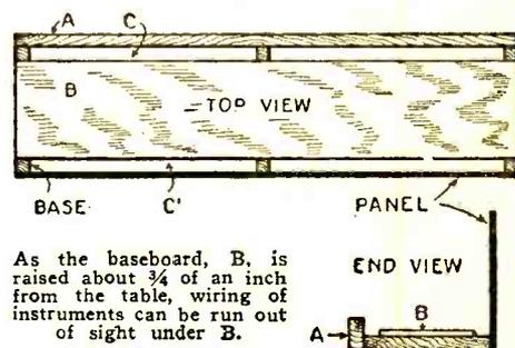
As the baseboard, B, is raised about ¾ of an inch from the table, wiring of instruments can be run out of sight under B.
