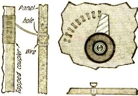
This scheme does away with the use of switch points. Loops of wire are used instead.
