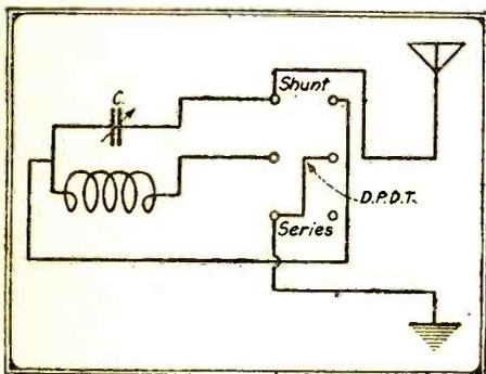
In this hook-up a double-pole double-throw switch affords a rapid means of placing the receiving condenser either in series or in parallel with the aerial and primary of loose coupler.
