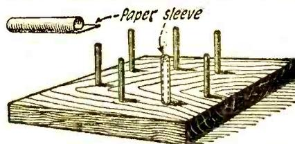
Paper sleeves slipped over the nails on a coil winding form make it easy to get the coil off when completed.
