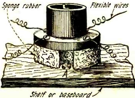
A mounting for a 199 tube made of sponge rubber will materially reduce microphonic tube noises.
