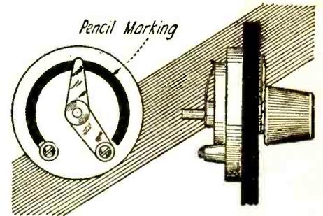
An old rheostat can be made into a variable grid leak by removing the resistance wire and making a pencil line on the fibre strip.
