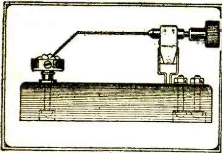
A crystal detector permitting ease of adjustment may be constructed as shown. Note the use of the magazine clasp.
