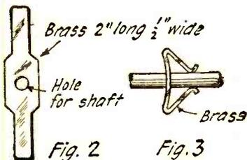
Details of the spring contact for variometers and variocouplers.
