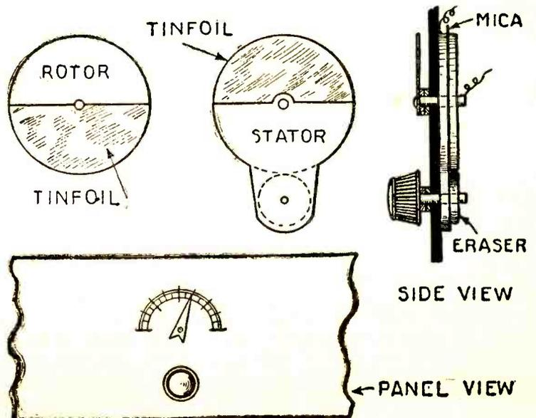
such a size as to fit the condenser and vernier shafts snugly. One half of the circle on this plate is also covered with tin or copper foil, except that a small space is left around the hole that the rotor shaft passes through. Now cut from a piece of mica, a disc slightly larger than the diameter of the condenser plates for a dielectric, which goes between the two plates and prevents shorting.
