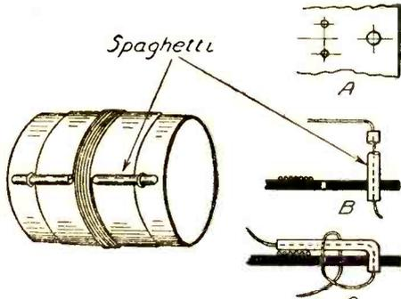
Method of securing the ends of narrow coils.
