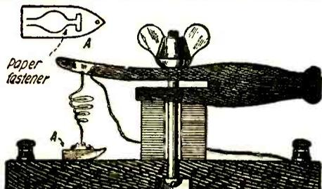
Here is a practical crystal detector stand, utilizing a clothes-pin as an adjusting arm.
