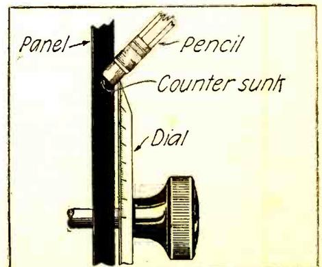
By twisting the pencil, the friction of the rubber against the periphery of the dial will turn it at a slow rate.
