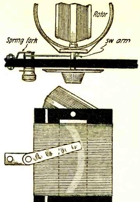
A very fine variation of inductance can be obtained by using this system, which is less complicated than the usual method.
