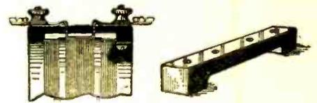
A good way to fasten the leads of the primary coil of an air core radio frequency transformer.
