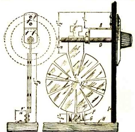
Details of the spider-web coil mounting. The coil forms can be made of any good insulating material.
