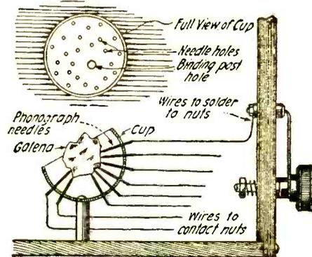
If one of the sensitive spots of this type of detector becomes dislodged another can be easily found by turning the switch lever.
