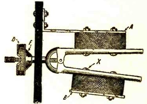
Here is a mighty clever scheme. A drawing compass is used to vary the coupling of unit inductance coils.
