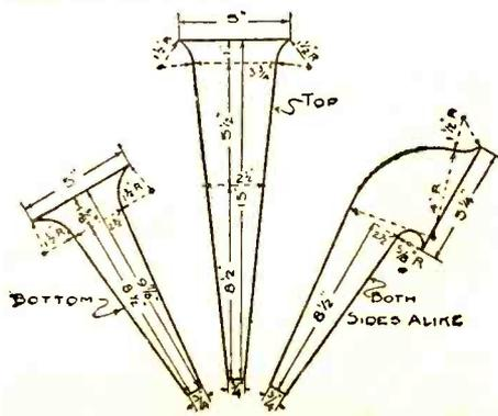
Accurate mechanical details are here given for the construction of the loud speaker.
