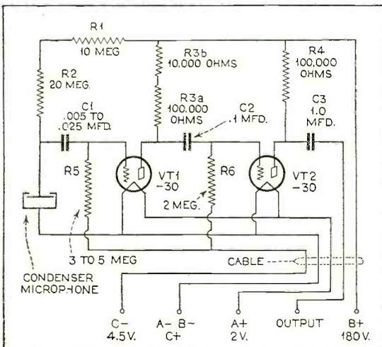
THE SCHEMATIC CIRCUIT DIAGRAM
