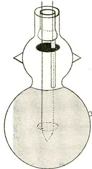
1. In combination, a light-sensitive device comprising a receptacle, a pair of electrodes mounted therein, one of said electrodes being capable of emitting electrons under the influence of light and a metal member mounted in said receptacle and coated with finely divided carbon.
