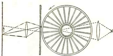
1. Scanning apparatus comprising an arc lamp, a rotary device carrying a plurality of separate light conducting rods positioned between said arc lamp and the subject or object to be scanned, means for concentrating and projecting the light from said lamp upon the inner ends of said rods in succession, and means for causing the light emerging from the outer ends of said rods to be imaged upon and to trace successive adjacent strips across the subject or object.
