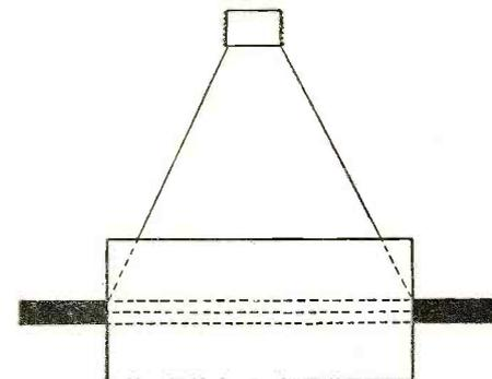
1. An acoustic device comprising a diaphragm sufficiently large to set up self-sustaining sound waves in free air, a cylindrical baffle member arranged co-axially with said diaphragm, said baffle member being positioned and arranged so that it surrounds the peripheral edge of said diaphragm and
