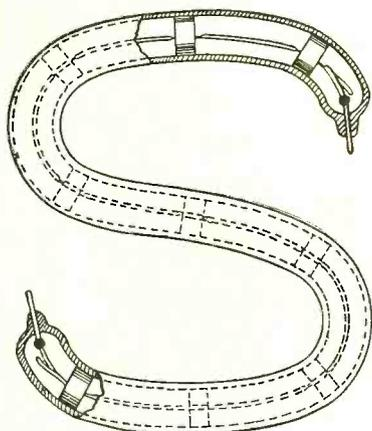
1. A glow lamp comprising a pair of wire electrodes, and insulating beads threaded upon said electrodes to maintain a substantially uniform spacing therebetween.
