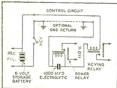
When the operating key is pushed down and held, the capacity across the power relay charges and furnishes current for holding the relay upon releasing the key. Operation may then be carried on in a regular manner, the keying relay following the dots and dashes of the key, and the power relay remaining closed unless the key is left up long enough.
