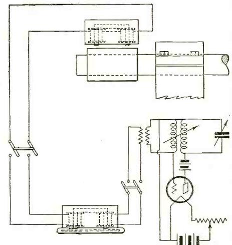
1. A magnetic and radioelectric goniometry device comprising a phasemeter, a stator of a multiphase generator creating an auxiliary field, a two-phase tetrapolar induction rotor in this field, an exploring element for the field in observation, said element and said rotor rotating together, and means to compare in said phasemeter the relative phases of the electromotive forces generated respectively in said rotor and in the exploring element.
