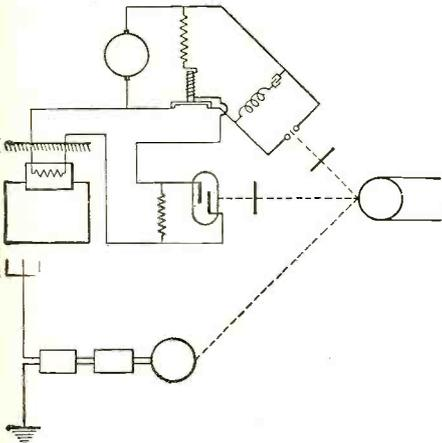
1. In combination with an electrical impulse receiving set, a condenser adapted to change in capacity in proportion to mechanical vibrations, a pair of tuned circuits, said condenser being connected in one of
