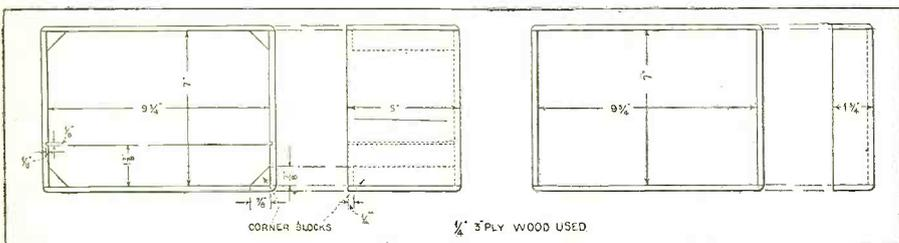
Figure 4. Specifications for the Carrying Case
