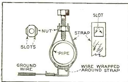
slotted with a hacksaw so that the slots are about one-half as deep as the nut is thick.
