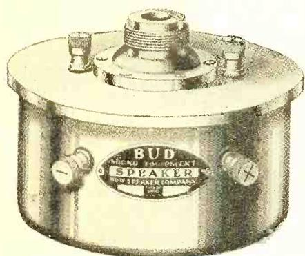
as to form its own core for the voice coil. This new design permits the operator to make a diaphragm or coil replacement in a few minutes. The impedance of the voice coil is 16 ohms and the field resistance 4 ohms. The voltage for the field coil is 6-8 volts d.c. at 1½ amperes, which is procurable from a storage battery or a specially designed Bud exciter unit. This loudspeaker unit will handle 25 watts input.
