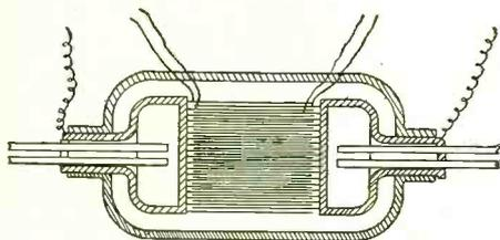
5. The combination of a containing vessel, condenser plates of conductive material supported in spaced relation within the vessel, the supporting means for the plates being adapted to convey a cooling medium to the condenser.
