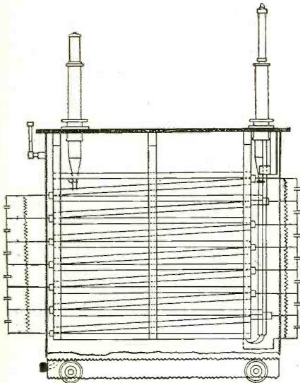
1. A high voltage rectifier comprising a plurality of sections disposed in zigzag fashion and immersed in a suitable insulating material, each section embodying plurality of elements of the copper oxide type electrically connected in zigzag fashion.
