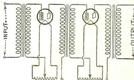
1. In an apparatus of the type described, the combination comprising a plurality of multi-electrode audions each including a control electrode, input and output circuits for each of said audions electrically associated to form an amplifier, means within the audion for dielectrically isolating the control electrodes of each audion to eliminate grid current flow, and means externally of the audions in the input circuits for dielectrically isolating the control electrodes.
