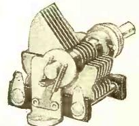
**SHORT-WAVE TUNING CONDENSER.** High capacity; wide range. Soldered brass plates. Rugged frame. Double four-point wiping contact. Isolantite insulation. Single and dual models; 20 to 325 mmf. per section.
