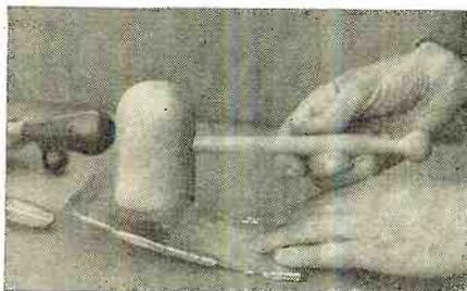
wood potato masher, which can be bought for ten cents. Cut the handle off and smooth up the round or top portion. Drill a hole an inch or so deep in the head and refit the handle as shown.
