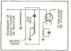
tions operating too close to the same frequency; also background noises of the receiver are greatly reduced. True some volume is sacrificed when the tone control is set for "deep" but this drop in volume is compensated for by clear signals.
