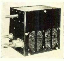
battery eliminator and dynamic type speaker are all housed in the one container. The set is tuned from an attractive instrument board control unit which is connected to the set by two flexible cables. This control unit is calibrated in kilocycles and the figures are large, therefore easily read. (Continued on page 121)
