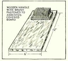
turned around when it is most needed. The broad asbestos surface of this support is hard to miss; and there is no danger of the hot iron burning through the layer of as-bestos. The bristles of the wire brush are excellent for cleaning off the tip of the soldering iron. A wipe of the iron on the brush each time it is used will remove the corrosion and keep the point clean and
