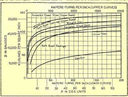
Fig. 2. "B-H" curves showing the relation between the magnetizing force H and the corresponding flux density B produced in various kinds of iron and steel. Fig. 3. Curves showing how the permeability of iron and steel varies when the magetic flux density is varied
