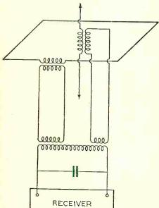
angles to each other, said antennæ being connected transmission lines with a joint radio-frequency circuit, one of said transmission lines being longer than the other by a length equivalent to one quarter of the communication wave whereby the oscillations of both antennæ are fed to said radio-frequency circuit with a 90° phase displacement.
