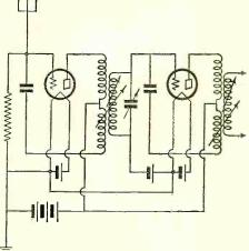
dary self-inductance, the mutual inductance and the ratio of secondary to mutual inductance of said transformer whereby the degree of amplification may be increased as the frequency to which the amplifier is tuned is decreased.
