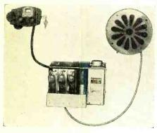
necessity of spark-plug suppressors. The set features convenience of installation, Class B amplification, automatic volume control and The following type tubes are used: two -6D6, one -6C6, one -37, one Wunderlich, one -79 and one BR type rectifier. The steering-column remote-control unit is of the gear-driven type.
