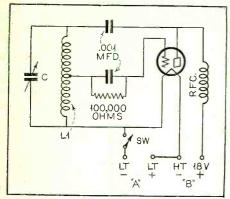
to the frequency range to be covered. audio pitch can be varied by substituting different values for the grid leak. Higher values will provide a lower note, while lower resistor values will raise the pitch.
