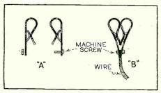
stripped two fahnestock clips from a discarded "B" battery, pressed the "faces" or spring sides together, as shown at "B" and held them in position by means of the machine screw.
