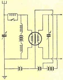
charge path between the anode and cathode and arranged to magnetically control the electron emission from said cathode, an input circuit including said coil connected directly in series therewith, and means for tuning the input circuit to establish current resonance in the control coil, said coil consisting substantially the entire inductance in the tuned input circuit.
