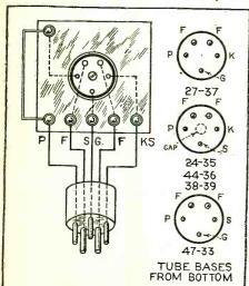
plainly marked. With all the terminals in a row on top, the filament, plate, or any of the grid voltages may be easily tested. opening, which may be shorted, is left in
