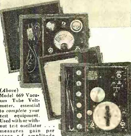
(Above) Model 669 Vacuum Tube Voltmeter, essential to complete your test equipment. Used with or without test oscillator . . . measures gain per stage, r.f. amplitude in oscillator circuit of superhets, makes all tests on AVC circuits, P.A. systems, and all measurements where high frequency is a factor. Direct reading . . . measures without guesswork or confusing adjustments. Price, \$45.00 net in U.S.A. (Carrying case extra.)
