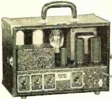
ploy the following type tubes: two 6F5's, one 6N7, and two 6L6's connected in push-pull in the output stage. It has input connection arrangements for 2 microphones and phonograph pick-up. The output impedance is 250 ohms.
