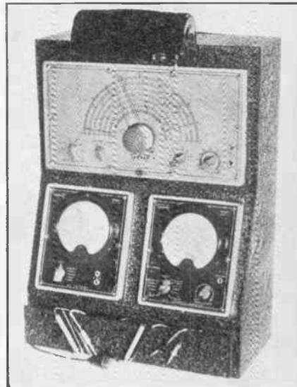
or more cabinets can be bolted together to form a continuous panel. There is a large drawer at the bottom for accessories. The measurements are: 22½ inches high by 16 inches wide by 7⅞ inches deep.
