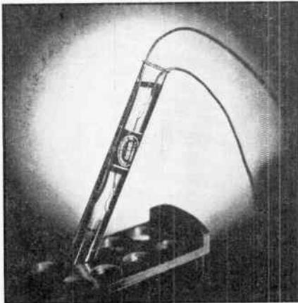
principal cause for failure of fixed condensers lies in the effect of humidity. In the "Glassmike" the condenser cartridge is contained in a glass tube, which is sealed with a special compound bearing the name of "Hillite." This compound adheres permanently to the walls of the tube preventing moisture seepage between it and the glass. The plates are tinfoil, not aluminum, and are contacted by flat helical pigtails which actually become part of the plates.
