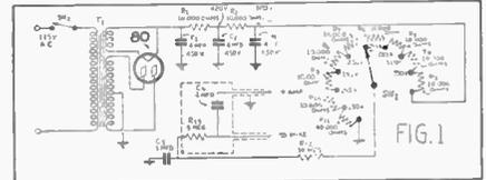
straightforward power supply employing resistance-capacity filtering. The tap switch affords a choice of 9 voltages. Lower voltages tend to accentuate low-frequency response while the higher voltage taps increase the "highs." By selecting the proper voltage, one may compensate in some degree for amplifier deficiencies.
