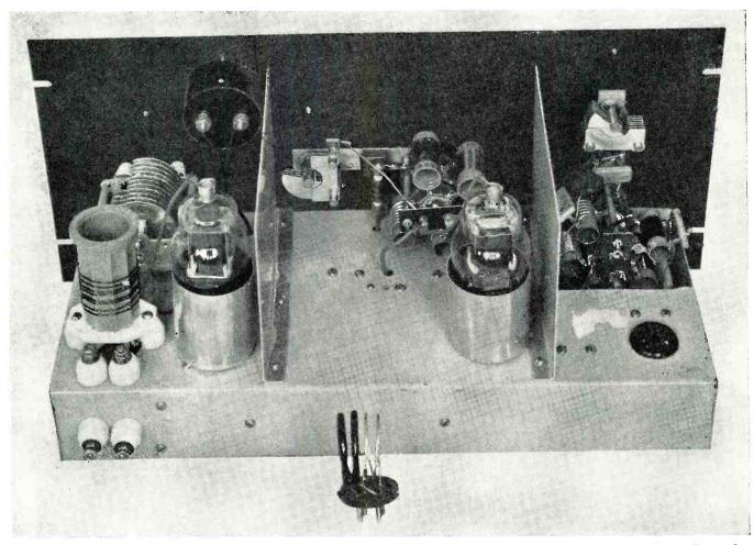
Rapid bandswitching plus the ability to shift frequency within any one band is provided for in this new unit.
