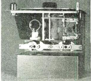
Main tuning condenser at the right, padding condenser to the back, insure proper connector lengths.
