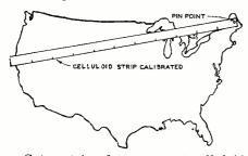
Cut a strip of transparent celluloid as long as the greatest distance across the map. One inch will be about right for the width. Then strike off points along the edge of the strip to correspond exactly with the scale of miles on the map. Scratch these in the celluloid with a sharp point and fill the scratches with black paint, wiping off the surplus. Mark these with numbers to show the number of miles that the scale length represents. Punch a pin hole at the exact zero mark.
