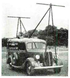
Using the old type flat-top antenna, this mobile broadcast unit gives f.b. results.
