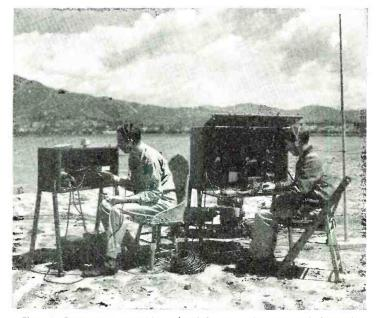
The Air Corps goes portable with u.h.f. Note the m-g, and the pedestalled antenna with single wire feed that can easily be set up.
