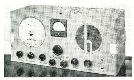
With conventional controls, the receiver is easy to tune, and bandspread is mechanical and continuous in operation.
