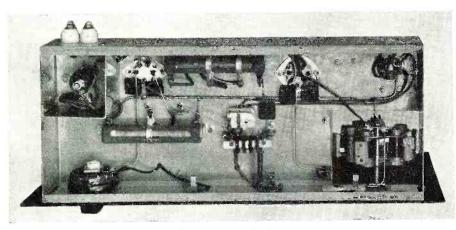
Note the extremely short leads and clean placement of parts.
