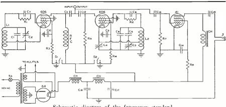
Schematic diagram of the frequency standard.
