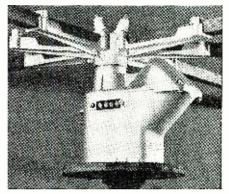
in a corrosion-proof aluminum alloy case which eliminates weather hazards and provides a small but strong power unit weighing only 17 pounds. The gears run in oil and main bearings are oilite metal and require no lubrication. The speed of rotation is 3/4 r.p.m.
