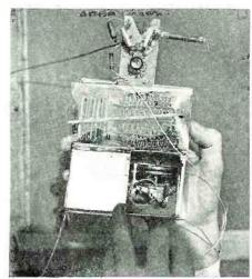
A I lb. transmitter costing \$30 which is used by the Weather Bureau for soundings.
