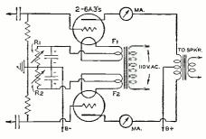
resistors,  $R_1$  and  $R_2$ , until the plate current of each tube is exactly the same under the same conditions. The adjustment should be made with a steady, fairly strong 400 cycle signal input to both grids.
