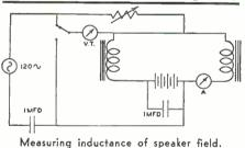
across the field and the voltage drop across the bias resistor, these values being 122.5 volts and 17 volts making a sum of 359.5 volts required at the rectifier tube socket. With a type 80 tube with four microfarads input condenser, and from data in the tube By LOUIS J. GAMACHE W9RGL
