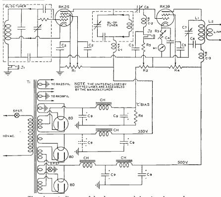
The schematic diagram of the electron-coupled exciter shows only one of each coil in circuit. The complete parts list is given below.
