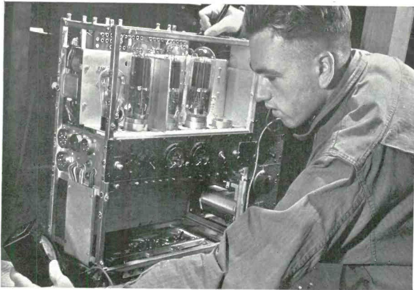
Radio transmitter test and repair by student at Signal Corps Training Center. Large tubes are 50-watters.
