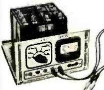
You make this MEASURING INSTRUMENT yourself early in the Course. Useful for practical Radio work on neighborhood Radios to pick up EXTRA spare time money. It is a vacuum tube voltmeter and multimeter, measures A. C., D. C. and R. F. volts, D. C. currents, Resistance, Receiver Output.
