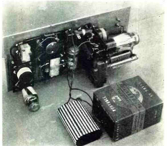
Interior view of chassis assembly showing location of various components. The unit is battery operated.
