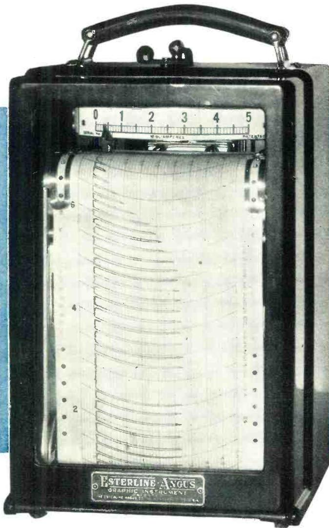
Fig. 1. Recorder employed in the Lie Detector used to plot variations in skin resistance and heart amplitude simultaneously.
