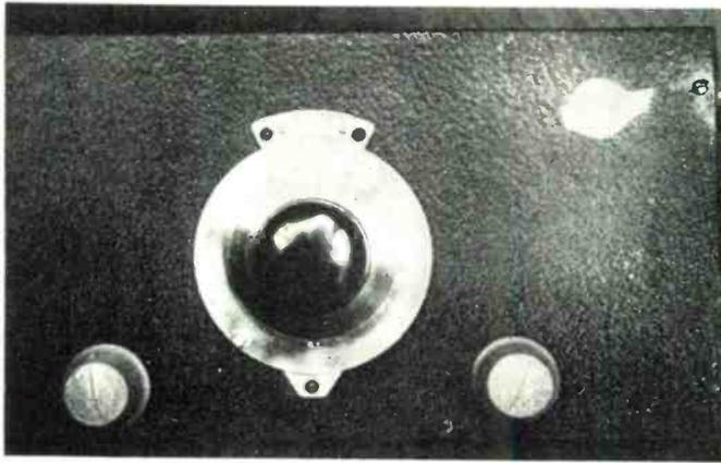
Precision tuning and logging is aided by using quality vernier dial.
