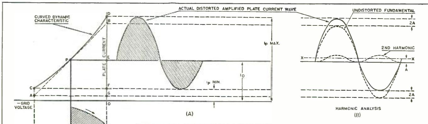
Fig. 2. Dynamic operating characteristic curve of a typical triode output tube used to illustrate the cause of harmonic distortion.
