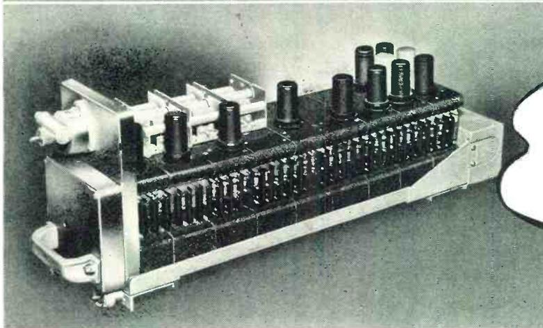
Unique and revolutionary methods have been developed by Harvey engineers for the production and assembly of communication receivers . . . which separate the circuits of the receivers into basic circuit-elements by the use of standardized R. F., I. F. and Audio cells that are complete self-contained circuits. Mass production is achieved by this method with important improvements in sensitivity and selectivity.
