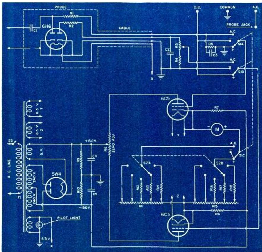
Fig. 2. Schematic diagram of the sensitive V.T.V.M.
