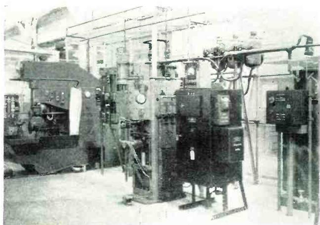
Resistance-welding area. General front view shows 200-kva. seam-welding machine and 75-kva. welding press.
