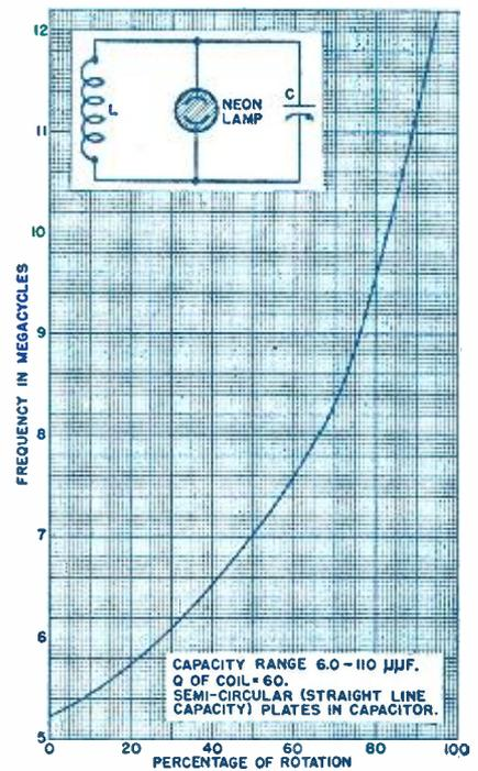
Fig. 3. Absorption wavemeter calibration.
