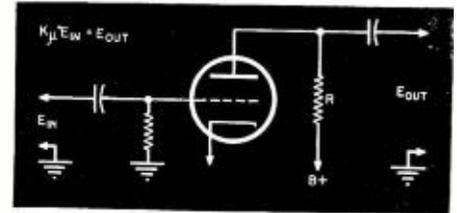
Fig. 3. Circuit for multiplication by a constant  $K\mu$ , where  $K\mu$  is the stage gain.
