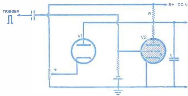
Fig. 8. Wiring diagram of gas triode single-sweep circuit.
