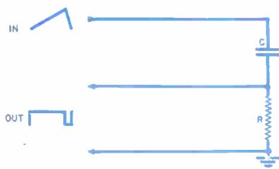
Fig. 2. Differentiating circuit to develop blanking pulse.
