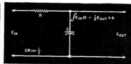
Fig. 6. Integrating circuit. In the above formula, K is a constant, depending on C, R, and frequency, while A is also a constant equal to the d.c. potential superimposed on E<sub>out</sub>.
