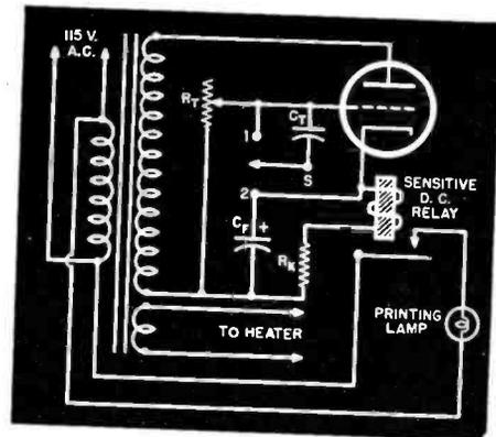
Fig. 9. Phototimer used for automatic control of lamps in enlargers and printing boxes.
