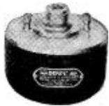
This famous MODEL 7 permanent magnet driver unit is ideal for most high-power sound projection installations. The unique magnetic structure employs a central cone-shaped magnet of ALNICO, weighing 3 lbs. 4 oz. with a flux strength of 12,000 gauss in the magnetic gap. Will not depreciate in strength through shocks nor ageing. Specifications: 16 ohms impedance; 18 to 20 watts continuous duty.
