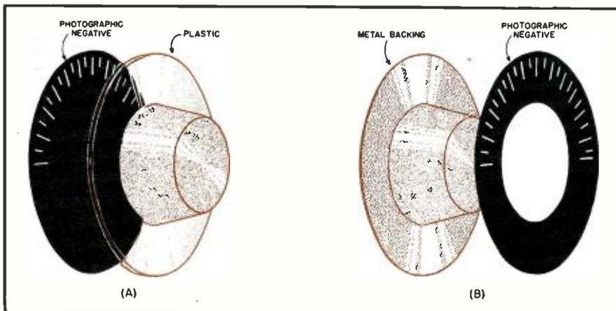
Fig. 2. Two methods of obtaining a professional-looking calibration. (A) The photographic negative with the calibration marking appearing thereon is glued to the panel or to the back of the flange. A transparent plastic knob is used with this arrangement. (B) Photographic negative is glued directly to the knob flange.
