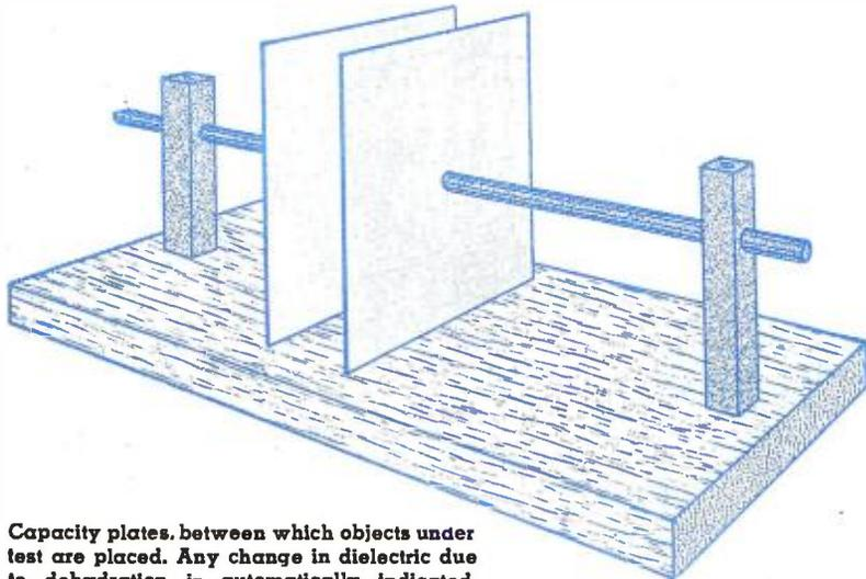
Capacity plates, between which objects under test are placed. Any change in dielectric due to dehydration is automatically indicated.
