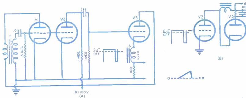
Fig. 11. (A) Blocking oscillator, amplifier, and sweep tube for linear sweep of coil current. (B) Sweep coil placed in plate circuit of V<sub>2</sub>, with damping diode.
