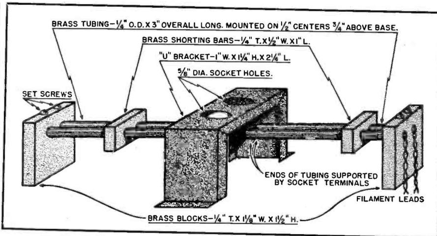
Fig. 5. Mechanical construction of the oscillator-tuning rods. The shorting bars may be varied to obtain any frequency between 400-500 megacycles.
