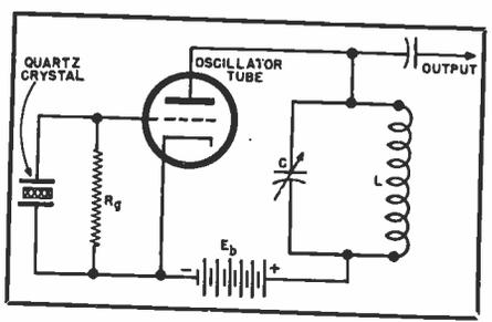
Fig. 9. A fixed-frequency quartz-crystal-controlled oscillator.
