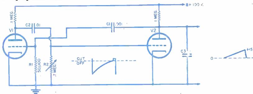
Fig. 7. Multivibrator sweep circuit, showing voltage wave applied to grid of V<sub>2</sub>.
