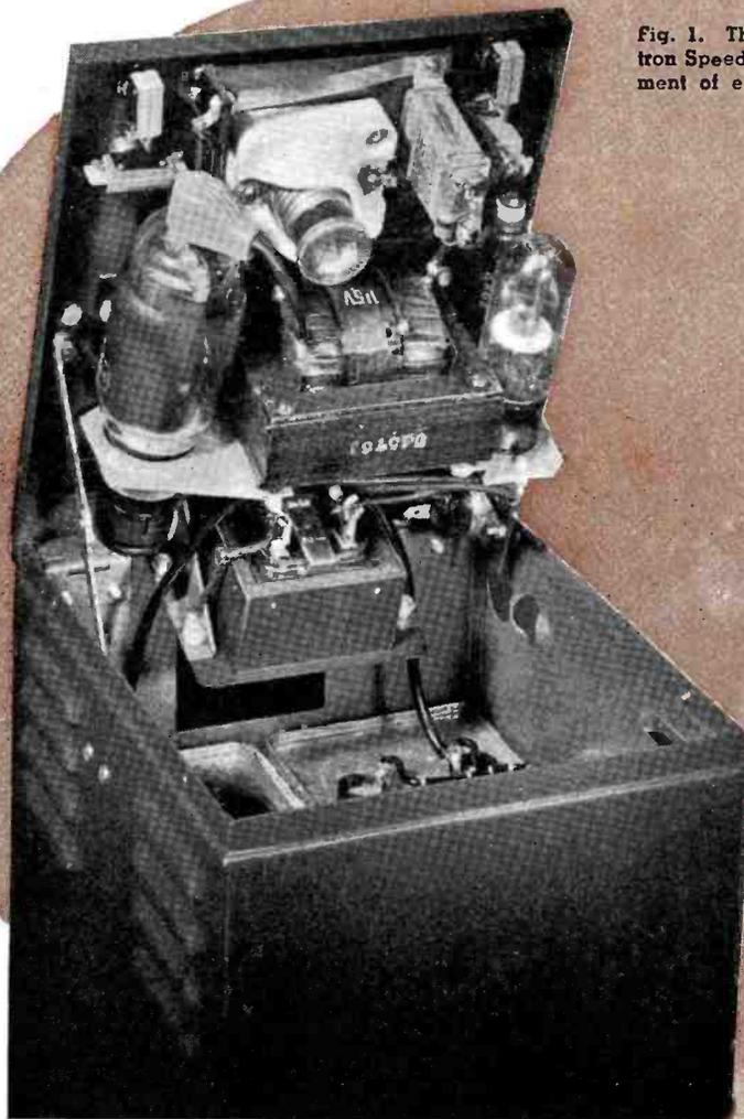
Fig. 1. The heart of the Kodatron Speedlamp, showing placement of electronic components.
