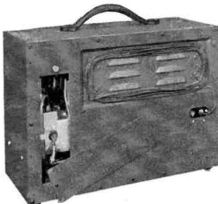
Rear view shows position of coiled antenna wire and a.c.-d.c. line cord.
