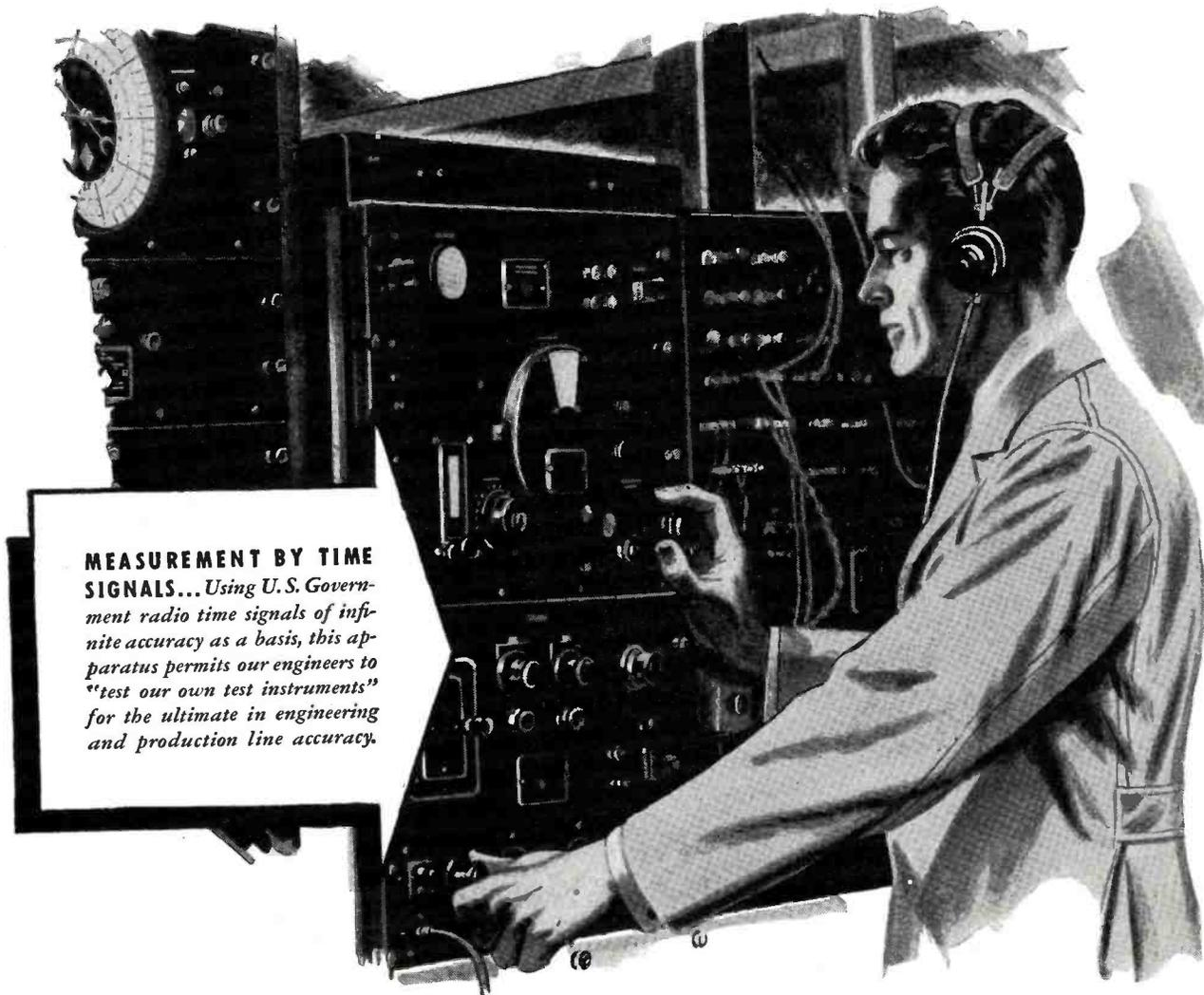
**MEASUREMENT BY TIME SIGNALS...** Using U. S. Government radio time signals of infinite accuracy as a basis, this apparatus permits our engineers to "test our own test instruments" for the ultimate in engineering and production line accuracy.
