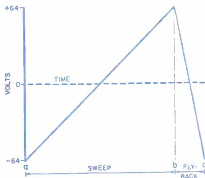
Fig. 10. Sweep voltage to horizontal plates.
