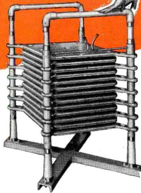
To meet the need for a light-weight, high-capacity, high-voltage tank condenser for transmitter applications, Johnson engineers developed a new type of condenser. The unit illustrated has a capacity of 1200 mmf. at a peak voltage of 40,000 volts at 2 megacycles. Nearly any combination of capacity and voltage ratings may be had. The capacity may be varied in the field by removing plates or altering spacing.
