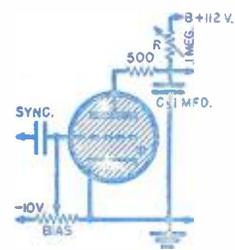
Fig. 6. Sweep circuit, using gas triode or discharge tube.
