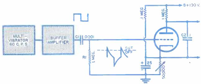
Fig. 4. Peaking circuit and biased triode for shortening fly-back time.
