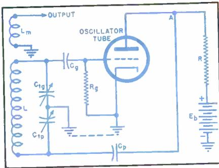
Fig. 4. Colpitts oscillator circuit in which the tank capacitance is tapped, dividing the grid and plate circuits. Capacitive feedback results.
