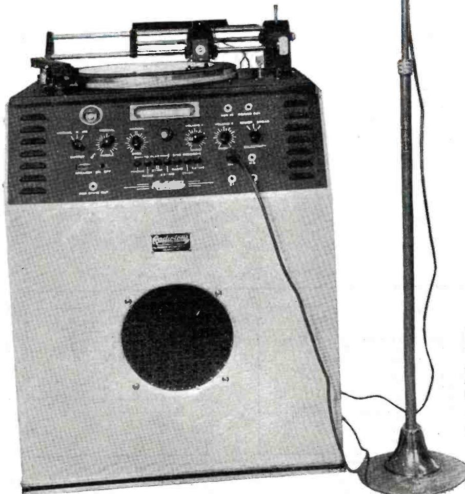
Console model features RA-16 recording unit and acoustical cabinet.
