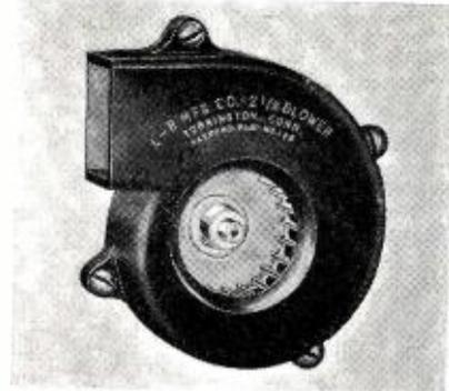
bottom. Operating under all conditions of climate and temperature, the unit which weighs but 3½ ounces, delivers 50 cubic feet per minute at 8000 r.p.m. It is available with shaft bores of either .1895 or ¼".
