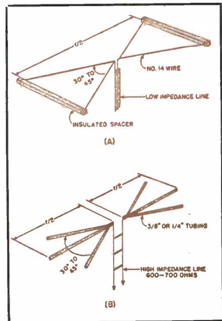
Fig 3. Two popular types of antennas: (A) V antenna; and (B) fanned antenna.
