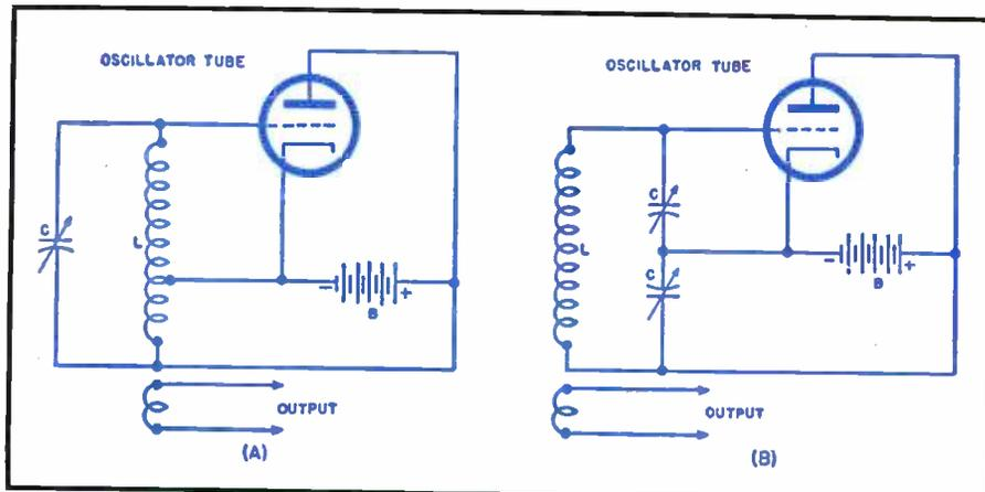
high-frequency end. Too loose a coupling may result in the oscillator ceasing to function on the low-frequency end of the band. Somewhere between these two conditions is found the best workable degree of coupling.
