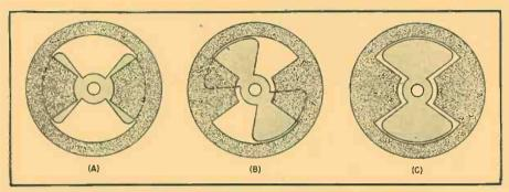
Fig. 7. Butterfly condenser. Refer to text for principle of operation.
