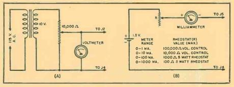
Fig. 5. Diagram for a.c. voltmeter calibration, (A); and for milliammeter calibration, (B).
