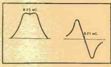
Fig. 7. Sound channel alignment curves.
