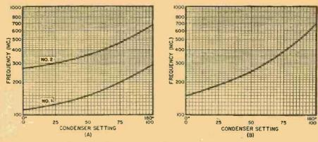
Fig. 3. (A) Tuning calibration curves of the two wavemeters shown in Fig. 1. (B) Tuning calibration curve of the wavemeter that is illustrated in Fig. 2.
