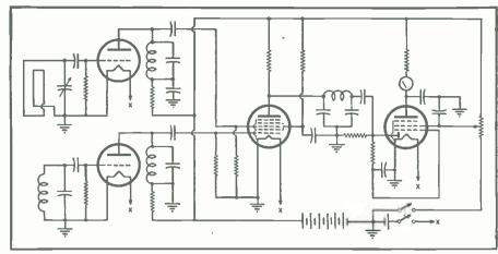
Fig. 2. General arrangement of a beat-frequency type metal locator.
