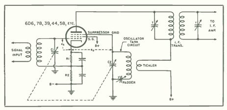
Fig. 1. Typical suppressor-grid type autodyne frequency converter employing electron coupling and used in early superheterodyne midget receivers as Majestic Model 370, etc.
