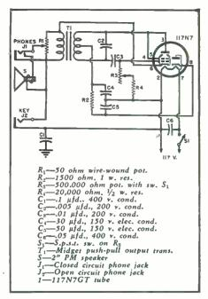
Fig. 3. Circuit diagram of the code practice oscillator constructed by the author and illustrated on page 29.
