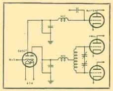
If the grid current greatly exceeds the supply rating, and the grid leak draws a small current, bias isolating rectiliers may be used. The grid leak values will depend on the type of tube in use.
