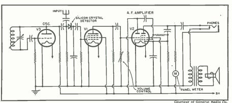
Fig. 12. Schematic diagram of the heterodyne frequency meter shown in Fig. 11.
