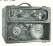
Filmgraph, a sound device for recording and reproducing sound on film instantaneously and at low cost.
