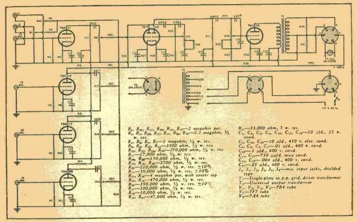
Fig. 1. Schematic diagram of basic pre-amp unit with six inputs, tone control circuit, and driver stage.
