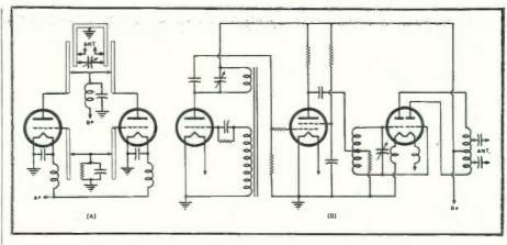
Fig. 4. Conventional diagram of two types of metal locators. (A) The self-pulsed radar type and (B) the triggered radar type.
