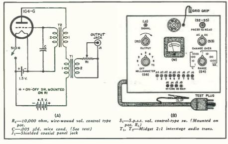
Fig. 3. (A) An alternative vacuum tube type oscillator that may be used in lieu of buzzer. (B) Front panel layout of completed test instrument.
