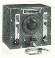
than .002% for each degree Centigrade of temperature change. Provision is made for an external crystal for spotting specific reference points.
