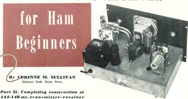
Rear view shows transmitter section (upper left) and receiver (lower right).
