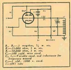
Fig. 3. Circuit diagram for control tube keyed radio frequency oscillator.
