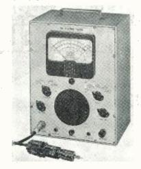
has a self-contained electronic a.c.-d.c. voltmeter and ohmmeter for additional testing if desired.
