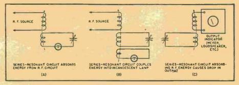
Fig. 4. Methods of using the absorption of energy, by a simple calibrated tuned circuit at resonance, as the basis of a wavemeter for measuring frequency.
