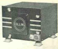
THE 180K-1 antenna loading unit efficiently transfers the power output from the 18S-1 to any standard commercial fixed antenna. Remote controlled, pretuned operation for ten channels is provided. The nominal input impedance is 50 ohms. Weight, 10 lbs. Size,  $7\frac{1}{2}$ " h,  $10\frac{1}{2}$ " d, 12" l.
