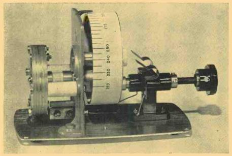
tograph, ¼ inch above the top stator plate, with its center above the center of the rotor. The slider arm is just another piece of No. 12 wire, of the proper length (about  $\frac{3}{4}$  inch) to mount the brass evelet slider correctly. and is soldered into a groove filed in the shaft of the rotor to give the solder connection a certain amount of mechanical strength. The total inductance of the circuit varies from about .02 to .06 microhenries.
