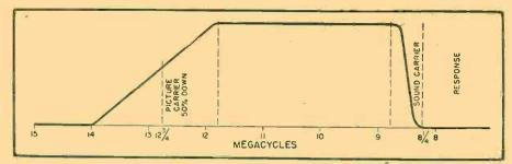
Fig. 1. Idealized band-pass characteristic of television i.f. amplifier.
