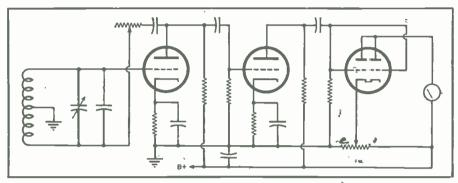
Fig. 3. Basic diagram of a super-sensitive type locator used by the , Australian troops in locating the so-called "non-metallic" mines.
