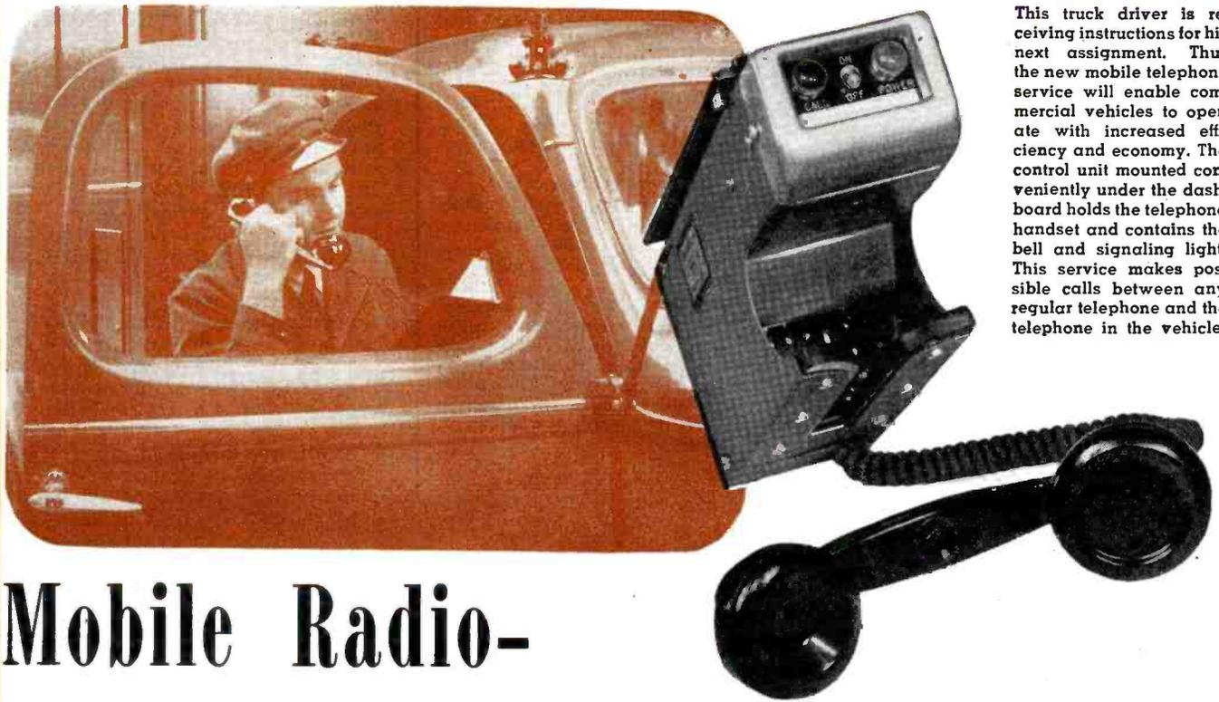
This truck driver is receiving instructions for his next assignment. Thus the new mobile telephone service will enable commercial vehicles to operate with increased efficiency and economy. The control unit mounted conveniently under the dashboard holds the telephone handset and contains the bell and signaling light. This service makes possible calls between any regular telephone and the telephone in the vehicle.
