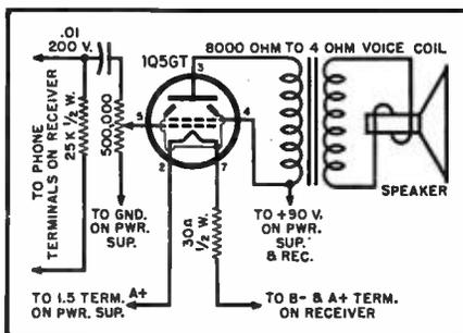
Wiring diagram of one-tube audio amplifier. This unit, when built, can be used in conjunction with the one-tube receiver covered in last month's issue, page 66.
