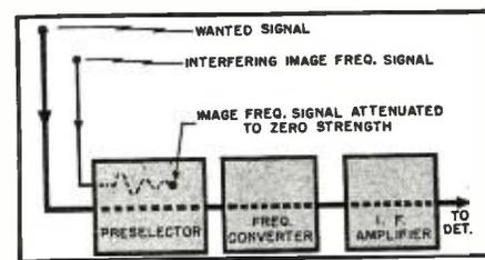
Fig. 3. Illustrating how an image frequency signal may be sufficiently attenuated by a preselector so that it does not reach the frequency converter.
