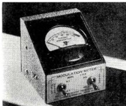
ulated carrier, as well as giving an indication of carrier shift. It enables the user to avoid over-modulation.
