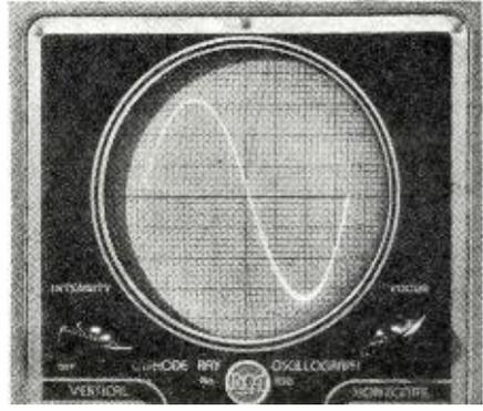
Fig. 5. Actual 400 cycle modulated waveform from signal generator described. This trace was taken after signal passed through the r.f. and audio stages of a commercial receiver. Buffer stage modulation is approximately 45%. A pure sine wave is a factor in checking over-all distortion taking place in r.f., converter, detector, and audio systems of receivers.
