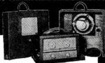
Portable system in a three-section, compact case. 15 watt amplifier with one phonograph and two microphone inputs, two heavy duty Alnico V reproducers, and 25 feet of durable cord with connectors attached. One case has the reproducer receptacle for connecting in cascade. Underwriters approved.
