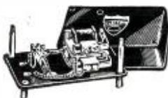
**T-100 Time Delay Relay.** In radio transmitter circuits, Guardian's T-100 Time Delay Relay prevents damage of rectifiers and tube filaments by preventing plate current before filaments are sufficiently heated. Laminated field piece and armature. Mounted in dust-proof metal box.
