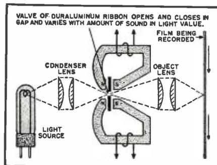
Fig. 5. The essential elements employed in variable density recording.
