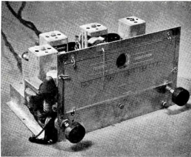
Fig. 3. Meissner tuner with the newly calibrated dial scale.
