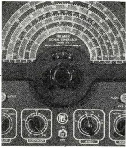
Fig. 6. Close-up view of vernier and "Micromaster" tuning dial of the signal generator shown in Fig. 1. Calibration reference points of from 0-100 available on the geared vernier provide a precision factor for aligning FM and TV sets.
