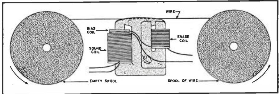
Fig. 11. Combined record-playback head assembly for wire.
