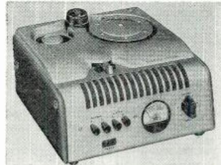
The Model 78 utilizes push-button controls for greater flexibility of operation in any of four "record" and "listen" positions. The unit consists of a wire transporting mechanism, a pre-amplifier, interstage amplifier, oscillator, and built-in power supply. An accurately calibrated recording level meter assures correct recording volume. The recorder is housed in a metal case measuring 11 1/2"x11"x5 1/2".
