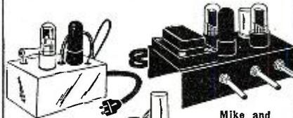
**Phono Pre-Amplifier \$4.95** This unit is for G. E. Reluctance type cartridge. Completely wired, tested. Supplied with diagram, and tube 6SC7.
