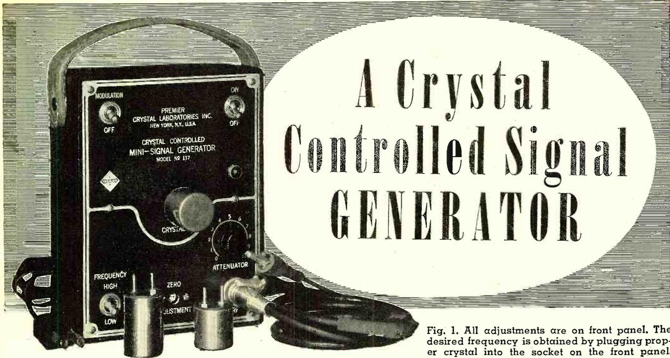
Fig. 1. All adjustments are on front panel. The desired frequency is obtained by plugging proper crystal into the socket on the front panel.
