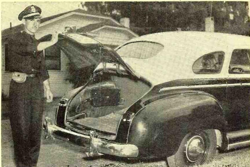
Taxi driver demonstrates the small size of two-way radio telephone units. The entire unit occupies little space in trunk compartment. Note antenna stub atop cab.
