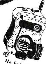
Transmits automatic SOS signal on 500 KC emergency wave. Can be manually keyed to transmit additional information. Hand cranked. Supplied with parachute, signal light, box kite, balloons with hydrogen generators. Complete, original pack.
