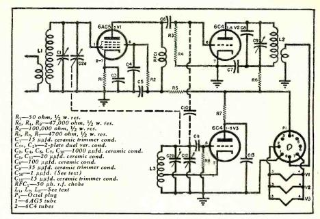
Circuit diagram and parts list covering the 6 meter converter unit.
