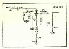
Fig. 8. The video second detector of UST sets is a 1N34 germanium crystal unit.
