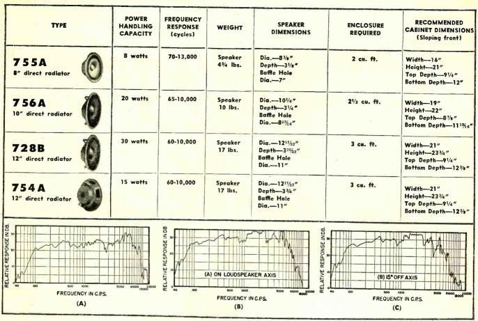
Fig. 4. Baffle requirements and dimensions for Western Electric 8, 10, and 12 inch speakers designed for use with totally enclosed cabinets. Frequency response curves shown are (A) for the Western Electric 8 inch (755A) speaker at a point on its axis; (B) and (C) for the Western Electric 12 inch (728B) speaker.
