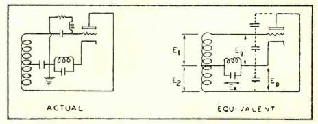
Fig. 5. Circuit diagram and v.h.f. equivalent of the hybrid circuit devised to compensate for transit time phase shift.
