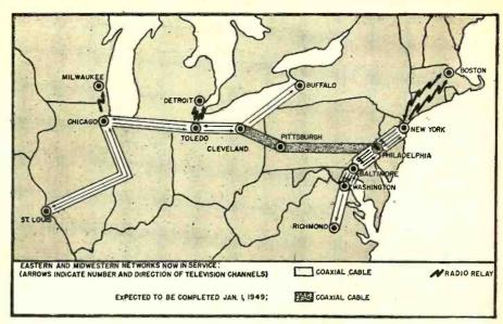
Fig. 1. Bell System TV network map showing coaxial cable and relay facilities as of Nov. 1948.
