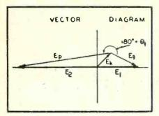
Fig. 7. Vector diagram showing phase shifting effect of the resonant cathode chokes in the hybrid v.h.f. oscillator circuit.
