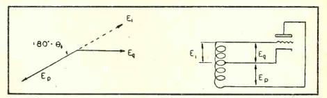
Fig. 4. Vector diagram showing how electron transit time can produce a feedback of incorrect phase in order to sustain oscillations.
