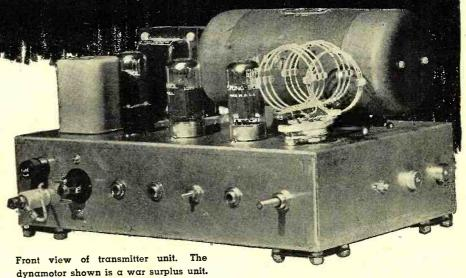
Part 2. Construction details for a 10-11 meter transmitter. The companion converter unit, for use with any auto radio, was covered last month.
