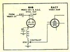
Fig. 7. The video detector of the Farnsworth Model GV 260 television receiver.
