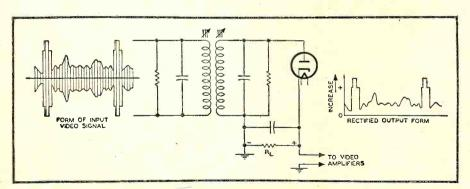
Fig. 1. A video second detector. In order to operate efficiently, peaking coils must be added to this basic circuit. See Figs. 2 and 3.
