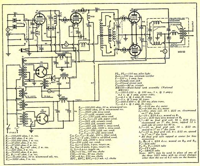
Complete circuit diagram and parts list for constructing the 3.5-30 mc. transmitter.
