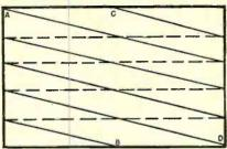
Starting at "A" terlacing easier. the spot scans the image and due to the  $\frac{1}{2}$ , (262 $\frac{1}{2}$ ), the spot ends its course at "B." Then going up to "C" it starts scanning again on the odd interlaced lines and terminates at "D." This completes one frame of interlaced scanning. The spot then returns to "A" to commence a new frame.
