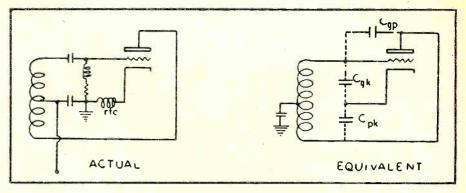
Fig. 3. A basic Colpitts oscillator circuit and the equivalent circuit at v.h.f.
