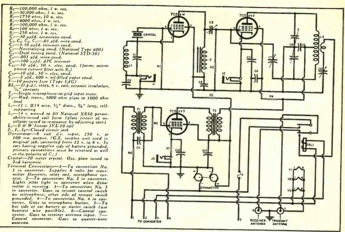
Fig. 1. Complete schematic diagram and parts list for mobile transmitter.
