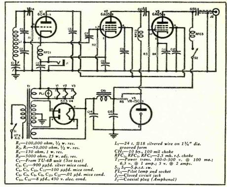
Fig. 1. Circuit diagram and parts list covering a stable v.f.o. unit.
