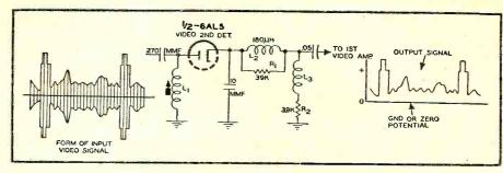
Fig. 3. The same circuit as shown in Fig. 2 with the exception that the tube terminals are interchanged to produce a negative phase output.
