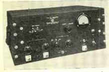
rapid comparison, are available. Operating frequencies are from 500 to 5000 cycles and operation can be wideband or highly selective as needed. The selective network is panel-tuned through the previously mentioned range. The output meter is calibrated directly in standing wave voltage ratio.
