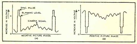
Fig. 4. Form of video signal in a negative (A) and positive (B) picture phase.
