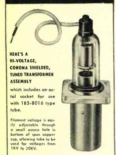
This unit is designed to operate in conjunction with RF step-up coils af approximately 200 KC frequency, solving the problem of research workers and experimenters in the construction of Corona-Free HI-Voltage RF Power Supplies.
