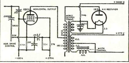
Fig. 1. A typical high voltage rectifier circuit as found in the RCA Model 630 TS receiver.
