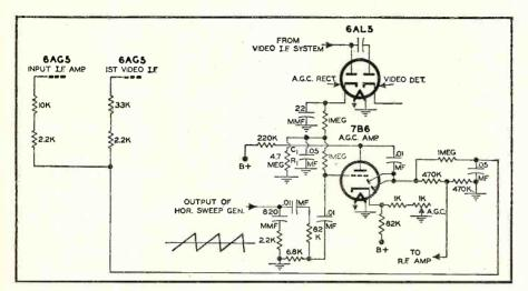
Fig. 8. The special a.g.c. network found in Philco television receivers.
