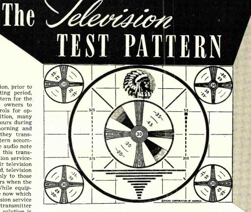
Fig. 1. "Indian Head" test pattern used by many television stations.
