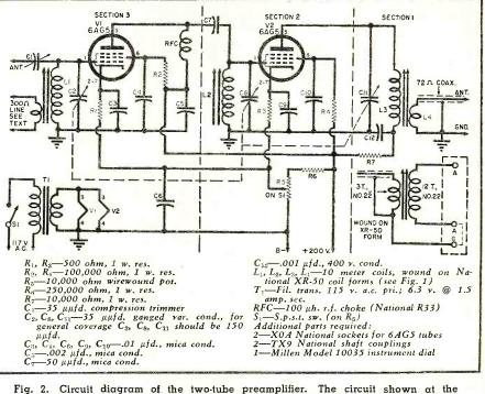
Fig. 2. Circuit diagram of the two-tube preamplifier. The circuit shown at the lower right may be used to match preamplifier to the normal 400 ohm receiver input.
