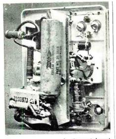
Closeup view of chassis showing parts layout.
