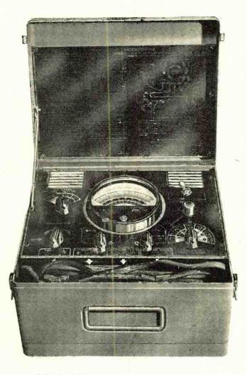
0-60 volts and 0-60 amperes. One switch box indicator has following ranges: 0-9 volts and amperes, scale deviation— 0-9 range in 1/10th of a volt, 0-18 in 2/10th's of a volt, 0-60 in 1 volt and ampere division, 0-9 in .05th of a volt and ampere.
