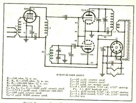
Circuit diagram and parts list for the two-meter converter unit.
