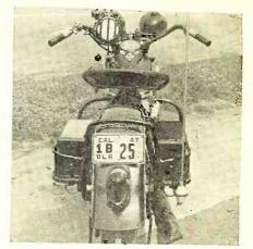
Rear view of complete assembly showing control head, mike, xmtr.-receiver, and antenna,
