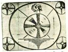
Fig. 3. Example of horizontal non-linearity.
