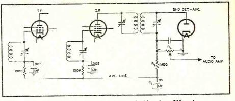
Fig. 1. A typical a.v.c. network found in standard broadcast AM receivers.
