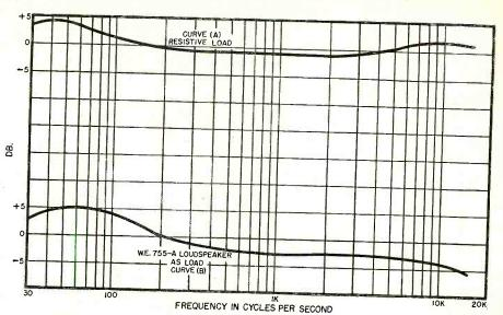
Fig. 6. Performance curves of the amplifier shown in Fig. 5. These curves were
