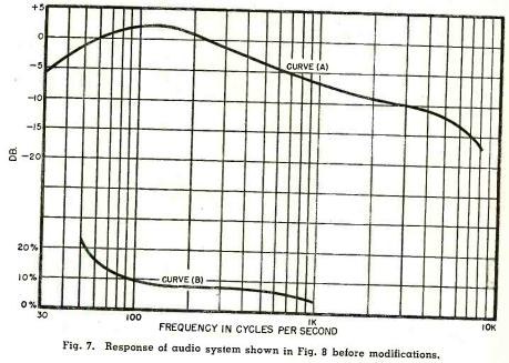
of the first audio tube, and the .005  $\mu$ fd. unit shunting the output transformer primary improved matters to some extent but was not the final solu-
