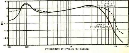
Fig. 2. Audio system response curves for original receiver with volume control set halfway.
