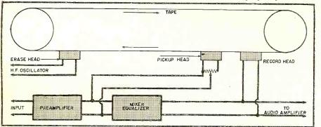
Fig. 2. Author's system supplies succession of echoes utilizing a single pickup head.
