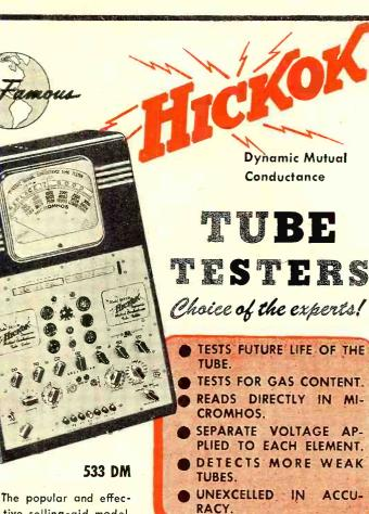
tive selling-aid model, for quick customer-convincing, counter demonstration and test. Large 9-inch meter reading directly in micromhos.
