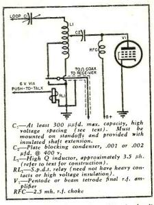
Fig. 2. Coupling network and tank circuit for use with single-turn loop of Fig. 3.
