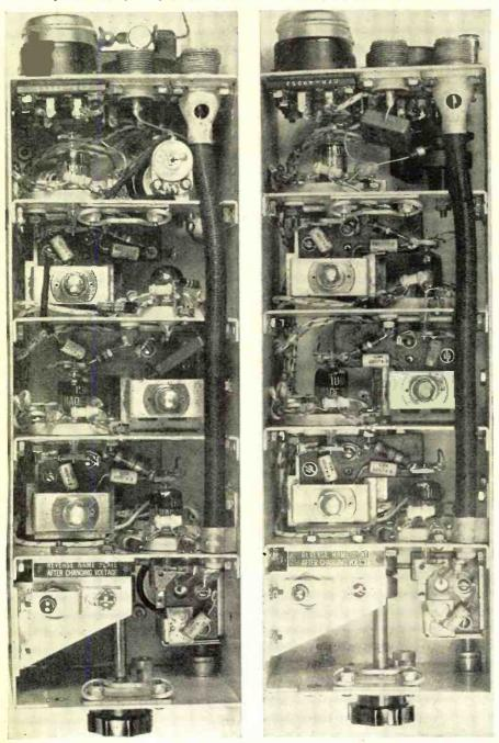
that when the voltages are applied the set will be on frequency. Lacking the grid dip meter, it is necessary to use the older, but still workable, method of "cut and try." It will simply consume more time and patience. Final tuning and padding of the oscillator is done with  $C_{\rm int}$ .
