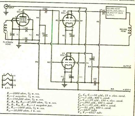
Fig. 4. Circuit diagram of a recording amplifier that may be built as a special unit to provide synthetic reverberation. Circuit is not critical and presents no construction difficulties.
