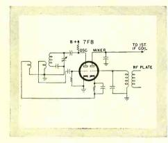
**TRIODE MIXING...** in the first detector. This quieter method of conversion greatly boosts the signal-to-noise ratio because there's almost no first detector "hiss." Inductive coupling (rather than electronic) of the oscillator signal avoids multi-grid noise in the sensitive 50-Mc range.
