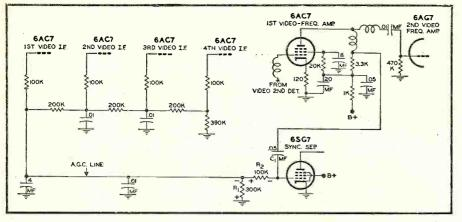
Fig. 7. The a.g.c. network used in Tele-King television receivers.
