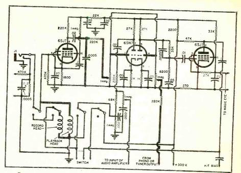
Fig. 3. Heavy lines show modifications made in author's "Soundmirror" recorder.
