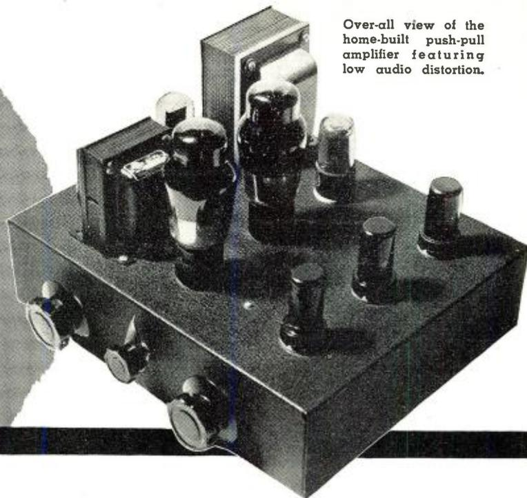
Over-all view of the home-built push-pull amplifier featuring low audio distortion.
