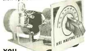
**YOU BUILD** this Wavemeter and use it to determine frequency of operation, make other tests on transmitter currents.
