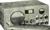
National NC-57: Five bands, 540 kc. to 55 mc.; bandspread tuning; built-in speaker; nine tubes; a.c. operation.
