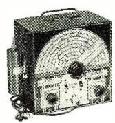
Signal Generator Specifications: Signal Generator Specifications: Frequency Range: 150 Kilo-cycles to 50 Megacycles. \*The R.F. Signal Frequency is kept completely constant at all out-put levels. \*Modulation is ac-complished by Grid-blocking ac-tion which is equally effective for alignment of amplitude and frequency modulation as well as for television receivers. \*R.F. ob-tainable separately or modu-lated by the Audio Frequency. tainable separately or mo lated by the Audio Frequency.
