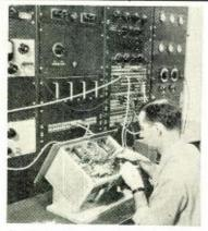
COVER PHOTO: The testing of precision audio equipment requires the use of laboratory instruments to insure proper operation. Here Ernest Baumeister tests an audio filter in the laboratories of Cinema Engineering Co., Burbank, Calif. Further details are given on Page 70. (Photo by Arthur Haug)
