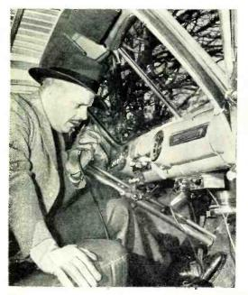
Fig. 4. The mobile unit used in this carrier system is operated through the control head mounted on the instrument panel of the car's or truck's dashboard. Push-to talk operation is customary. Fig. 5. The main station transmitter-receiver is remotely operated by the REA dispatcher through the office control unit. Transmitter is linked to office by means of a single circuit phone line.
