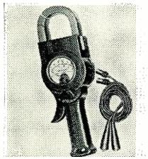
1000 amperes and three voltage ranges up to 700 volts has been introduced by the Weston Electrical Instrument Corporation, 617 Frelinghuysen Avenue, Newark 5, N. J.
