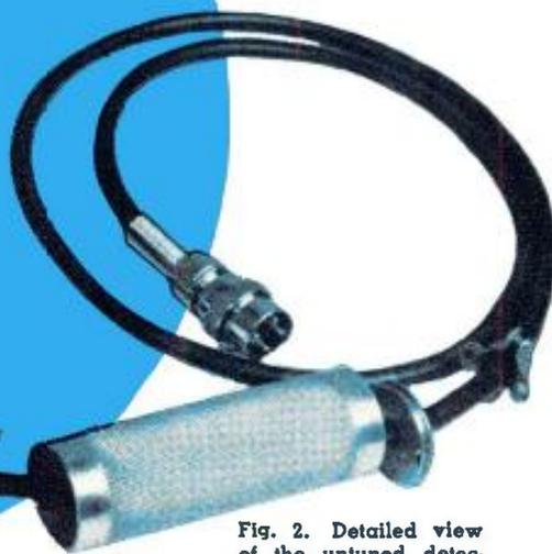
Fig. 2. Detailed view of the untuned detector probe assembly.
