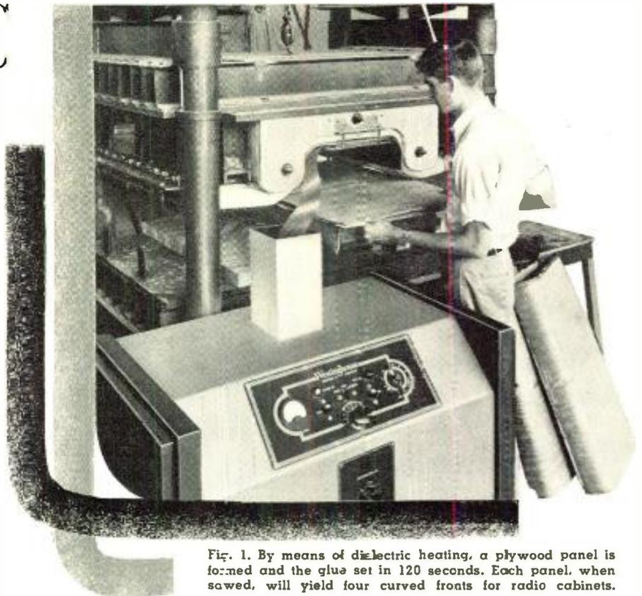
Fig. 1. By means of dielectric heating, a plywood panel is formed and the glue set in 120 seconds. Each panel, when sawed, will yield four curved fronts for radio cabinets.
