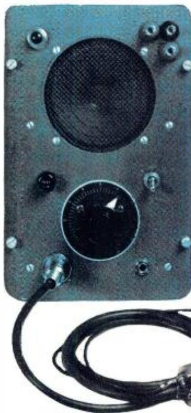
Fig. 1. View of signal tracer. The panel measures 10 $\frac{3}{8}$ " x 7". Unit is 6" deep.
