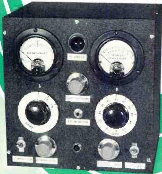
Fig. 1. Front view of unit. Modulation peak percentages up to 100% can be measured.
