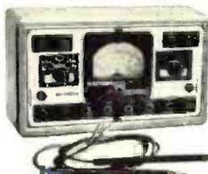
This versatile testing instrument is portable and complete with test leads. Simple to operate, accurate and dependable. You will be able to quickly locate trouble and adjust the most delicate circuits. You can use the Multitester at home or on service calls. It is designed to measure AC and DC volts, current resistance and decibels. You will be proud to own and use this valuable professional instrument.
