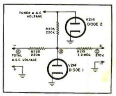
Fig. 5. Diode 1 of V214 produces the delay action of the a.g.c. circuit of Fig. 4.
