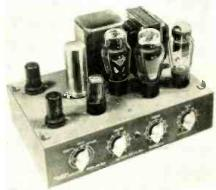
separate jacks are provided for magnetic pickup, microphone, crystal pickup, and radio or TV. Volume, bass, and treble control switches are on the front panel. The rear panel carries
