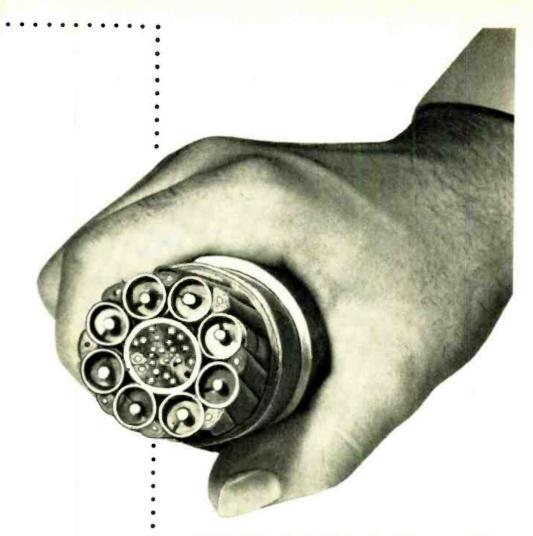
Cross-section of ccaxial cable. To triple capacity, Bell Laboratories and Western Electric engineers had to make 1000 amplifiers work perfectly in tandem . . . feed repeater power along the same cable that carries messages . . . put signals on and off the line at numerous cities along the route without distortion.
