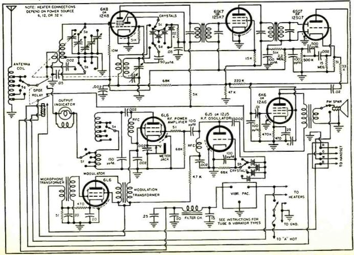
for marine type broadcast receivers and two-way radiotelephones.
