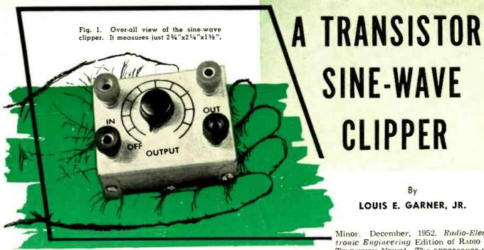
This useful test accessory can be used alone or built into an existing audio oscillator. It is compact and reliable.
