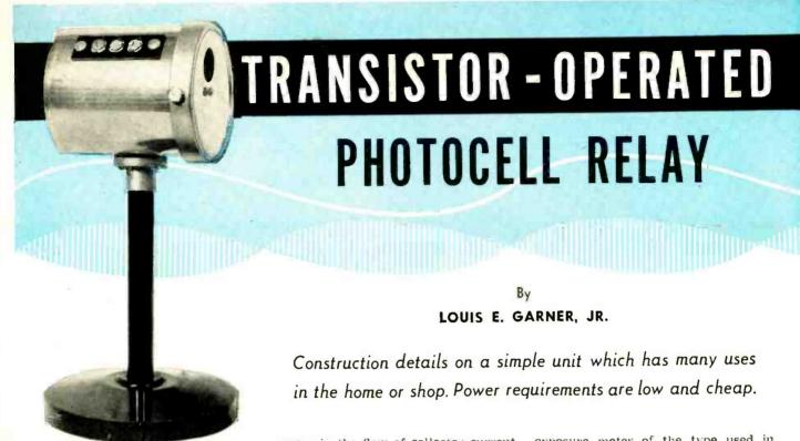
Fig. 1. Over-all view of author's unit. A discarded exposure meter cell was used.
