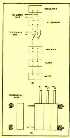
Fig. 2. Calibration of vibration pickups by the reciprocity method.
