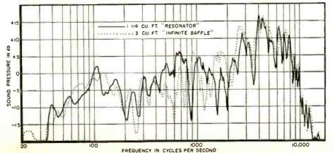
air resonance of the speaker. The general effect of the infinite type of baffle with no acoustic compensation is to tighten up the speaker in a limited frequency range.
