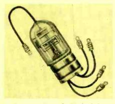
medium cap without flexible lead. Average anode current is 3 amp., peak anode current 30 amp., peak anode voltage 1000 volts. Deionization time is under 175 microseconds.
