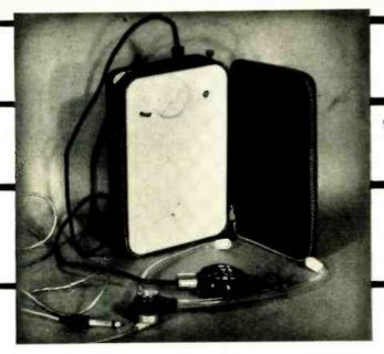
Fig. 1. The "Minifon" measures but 45%" x 7" x 2" when contained in its soft leather zipper case. Crystal diaphragm microphone and stethoscope-type earphones come with each recorder.
