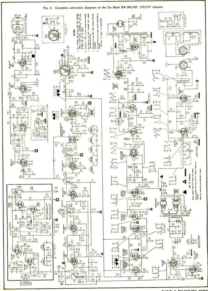
single tuned. A 47.25 mc. absorption type, adjacent-channel sound trap is provided in the plate circuit of the second i.f. stage.
