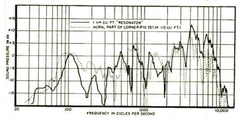
Fig. 11. Relative response of the  $1\frac{1}{4}$  cu. ft. resonator and a  $4\frac{1}{2}$  cu. ft. horn which is a part of the corner of the test room. Refer to Fig. 3E for details.
