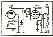
Fig. 7. A noise suppression circuit used by RCA. See text for operational details.
