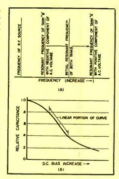
Fig. 4. (A) Tank circuit relationships of Fig. 5B. (B) Capacitance vs. d.c. bias curve for K = 3300 dielectric material.
