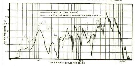
Fig. 10. Relative response of a  $1\frac{1}{4}$  cu. ft. resonator and a  $4\frac{1}{2}$  cu. ft. horn which is not part of the corner. See the test set-up shown in (D) of Fig. 3.
