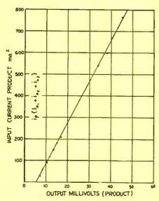
Fig. 4. Open-loop multiplication.
