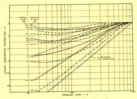
Fig. 4. Dynamic compensation required in addition to that afforded by the so-called static type of loudness control.
