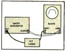
Fig. 2. Test setup for visual alignment.
