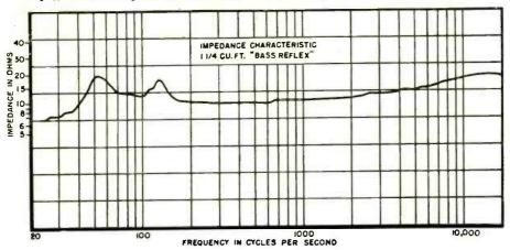
Fig. 7. Impedance characteristic of the 11/4 cubic foot bass reflex type cabinet.
