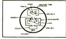
Fig. 5. Internal construction of the 6BN6.
