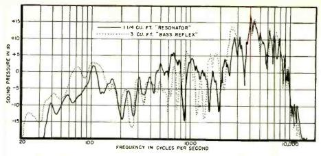
Fig. 9. Relative response of a 11/4 cu. ft. resonator and a 3 cu. ft. bass reflex.
