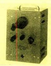
the addition of 4-, 2- or 0.5-mc. markers to the cathode-ray tube display of any S-band spectrum analyzer. Model MG10S will make possible quick visual interpolation and differential estimates without reference to charts or dials.
