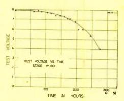
Fig. 3. Actual measurements of gradually decreasing test voltage, corresponding to gradually decreasing gain, for one amplifier stage. Over-all performance was not measurably affected until the test voltage had fallen to little more than half its original value; by then the deteriorating stage was almost ready to cause a complete receiver failure.
