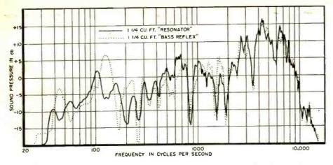
Fig. 6. Relative response of a 11/4 cubic foot resonator and bass reflex of same size.
