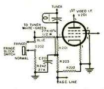
sistor between the junction of R201-R203 and the junction of the blue and white-green leads.
