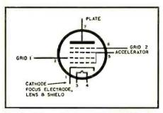
Fig. 3. Schematic symbol of the 6BN6 tube.
