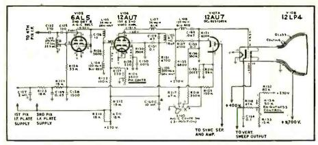
Fig. 2. Improved version of noise suppression circuit shown in Fig. 1.
