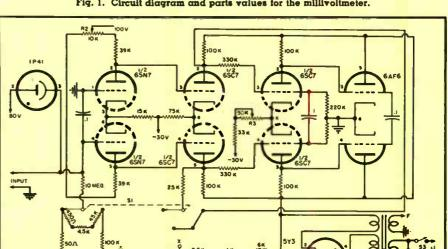
Fig. 1. Circuit diagram and parts values for the millivoltmeter.
