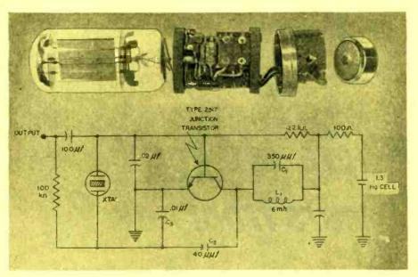
Exploded view and circuit diagram of the NBS transistor oscillator.
