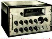
TVI Suppressed 100 Watter—Model HT20-Here's the transmitter you've been waiting for! Continuous coverage from 1.7 Mc to 30 Mc. Full band switching, no more plug-in coils; choice of 10 crystals. Shielded, filtered r-f compartment plus low-pass 52 ohm co-axial line output filter assures at least 90 db suppression of all harmonics above 40 Mc. Only \$449.50
