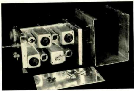
Fig. 3. Top view, showing tube and transformer layout and sheet-metal covers. The method of adjusting the coupling of  $T_{\alpha}$  (lower right) is explained in the text.
