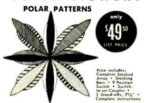
The polar directivity response patterns show the major lobes of the "Riviera" antenna an VHF. It shows the fuliness of coverage in all directions of this remarkable, patented antenna as it is surned through each of the nine switch positions. Each degree of shading constitutes a different switch position. This excellent directivity responses, which can be switched at will, plus the extremely high gains, clearly indicate why the Riviera is such a superior performer.
