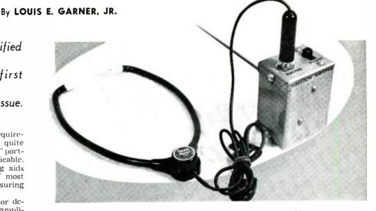
Fig. 1. Over-all view of transistorized vibration pickup and its amplifier.
