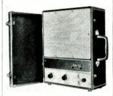
complementary 10-watt audio amplifier in an acoustically correct enclosure. Response of the 620, measured in air by accepted acoustical standards, is essentially flat from 60 to 10,-000 cycles. The unit is encased in a Samsonite luggage-type carrying case.
