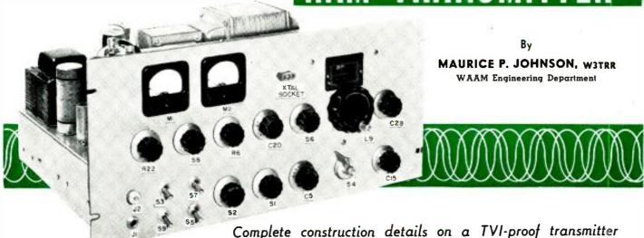
Complete construction details on a TVI-proof transmitter which uses standard components and covers five ham bands.
