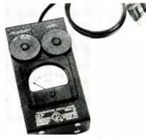
currently offering a pocket-size transistor oscillator for audio-frequency testing, the Type 1307-A.
