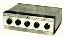
selection of radio, TV, tape or phono inputs, separate turnover and roll-off controls for record compensation, continuously adjustable bass and treble controls, and a loudness control. The audio control measures 31/2" x 10 1/4" x 6". Three tubes are used.
