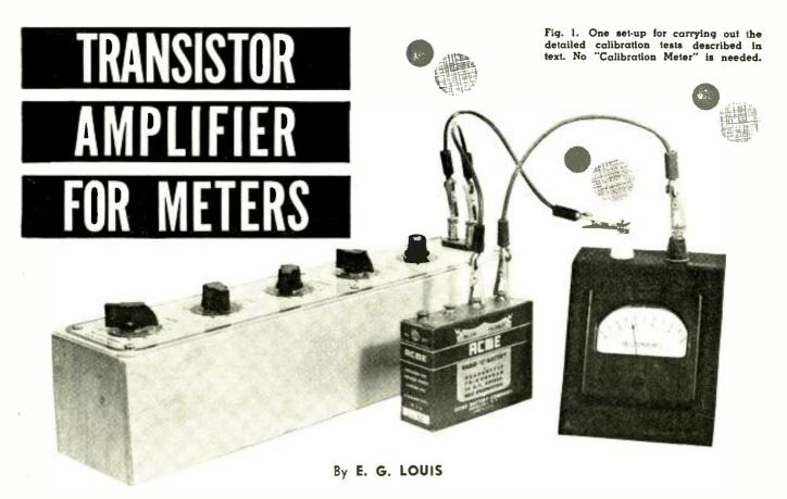
A simple amplifier circuit which can be added to standard 0-1 ma. meters to increase sensitivity by a 10:1 ratio.
