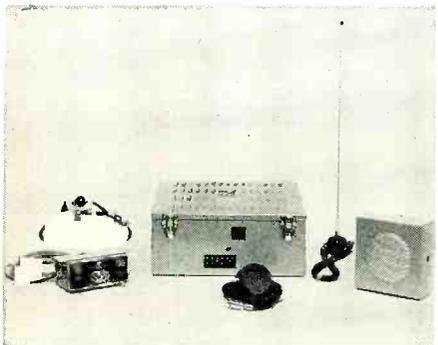
airport vehicles and ground stations, features a v.h.f.-AM two-way radio unit for use in ramp jeeps, electricians' trucks, crash trucks, tow tractors, snow plows, executive cars,
