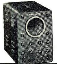
Wide-band, 5" Oscilloscope; equals or betters the performance of commercially.
