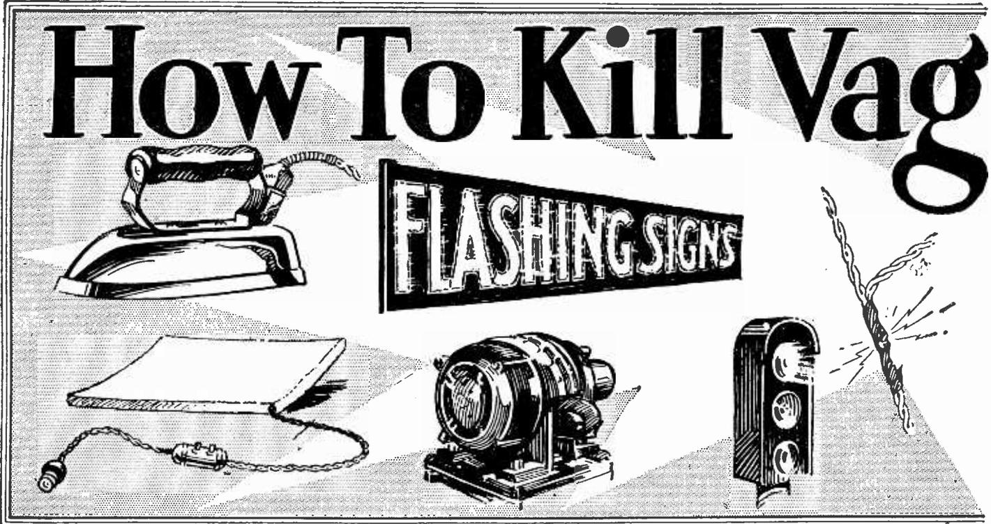
Some of the radio noise-makers. Top row: electric flat iron with poor contact or defective resistance; flashing signs or flashers in window displays. Bottom row; electric heating pad, sparking motor, railroad signals, faulty connections in lamp leads.
