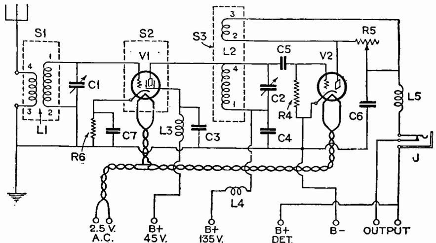
A.C. tubes in a two tube Tuner
