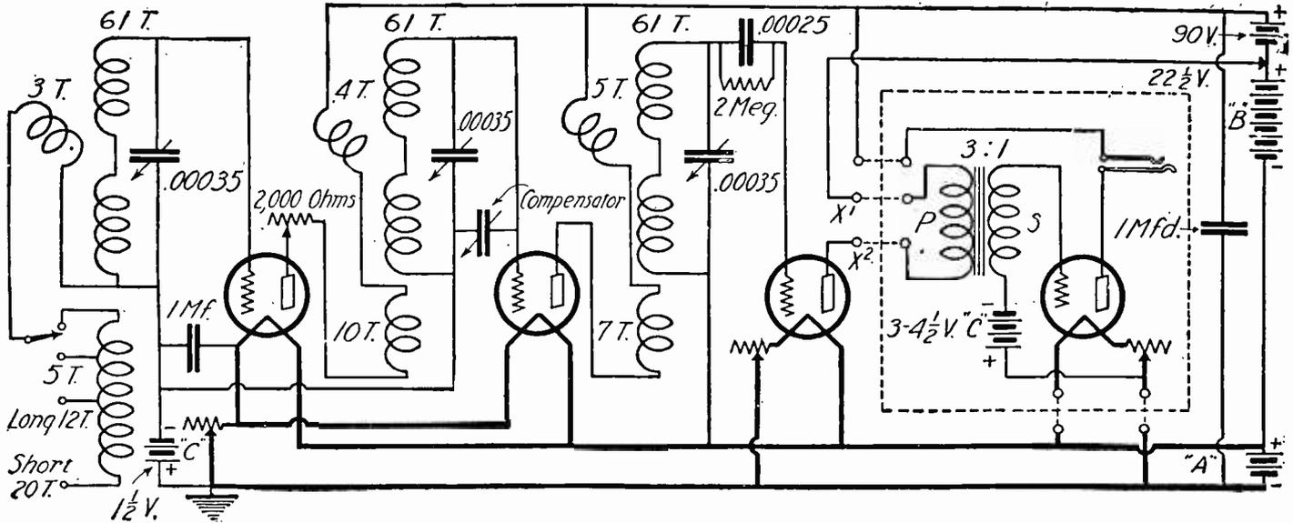
the wave-length peak (that is, the wave-length at which the amplification is greatest) of the intermediate frequency transformers selected. For that reason it will be necessary to use larger honeycomb coils than you now have. Try two 600-turn honeycomb coils shunted by two variable condensers having maximum capacities of about .001 mf.
