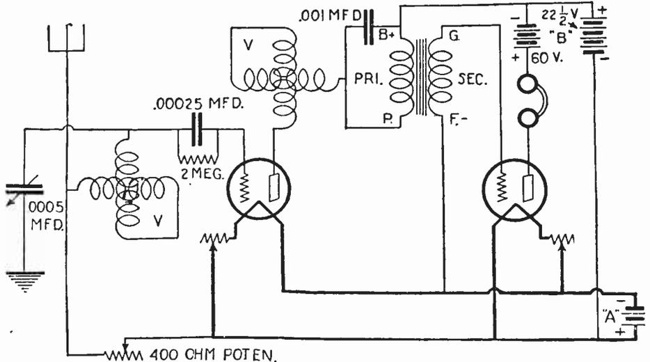
Variometers are used in this circuit
