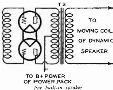
a little timid at the idea of tinkering with the family receiver. In Fig. 7 is shown the average push-pull commercial hook-up. Here T2, the output transformer of the push-pull stage, is of the step-down variety. This transformer has in some cases a step-down
