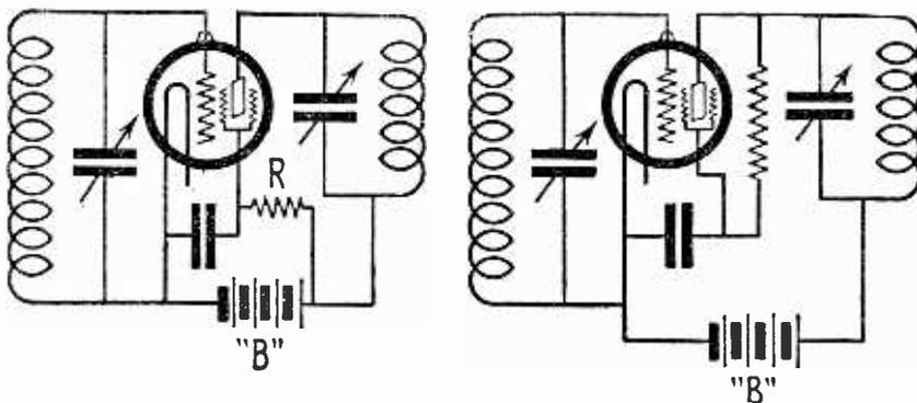
Figs. 1 and 2 show alternative methods of insuring automatically a proper voltage between screen-grid and plate. The latter is somewhat easier mechanically.
