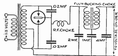
The new method of connecting condensers is more effective with smaller capacities.
