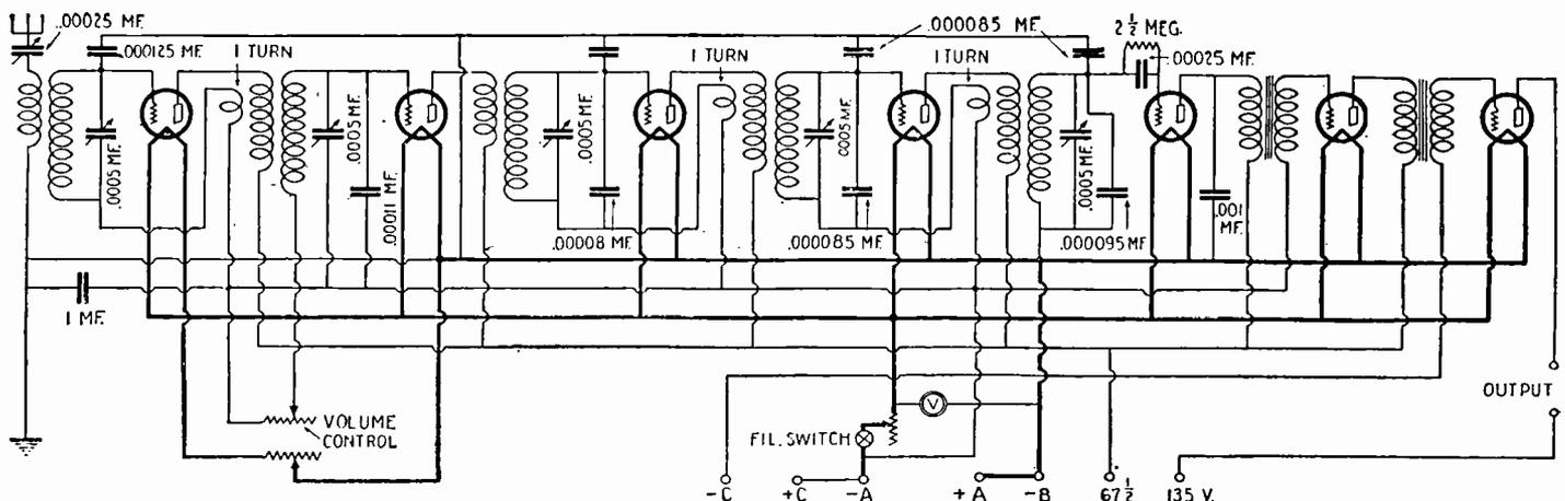
The schematic wiring diagram of the Kellogg R.F.L. receiver. This set combines many desirable features which are very popular with the broadcast listener; the most important of which are four stages of tuned-radio-frequency amplification before a detector, and two stages of audio frequency amplification. A power tube is used in the last audio stage, using the voltage shown.
