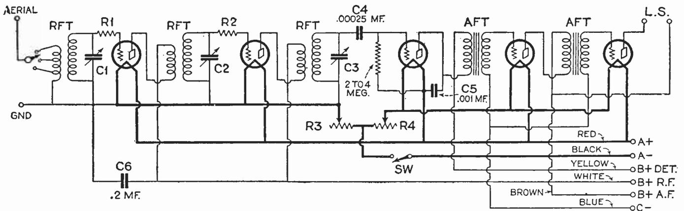
The Atwater Kent "Model 20," one of the most popular receivers ever built, in its day, used the circuit shown above. In the July, 1928, issue of *RADIO NEWS* (page 44) will be found an article on adapting this receiver to modern conditions with an added power stage for a large cone speaker.
