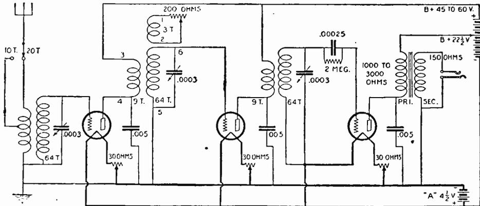
one stage of push-pull audio frequency amplification with a phone jack so arranged that plugging the phones into the detector jack will automatically disconnect the push-pull amplifier tube filaments. When the head-phones are removed from the detector jack, the loud speaker should be automatically connected to the output of the amplifier.
