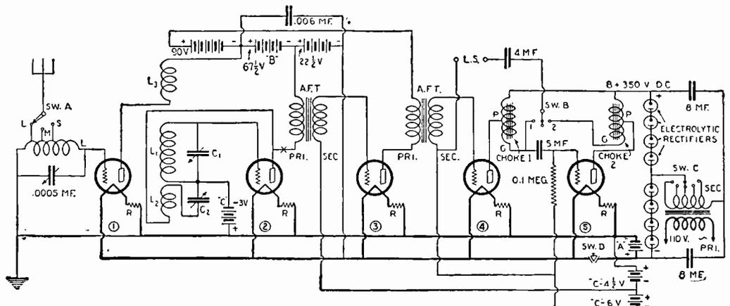
To eliminate strong hand-capacity effect, the writer has shown the rotor of C-2 connecting to the "C" battery side of the instrument.
