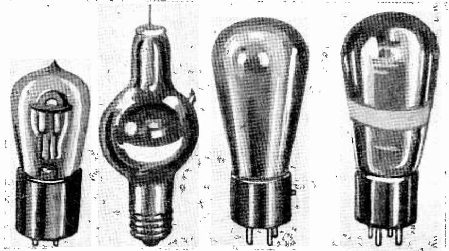
Well-known rectifying tubes; left to right, gas-filled filamentless, gas-filled filament, half-wave (one-plate), and full-wave (two-plate) filament types.
