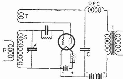
The choke coil RFC and condenser C are connected as shown, in order to keep R.F. currents out of the A.F. amplifier, where they would tend to overload the tubes.
