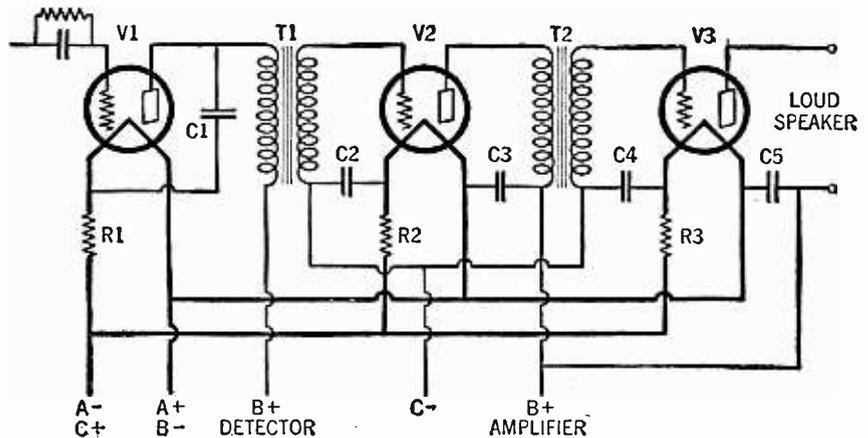
Schematic circuit of the arrangement when transformers are used. C1 may be from .001-mf. up; C2 and C4 are usually 0.25-mf., C3 and C5, 1 mf., though such values are not critical.
