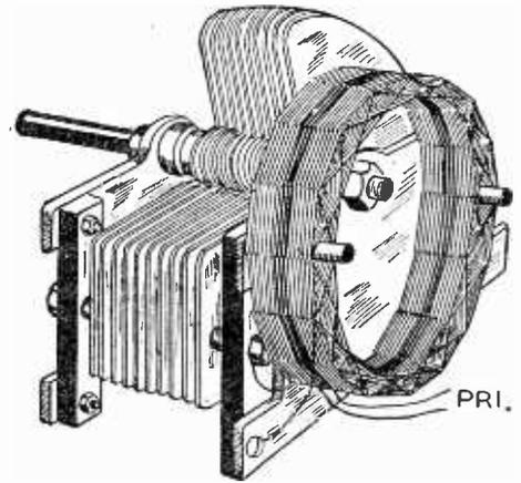
The Freshman "eddy currents" method of oscillation control. The inductance is placed sufficiently close to the condenser end-plate for the lines of force of the coil to cause eddy currents (a form of loss).
