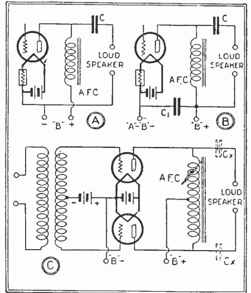
appeared in a past issue of *Radio News*. In this article it is explained that regeneration is caused by coupling between the plate and grid circuits of a vacuum tube; as such coupling makes it possible for plate-circuit energy to be returned to the grid circuit and to be re-amplified excessively. This coupling may be effected by the use of either condenser, induc-
