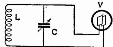
A neon lamp connected to a resonant circuit indicates, by lighting, the flow of current which creates voltage across the plates of the condenser and the ends of the coil.
