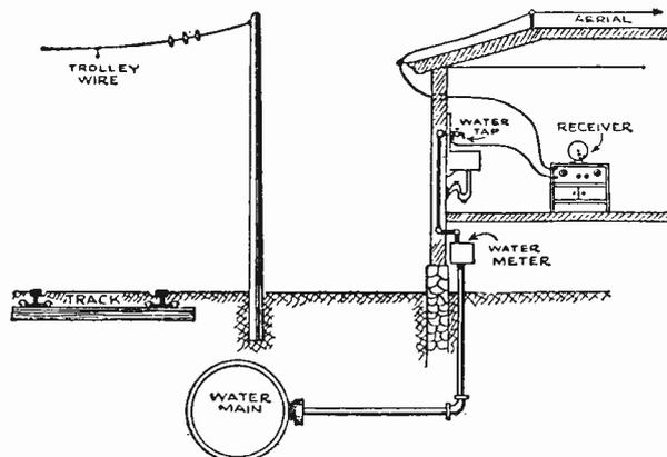
The phenomenon of inductive pick-up accounts for interference, when there is a filter in the light-line; or even when no house-current connection is made. The water pipe, parallel to track and trolley wire, may cause this disturbance to become very strong. A separate ground should be devised in this case.
