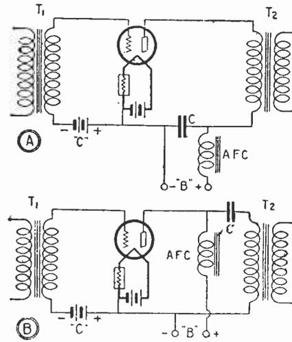
Two methods of using A.F. choke coils and condensers. A is the more usual, and B one used when the plate-supply current is heavy, to keep the plate current from the transformer's primary.
