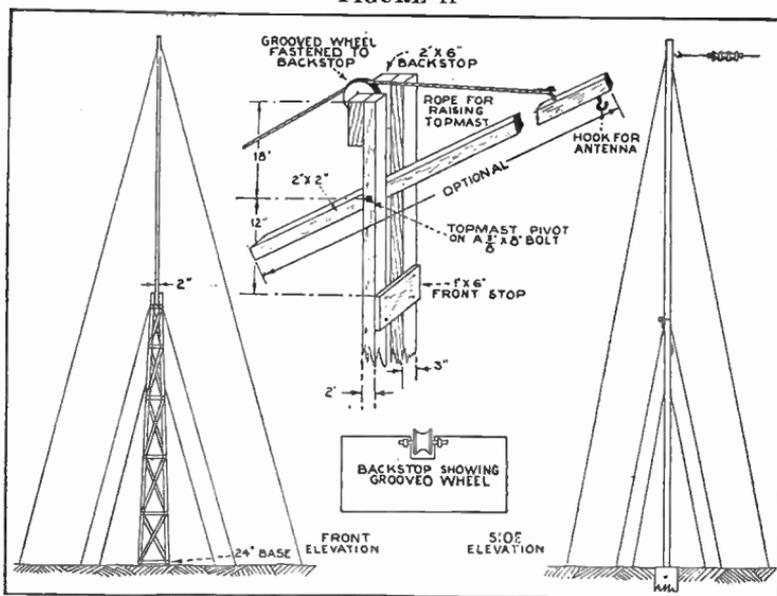
those generally erected, in that the aerial wire and its attachments can be fixed at any time from the ground without lowering the main mast. It is light, but strong, and is pleasing in appearance. These points, ~~coupled with simplicity and cheapness, make it worthy of the attention of the radio fan.~~
