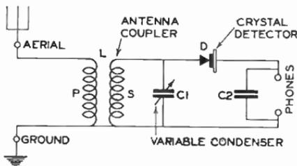
length. The primary winding takes approximately 10 to 15 turns and the secondary winding 90 turns of No. 24 D. C. C. wire.
