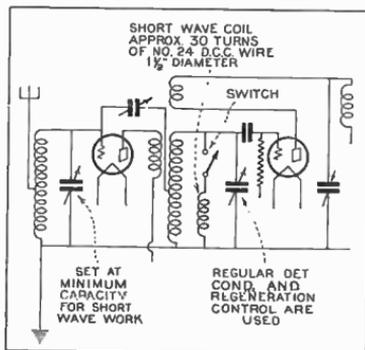
station may be off the dial if the capacity is too great. Get the short-wave stations first before operating on the secondary coil. It is best to use a snap switch set back from the panel and connected with a bakelite shaft.
