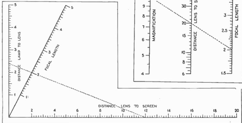
lenses having focal lengths from 1.5 to about 3 inches. Generally speaking, lenses of the larger diameters are designed with longer focal lengths to decrease errors. On the other hand, the greater distance that the screen must be moved out to secure the required magnification precludes the idea of having the screen integral with the television cabinet.
