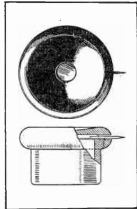
By screwing the nut down onto this expanded portion, the phonograph needle is firmly clamped in place.
