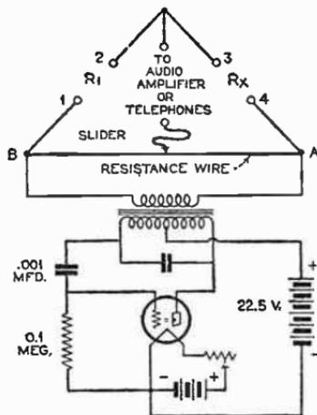
indicating device. For a number of reasons, including the fact that satisfactory meters may not be found in the laboratories of many experimenters, it is suggested that the bridge be designed for a.c.
