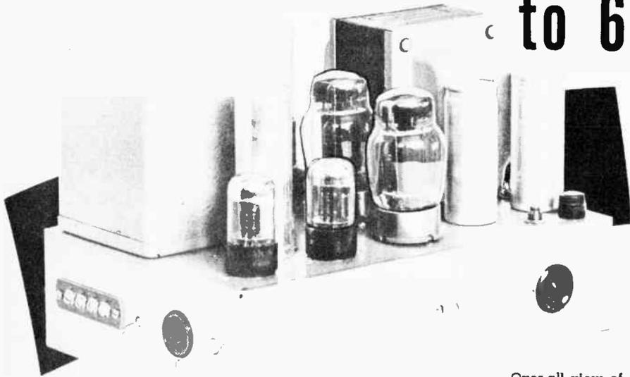
Over-all view of the "Ultra-Linear" amplifier that has been adapted for Tung-Sol 6550's.
