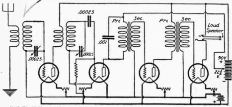
(246) The Unidyne receiver has only two tuning controls. The condenser rotor plates connection for least capacity effect is indicated by the arrowhead location, the point of the arrow designing the side upon which are the rotor plates.
