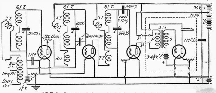
(198) The Super-Zenith circuit. This is a successful method of preventing tube oscillation, without using neutralising condensers. The construction details are quite complete. Regeneration and oscilla-tion in the first tube circuit are perfectly controlled by a variable plate resistance.
