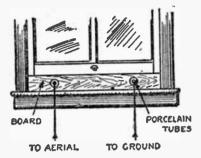
(352) One manner of leading the aerial and ground wires to the receiving set without making holes in the window asah. The window can be raised or lowered without disturbing the wires.
