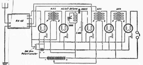
(55) Two Stages of Radio and Two of Audio Frequency Can Be Added to an RA-10 Receiver as Shown Here. Tuned R.F. is Used in the Second Stage for Selective Tuning.
