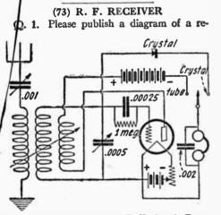
(56) A Crystal or a Tube May Be Used as the Detec-tor in This Circuit by Means of the Single Pole, Double Throw Switch.
