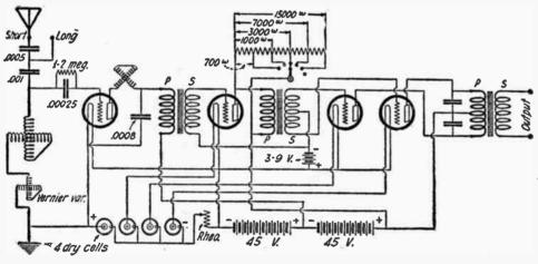
(247) The Circuit of the Radiola Grand. The Push-pull Method of Amplification Is Used, and Special Transformers Are Necessary.
