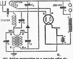
(92) Adding regeneration to a one-tube reflex cir-cuit of standard type. A short serial must be used, selectivity is a prime requisite. Any type of tube may be employed.
