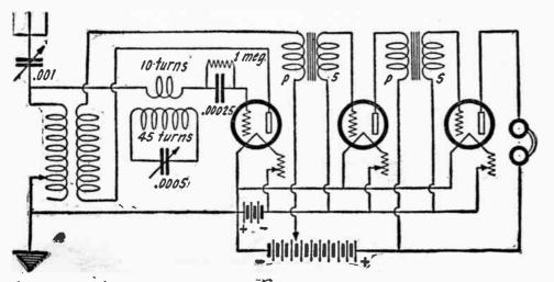
(53) Great Selectivity Can Be Obtained with a Single Circuit Receiver by Using the System Shown Here. Both Coils Are Wound on the Same Tube.
