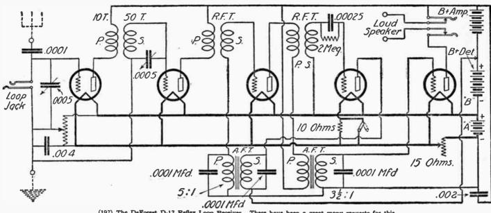
(197) The DeForest D-17 Reflex modern reflex circuit. The second lex Loop Receiver. There have been a great many requests for this The usual crystal detector has been replaced by a tube detector.
