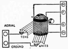
(111-B) The "2-coil variocoupler with tapped pri-mary" unit. This is submitted for those who wish to construct the simple 2-coil variocoupler regenera-tive circuit.
