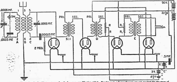
(207) The Heteroplex circuit with two stages of audio frequency amplification added. Regular push-pull transformers are not required for the stage of push-pull amplification. High selectivity, excellent sensitivity and considerable amplification with little distortion are the virtues of this system of connections.
