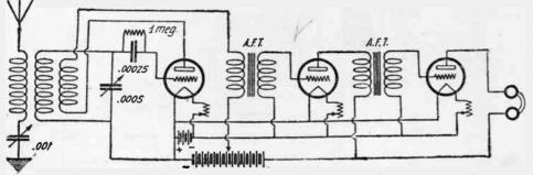
(36) A circuit for the reception of long wave European stations, together with a two-stage amplifier to permit sufficient volume. Honeycomb coils are used for tuning and regeneration.
