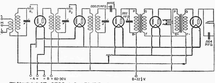
(201) Schematic circuit of "Type F-5" DeForest radio set. Units "R-1" and "R-2"are termed "anti-radiation devices." They control circuit oscillation. Ground is connected to "A" minus. Grid and plate leads must be short, while battery leads may be bunched like a telephone cable.
