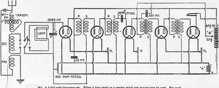
(83) A 2-dial radio frequency set. Either a loop aerial or a regular aerial and ground may be used. For good operation over the entire broadcast wave-length range it will be necessary to use a good make of radio frequency transformer. Dry cell tubes may be used.
