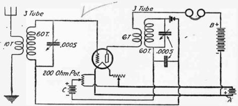
(95) The experimenter will welcome this reflex circuit wherein audio frequency current variations in the .0005 mfd. fixed condenser, due to the rectifying action of the crystal, are impressed upon the grid of the tube, resulting in dual amplification.
