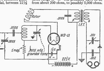
(75) One Stage of R. F. May Be Added to a Standard Three-Circuit Receiver, as Shown Here. No. R. F.
