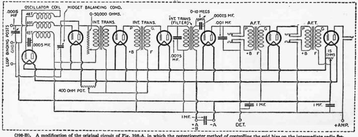
(398-B). A modification of the original circuit of Fig. 398-A, in which the potentiometer method of controlling the grid bias on the intermediate radio fre-quency stages is used. Two stages of audio amplification are used instead of one, as in the original. The 0 to 50,000-ohm variable resistance, which is used as a volume control, may be eliminated.
