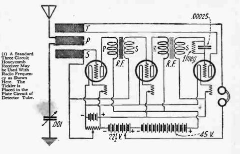
circuit tuner, using the Atwater-Kent twostage amplifier.
