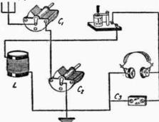
(88-B) A two-dial crystal set. Winding the single coil inductance should present no difficulties to the experimenter. Sharp tuning is not a feature.
