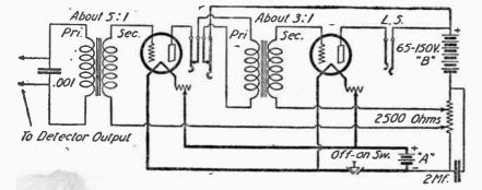
(337-C) "C" battery potential, but no "C" battery. Seemingly paradoxical, explained by the resistance in series with the "B" battery supply. The voltage drop is at negative potential.
