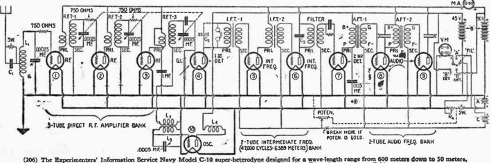
(206) The Experimenters' Information Service Navy Model C-10 super-heterodyne designed for a wave-length range from 600 meters down to 50 meters, the band being covered through the expedient of interchangeable coils. Blueprints are not available.
