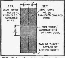
398). Design of an intermediate transformer thich operates with maximum efficiency at 50 to 0 kilocycles. The correct amount of iron core must be determined experimentally. (398). 60
