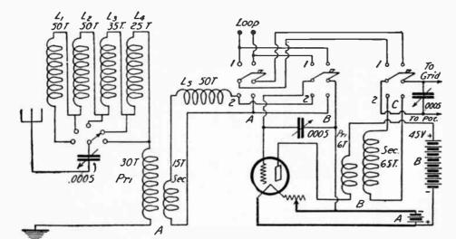
(51) This radio frequency amplifier has been designed to be adaptable to any set using a loop. Some Super-Heterodynes are exceptions. The switches must be well insulated; their bases should be tested for leakage by means of headphones and a battery of about 60 volts. Correct layout of the apparatus is another important consideration.
