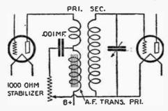
(214-E) The method of oscillation control used in the type 4-DL reflex set.
