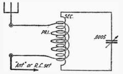
(188) This wave trap may be used with any re-ceiver. The primary may consist of 10 turns of No. 18 S.C.C. wire.
