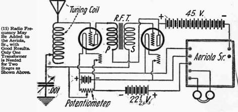
detector and two stages of audio frequency. Q. 3. How is it possible to use a tube as a radio frequency amplifier in conjunction with
