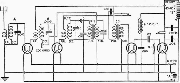
(215) The Double Selector Multiflex circuit of Victor Greiff. This diagram shows two stages of tuned radio frequency amplification and three stages of audio frequency amplification, using a crystal detector instead of the usual tube detector. The second radio frequency tube circuit is reflexed for one stage of audio frequency amplification.
