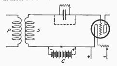
(253) Replacing grid leak and condenser with a "C' battery often increases Super-Heterodyne selectivity.
