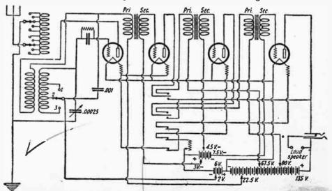
(230) This is the Zenith 3-R circuit. A special switching system for selecting the amplifier stages is used which eliminates the usual jack-and-plug method.
