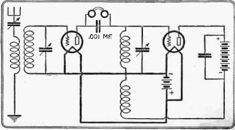
The fundamental principle of the Ultradyne receiver, showing the first detector and circuit employing the efficient modulation system. This method is a radical departure from the conventional, and results in a receiver of remarkable efficiency. (399-C).
