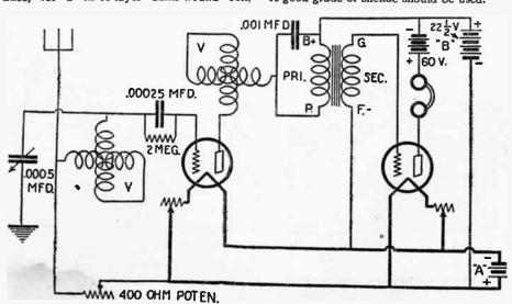
(92-B) A circuit employing the use of two variometers and a potentiometer to control regeneration.
