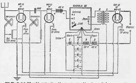
(41) The Radiola III used in conjunction with a two-stage tuned impedance radio frequency amplifier and an extra stage of audio frequency amplification. Note that there are five tubes altogether and that for every tube there is a dry cell.
