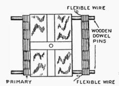
The method used for mounting the coils variometer for the modified Monophase circuit shown on previous page. (390). to the
