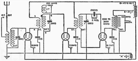
(205-A) The "Airtrola," shown above, and the "Radio Knight" tuned radio frequency receivers both use the "absorption losser" method for preventing oscillation in such receivers. Varying the amount of loss, or absorption, of the circuit by means of a variable resistance makes it possible to adapt the set to any tubes and particular set conditions for maximum results.
