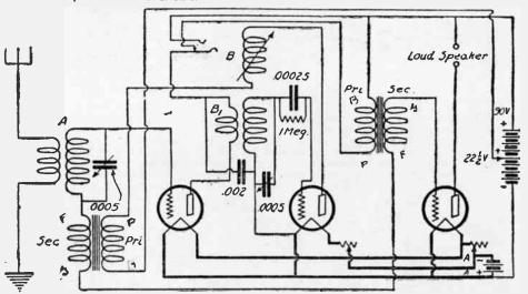
(238) The 3-control Trirdyn circuit is espable of high amplification. One tube is reflexed. It consists of one stage of tuned radio frequency amplification, a detector and two stages of audio frequency amplification.
