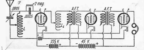
(15) The "Phantom" Circuit. Upon Examination It Will Be Seen That It Is a Single Circuit Tuned Plate Receiver.
