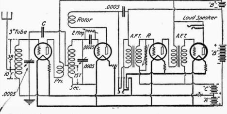
(216-A) Radio frequency amplification added to a regenerative receiver. This is possible only through extremely careful design and construction. This circuit shows how to do it. There are other features to this circuit, the Browning-Drake, as well.
