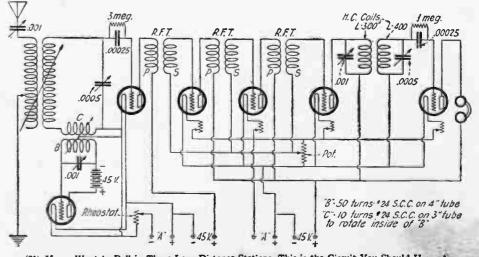
(71) If you Want to Pull in Those Long-Distance Stations, This is the Circuit You Should Use. A Six-Tube Super-Heterodyne, Using Transformer Coupled R.F. Amplification.
