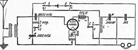
(31) Three combinations may be had with this combination. For tube detector alone place all switches on points 1. For crystal alone the tube is turned out and switches "A" and "B" are placed on point 2. For R. F. amplifier and crystal detector place "B," "C" and "D" on points 2 and "A" on 1.
