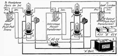
(329) This circuit shows how to connect two stages of audio frequency amplification, both of the push-pull type. A special "interstage" transformer is required. /
