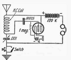
(288) The Colpitts Circuit is an Excellent Oscillator, and Will Give Good Results as a Receiver or a Transmitter.
