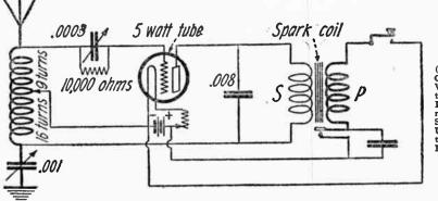
(290) Very Good Results Will Be Ob-tained With the I.C.W. Transmitter. A Spark Coil Is Used to Supply the Plate Potential.
