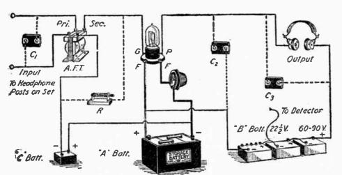
(337-A) Picture diagram of a standard audio frequency amplifier, showing tone quality controls in dotted lines. Connect "B" minus to "A" minus if the balance of set is so connected. A separate current supply may be used for this unit.
