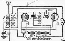
ery Good Results Will be Had by Using One of Tuned Radio Frequency. The Inductance May be the Primary of a Variocoupler.
