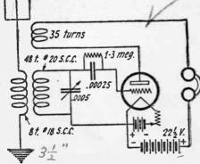
49) Very good results are secured with this circuit using a fixed coupler. A tickler coil provides re-generation.
