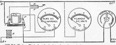
(257) Tube Checker. This is about the simplest and most inexpensive instrument one can have for rapidly determining the D. C. characteristics of vacuum tubes.
