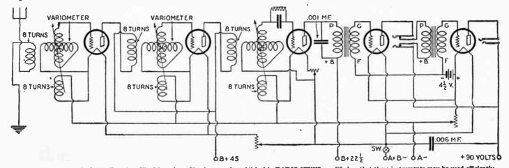
(390-A) Variometers "in fashion" again. The Monophase Circuit, recently published in RADIO NEWS, modified so that these instruments may be used efficiently. The method of mounting the coils necessary to the variometer is shown in another illustration, 390.
