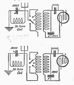
(27) A simple method of sharpening tuning. Both connections shown should be tried.
