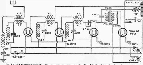
(91-A) The Garrison circuit. An unusual arrangement of coils with the object in view of preventing circuit oscillation, and at the same time retaining selectivity and a negative grid bias of the radio frequency tube grids.
