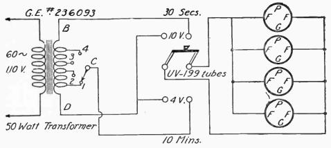
(261) By this simple expedient of applying an alternating current of higher-than-usual value, for a short time, to coated filaments, tubes using this filament construction may be made to function perfectly. This system is only for tubes that light but operate poorly.
