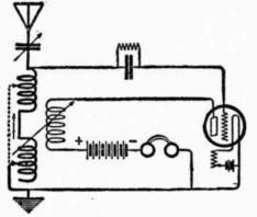
(243) Single circuit tuner with tickler feed-back. The main inductance is split at the center, the tickler thereby being in equal inductive relation to the entire coil.
