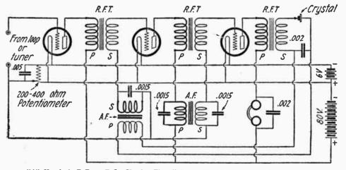
(244) Here is the DeForest Reflex Circuit. Three Tubes Are Used for Five Stages of Amplification. A Crystal is Used for the Detector.
