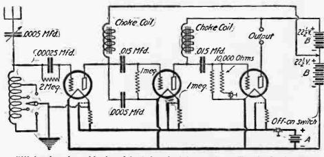
(211) A variocoupler used in place of the single tuning inductance shown will result in considerably sharper tuning. Audio frequency transformer secondaries make excellent choke coils for such a circuit. Being non-oscillating, this receiver cannot radiate, but sensitivity is sacrificed thereby. This is a Signal Corps Airplane receiver.
