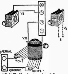
(111-A) The "2-variometer, variocoupler" regener-ative arrangement. This was once the standard of reception circuits, but a demand for simplicity of control forced the "untuned primary" receiver into the lead.
