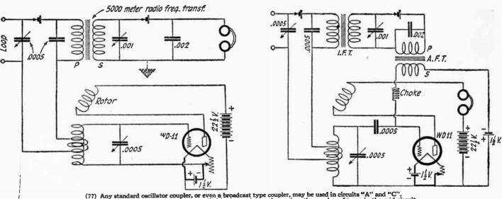
(77) Any standard oscillator coupler, or even a broadcast type coupler, may be used in circuits "A" and "C". The wave-length variation is easily controlled by increasing or decreasing the number of turns in the grid circuit of the oscillator tube. The loop condenser must be of low loss type. Do not use a phone plug for loop connecting.
