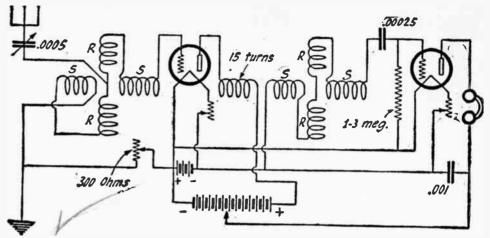
(227) The Circuit Abov e is That Used in the Grebe CR-13 Amateur Short Wave Receiver. This Arrangement Employs Two Split Variometers.
