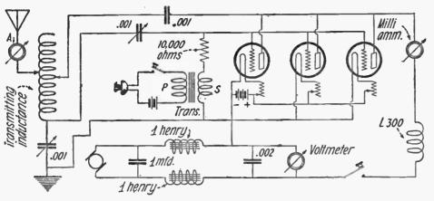
(283) Here is Shown an Efficient 15-Watt Transmitter. The Colpitts Oscillator Circuit is Used and a Very Good Range Can Be Obtained.
