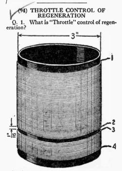
(90-A) A standard two-coil unit. This may be used in a great many different circuits and sets. This is a convenient coil for tapping or otherwise altering.
