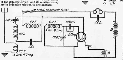
(97) The increasingly popular Filter Circuit is seen to be that of an exceptionally sharp-tuning, complete receiver. Careful instrument layout, careful construction and good apparatus will be required for best results.
