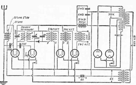
(23) A receiving circuit equipped to derive the necessary "A" and "B" potentials direct from a 110-volt alternating current source. A rectifier and filter system is utilized to eliminate the A. C. hum.
