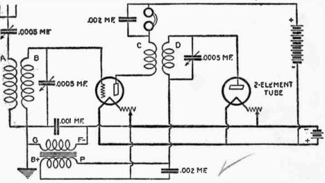
(90-B) A two-tube reflex. In this circuit a two-element tube supplants the usual crystal detector or three-element tube detector. The descriptive text is quite complete. Battery potentials and condenser values should be varied for best results.
