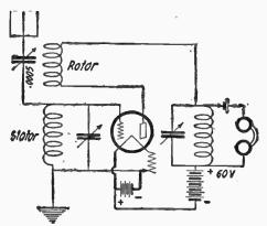
(24) A circuit employing the vacuum tube as a radio frequency amplifier and a crystal as the detector. This circuit should prove quite sensitive and selective. detector.
