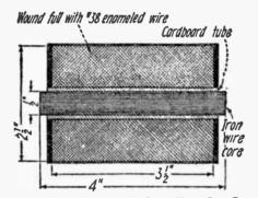
(328) Constructional Details of a 30 Henry Iron Core Choke Coil To Be Used in a Power Amplifier Circuit.
