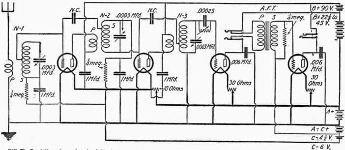
(202) The Garod Neutrodyne. A study of this circuit shows it to be one difficult to surpass, where a prime requisite is tone quality, yet also, it is extremely sensitive. Although reception may be excellent at the detector, a very careful audio frequency amplifier design must be employed to retain this quality. Note resistances in the radio frequency amplifier grid return leads.
