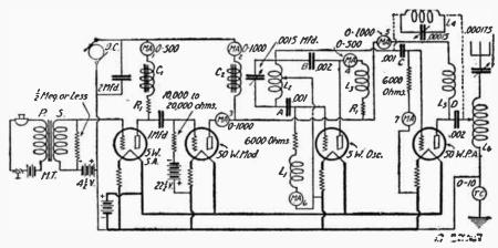
(280) This is the schematic diagram of one of the most efficient radiophone transmitters it is possible to construct. Constant wave-length and nearly complete modulation are outstanding features of this exceptionally efficient transmitter.
