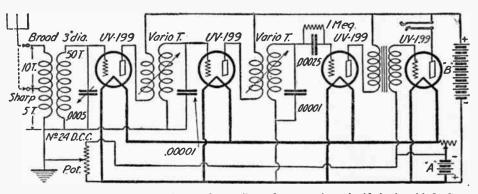
(189-D) Voltage step-up through the use of two-coil transformers, and tuned grid circuits with fixed condensers, are outstanding features of this receiver. Loud speaker reproduction of local signals, and loud headphone reproduction of very distant stations, using only dry cell tubes, is had.
