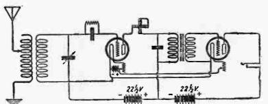
a six volt, 80-ampere storage battery for heating the tube filaments and 45 volts "B" battery for the amplifier plates with a tap off at  $22\frac{1}{2}$  volts for the detector tube.
