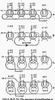
(214-A, B, C, D) The sequence of amplification in four different circuits is depicted above.
