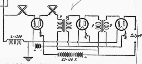
(64) Audio Frequency Can Be Added to the Autoplex Circuit in the Usual Manner. A Loud Speaker Must Be Used with Two Stages.
