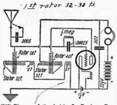
(245) Diagram of the Aeriola, Sr. Receiver. Two Variometers Are Used, Ont as the Tuning Unit and the Other in the Plate Circuit.
