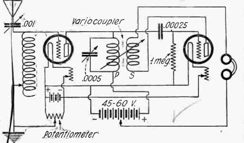
(70) One Stage of Tuned Radio Frequency Amplification Can Be Used in a Regenerative Receiver By Following This Circuit.
