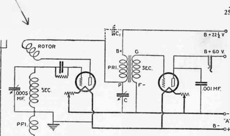
(94) A regenerative circuit employing the use of inductive and capacitative feed-back, termed "throttle control."
