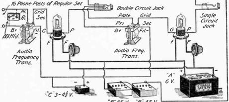
(337-B) If this picture diagram is followed correctly, no one should have any difficulty in adding audio fre-guency amplification to any set.
