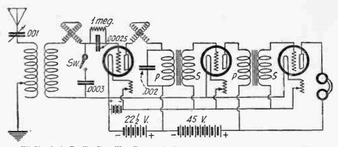
(69) Here is the Familiar Short-Wave Regenerative Receiver. This Circuit is Hard to Beat for Efficient Results. A Small Fixed Condenser is Used in the Secondary Circuit for Higher Wave-Lengths.
