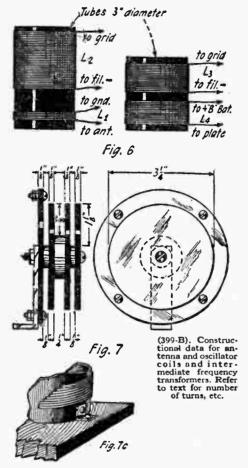
Using only the secondary coil, composed of 72 turns of wire wound on a tube 3 inches in diameter, stations in Cincinnati, Detroit, Atlanta, Chicago and other cities are heard practically every night and with good audi-bility. No audio-frequency amplification is used, and no loop, aerial or ground is con-nected to the receiver. With one or two stages of audio frequency the loud speaker may be operated and, of course, the music and speech are audible throughout the apartment.
