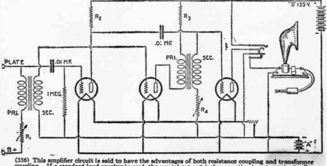
(336) This amplifier circuit is said to have the advantages of both resistance coupling and transformer coupling. If a standard loud speaker is used, the special out-put jack connection is not required. Do not place the audio transformers too close, and connect their cases or cores to "A" minus.
