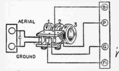
(111-C) The "3-coil honeycomb" regenerative unit. The standard way of receiving long-wave stations.
