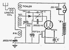
(92-A) A three-circuit tuner, arranged so that a crystal detector, grid leak and condenser, or grid bias method, of rectification may be obtained.
