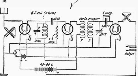
(62) Here is the Best Method of Adding Two Stages of Tuned Radio Frequency Amplification to a Three-Circuit Regenerative Receiver. The Variocoupler is Used as Tuned R.F. Transformer.
