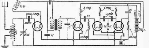
(332) Resistance Coupled Push-Pull Amplification is employed in this circuit. Tubes of 5-watt size will be better than the usual type for the power tubes. Use a plate voltage of 200.
