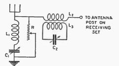
(393). An exceedingly efficient wave-trap to elim-inate that "local station" interference. The cir-cuit is similar to that employed by broadcast sta-tions to "eliminate their own" interference, thus enabling them to listen to other stations.
