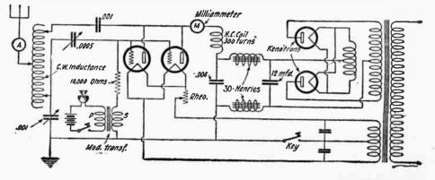
(282) Here is the Circuit for a Good 10-Watt C.W. and Phone Transmitter. Kenotron Tubes Are Used to Rectify the Plate Voltage.
