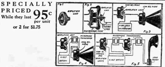
**ICROPHONE** Transmitter Buttons have been used for a number of years to make powerful sound transmitting elements. These very sensitive amplifiers offer every "Radio Fan" the means of building his own powerful speech amplifier. We offer herewith to the constructor these special Amplifier Units.
