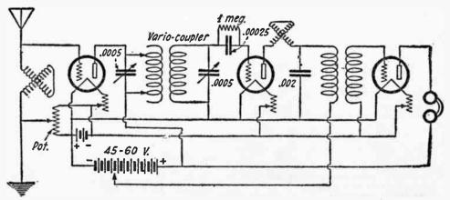
(13) Here is Shown the Best Method of Using One Stage of R.F. Amplification with a Standard Regenera-tive Receiver.
