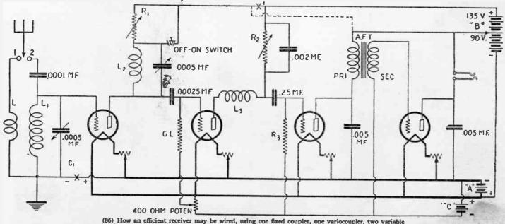
(86) How an efficient receiver may be wired, using one fixed coupler, one variocoupler, two variable condensers and two variable plate resistors, in addition to the customary equipment. Coils L2 and L3 are in inductive relation to one srother.
