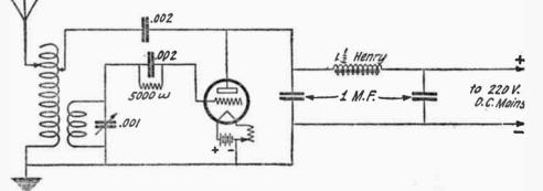
(286) A five-watt C.W. transmitter circuit of the reversed feed back type employing 220 volts D.C. for the plate supply. A choke coil and two fixed condensers serve to smooth out the commutator ripple of the generator. The key is placed in series with the negative side of the 220-volt main.
