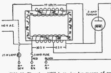
(323-A) Charging "B" batteries by means of an "A" battery-charger of the regular 2-ampere or 5-ampere type.
