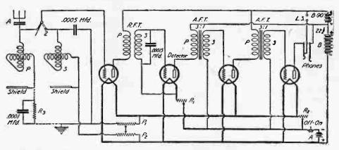
(217) The Amrad "Inductrole." Variometers are employed in an efficient manner. The receiver is so designed that grid current leakage through the set is just sufficient to prevent the first tube from "blocking." The commercial receiver reproduces with excellent fidelity.
