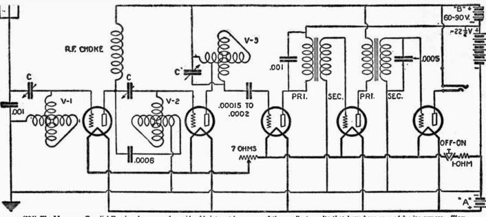
(204) The Magnavox One-dial Receiver has aroused considerable interest by reason of the excellent results that have been secured by its owners. white knobs control the "ratio condensers" used to balance the circuits to the particular tubes and local conditions encountered. Tiny
