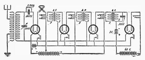
(54) Plenty of Volume Will Be Had from This Three Stage Audio Frequency Amplifier. A Separate "B" Battery is Used on the Plate of the Last Amplifier Tube.
