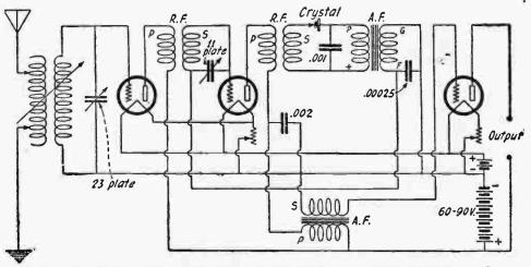
(217-A) Remarkable Results Are Claimed for the Erla Triplex Circuit Shown Here When Erla Transfor-mers and Fixed Crystal Detectors Are Used.
