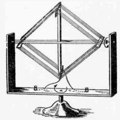
(368) The Gimbal Loop. Wave front of broadcast signal travels in vertical plane, while that of some forms of static is said to travel horizontally, en-abling one to balance out either, optionally, with a gimbal-mounted loop.
