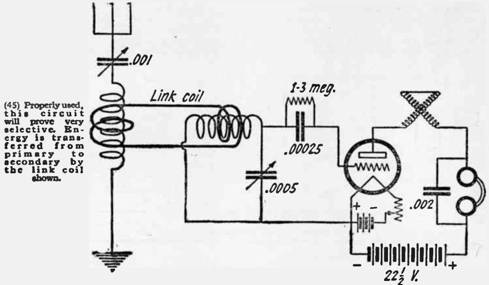
(45) Properly used, this circuit will prove very selective. Energy is transferred from primary to secondary by the link coil shown.
