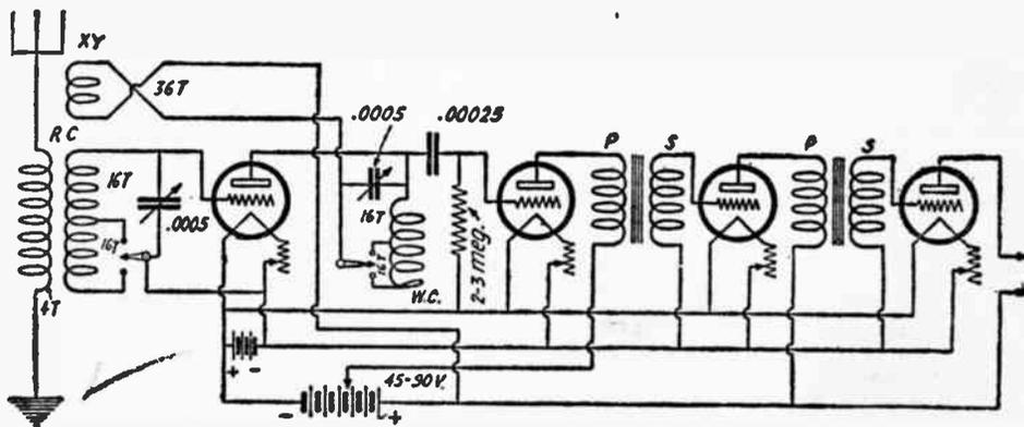
(228) The Superdyne circuit with two stages of audio frequency. Reversed feed back controls the oscillation of the R. F. tube.
