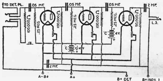
the filaments of the tubes of the receiver are placed in series instead of the conventional parallel method. Parts necessary are:
