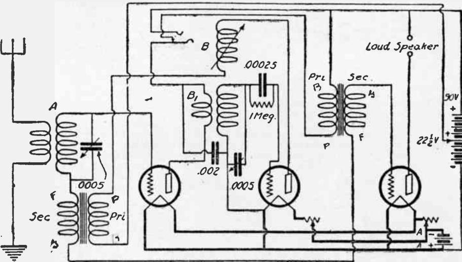
(238) The 3-control Trirdyn circuit is capable of high amplification. One tube is reflexed. It consists of one stage of tuned radio frequency amplification, a detector and two stages of audio frequency amplification.
