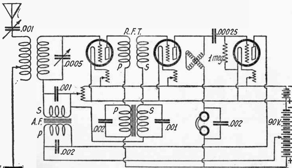
(66) Tuned R.F. Amplification May Be Used in a Reflex Circuit by Following This Diagram. Only One Stage Is Tuned and It Must be Next to the Detector.
