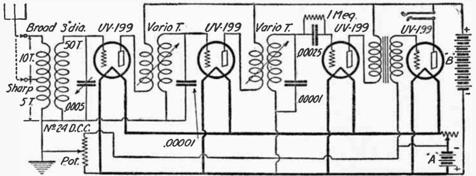
(189-D) Voltage step-up through the use of two-coil transformers, and tuned grid circuits with fixed condensers, are outstanding features of this receiver. Loud speaker reproduction of local signals, and loud headphone reproduction of very distant stations, using only dry cell tubes, is had.
