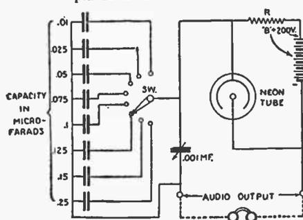
(377) An audio frequency oscillator, involving the use of a Neon tube.
