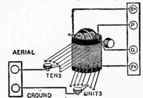
(111-B) The "2-coil variocoupler with tapped primary" unit. This is submitted for those who wish to construct the simple 2-coil variocoupler regenerative circuit.
