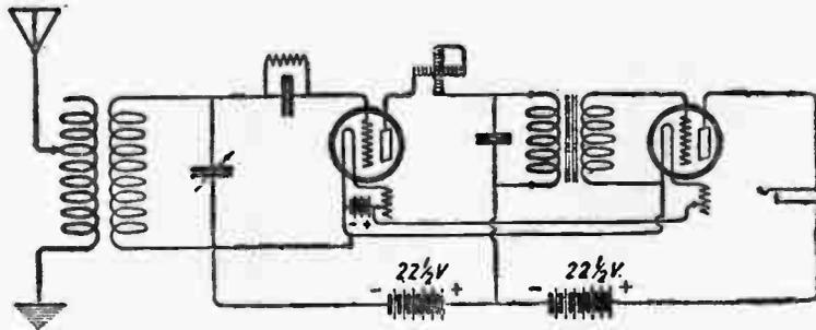
use a six volt, 80-ampere storage battery for heating the tube filaments and 45 volts "B" battery for the amplifier plates with a tap off at 22 1/2 volts for the detector tube.
