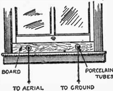
(352) One manner of leading the aerial and ground wires to the receiving set without making holes in the window sash. The window can be raised or lowered without disturbing the wires.
