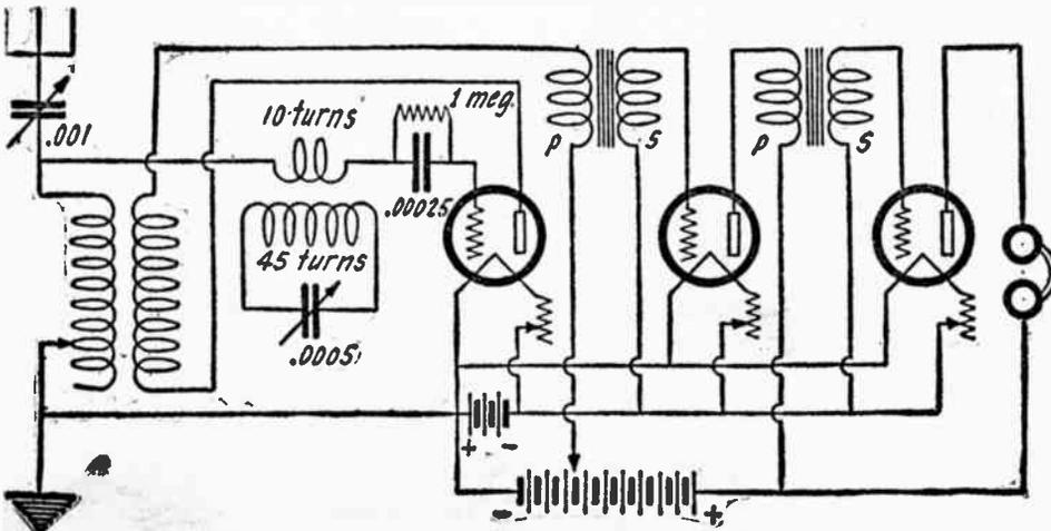
A. 1. This circuit appears in these columns. Iron-core transformers, designed to operate efficiently on 3,000 meters, are used.
