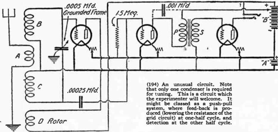
(194) An unusual circuit. Note that only one condenser is required for tuning. This is a circuit which the experimenter will welcome. It might be classed as a push-pull system, where feed-back is produced (lowering the resistance of the grid circuit) at one-half cycle, and detection at the other half cycle.
