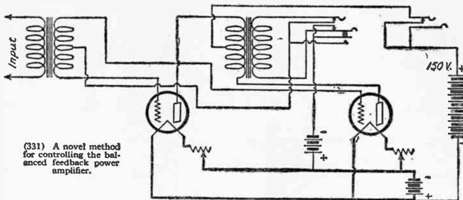
(331) A novel method for controlling the balanced feedback power amplifier.
