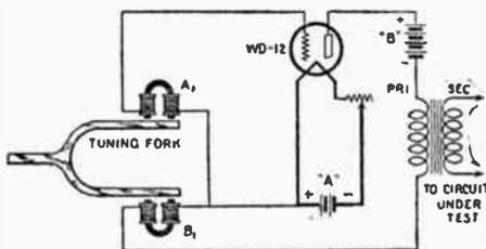
(375-A) Maintaining constant vibration of a tuning fork, by means of a vacuum tube. An application of the device is described.
