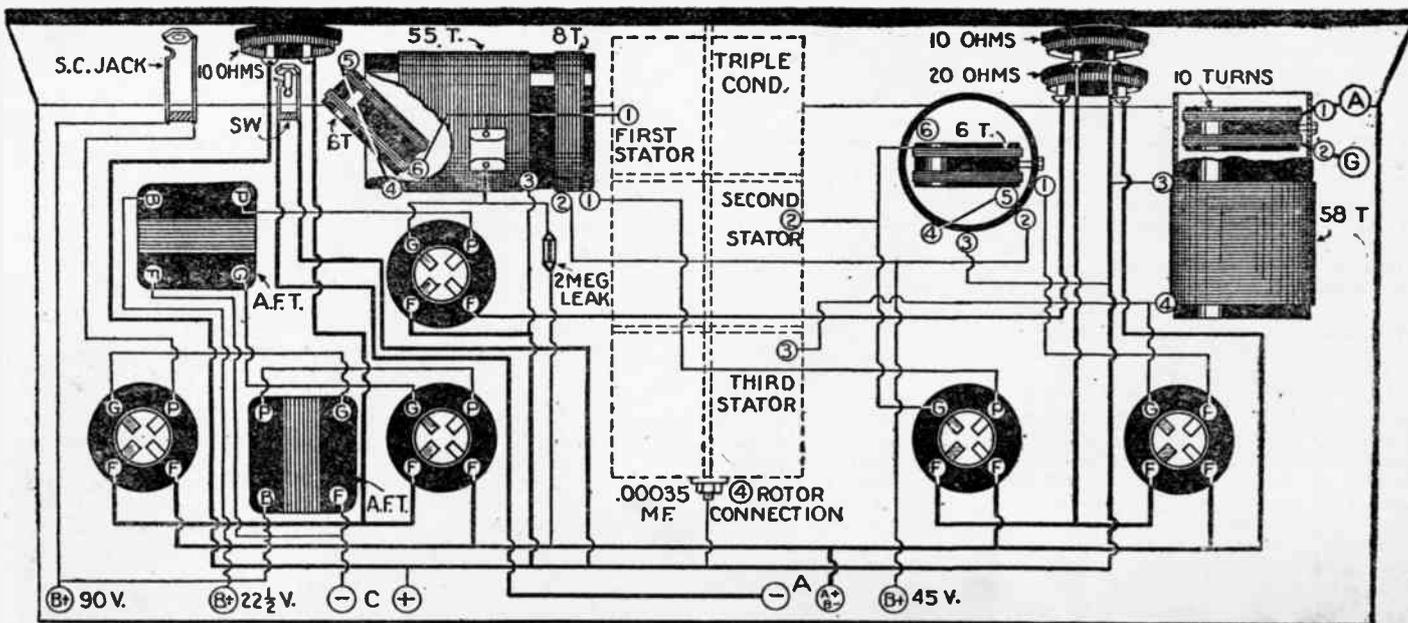
(400A). The Journal One-Knob, five tube, receiver consisting of two stages R. F. amplification, regenerative detector, and two stages A.F., extremely efficient and selective receiver, although only one dial is employed for tuning. Any type of tubes may be employed in this receiver, although for best results it is advisable that storage-battery type, 201-A or 301-A tubes be used throughout.
