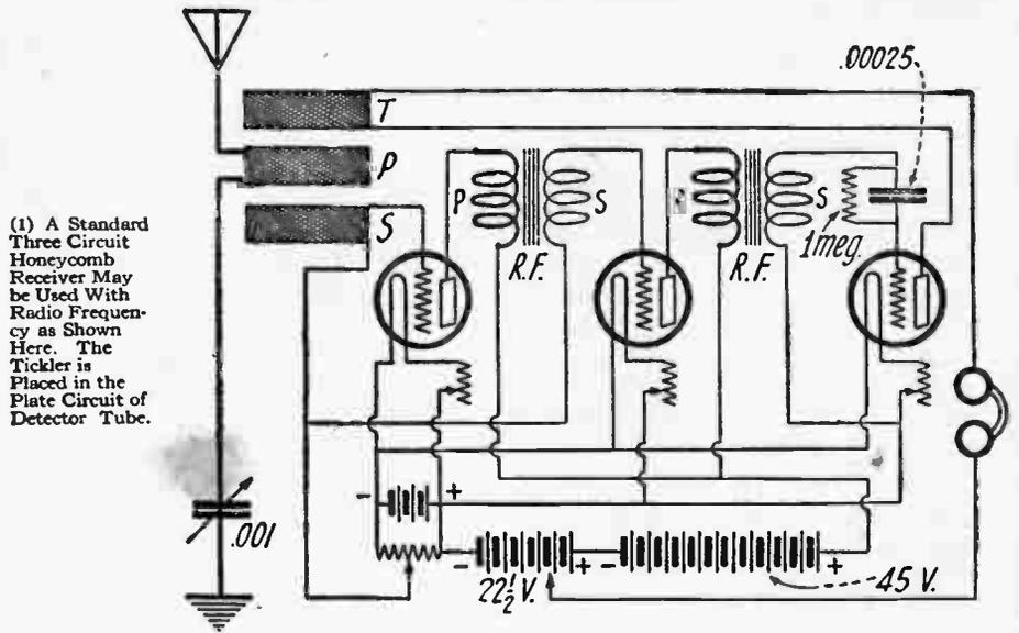
(1) A Standard Three Circuit Honeycomb Receiver May be Used With Radio Frequency as Shown Here. The Tickler is Placed in the Plate Circuit of Detector Tube.
