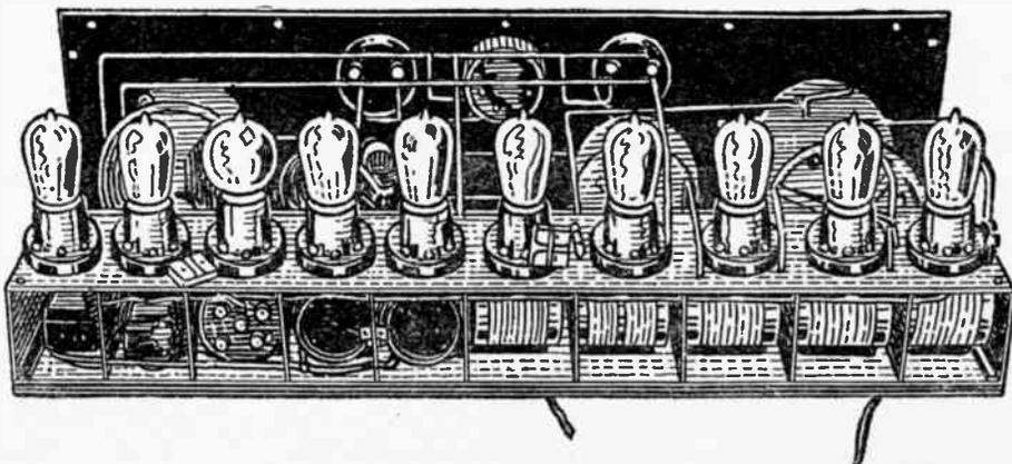
(206) How "the makin's" of the E.I.S. super-heterodyne look when put together. All the sockets are on a metal panel or a strip. General Radio No. 271 I.F. transformers and filter were used. Note vertical shields between each unit.
