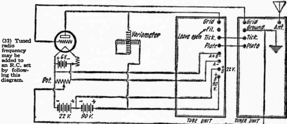
(32) Tuned radio frequency may be added to an R.C. set by following this diagram.
