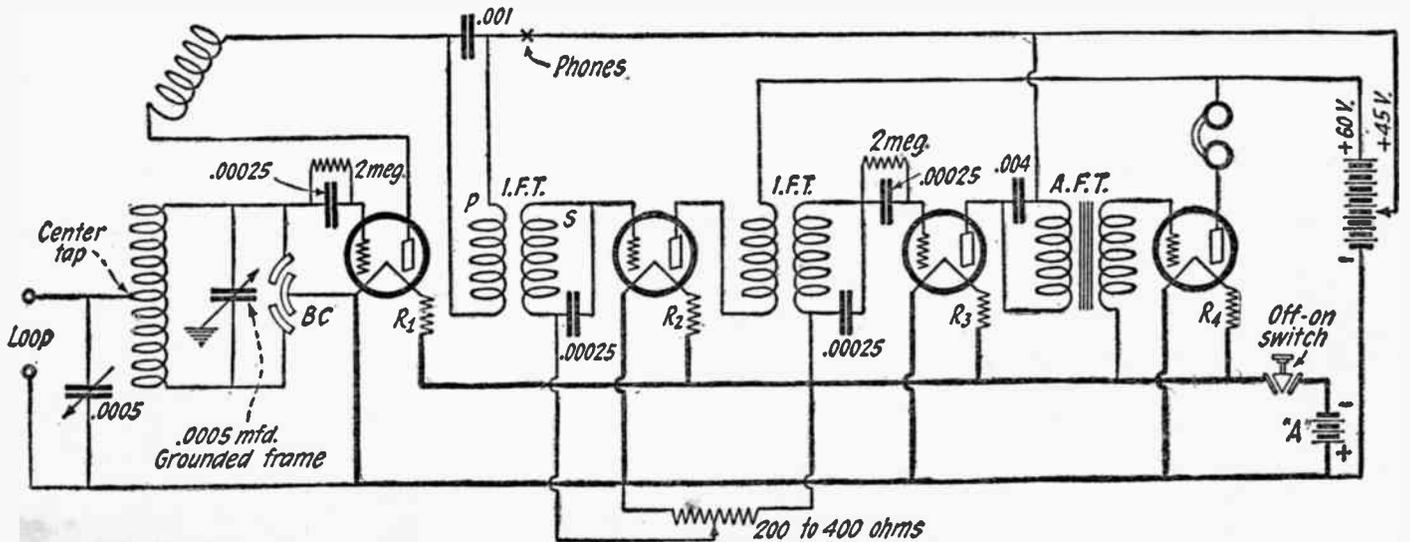
(216) A variation of the Tropadyne principle described in the August, 1924, issue of *RADIO NEWS* is here illustrated as the new Signal Corps Super-Heterodyne. Additional stages of intermediate frequency amplification may be added if desired.
