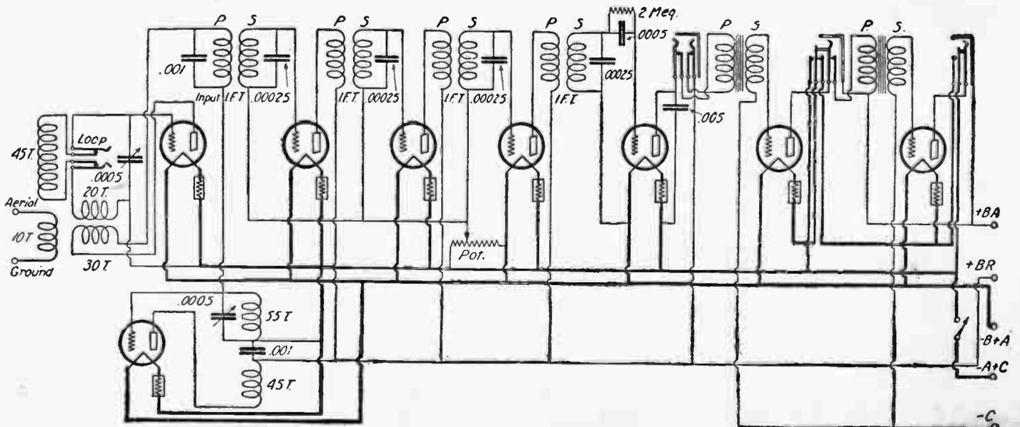
(192) The Model L-2 Ultradyne is seen to incorporate the latest developments in Super-Heterodyne construction. While the major portion of the amplification at radio frequency is dependent upon a properly designed and constructed intermediate frequency amplifier, considerable additional selectivity and sensitivity are had by the incorporation of regeneration in the first tube, as shown.
