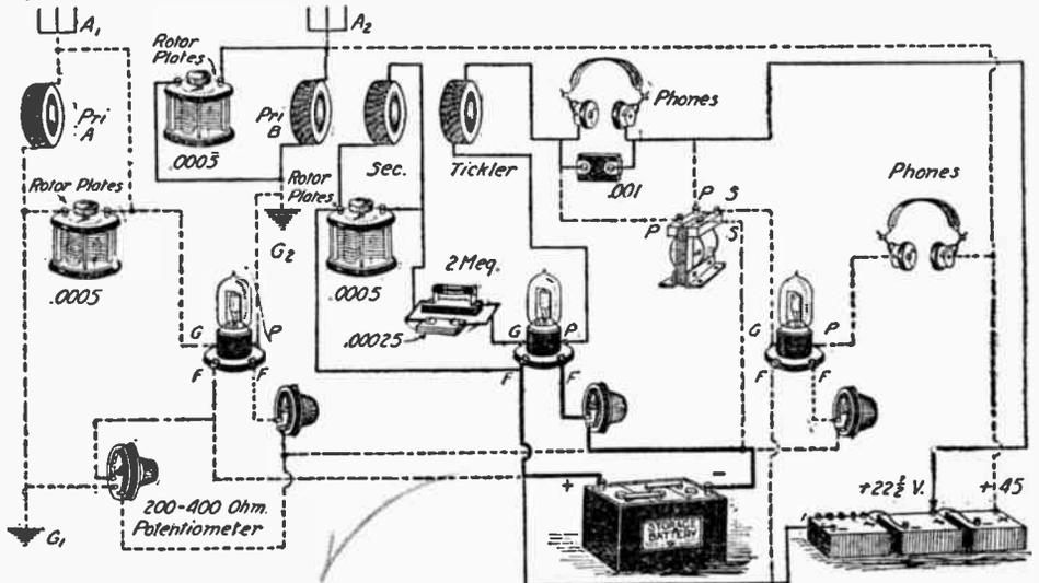
(79) One stage of tuned radio frequency amplification and one stage of transformer coupled audio frequency amplification may be easily added to the three-honeycomb type of regenerative receiver, as shown in this picture diagram.
