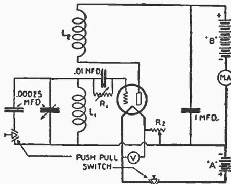
(370) The "Buzzerdyne." An improved wavemeter. By peculiar electrical action, a pure audio note modulation is obtained.
