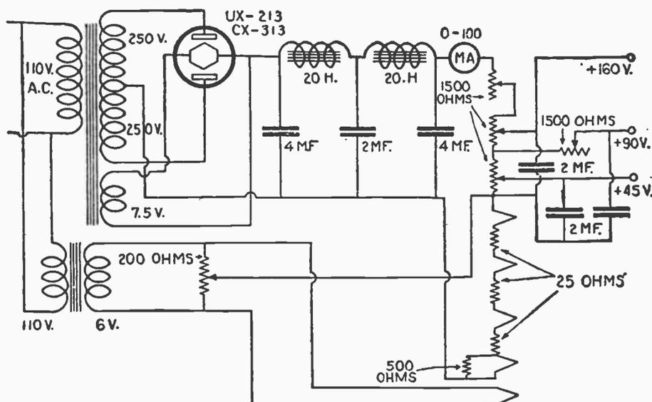
(391). "Just what you wanted." An "A," "B" and "C" battery eliminator, giving an unusually "pure" output, free from A.C. hum or distortion. Note that the filaments of the receiving tubes must be connected "in series," instead of the usual "parallel method."
