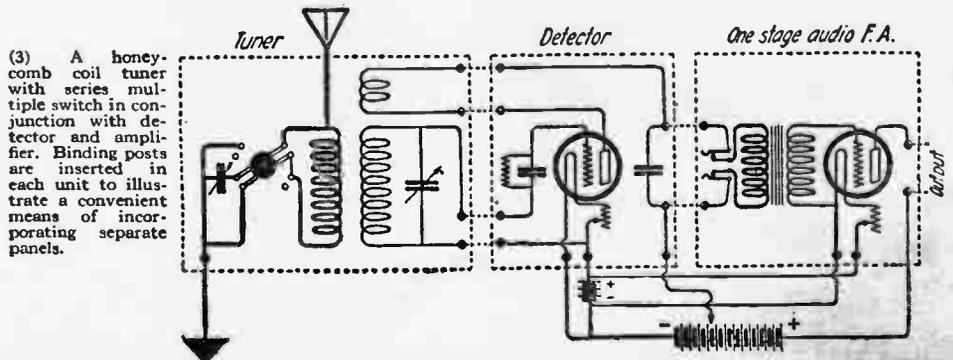
(3) A honeycomb coil tuner with series multiple switch in conjunction with detector and amplifier. Binding posts are inserted in each unit to illustrate a convenient means of incorporating separate panels.
