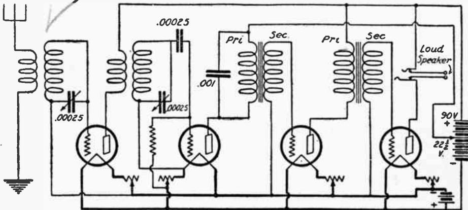
(246) The Uniodyne receiver has only two tuning controls. The condenser rotor plates connection for least capacity effect is indicated by the arrowhead location, the point of the arrow designating the side upon which are the rotor plates.
