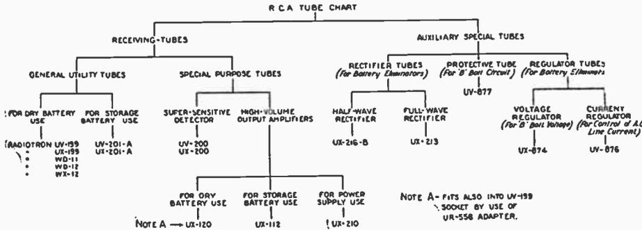
(258) This chart may be used to determine the best tube for receivers, both plain and those employing various methods of amplification, or using dry cells in place of storage batteries.
