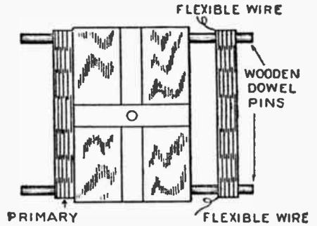
(390). The method used for mounting the coils to the variometer for the modified Monophase circuit shown on previous page.
