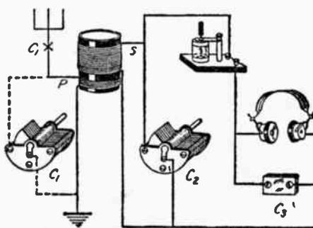
(88-C) A very simple crystal set. The inductance coil shown may be a standard two-coil vario-coupler either tapped or untapped.
