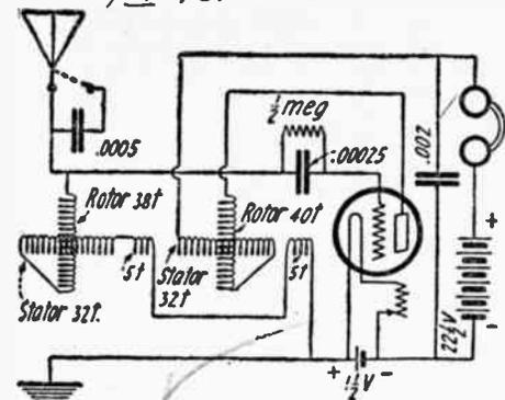
(245) Diagram of the Aeriola, Sr. Receiver. Two Variometers Are Used, One as the Tuning Unit and the Other in the Plate Circuit.
