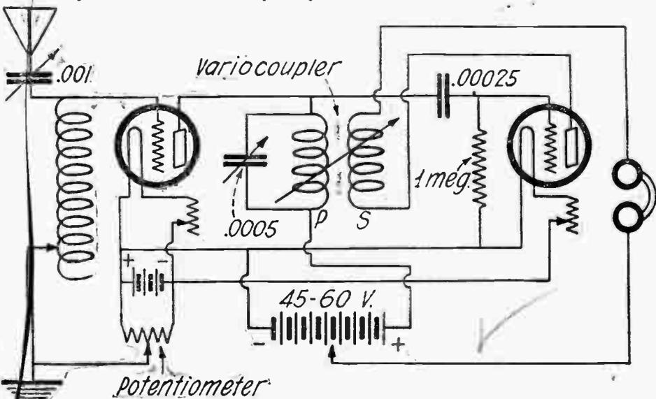
(70) One Stage of Tuned Radio Frequency Amplification Can Be Used in a Regenerative Receiver By Following This Circuit.
