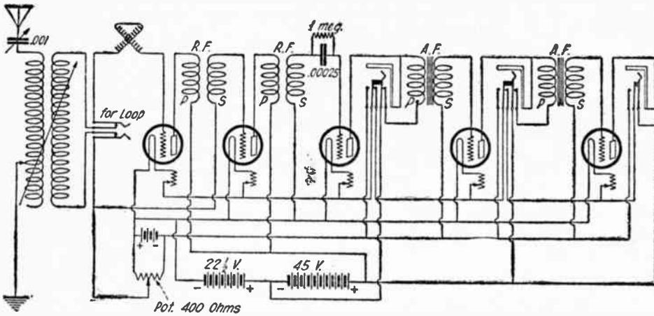
(73) This Circuit Will Give Very Good Results, if Correctly Handled. Two Stages of Radio and Two Stages of Audio Frequency Amplification Are Shown.
