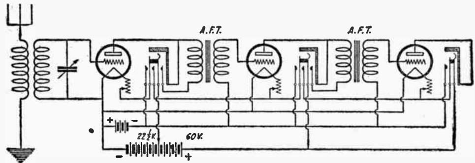
(11) Filament connections may be employed in any circuit in place of double circuit jacks. This diagram shows the proper connections.
