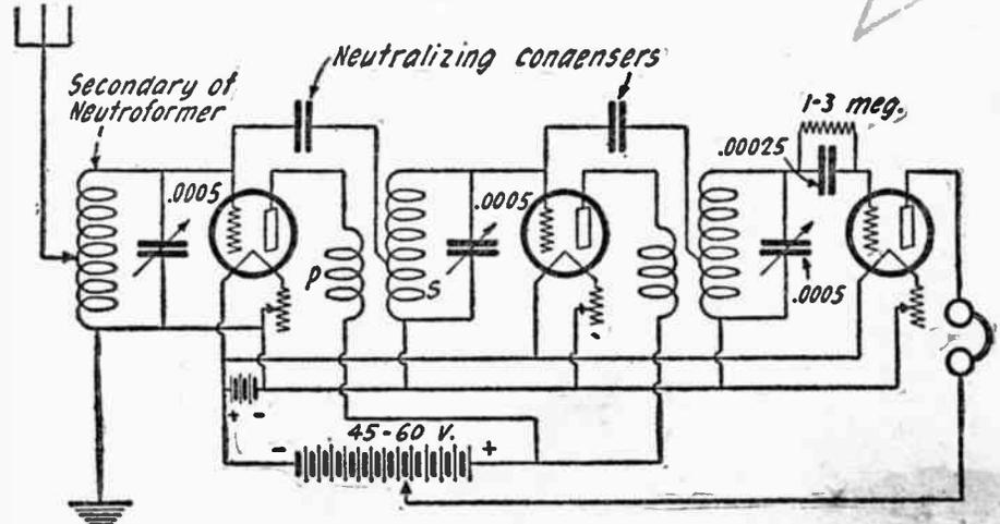
(60) The Neutrodyne Circuit Using Two Stages of Radio Frequency. The Secondary of the First Neutrodyne is Used as the Tuner.
