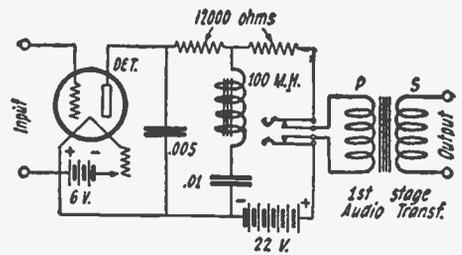
(366) A filter system consisting of two resistances, two fixed condensers and a choke coil will help materially to eliminate stray noises in any form of receiving set.
