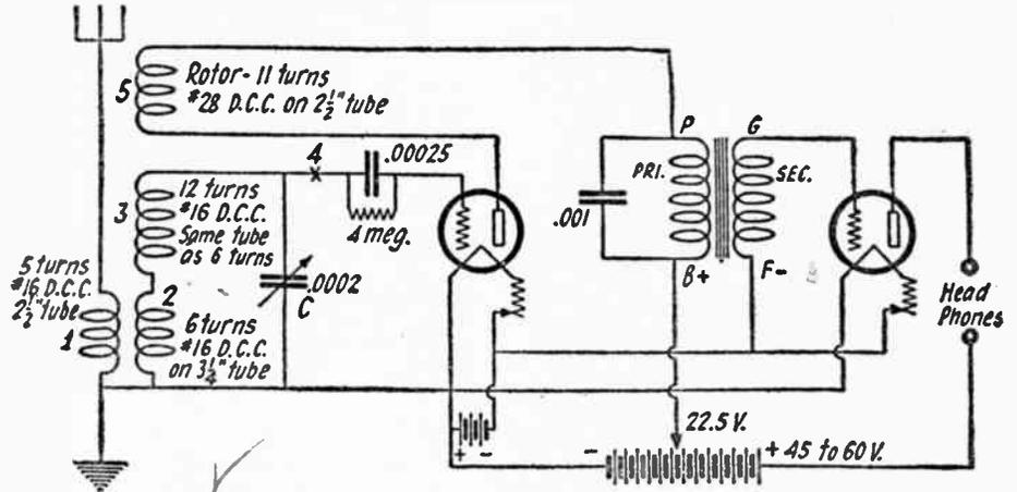
(101) Low losses and a minimum wave-length of 65 meters are the features of this set. It is primarily designed for the reception of telegraphic code signals.
