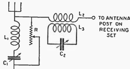
(393). An exceedingly efficient wave-trap to eliminate that "local station" interference. The circuit is similar to that employed by broadcast stations to "eliminate their own" interference, thus enabling them to listen to other stations.
