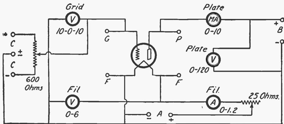
(256) Direct current tube characteristics are indicated with test sets connected as shown. A different circuit arrangement is required for determining the exact characteristics under alternating current conditions.
