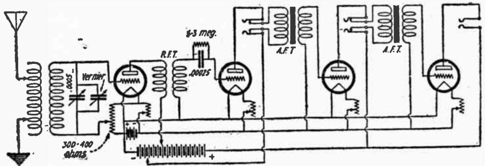
(222) Circuit diagram of the Federal Type 59 Receiver. This employs one stage of transformer coupled radio frequency amplification and two stages of audio frequency amplification.
