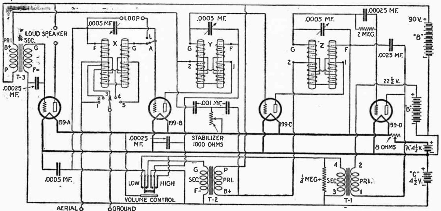
314) This type 4-DL Grimes Inverse Duplex (reflex) circuit. This is one of the latest developments of the reflexed principle. There is wide room for experiment in this field. Note the "C" battery biasing all amplifier tube grids, resulting in low "B" battery consumption.
