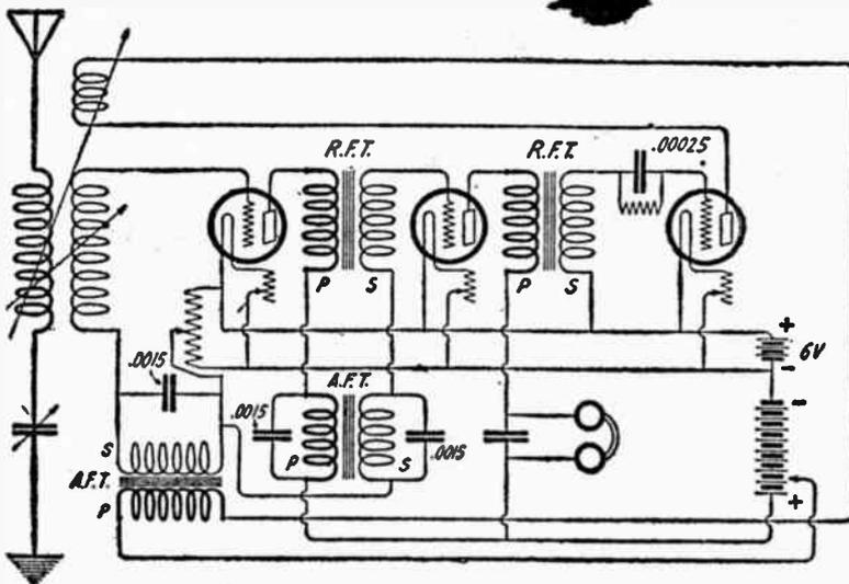
(9) In this circuit, the same tubes are used for both radio and audio frequency amplification. Ticker feedback regeneration is also employed.
