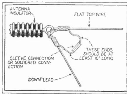
Fig. 286. Careful attention should be paid the connection of the lead-in to the aerial proper. Above is illustrated the best method for making this joint so that it will be strong and electrically perfect.
