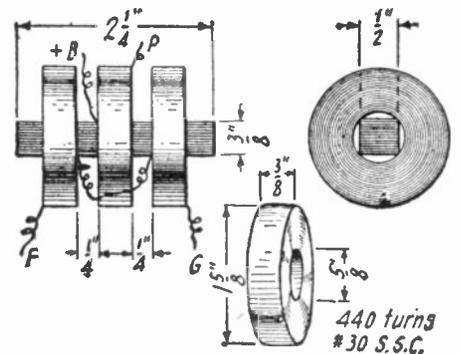
Fig. 244E. The design of a tuned intermediate-frequency transformer, employing an iron core. A small variable condenser, approximately .00025-mf., is connected across the secondary and varies the wave-length range from approximately 2,000 to 7,000 meters.
