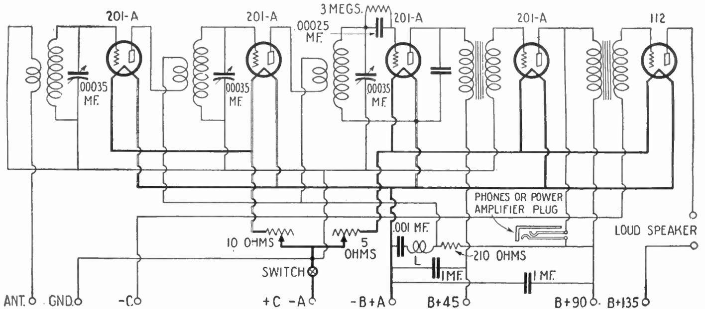
Fig. 162. The latest available circuit diagram of the Freshman Masterpiece three-control receiver. A special R.F. choke and a fixed resistance, which do not appear in the earlier types, are employed in this receiver. The receiver is also designed for power-tube operation.
