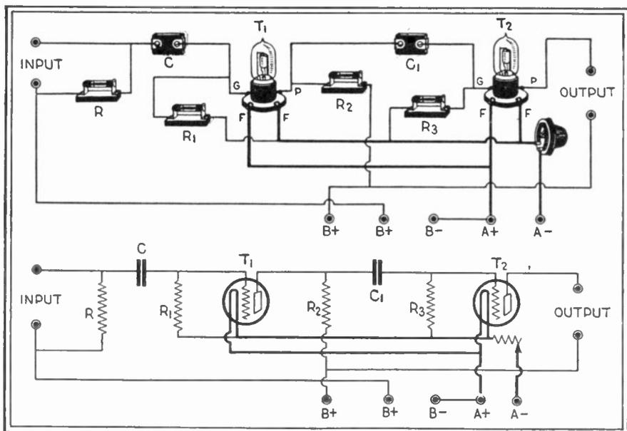
Fig. 222. A resistance-coupled amplifier is comparatively inexpensive to construct and two stages will give fair volume although not as much as a two-stage transformer-coupled amplifier. The above diagram shows a standard two-stage resistance-coupled amplifier.
