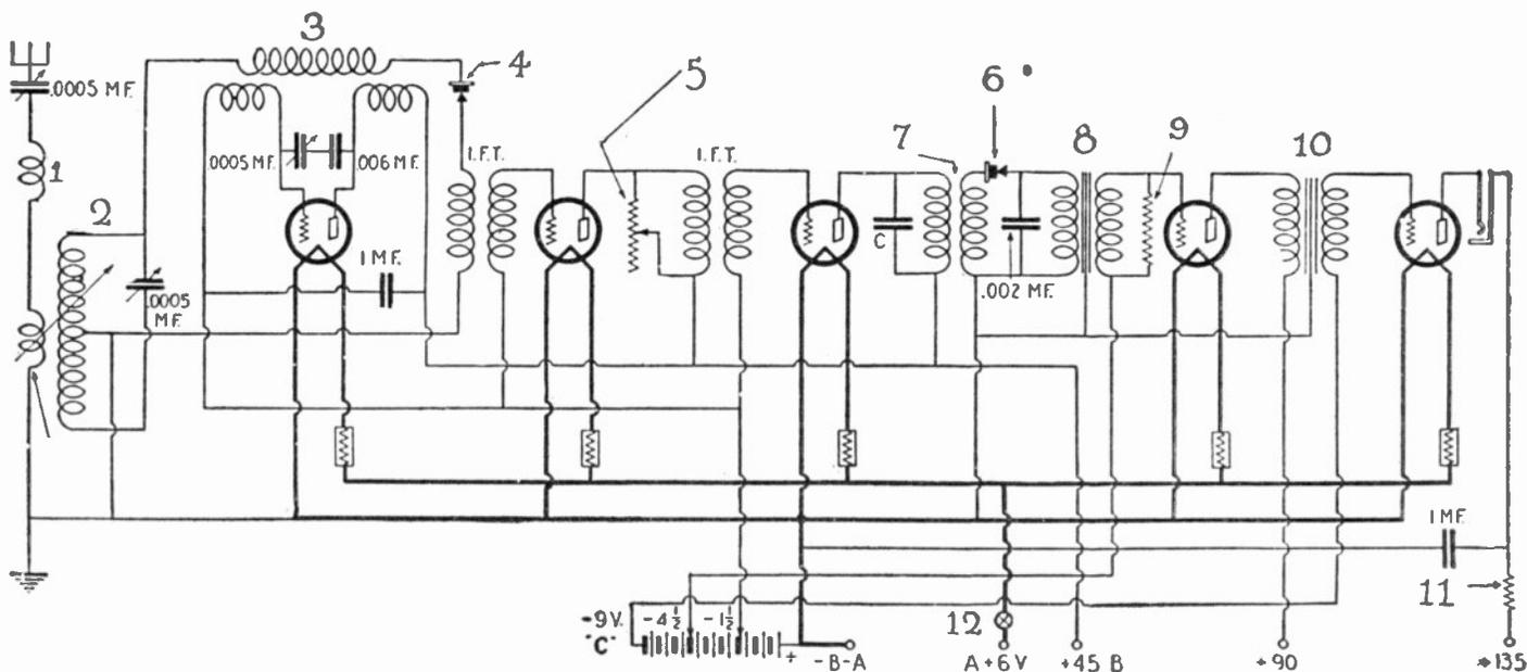
Fig. 88. Best's 5-tube super. An innovation in supers, in that three tubes are eliminated by means of two crystal detectors. Although the sensitivity of the original receiver decreases somewhat, the set is unusually efficient and will satisfy particular constructors, especially as regards DX, volume, and clarity.
