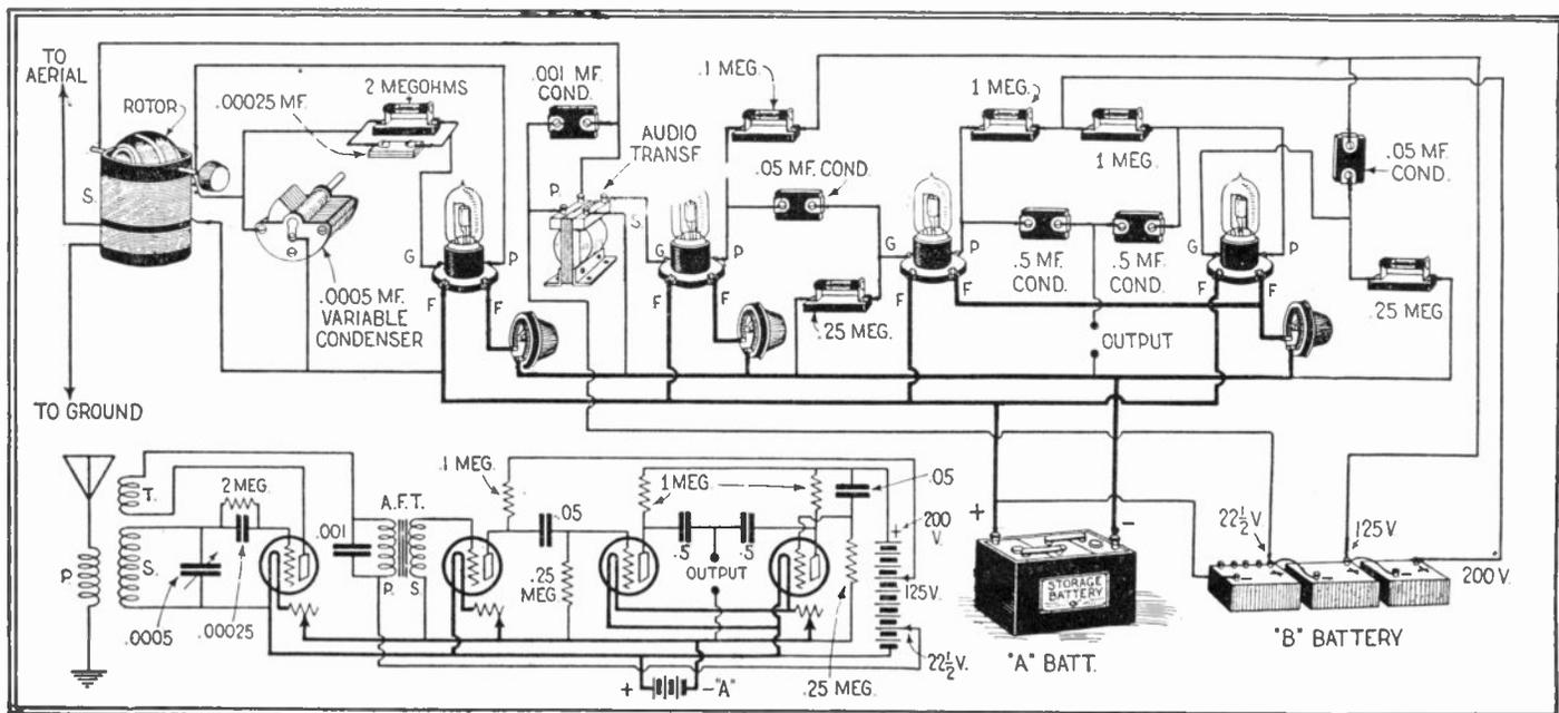
Fig. 221 Resistance-coupled audio-frequency amplification is claiming quite a bit of attention in the radio world today, and above we show a very unusual circuit employing resistances for coupling vacuum tubes together in a push-pull audio-frequency amplifier circuit. Since all of the values are given in the schematic and pictorial circuits, the interested experimenter should find no trouble in trying out this circuit.
