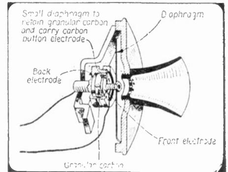
Fig. 307. Above: A cross-section view of a standard telephone microphone employing carbon granules for varying the current in accordance with the fluctuations of the voice.
