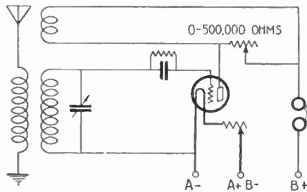
Fig. 130. One of the simplest methods of controlling regeneration.
