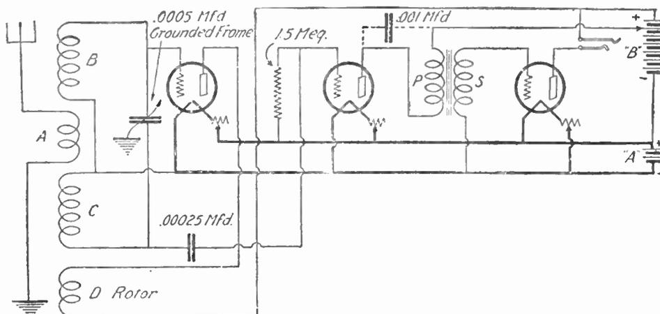
Fig. 70. An unusual circuit. Note that only one condenser is required for tuning. This is a circuit which the experimenter will welcome. It might be classed as a push-pull system, where feed-back is produced (lowering the resistance of the grid circuit) at one-half cycle, and detection at the other half cycle.
