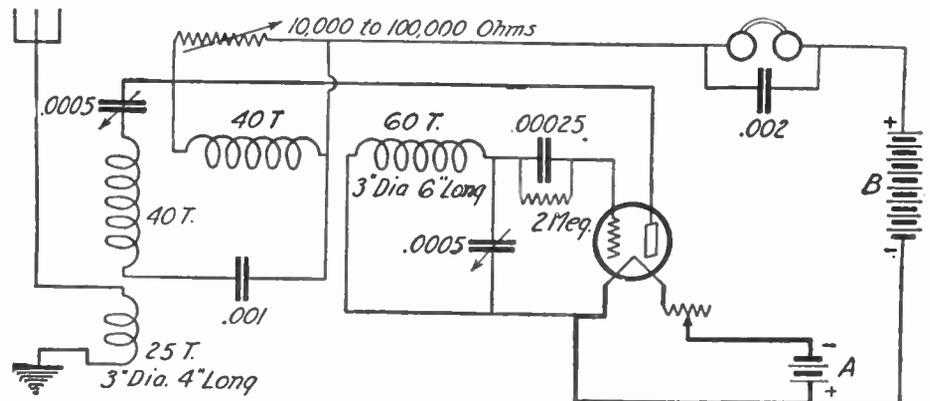
Fig. 228 The increasingly popular Filter Circuit is seen to be that of an exceptionally sharp-tuning, complete receiver. Careful instrument layout, careful construction and good apparatus will be required for best results.
