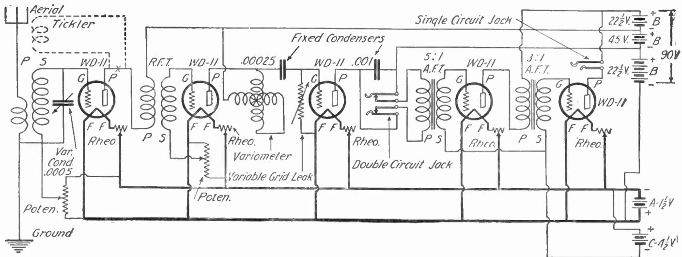
Fig. 15. One of the many variations possible wherein a variocoupler, fixed-tune radio frequency transformer, and continuously variable inductance (variometer) are used. Only two dials are required for this set. The R.F. transformer should not have a sharp peak at one wave-length.
