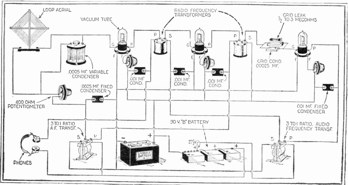
Fig. 290. The inverse duplex receiver has the advantage of not overloading the tubes and rendering them inefficient as is the case in the standard straight type of reflex circuit. The connections for a three-tube set of the inverse duplex type are given above. Two radio- and two audio-frequency transformers are used in connection with the three tubes giving practically the same form as two stages of radio-frequency, detector and two stages of audio-frequency amplification.
