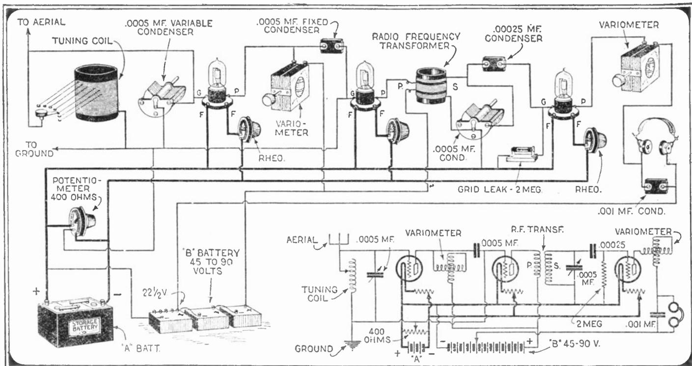
Fig. 41. A circuit diagram of two stages of tuned radio frequency amplification with a vacuum tube detector. The correct constants are given on the diagram. This circuit is quite selective and is an excellent one for the "DX hound" who does not care for ear-splitting volume.
