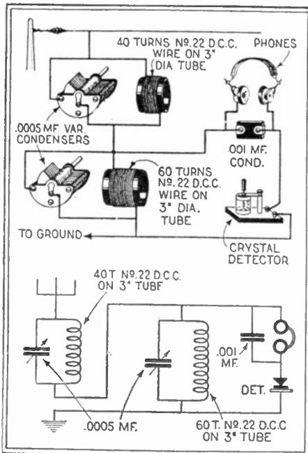
Fig. 101. The above circuit diagram is given for the benefit of the thousands of crystal detector owners who are always looking for a more selective circuit.
