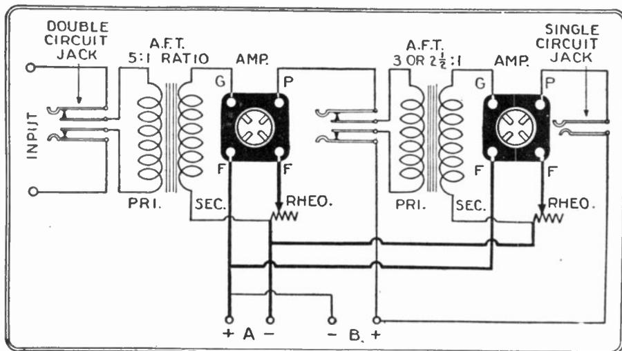
Fig. 214. The circuit diagram of a conventional two-stage audio amplifier, with jack connections after each stage. This amplifier may be added to a one-tube receiver, or any other type in which audio-frequency amplification is desired after a detector tube.
