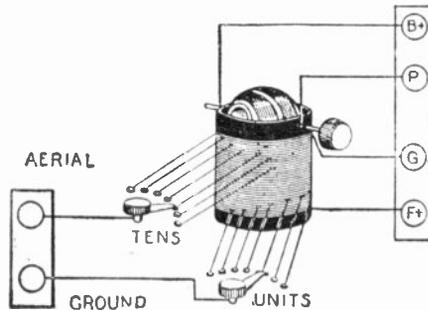
Fig. 19B. The "2-coil variocoupler with tapped primary" unit. This is submitted for those who wish to construct the simple 2-coil variocoupler regenerative circuit.
