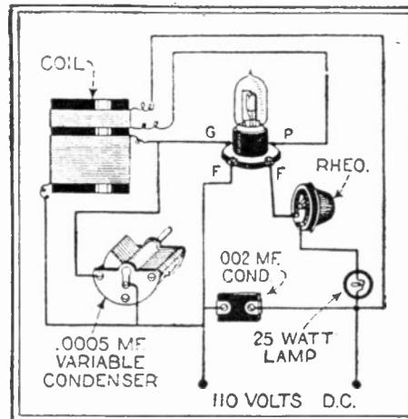
Fig. 151. The diagram above shows the hook-up of an oscillator and wavemeter which operates from the 110-volt lighting circuit.
