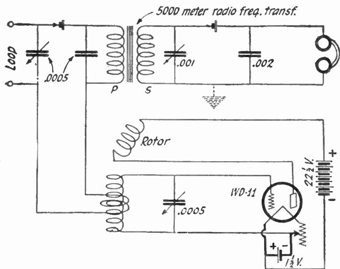
Fig. 5A. Diagram showing method of reducing the number of tubes in super-heterodyne construction. Two detectors of the usual crystal type are required.
