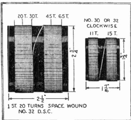
Fig. 244F. The design of an oscillator and an oscillator coil in conjunction with a .0005-mf. condenser, in a super-heterodyne receiver employing 50 to 60 KC type intermediate-frequency transformer.
