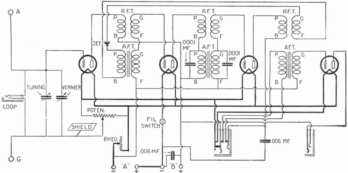
Fig. 22. The DeForest D-10 reflex circuit, employing 3 radio-frequency stages of amplification, crystal detector rectification, two stages of reflexed audio-frequency amplification and one straight stage of audio amplification. This is an excellent combination for portable types of receivers; and will be found to be exceedingly satisfactory and efficient when used in conjunction with a loop.
