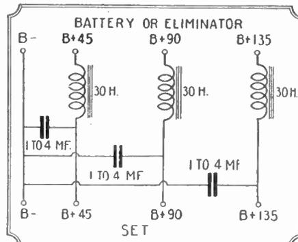
Fig. 189. The circuit above shows the connections for a filter system which may be connected to the output of any type of B eliminator. This filter will serve to iron out line noises and fluctuations in voltage which might otherwise cause considerable trouble. Aged B-batteries will be helped by the use of such a filter.
