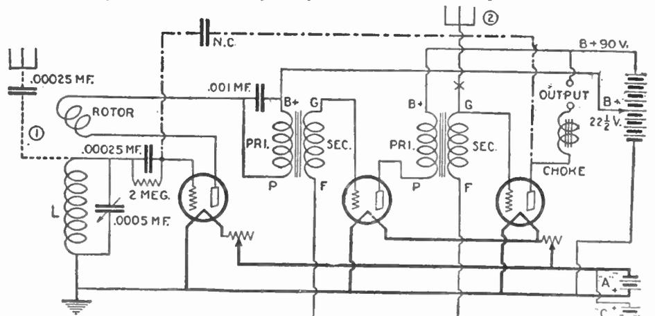
Fig. 154B. A single circuit receiver designed so as to reduce radiation to a minimum.
