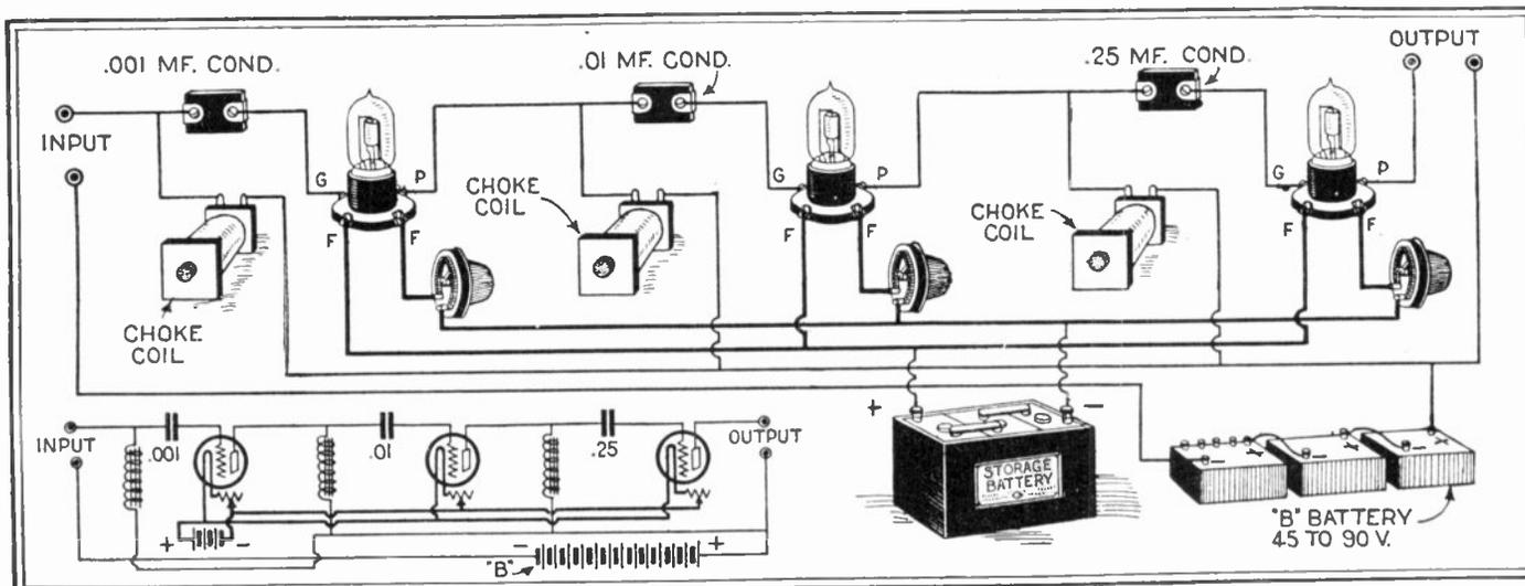
Fig. 216 The choke coils in the above circuit may consist of approximately 10,000 turns of No. 36 enameled wire, wound on a 1/2-inch iron wire core 3 inches long. Suitable end plates should be provided. If desired, the secondaries of small spark coils may be used as the chokes.
