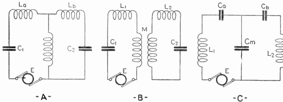
Fig. 61. The three types of coupling used in transferring energy from one circuit to another are shown above. A indicates the type known as direct coupling, where the circuits are connected together by conductors. B illustrates inductive coupling, while C represents capacitive coupling.
