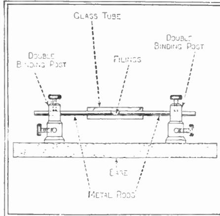
Fig. 296. The details for the construction of a coherer are given above. This type of detector is obsolete at the present date, but sometimes is used in connection with experimental radio control apparatus.
