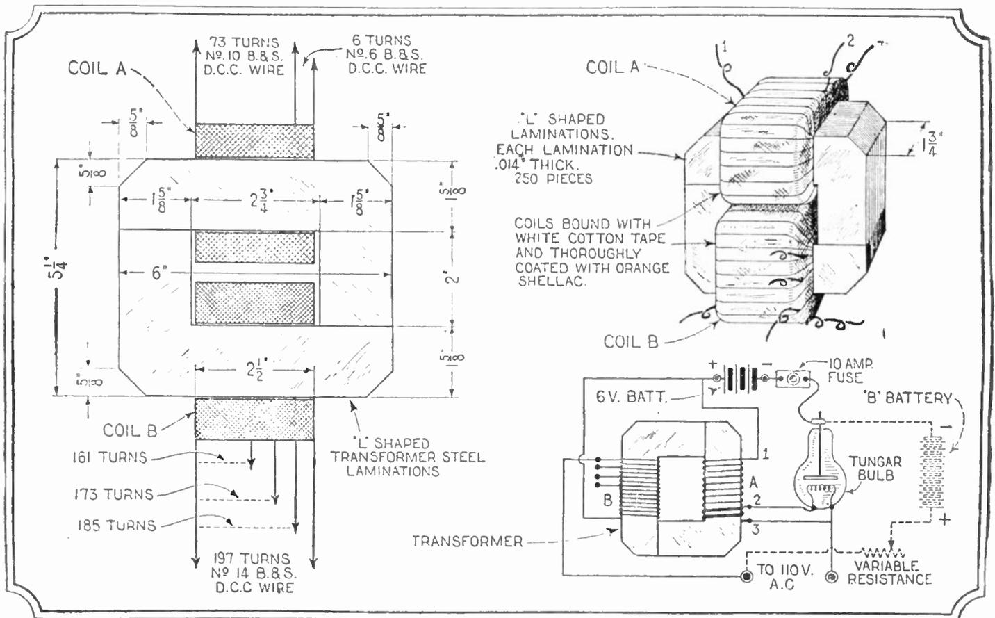
Fig. 167. A transformer for the purpose of charging both the "A" and "B" batteries is detailed clearly above. It is well worth the trouble to construct. It is designed for operation on 110 volt, 60 cycle alternating current, and if carefully built will last indefinitely.
