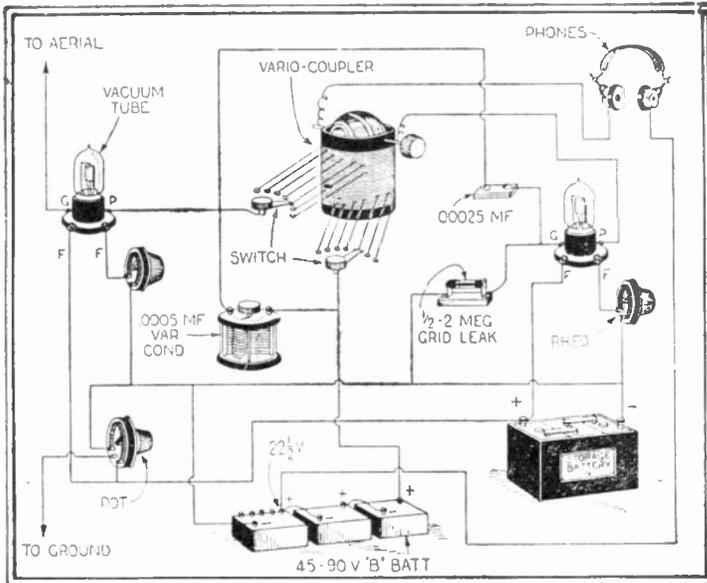
Fig. 280. In some cases it is possible to use radio-frequency amplification without any tuning arrangement between the R.F. amplifier tube and the antenna. Such a circuit diagram is shown above. At times it will be necessary, however, to place a one-slide tuning coil in series with the antenna.
