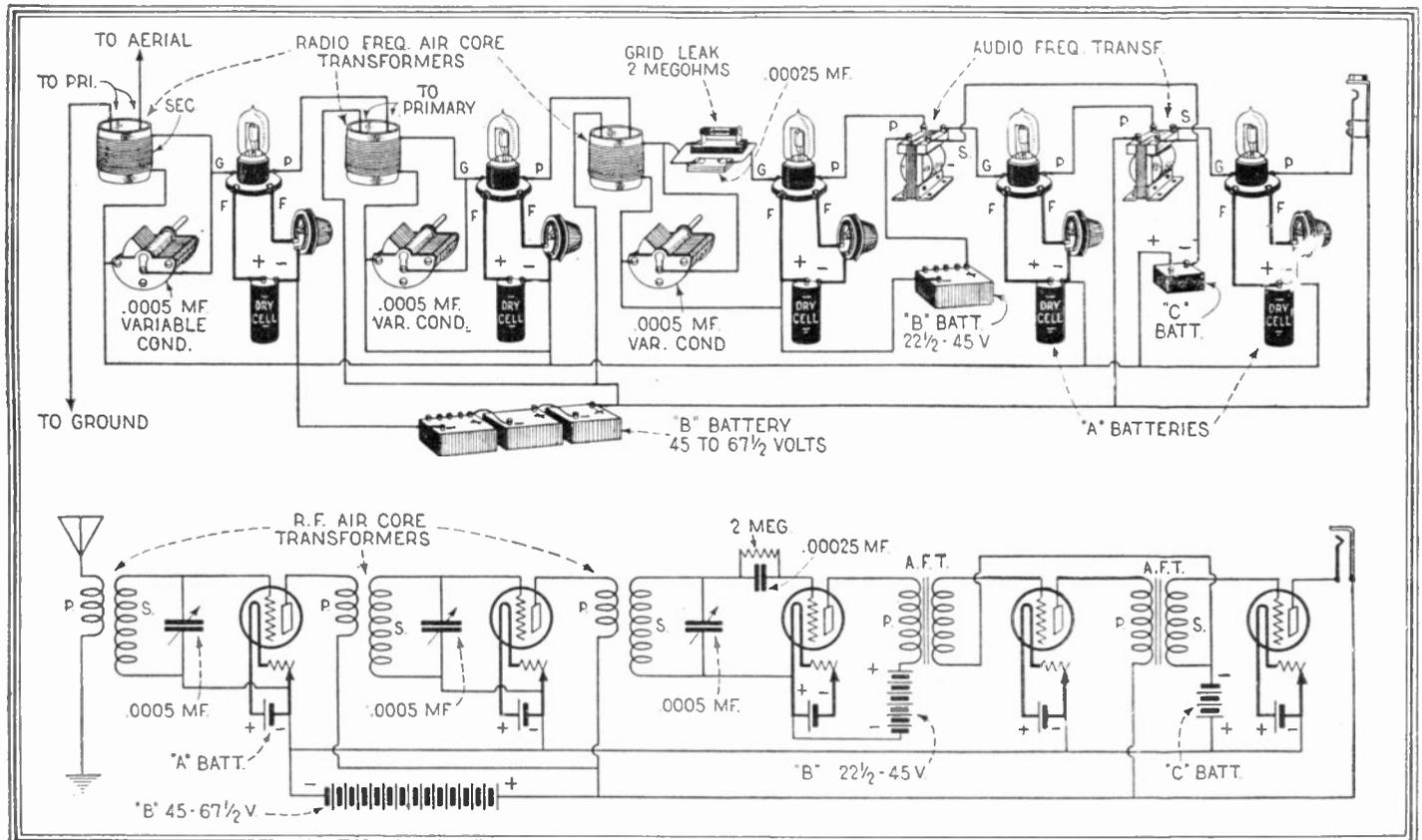
Fig. 172. When using dry cell tubes, one "A" cell can very readily be used for each tube. Use either separate rheostats or fixed resistances in the amplifier filament circuits. Many experimenters report excellent results with the system as shown with all filaments and batteries in parallel.
