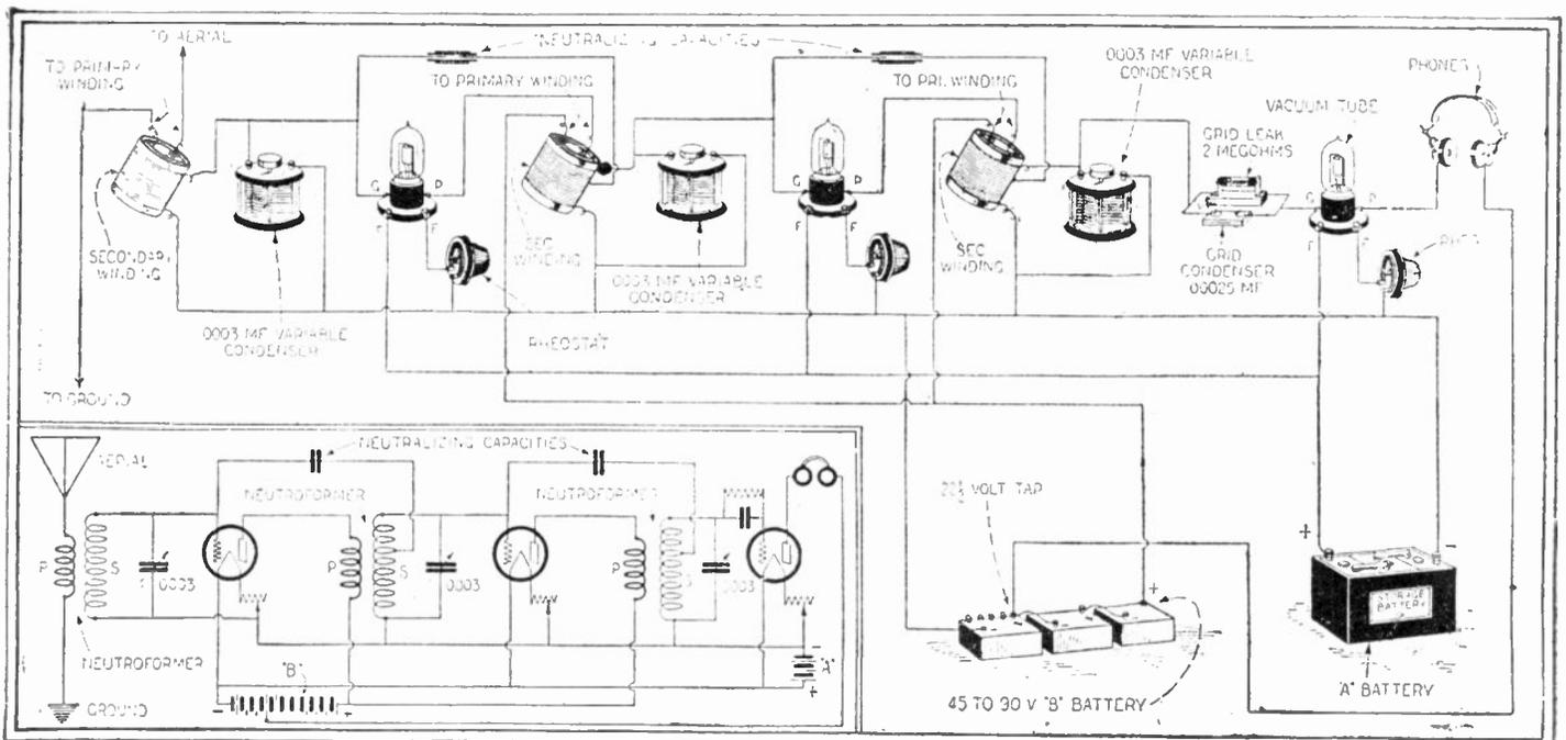
Fig. 304. The circuit diagrams above show all the necessary connections for a three-tube Neutrodyne receiver using Neutroformers with tapped secondaries. The antenna circuit is aperiodic while the secondary circuit and the secondaries of the second and third Neutroformers are tuned. The two diagrams above both show the same set.
