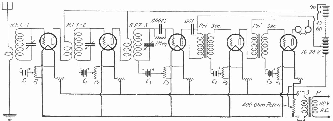
Fig. 153. This circuit uses the house lighting current for filament heating. A transformer steps the current down to six volts A.C. To prevent a tube burn-out by overloading, all tubes should be lighted when set is in use.
