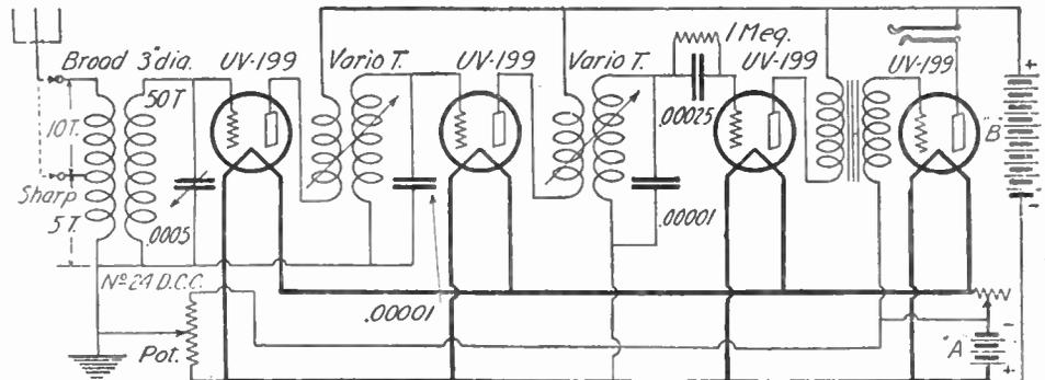
Fig. 12. Voltage step-up through the use of two-coil transformers, and tuned grid circuits without condensers, are outstanding features of this receiver. Loud speaker reproduction of local signals, and loud headphone reproduction of very distant stations, using only dry cell tubes, is had.
