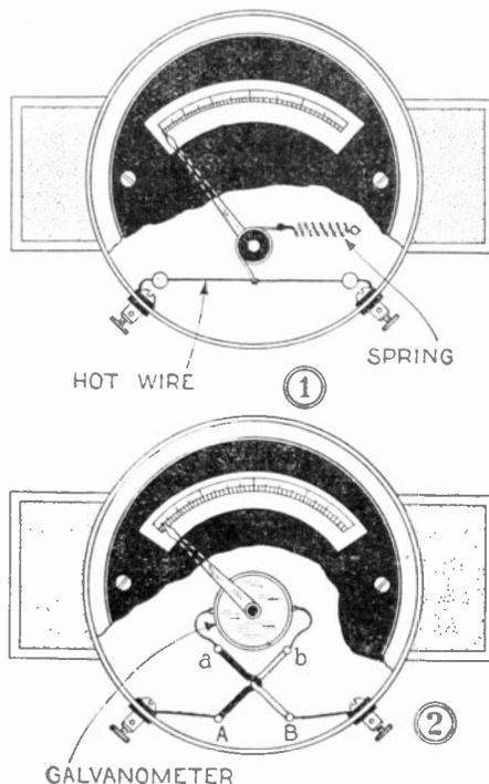
Fig. 265. A hot wire and a thermo-coupler ammeter are shown above in Figs. 1 and 2 respectively.
