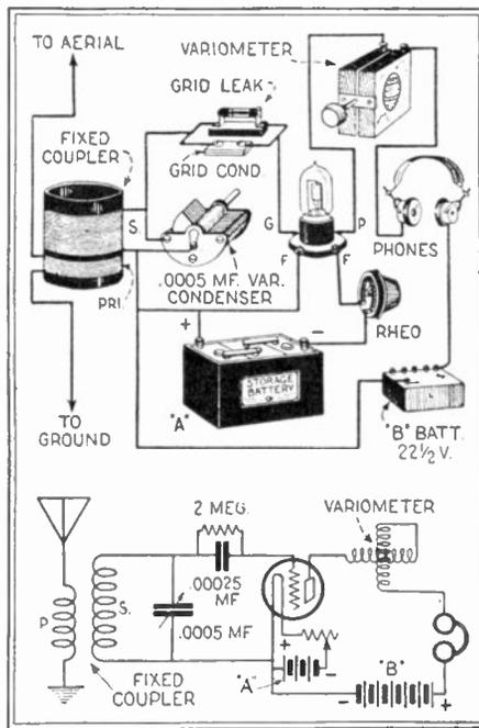
Fig. 114. A very simple yet selective and stable single tube regenerative circuit is shown above. This set is easy to hook up as well as to operate.
