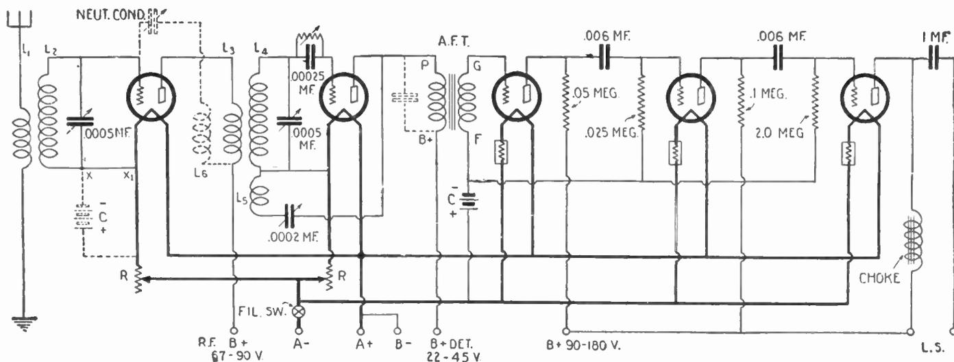
Fig. 89. A composite 5-tube set, whose peculiar features are a combination to make up a set that will be noted for its performance. It consists of a neutralized tuned RF stage, a modified Hartley type of detector, one stage of transformer-coupled audio-frequency amplification, and two stages of resistance-coupled audio-frequency amplification.
