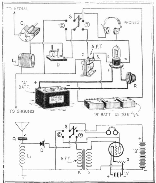
Fig. 59B. With this system, the crystal detector may be used alone, or by means of switch S it may be used with an amplifier.
