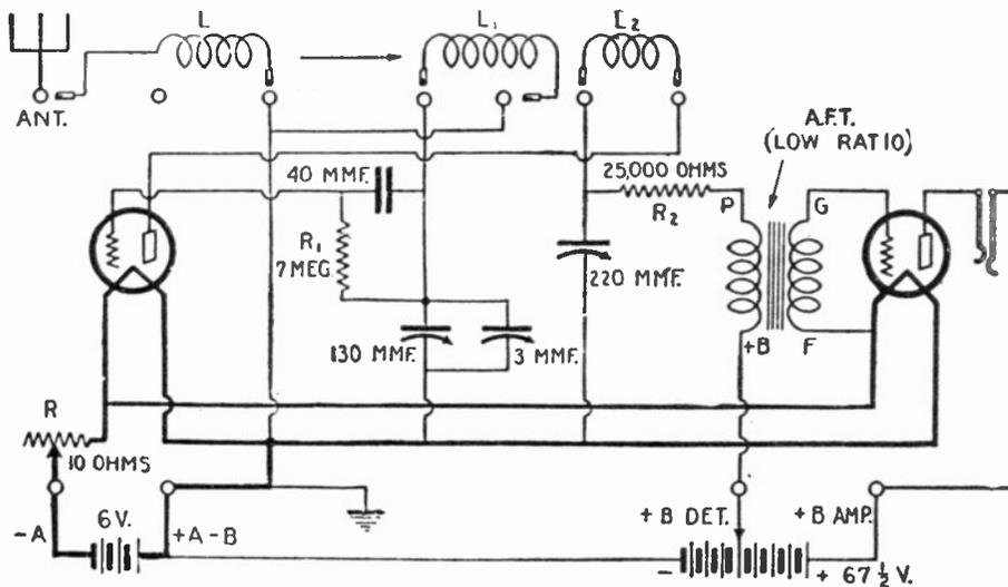
Fig. 86. The Grebe Short-Wave receiver (CR-18), employs plug-in coil inductances, by which a variable wave-length range of from approximately 8:52 to 216 meters may be covered. Constructional data for the receiver are given.
