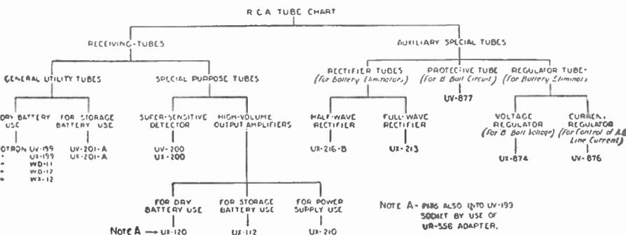
Fig. 199. This chart may be used to determine the best tube for receivers, both plain and those employing various methods of amplification, or using dry cells in place of storage batteries.
