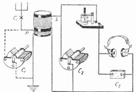
Fig. 16C. A very simple crystal set. The inductance coil shown may be a standard two-coil variocoupler either tapped or untapped.
