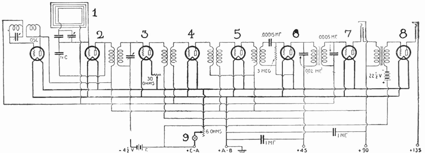
Fig. 87. The circuit diagram of the Radiola 28 receiver (superheterodyne type). Superheterodyne parts designed to operate with an intermediate-frequency amplifier of the 5,000-meter type (60 kc.) may be employed satisfactorily with this particular circuit.
