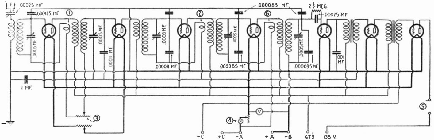
Fig. 90. The schematic wiring diagram of the Kellogg R.F.L. receiver. This set combines many desirable features which are very popular with the broadcast listener; the most important of which are four stages of tuned-radio-frequency amplification before a detector, and two stages of audio-frequency amplification. A power tube is used in the last audio stage, using the voltage shown.
