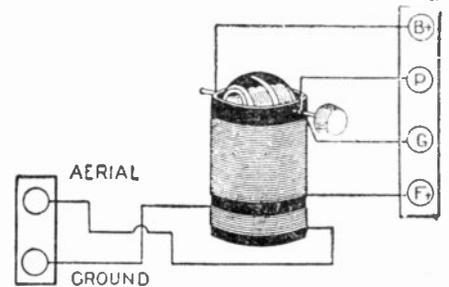
Fig. 19D. The "untuned primary" type of set. This is the standard regenerative circuit of today for broadcast reception.
