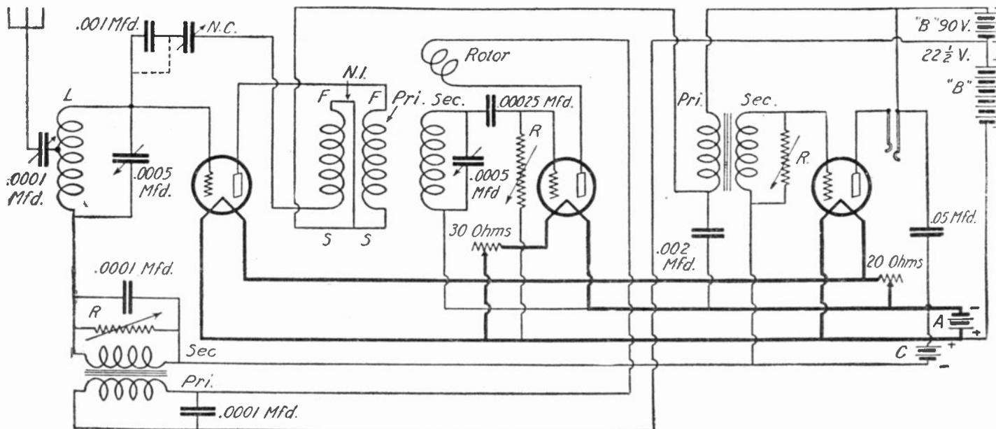
Fig. 75. Roberts' non-oscillating reflex. One of the latest reflex circuits. Careful construction will result in an excellent receiver. It is advisable to experiment somewhat with this circuit as slight changes, particularly in coil relations, affect the reproduction quality.
