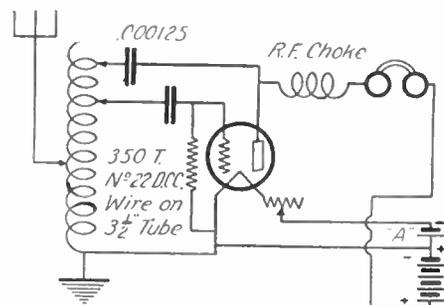
Fig. 74A. Weagant circuit applied to a three-slide tuner. When oscillating a loud click is heard as the sliders are moved.
