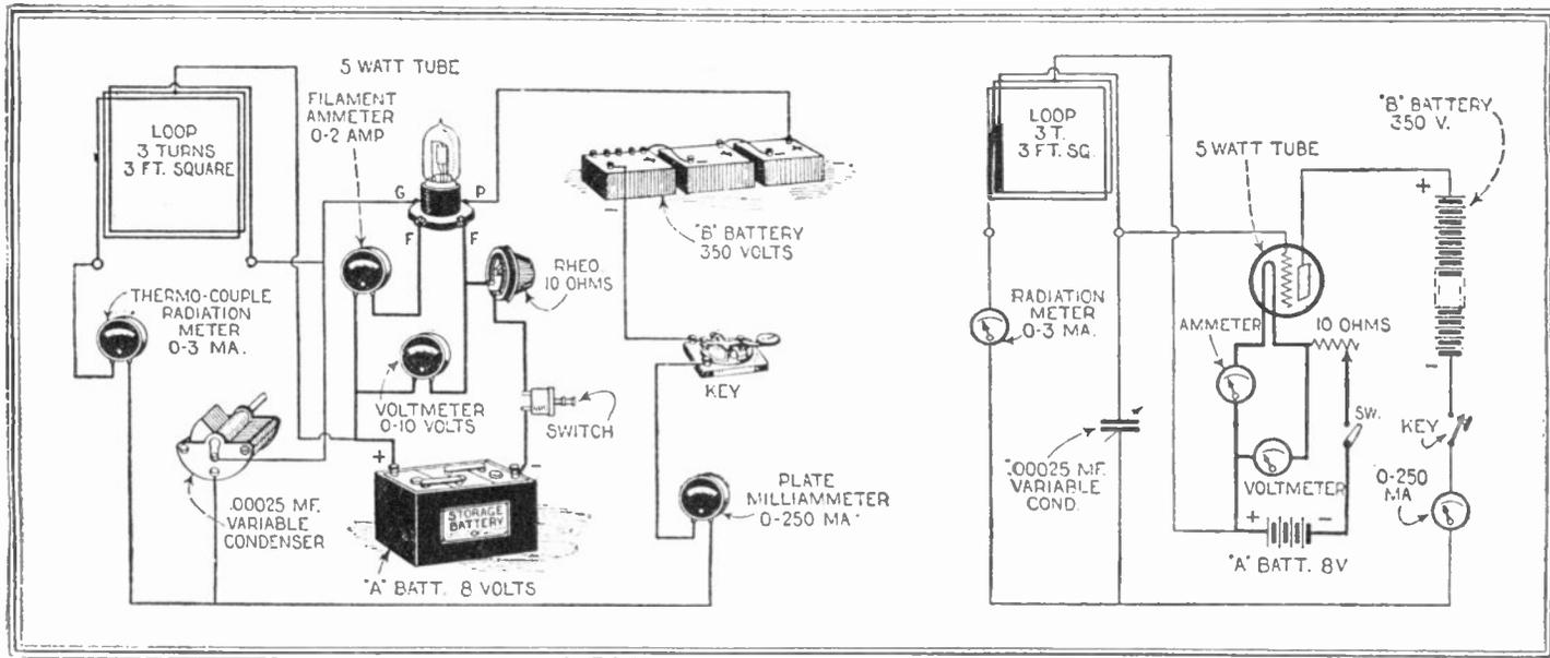
Fig. 140. A simple loop "C.W." transmitter. When properly built this set will give excellent service. Its low first cost and up-keep should make it very popular with the beginner. It can readily be equipped for phone transmission.
