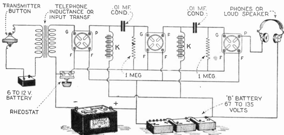
Fig. 225. The amplifier shown here is designed to build up the sound picked up by a microphone so that it will operate a loud speaker. Impedance coupling is used to reduce distortion, and the amplification obtained is about equivalent to two stages of transformer-coupled amplification.
