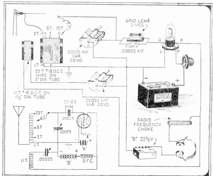
Fig. 37. Short waves are rapidly coming into use for broadcasting purposes, on account of the greater carrying powers and less fading experienced on these waves. The circuit shown is the latest Reinartz type.
