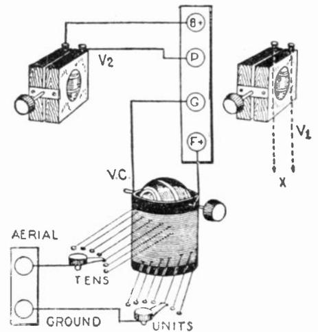
Fig. 19A. The "2-variometer, variocoupler" regenerative arrangement. This was once the standard of reception circuits, but a demand for simplicity of control forced the "untuned primary" receiver into the lead.
