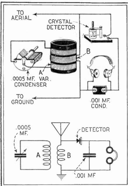
Fig. 110. A simple crystal detector circuit using the absorption method of tuning is shown above.
