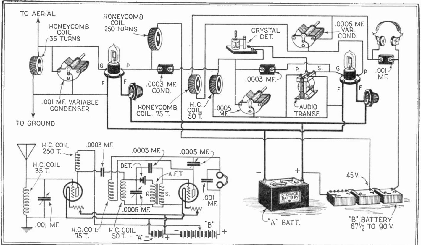
Fig. 102. Many experimenters seem to always be desirous of trying out something new in reflex circuits. Here is one that will keep you busy for some time. It is of English origin and using honeycomb coils throughout, will give good results when properly operated.
