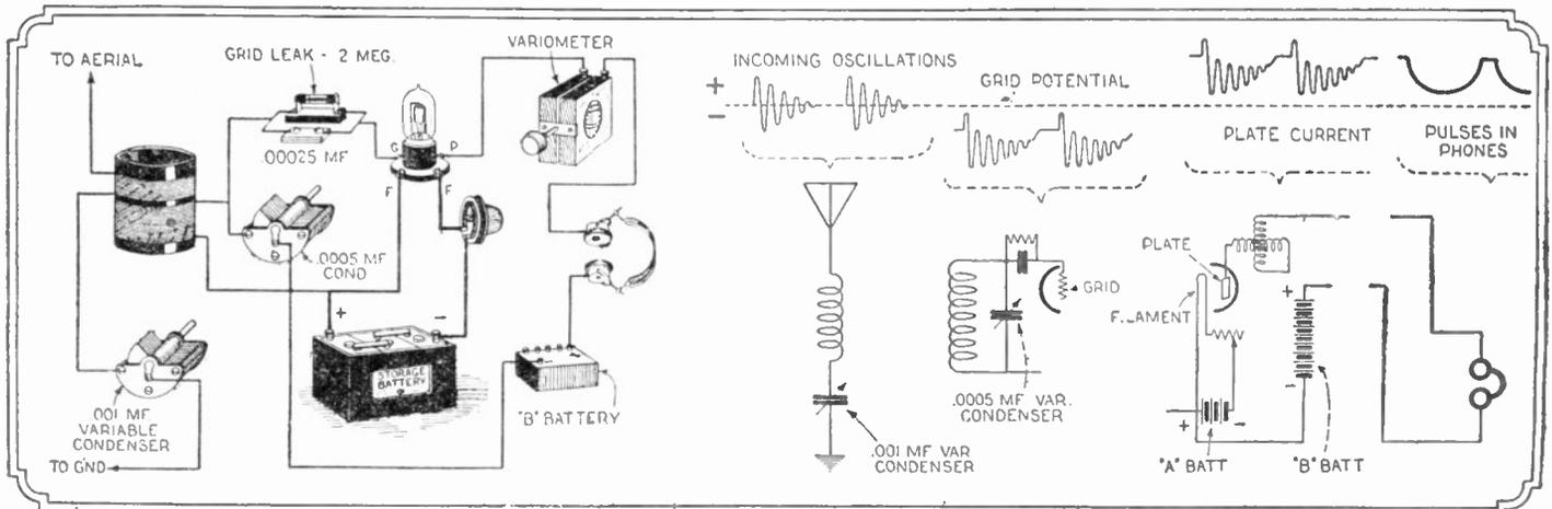
Fig. 3. Just what happens in the different parts of a simple regenerative circuit is depicted here. Memorize the diagrams. They will help you in solving and understanding more complicated hook-ups.
