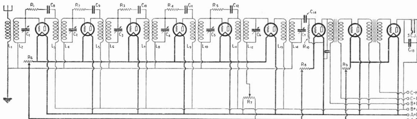
Fig. 26. Wiring diagram of the Super-Pliodyne 9-tube receiver, which employs six stages of tuned radio-frequency amplification, and incorporates a novel means of suppressing oscillations. The amount of radio-frequency amplification obtained is tremendous, resulting in a very sensitive and selective receiver.
