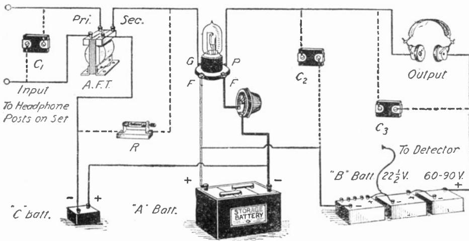
Fig. 16. Picture diagram of a standard audio frequency amplifier, showing tone quality controls in dotted lines. Connect "B" minus to "A" minus if the balance of set is so connected. A separate current supply may be used for this unit.
