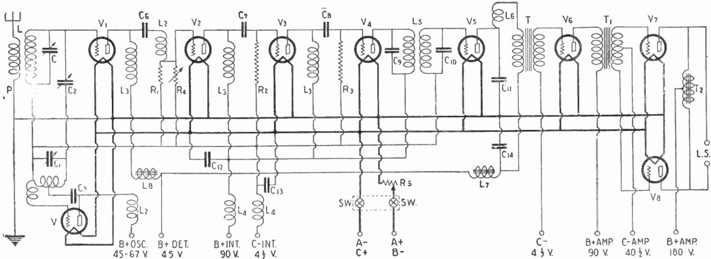
Fig. 65. Circuit of an improved superheterodyne which employs impedance-coupled intermediate-frequency amplifiers and a push-pull audio amplifier.
