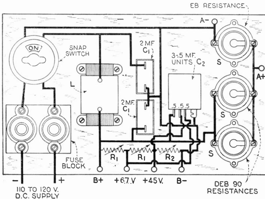
Fig. 159. An "A" and "B" battery eliminator, operating from a Direct Current source only. The "B" battery voltage output is approximately 100 volts at maximum. By varying the amount of D E B resistances employed, any number of tubes up to 10 (201-A type) will be supplied with filament current (see the table, "Figuring the Resistances.")
