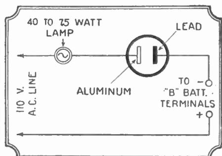
Fig. 160B. The parts and connections necessary for a "B" battery charger, operating from an A.C. source are shown. With this device, it is possible to charge only one 45-volt block at a time.
