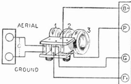
Fig. 19C. The "3-coil honeycomb" regenerative unit. The standard way of receiving long-wave stations.
