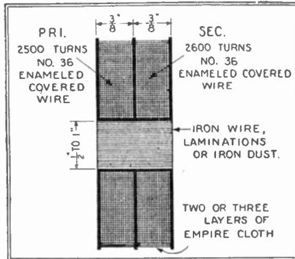
Fig. 240C. Design of an intermediate transformer which operates with maximum efficiency at 50 to 60 K.C. The correct amount of iron core must be determined experimentally.
