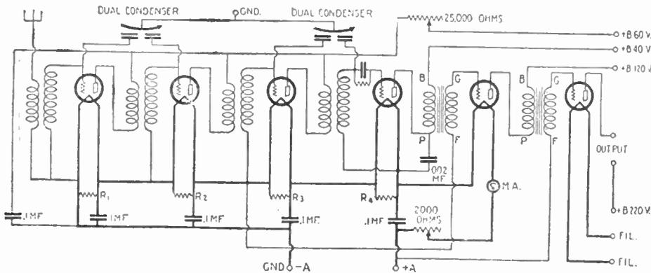
Fig. 161A. Hook-up of the Varion, which is designed for use with an "A, B & C" battery eliminator, such as that shown in Fig. 2205-B. The filaments of all tubes are wired in series to keep down their current consumption. Ballast resistances are placed across each tube. Only 199-type tubes may be employed in the first five stages of the receiver.
