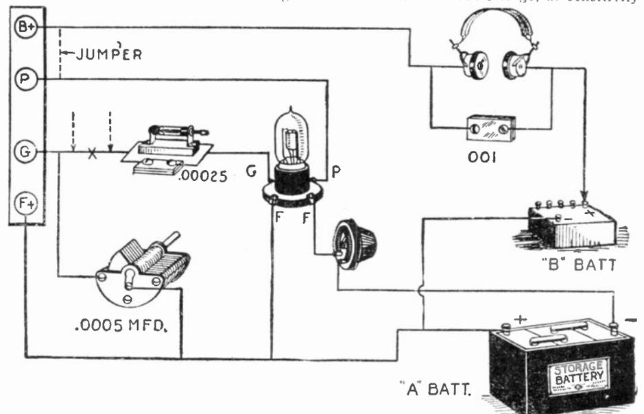
Fig. 19. This picture diagram of a tube unit and the diagram of one of the coil units shown above, should enable anyone to construct a very efficient 1-tube receiver. The completed set may be later enlarged to include audio frequency amplification if the owner desires to operate a loud speaker.
