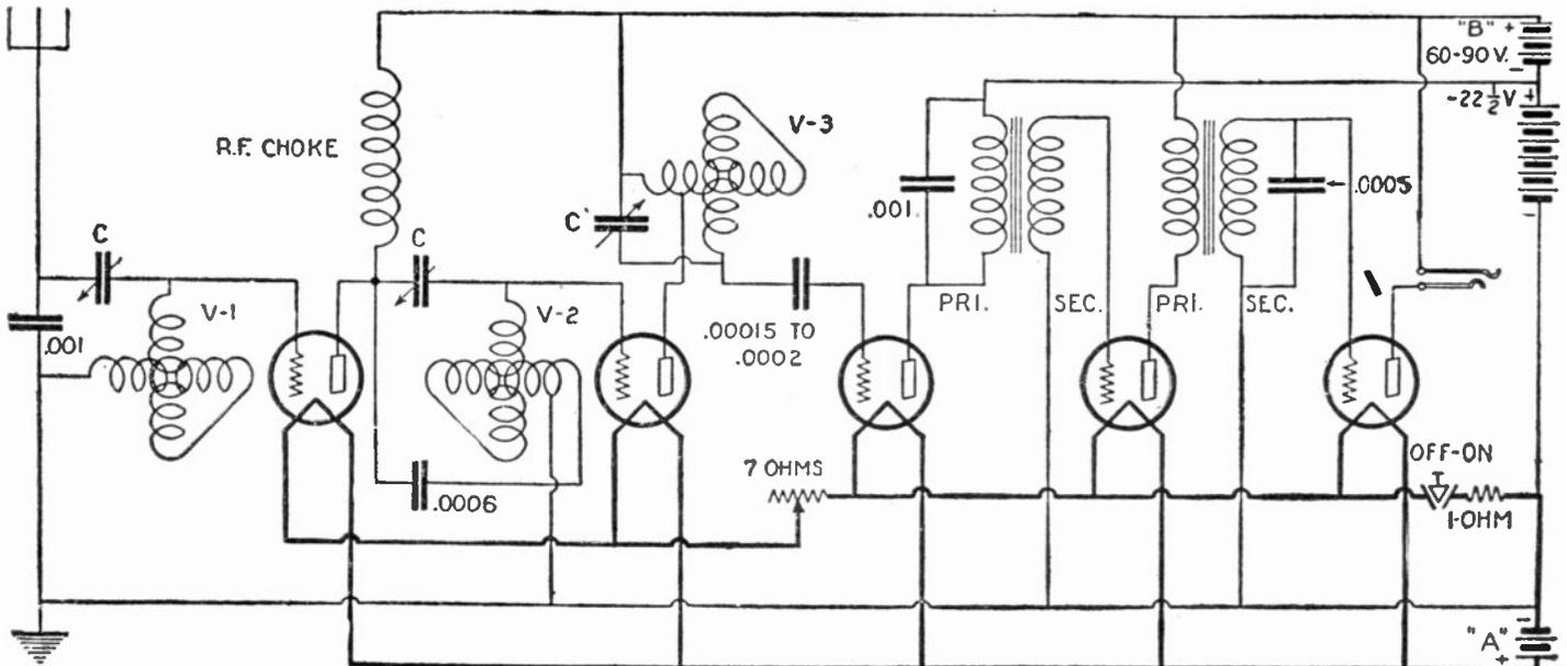
Fig. 77. The Magnavox One-Dial Receiver has aroused considerable interest by reason of the excellent results that have been secured by its owners. Tiny white knobs control the "ratio condensers" used to balance the circuits to the particular tubes and local conditions encountered.
