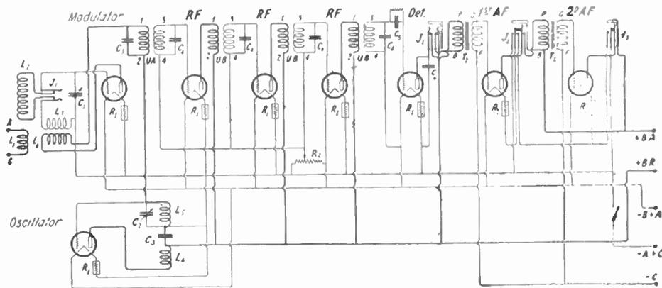
Fig. 84. Wiring diagram of the Ultradyne L-2. L1 has 7 turns, L2 36 turns, L3 20 turns, L5 36 turns, L6 22 turns.
