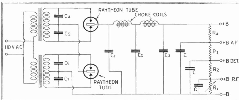
Fig. 191. The connections for a B-power supply unit, employing two Raytheon tubes, and two transformers having an output of about 435 volts D.C., are shown above. Using the type B Raytheon tube 20 milliamperes of current will be delivered and with the type BH 35 milliamperes.
