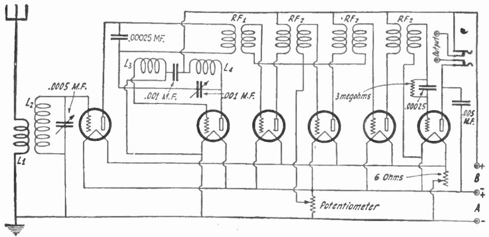
Fig. 81. This is the complete circuit diagram of the Ultradyne L-1 receiver, which incorporates the "modulation system." As explained in the text, one or two stages of audio frequency amplification should be added so that loud speaker results can be obtained on distant stations.
