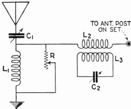
Fig. 247. A very efficient wave trap which can be constructed at a very low cost. It will be found of great benefit by those located in the vicinity of a broadcast transmitter.
