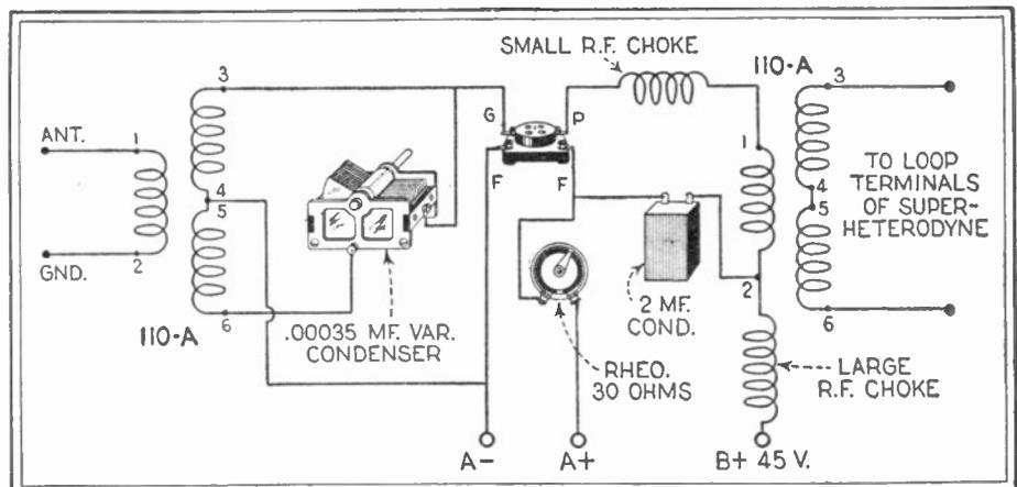
Fig. 126 The method of coupling the antenna and ground to a Radiola superheterodyne receiver is clearly shown above. This system will give excellent results and selective tuning.
