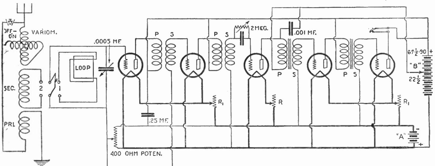
Fig. 20. A 2-dial radio frequency set. Either a loop aerial or a regular aerial and ground may be used. For good operation over the entire broadcast wave-length range it will be necessary to use a good make of radio frequency transformer. Dry cell tubes may be used.
