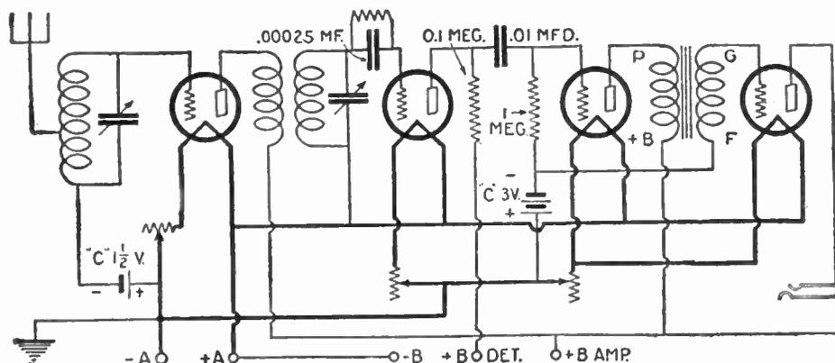
Fig. 79. The Sleeper RX-1 Receiving Circuit. Inexpensive and simple to build, one wonders at the results obtained in regard to both sensitivity and quality, for the time and money spent. The stage of resistance-coupled amplification before the ordinary transformer-coupled stage, accounts for the set's unusual quality of reproduction.
