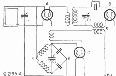
Fig. 66A. Schematic wiring diagram showing the floating-beat-note system used in some super-heterodynes.
