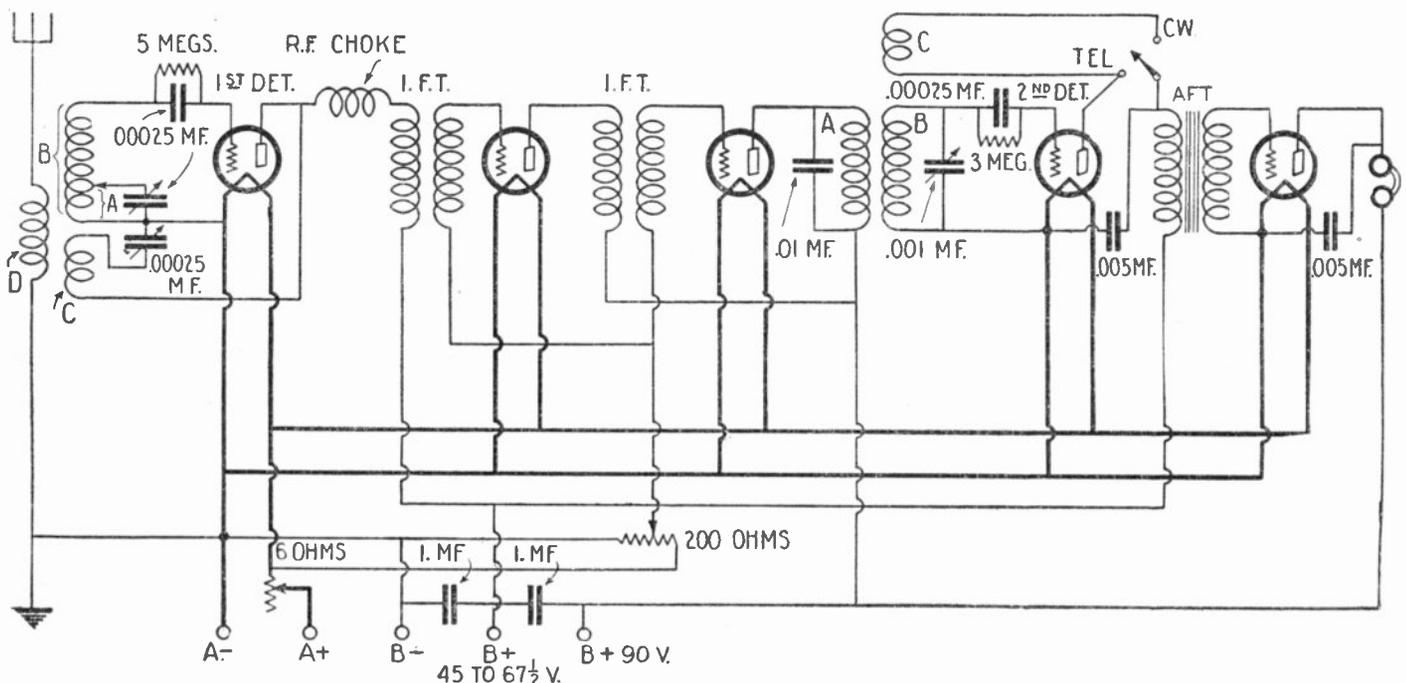
Fig. 28A. The schematic wiring diagram of the Short Wave Superheterodyne receiver. The following features are incorporated in the set: detector and oscillator functions are accomplished by one tube, the "autodyne" principle being employed; a regenerative second detector, with a short circuiting switch so that this feature may be eliminated at will, permits either C.W. or phone reception.
