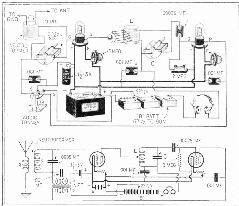
Fig. 50. Here is a novel type of two tube reflex receiver giving the effect of one stage of radio frequency amplification, detector and one stage of audio frequency amplification. Use good instruments in a set of this nature and you will be assured of good results.
