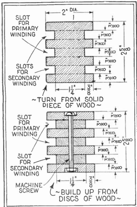
Fig. 217. The experimenter will find much of interest in constructing various sizes of radio-frequency transformers. A form such as the one illustrated will aid materially in this work.
