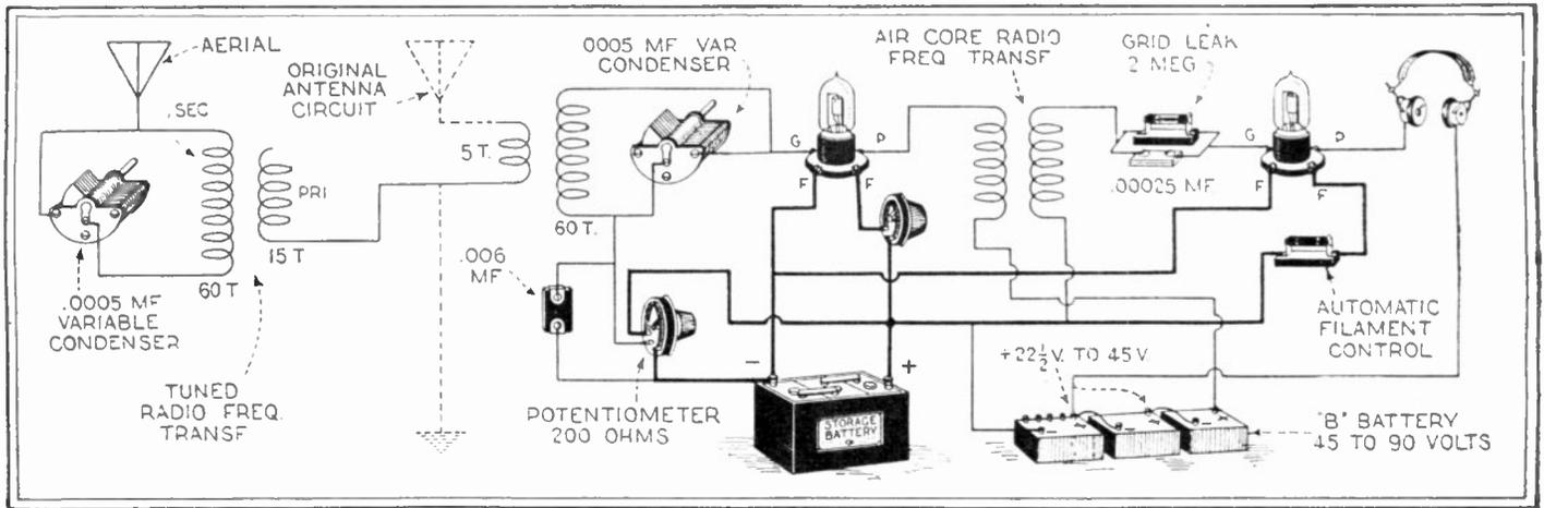
Fig. 122. The circuit above may seem rather strange, but it has been tested and found to be very selective. Both oscillating circuits are tuned sharply to the incoming wave. If a ground connection is desired, it should be made to the filament negative.
