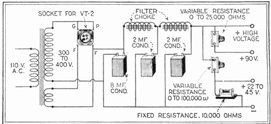
Fig. 190. The above diagram shows a good method for utilizing the VT-2 tube as a rectifier. As the tube is capable of operating at a plate voltage of 400 volts, it will deliver sufficient voltage when used as a rectifier.
