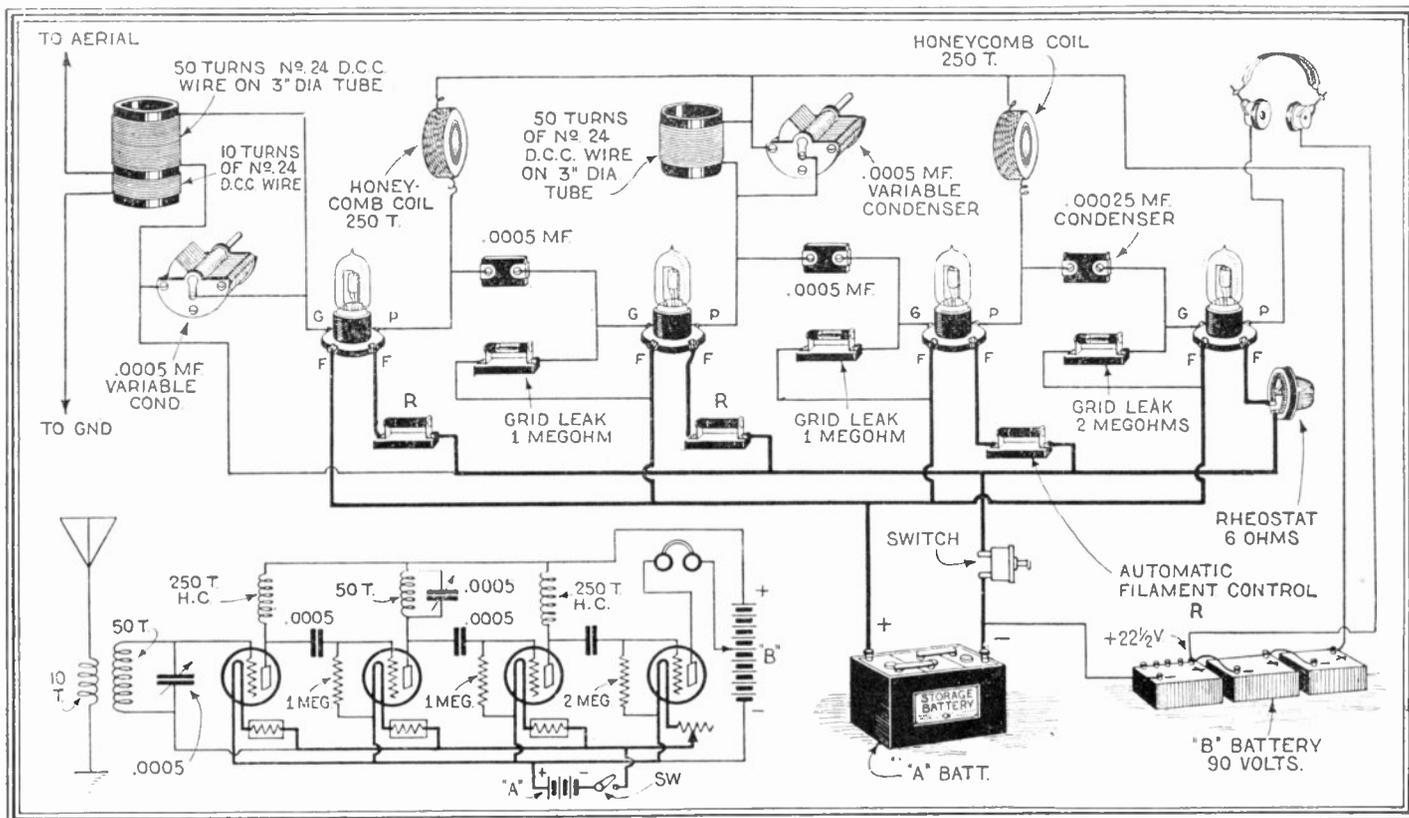
Fig. 38. The above diagram shows what is called the T.A.T. system. It is used very much in England because it does not oscillate. The reason for this is that an aperiodic circuit is placed between two tuned ones. By following the diagram an efficient and unusual set can be constructed.
