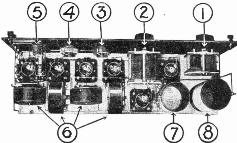
Fig. 81C. Illustration of the Ultradyne L-1 receiver showing panel and parts layout. Note that the intermediate frequency transformers are mounted at right angles at each other to prevent interstage coupling. A slightly larger panel is required, if audio frequency amplification is to be added to the receiver.
