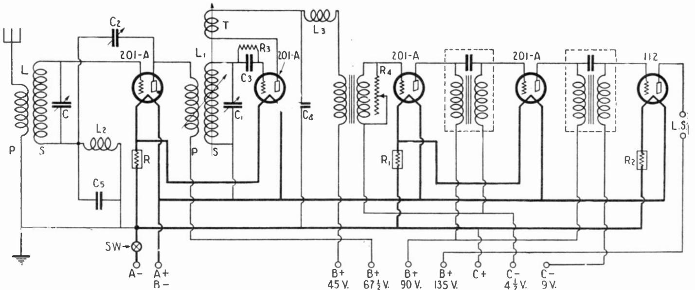
Fig. 93D. The circuit employed followed in the wiring of the Samson Dual T.C. receiver consists of a stage of neutralized R.F. amplification, a regenerative detector, one stage of transformer coupled audio-frequency amplification and two stages of a new, improved type of audio amplifier.
