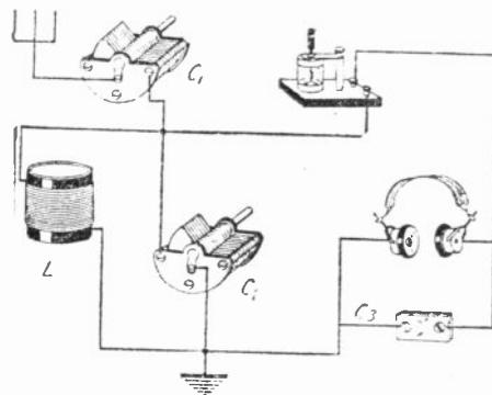
Fig. 16B. A two-dial crystal set. Winding the single coil inductance should present no difficulties to the experimenter. Sharp tuning is not a feature.
