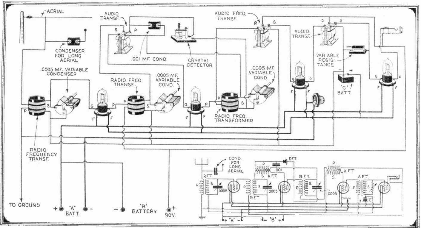
Fig. 100. The well known and justly famous Tu-Ra-Flex circuit is shown in both picture and schematic form above with the addition of a single stage of audio-frequency amplification giving the results of three stages total. The variable resistance shown is of assistance in controlling the circuit.
