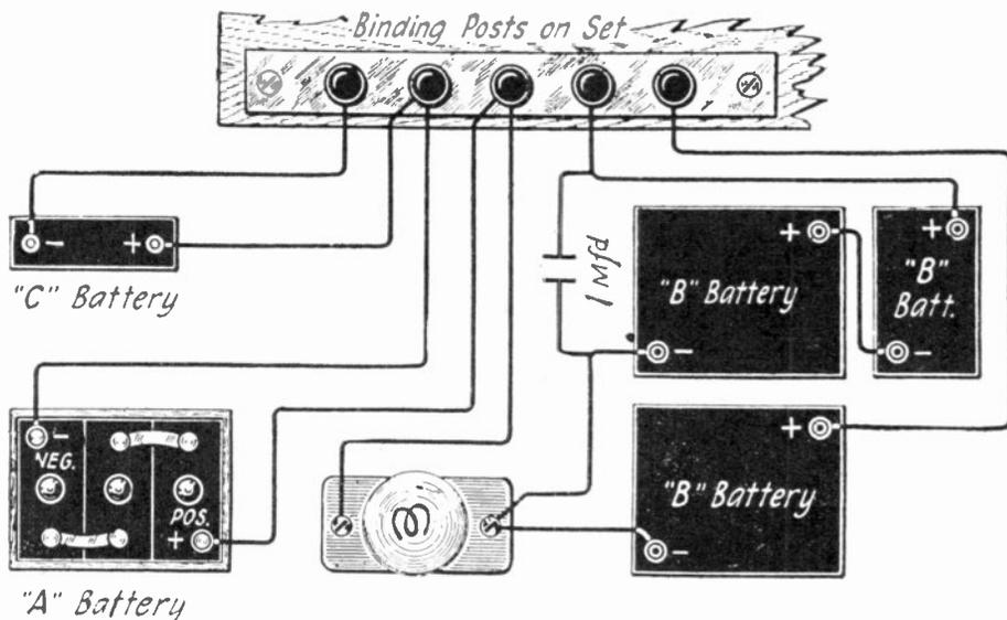
Fig. 84A. Method of connecting batteries to the Ultradyne L-2 receiver. A special test lamp is used to detect a possible short circuit in the receiver, and prevent burning out tubes.
