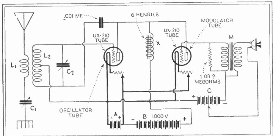
Fig. 152. Compact low power transmitters seem to interest a large number of our readers, so we are publishing another diagram suitable for this type of work above. Note that a B battery voltage of 1000 is used. This is the maximum for the 210 type tube, but less may be used if desired.
