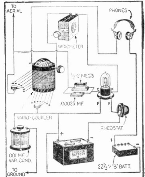
Fig. 282. If a variometer is placed in series with the plate of a vacuum tube in a standard single circuit tuner, much greater selectivity will result as a combination of the feed-back and tuned plate system.
