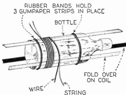
Fig. 246. The novel method employed in winding the low-loss coil is shown above.
