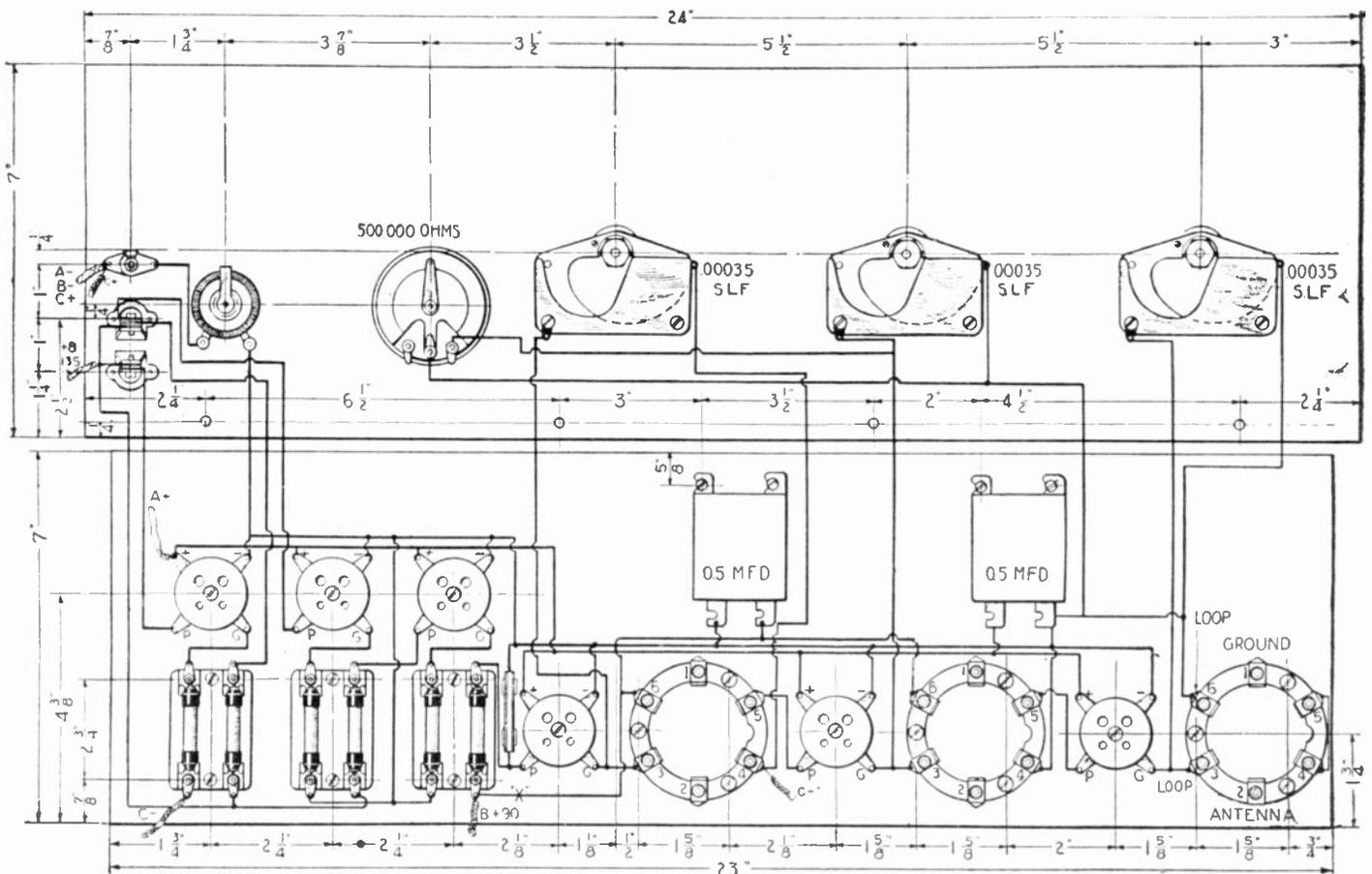
Fig. 35. Wiring diagram of the Silver Six receiver; two stages of tuned R.F., detector and three stages of resistance-coupled audio. A special means of controlling oscillations in the R.F. stages is provided. Plug-in inductance coils are used, so that a wave-length range from approximately 50 to 500 meters may be covered.
