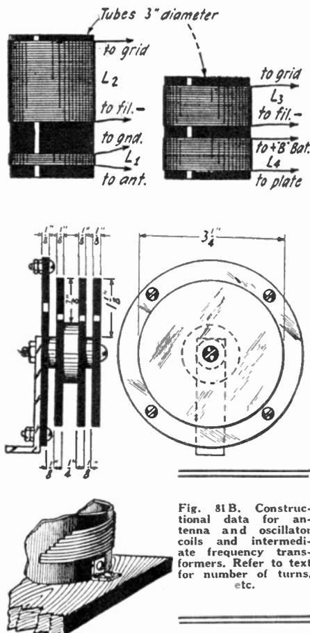
Fig. 81B. Constructional data for antenna and oscillator coils and intermediate frequency transformers. Refer to text for number of turns, etc.
