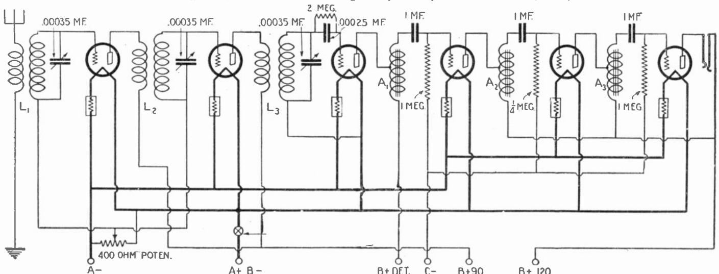
Fig. 23. A standard six-tube receiver designed especially to amplify musical notes without distortion. What are known as "autoformers" are used in place of the conventional audio transformers to couple the audio stages.
