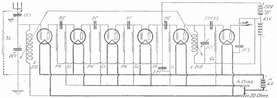
Fig. 72. This efficient receiver is not difficult to tune. It is easy to construct. This is an "all-wave" receiver. One need only change coils, to cover practically all wave-lengths in use today.
