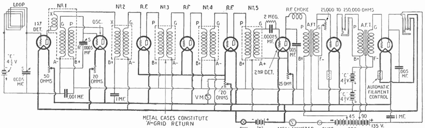
Fig. 91. The Madison Moore Super-heterodyne circuit, one of the most recent along super-heterodyne lines. Special intermediate-frequency transformers are designed for the 199 and 201-A type of tubes, which make possible perfect matching between tubes and transformers, and result in the utmost quality possible to obtain when using either type of tube.
