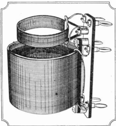
Fig. 94B. The appearance when completed of the coil L<sub>1</sub>, which is used in the Henry-Lyford receiver. L<sub>2</sub> is very similar in construction, except that the third or semi-variable winding at right is omitted.
