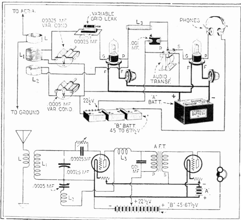
Fig. 107. A short-wave receiver opens new fields for the radio enthusiast. An excellent type for use with headphones is shown above. The data for coils covering the 40 and 80 meter amateur band is given in the text. Follow it carefully in order to obtain the best of results.
