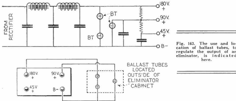
Fig. 163. The use and location of ballast tubes, to regulate the output of an eliminator, is indicated here.
