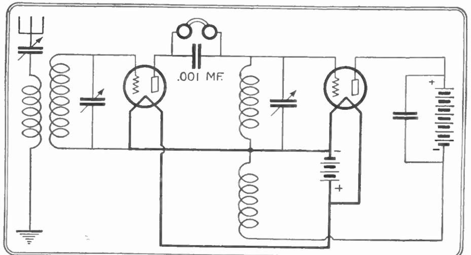
Fig. 81A. The fundamental principle of the Ultradyne receiver, showing the first detector and oscillator circuit employing the efficient modulation system. This method is a radical departure from the conventional, and results in a receiver of remarkable efficiency.
