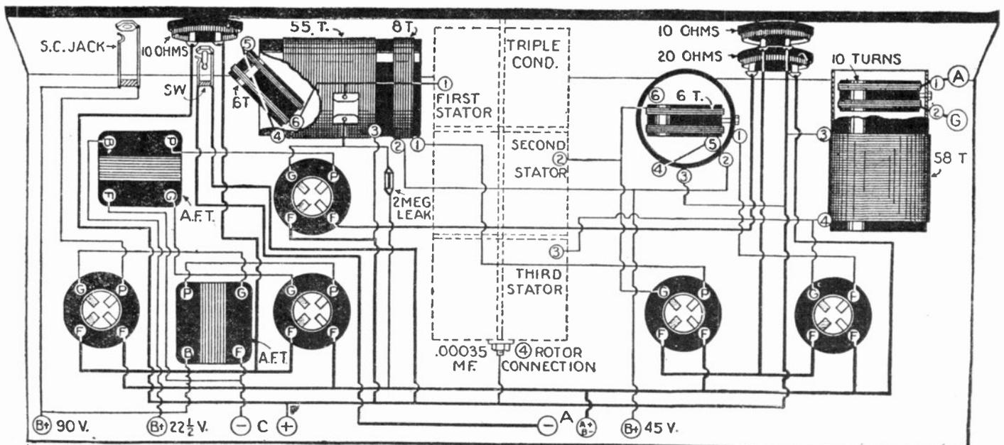
Fig. 82A. The Journal One-Knob, five-tube, receiver consisting of two stages of radio frequency amplification and regenerative detector, resulting in an extremely efficient and selective receiver, although only one dial is employed for tuning. Any type of tubes may be employed in this receiver, although for best results it is advisable that storage-battery type, 201-A or 301-A tubes be used throughout.
