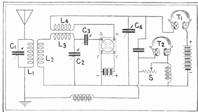
Fig. 62B. This hook-up is designed to be used in measuring the amount of energy received from transmitting stations at distances as great as 4,000 miles. The station is tuned in by using phones T1, while T2 is used for measurements.
