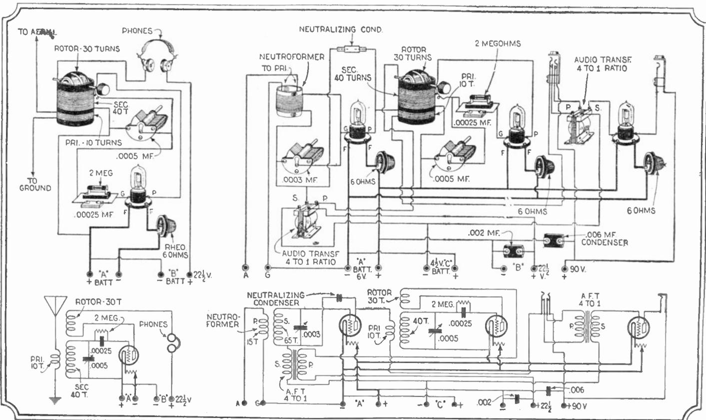
Fig. 98. The beginner's set is rapidly being improved by the addition of more tubes. If you want good results you should try this circuit.
