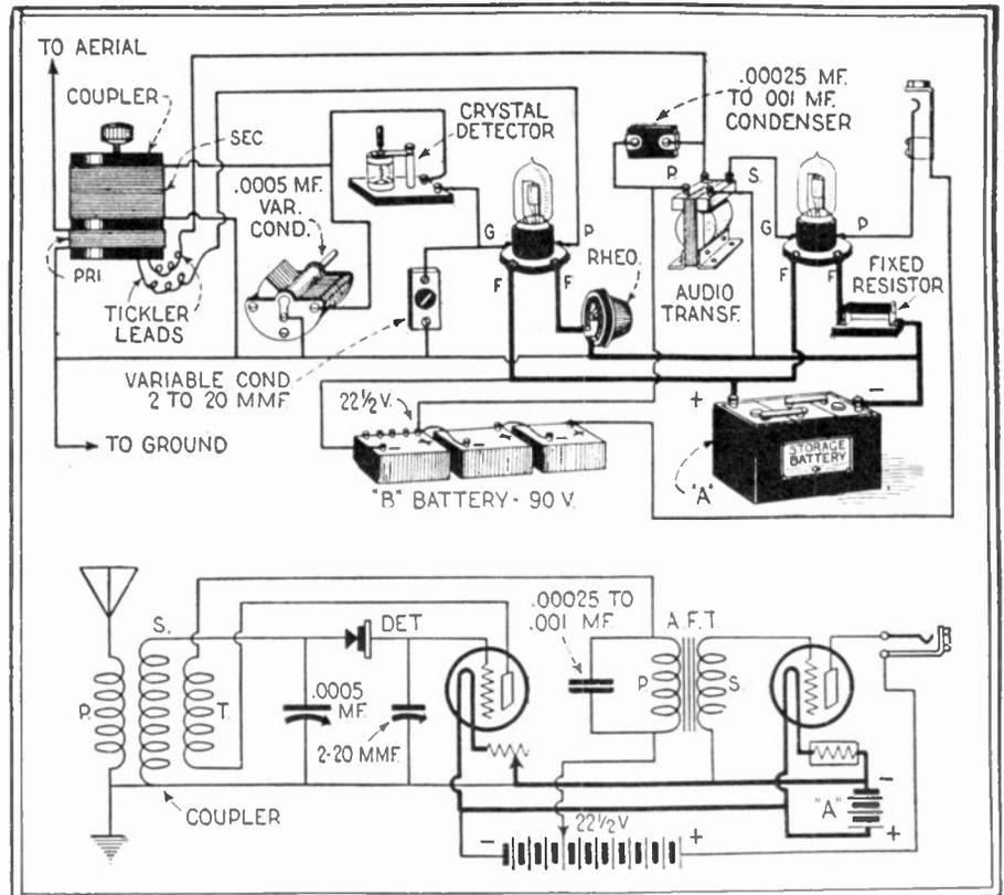
Fig. 111. The Interflex circuit, such as described in the December, 1925, issue of Radio News will give loud speaker volume on many stations if equipped with a single stage of audio-frequency amplification. The complete circuit for this work is shown in the diagram above.
