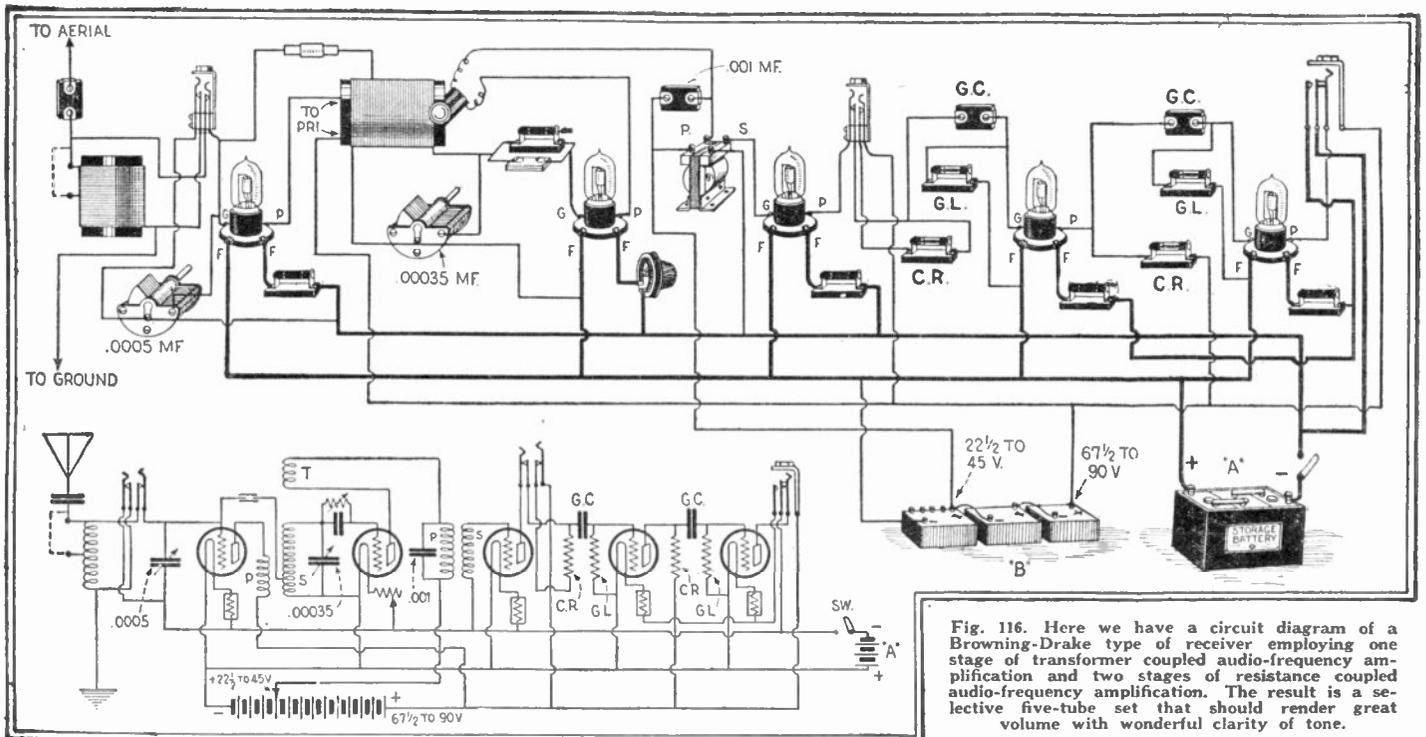
Fig. 116. Here we have a circuit diagram of a Browning-Drake type of receiver employing one stage of transformer coupled audio-frequency amplification and two stages of resistance coupled audio-frequency amplification. The result is a selective five-tube set that should render great volume with wonderful clarity of tone.
