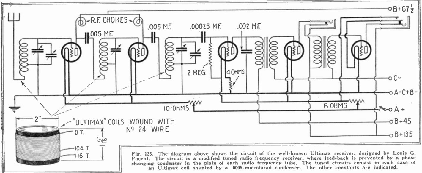
Fig. 125. The diagram above shows the circuit of the well-known Ultimax receiver, designed by Louis G. Pacent. The circuit is a modified tuned radio frequency receiver, where feed-back is prevented by a phase changing condenser in the plate of each radio frequency tube. The tuned circuits consist in each case of an Ultimax coil shunted by a .0005-microfarad condenser. The other constants are indicated.
