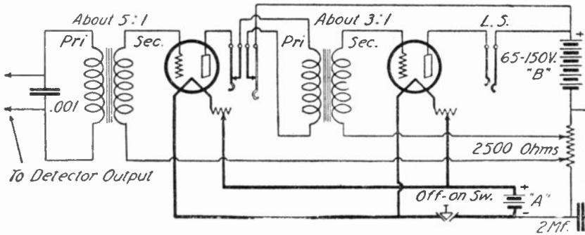
Fig. 11. "C" battery potential, but no "C" battery. Seemingly paradoxical, explained by the resistance in series with the "B" battery supply. The voltage drop is at negative potential.
