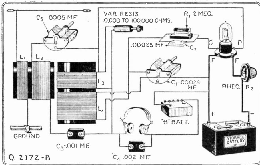
Fig. 82B. The Journal One-Knob Filter Tuner, is an efficient one-tube receiver which is very popular with New York fans. A consistent DX-getter, and yet easily operated. Either the dry-cell or storage-battery type tube may be employed, with practically equal efficiency.
