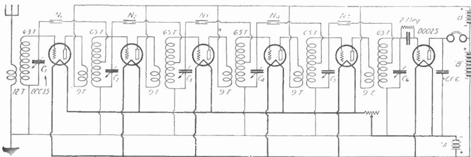
Fig. 74. This is an experimental Neutrodyne diagram. A detector rheostat, not shown, is required in the positive lead of this tube. Reception reports should be addressed to the "I-Want-To-Know" department.
