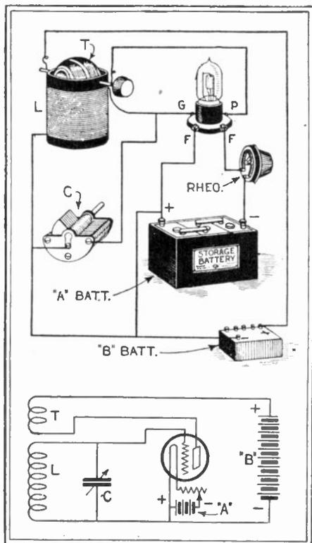
Fig. 256. Herewith is shown a fundamental oscillatory circuit.
