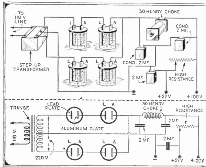
Fig. 168. No modern set is complete unless a good "B" battery eliminator is used to supply the "B" voltage to the plates of the tubes. By the use of large condensers and correct size choke coils the A. C. ripple can be eliminated.
