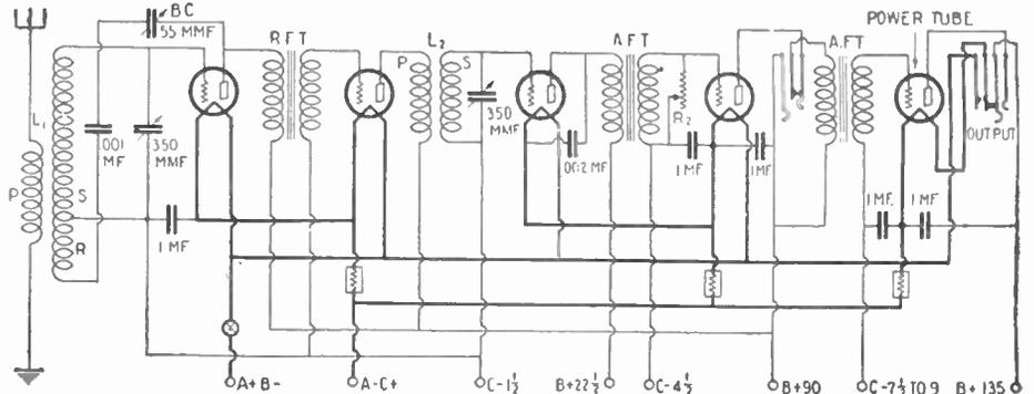
Fig. 94. The circuit diagram employed in the wiring of the Henry-Lyford receiver. A stage of neutralized T.R.F. is used in conjunction with an untuned stage, detector, and two stages of A.F. amplification. A power tube is recommended in the last audio stage.
