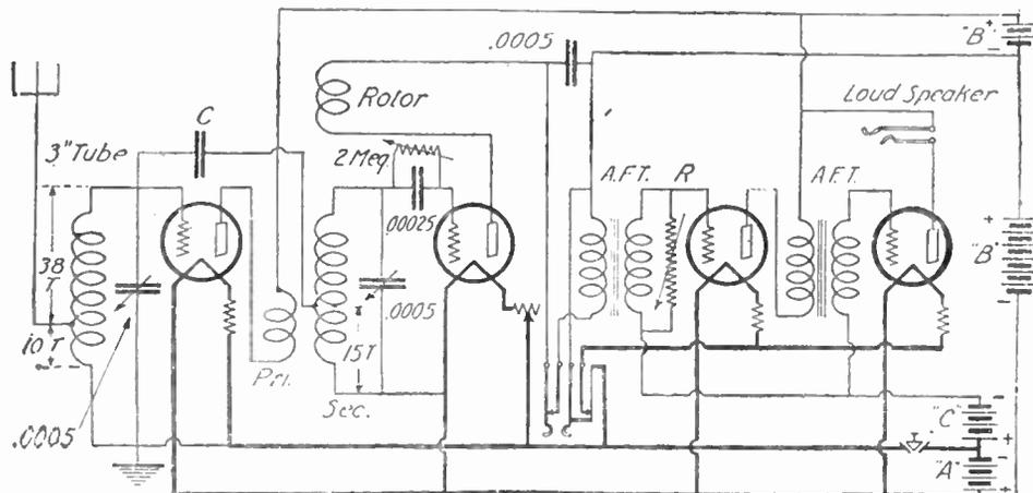
Fig. 71. Radio frequency amplification added to a regenerative receiver. This is possible only through extremely careful design and construction. This circuit shows how to do it. There are other features to this circuit, the Browning-Drake, as well.
