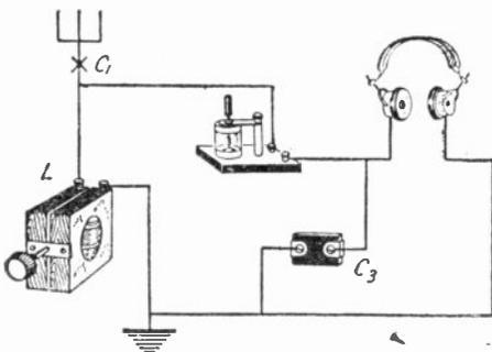
Fig. 16A. A complete radio set is shown. Anyone can make this receiver at slight expense. The few parts may be made or purchased.
