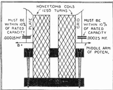
Fig. 244D. The design of the filter or input transformer. Although these coils may be wound similarly to ordinary transformers, ordinary honeycomb coils may be used with the same efficiency.
