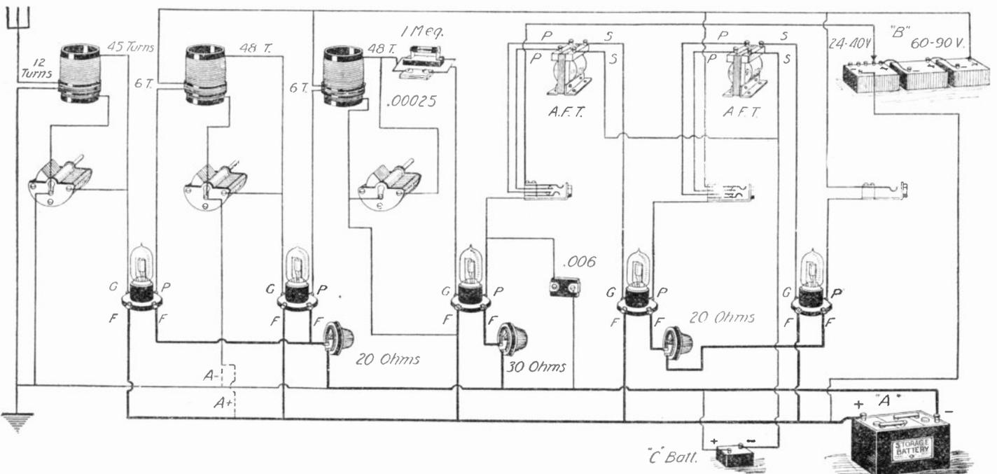
Fig. 73. The Freshman circuit, two stages of tuned radio frequency amplification (non-oscillating), detector and two stages of audio frequency amplification. Twenty-three variable condensers may be used. Once logged, a station will always be received at the same three points on the dials.
