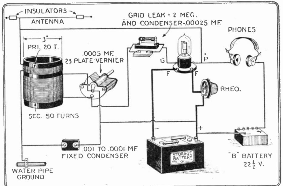
Fig. 83. The Journal One-Knob One-Tube set. An unusually efficient receiver employing regeneration, with only one dial to tune. Extraordinary results have been reported from this set.
