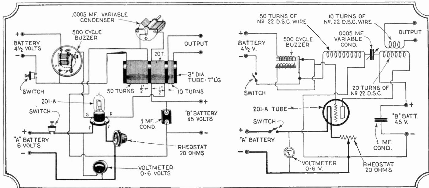
Fig. 260A. A laboratory is not complete without a calibrated oscillator. Full constructional details are given so that the experimenter can readily build one for himself. The list of materials is evident from the picture diagram, a shielded box being used to contain it.
