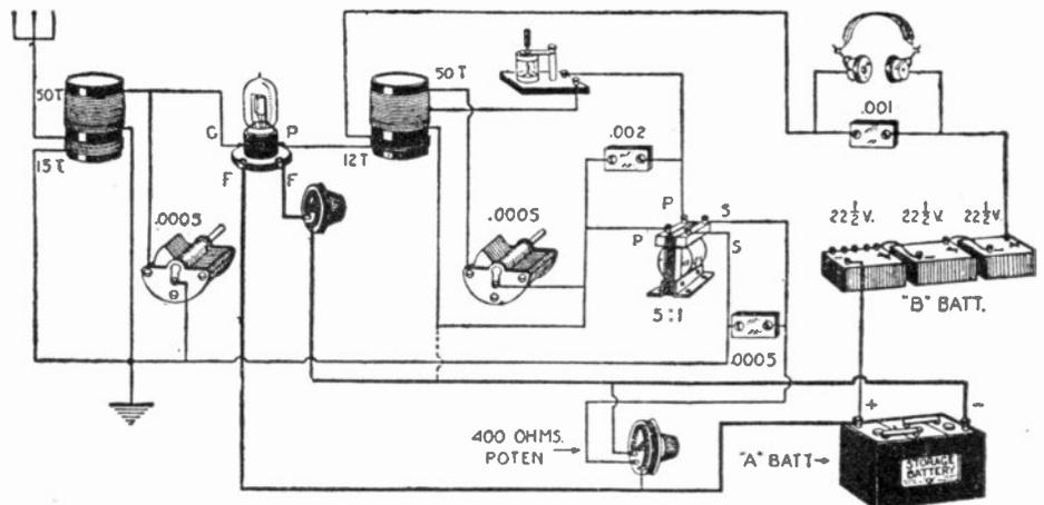
Fig. 78. This month we are showing an efficient 1-tube reflex circuit. Good quality and range are promised to constructors who build this set with care. An adjustable detector may be used, but fixed ones are now obtainable.
