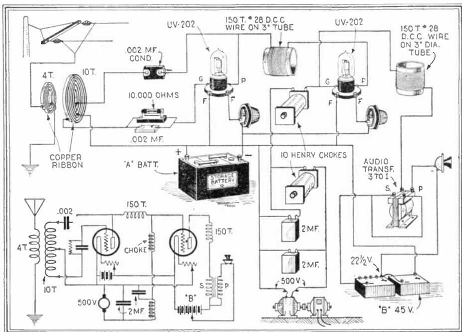
Fig. 141. The low power broadcasting set shown above can be used to communicate with stations about 10 to 15 miles apart. The modulation system is of the best and latest design.
