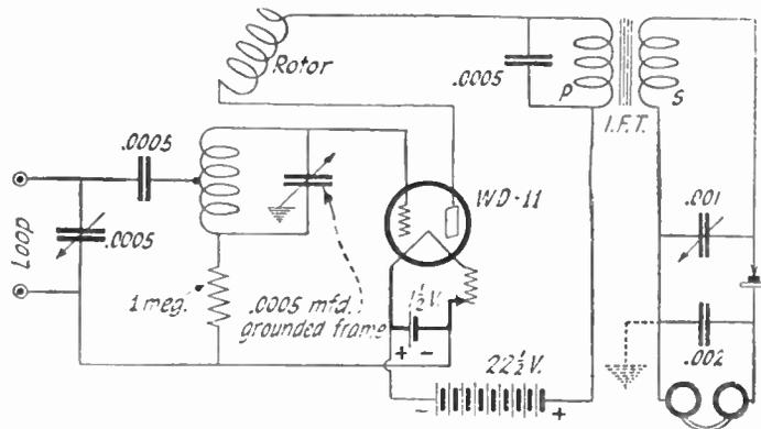
employment of a hard tube for detection, the gas content being relatively much lower, the negative charges, if no grid leak is employed, actually become sufficient to paralyze the rectifying action of a tube and no signals will be heard. In this connection especially when a high voltage "B" battery is used, it is best to use a grid leak.
