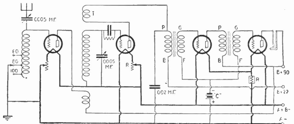
Fig. 24. The Arkay receiver, a very efficient and sensitive four-tube set, incorporating a stage of tuned radio-frequency amplification, the tuner of which is extremely novel, and a detector stage combining regeneration besides the usual two stages of audio-frequency amplification.
