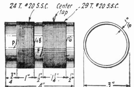
Fig. 244DO. Constructional data of an oscillator coil to operate in conjunction with the tuned intermediate-frequency transformer; designed so that it may be used in the Tropadyne, which receiver incorporates both detector and oscillator in one tube.
