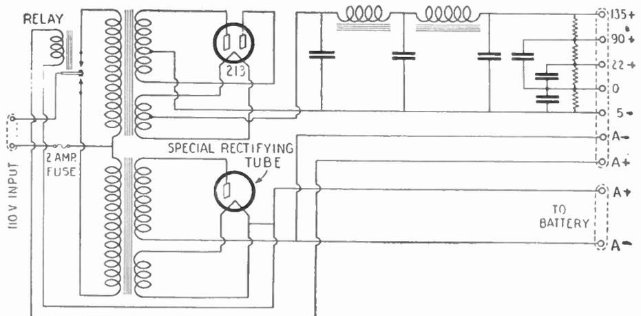
Fig. 162B. The wiring diagram employed in the Freshman "A, B and C" power unit. The "A" current delivered is really that of a trickle charger and is connected to a storage battery. This current is sufficient to keep the storage battery in a constantly charged state.
