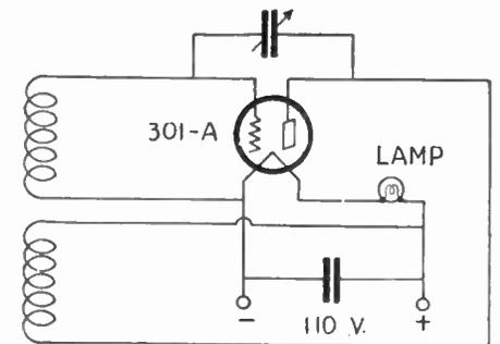
Fig. 250. An experimental oscillator utilizing the power line for its "A" and "B" supply.
