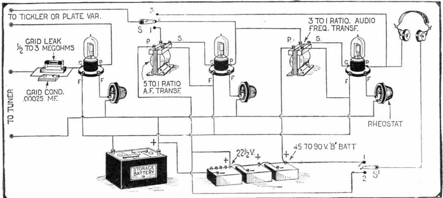
Fig. 284. Since jacks are rather inefficient instruments and often cause trouble because a slight amount of grit or dirt between the contact points causes an open circuit, they should be avoided. An efficient way of eliminating jacks is to make use of two switches, one of the three-point type and the other of the two-point type. All the necessary connections are indicated above and the manipulation of the switches is described in the text.
