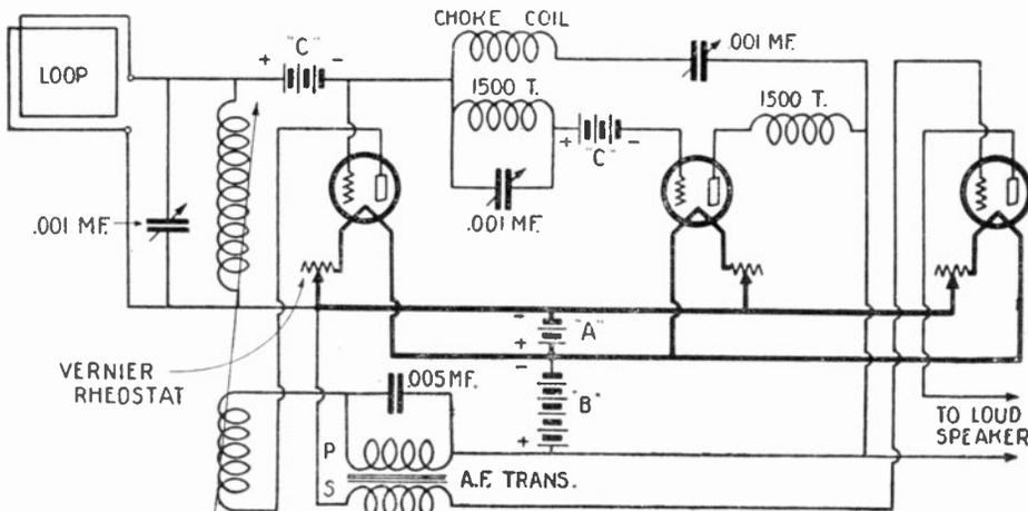
Fig. 25. A three-tube Super-Regenerative Circuit which the average constructor can build with the assurance that the troublesome defects, usually encountered in this type of circuit, are eliminated or minimized to a great extent. Very satisfactory loop reception may be expected, if this circuit is constructed properly.
