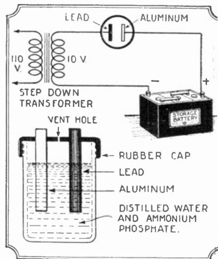
Fig. 160A. Wiring diagram of a trickle-charging system, and the construction of a chemical rectifier employed in trickle chargers.
