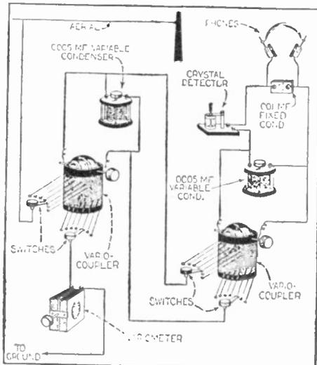
Fig. 301. In congested districts, a receiving set capable of very fine tuning is desirable. Such a tuner used in connection with a crystal detector is shown herewith.
