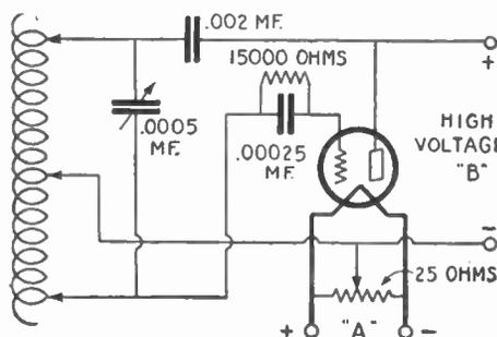
Fig. 241. Schematic circuit diagram of a laboratory type oscillator. This instrument is employed extensively for measurement and calculation work of radio apparatus. It can also be calibrated and used as a wave meter.
