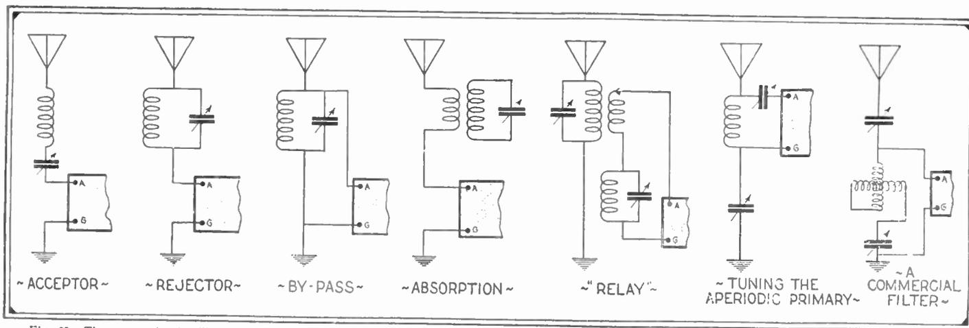
Fig. 63. The seven circuits illustrated in the diagram above cover the basic principles used in the design of interference eliminators or wavetraps. It will be found that each type is best suited to a condition, and a judicious selection is possible only after a reasonable amount of experimentation. In most cases the absorption filter will be found sufficiently practical for use in all but the most congested localities.
