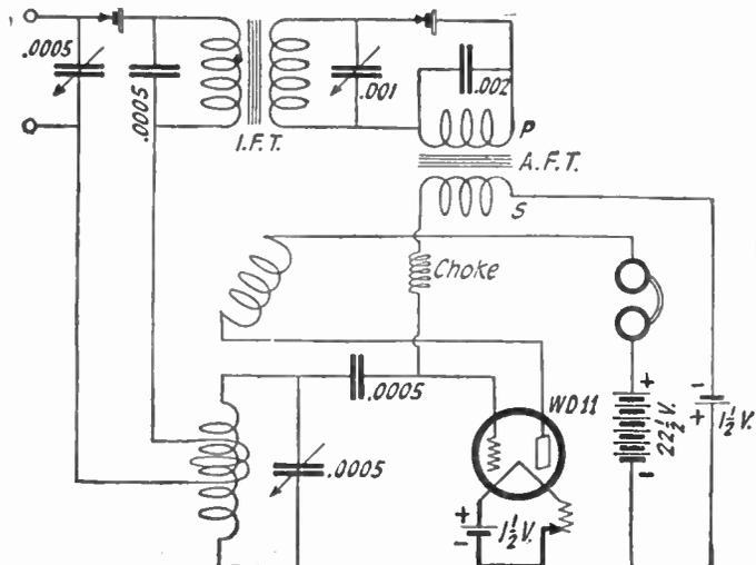
Fig. 5C. This circuit shows how it is possible to reflex the oscillator tube in a super-heterodyne in order to obtain an additional stage of audio amplification.
