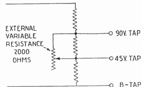
Fig. 165. Showing the use of a separate resistor to stabilize the output from a "B"-power unit.
