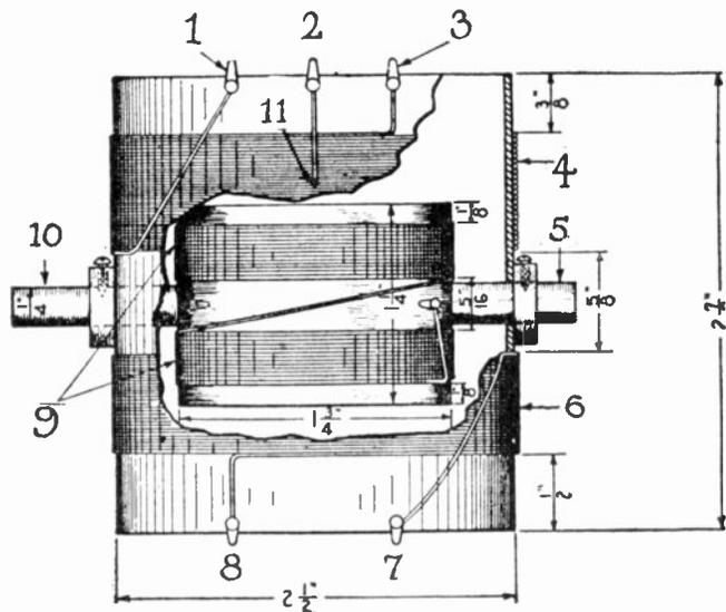
Fig. 242. Constructional and winding details of the Ghirard oscillator-coupler. This instrument may be employed as an oscillator coil in any other similar super-heterodyne circuit whose intermediate-frequency transformers have a characteristic peak of 5,000 meters (60 kc.)
