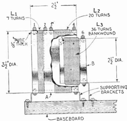
Fig. 240B. The design of an oscillator coil to operate in conjunction with a .001-mfd. variable condenser for a 10,000-meter type super-heterodyne receiver.
