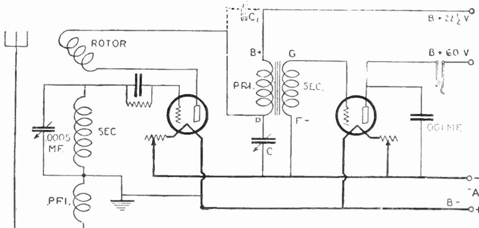
Fig. 21. A regenerative circuit employing the use of inductive and capacitive feed-back, termed "throttle control."
