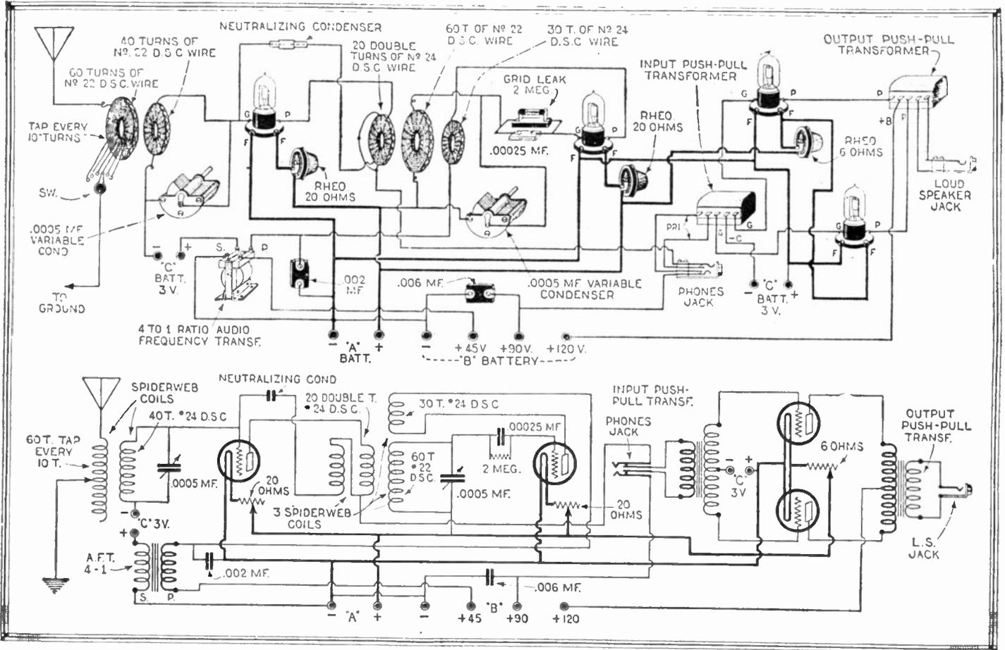
Fig. 99. The addition of a push-pull amplifier to the All Circuit Set will greatly enhance its reproductive qualities. This circuit is an entirely new one which is rapidly meeting with favor by all who have constructed it.
