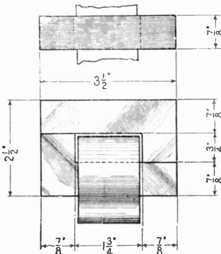
Fig. 184. The form above is that recommended by the manufacturers of the Raytheon tube for chokes and transformers in their "B" eliminator circuit.
