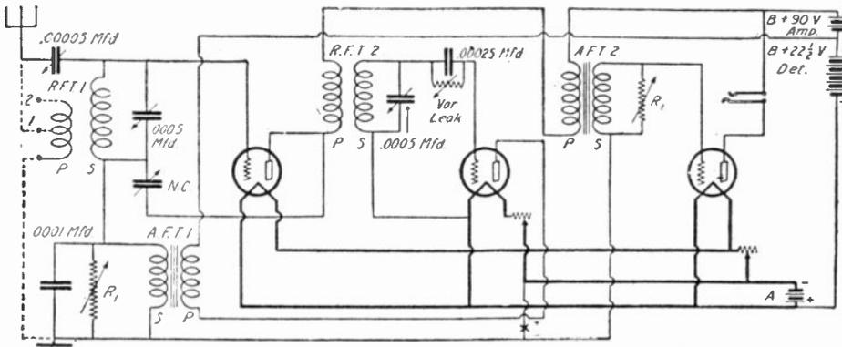
Fig. 76. The new Harkness reflex circuit, neutralized. This set will be found extremely selective if apparatus of good quality is used. Any type of tube may be used if sockets and rheostats are changed accordingly.
