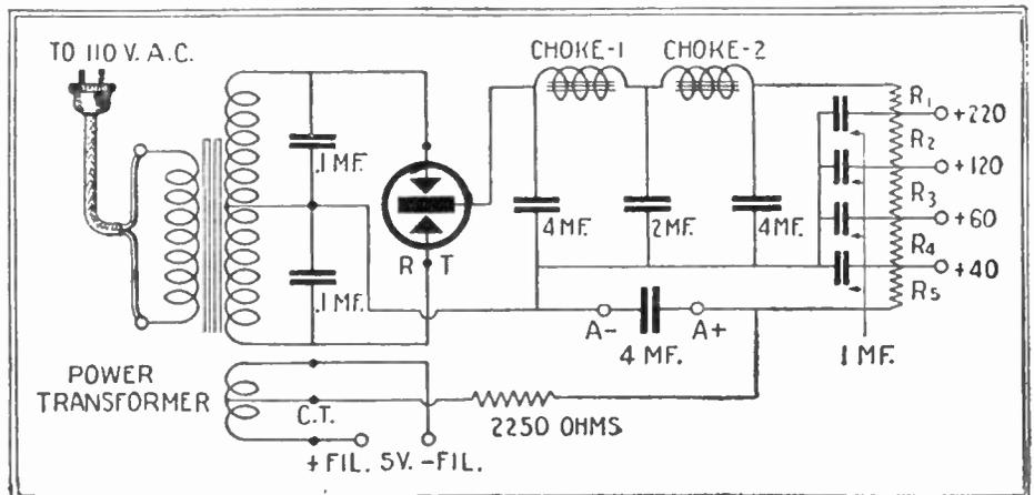
Fig. 161B. The schematic wiring diagram of an efficient "A, B & C" battery eliminator. This power unit may be used in conjunction with any type of receiver constructed along similar lines to those of the Varion A.C. set diagrammed above. A rectifying tube with a current output of 80 milli-amperes should be used.
