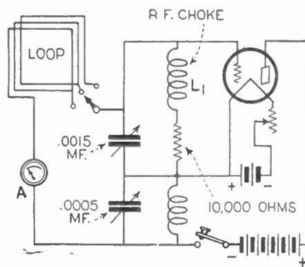
Fig. 138. A loop is used in this Portable Transmitter to give a directional effect to the signals.
