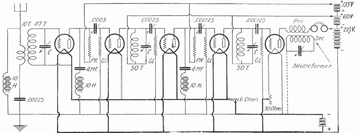
Fig. 14. This circuit is designed for the reduction of static effects to a minimum. During exceptionally strong static it may be advisable to disconnect the aerial and change the ground connection over to the antenna post. Note the neutroformer for regeneration.
