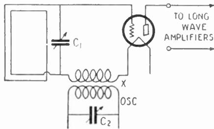
Fig. 66B. How the frequency changer of a super-heterodyne is shown in this schematic diagram.
