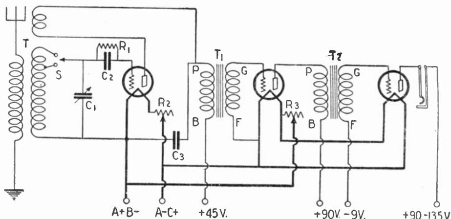
Fig. 97. A dual-range three-circuit receiver. By means of an S. P. D. T. switch it may be changed over instantly to the 150-200 meter band. This will be interesting to many experimenters.
