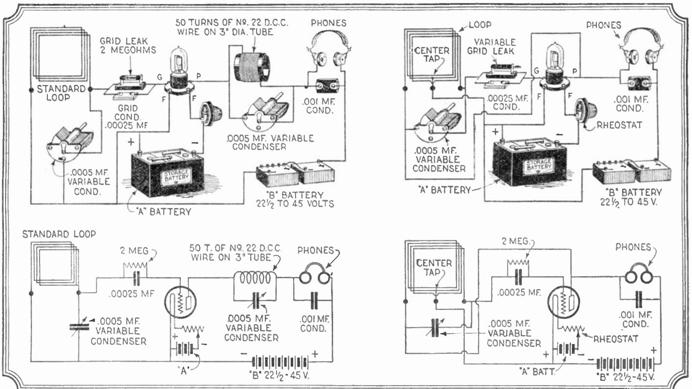
Fig. 43. Some very interesting results can be obtained with a single tube and a loop aerial when regeneration is employed to build up the signal strength. Two circuits for this work are given above. One uses a standard loop and the other a home-made type with a center tap.
