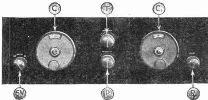
Fig. 93B. The panel view of the Dual T.C. receiver shows a neat and symmetrical appearance. The knob T controls the tickler, shown above; the knob P the primary, which is similarly wound on a rotatable form and may be varied in its relationship to the secondary. This primary knob on this receiver is marked "selectivity."
