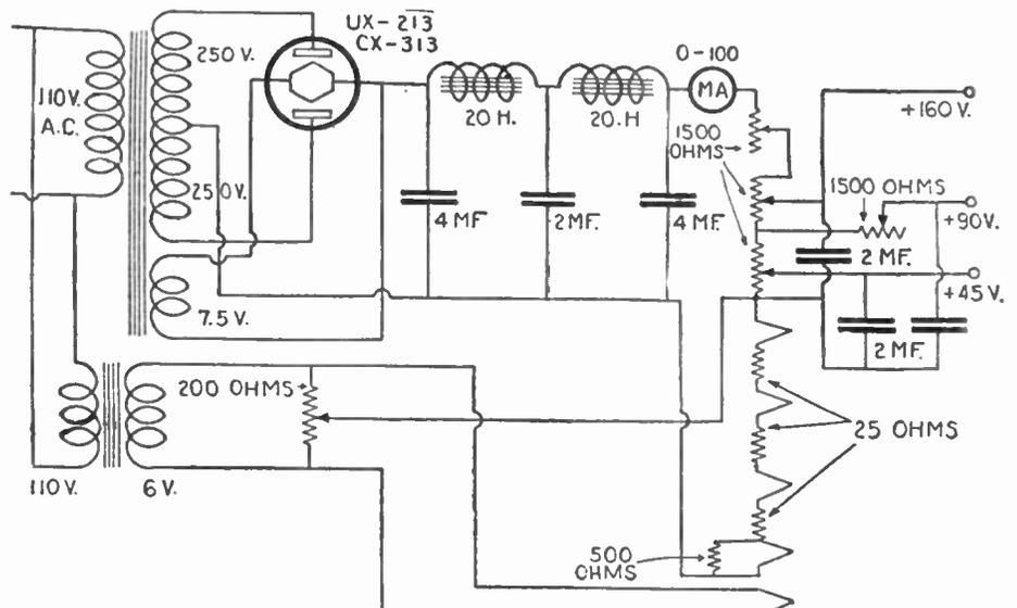
Fig. 156. "Just what you wanted." An "A," "B" and "C" battery eliminator, giving an unusually "pure" output, free from A.C. hum or distortion. Note that the filaments of the receiving tubes must be connected "in series," instead of the usual "parallel method."
