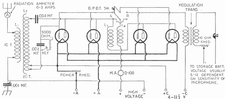
Fig. 134. A low power transmitter, which changes from phone to continuous wave transmission, by a throw switch. The very efficient Heising system of modulation is employed.
