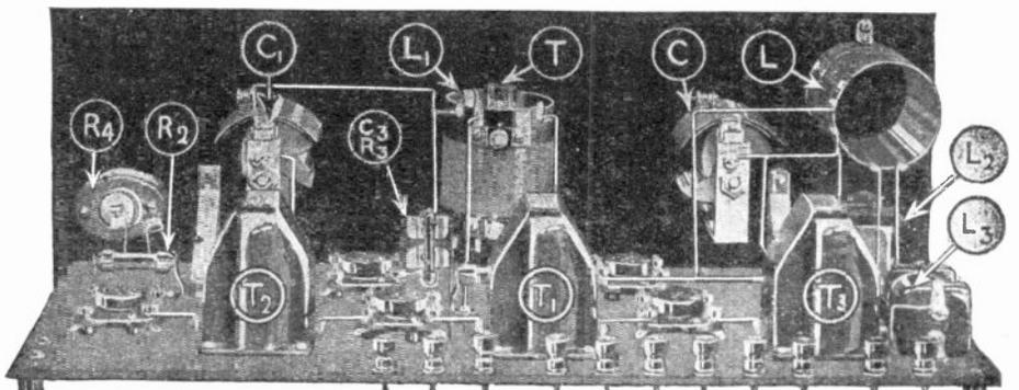
Fig. 93C. A top view of the Samson Dual T.C. receiver. A power tube is employed in the last audio stage to enhance the quality of reproduction obtained. A 500,000-ohm variable resistance to obtain volume control is also incorporated, and is indicated as R-4 in this view.
