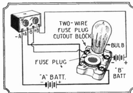
Fig. 209. One of the simplest methods of protecting the tubes of a radio set from being burned out is to place a current-controlling device in both the filament and plate circuits. Above, a 40-watt bulb is placed in series with the negative B-battery lead, with a small fuse in the A-battery circuit.
