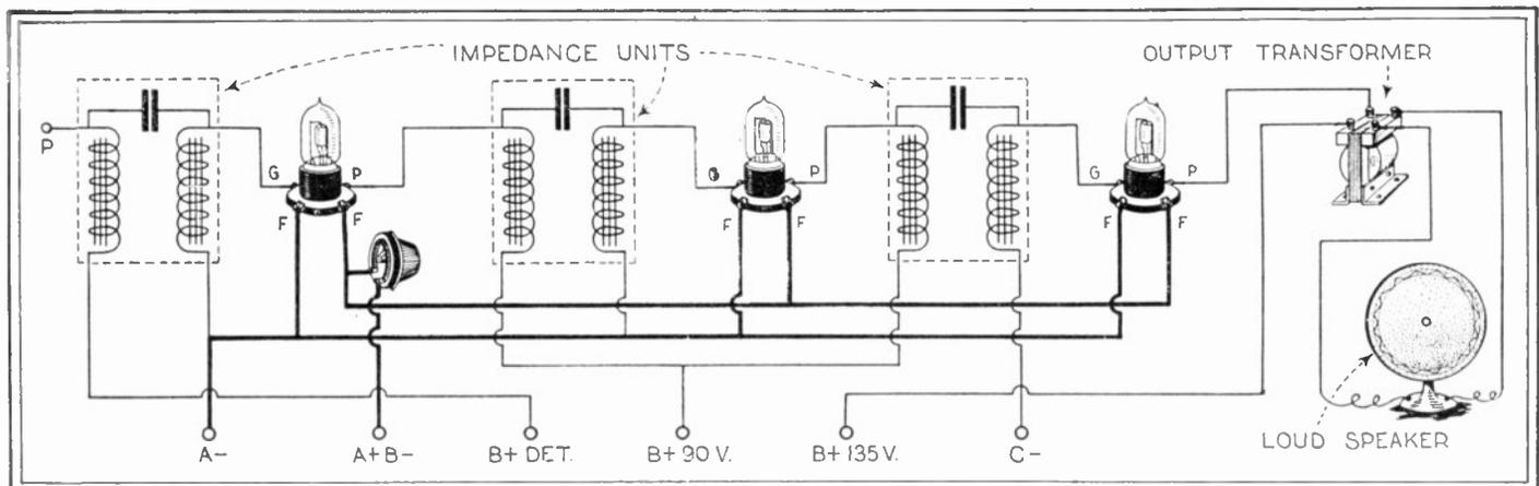
Fig. 32. Several manufacturers have recently introduced amplifiers employing the Donle system of impedance coupling, the circuit diagram of which is given above. The amplification available with this system is nearly equal to transformer coupling, and is almost completely distortionless.
