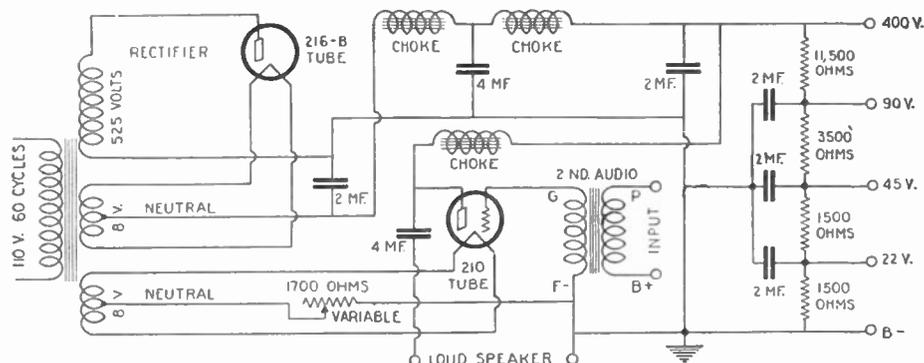
Fig. 158. A one-stage power audio amplifier, operating direct from the A.C. lighting socket, which supplies both A and B current for this particular unit. There is also a sufficient remainder to supply "B" current for the receiver.
