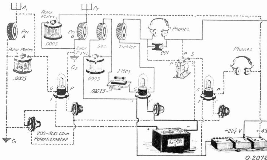
Fig. 67. Picture wiring diagram of three-tube regenerative receiver using honeycomb coils.
