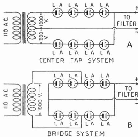
Fig. 164. Two very effective methods of connecting a high voltage rectifier. The number of jars is computed as explained in the text.
