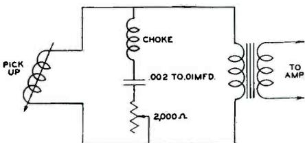
honeycomb coil or a standard 125 or 85 millihenry choke. All three units are obtainable from any radio store but if the reader wants to roll his own, wind approximately 1800 turns of No. 28 d.c.c. wire on a form 2 inches in diameter by 1½ inches long.
