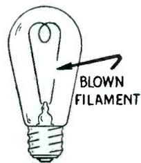
For use in a wave meter the filament can be used either intact or "blown." With a whole filament the usual glow is produced just as with a neon. With a blown filament the tuning is sharper. Operating in series will produce a broader glow point than if the lamp is shunted across the circuit. The filament can be blown by shooting about 500 volts through it.
