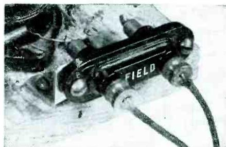
soldered to the tip. The knurled nut should be drilled out so that it can be passed over the phone tip and soldered to the end, as illustrated. The knurled edge makes removal and insertion of the tips, extremely simple.
