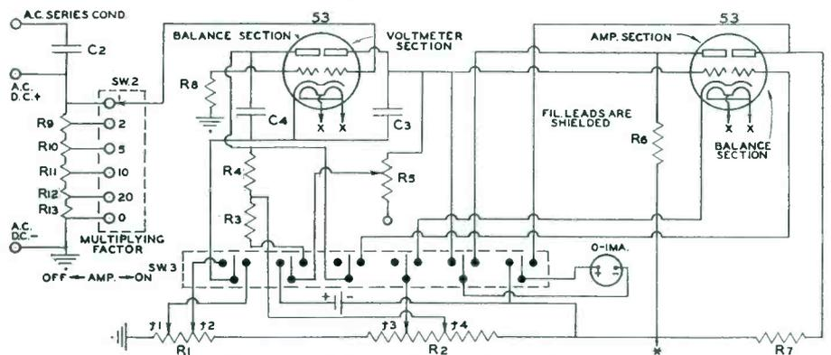
The circuit of the 2-5 Vacuum Tube Voltmeter.
