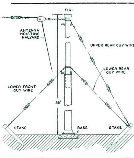
mast 22 feet high. The constructional details given here can easily be modified if masts of lesser heights are desired.
