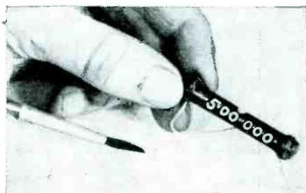
when selecting the correct resistor in set building or in repairing. Condensers, r.f. chokes, etc., too, can also be labeled with their capacities.
