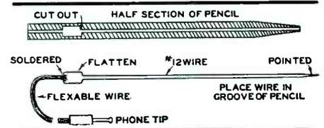
number 12, hard copper wire. Cut two 5 1/4-inch lengths, sharpen points on one end, flatten the other ends. Then solder four feet of flexible wire to the flattened ends. Place into the pencil as shown, and cement it together. Fix carter phone tips or spade tips to the end of the flexible wire and you have a good pair of test leads.
