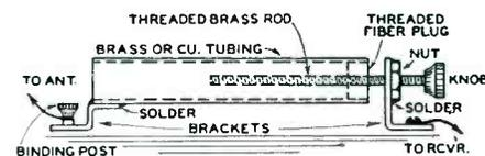
Attach a bakelite binding post knob to one end of the threaded rod. Run the rod through the brass nut and threaded plug as shown. The antenna lead-in is connected to the binding post and the wire to the receiver grid circuit to the brass nut. Screwing the thread in the tube increases the capacity; threading it out decreases it. If there is any tendency for the rod to touch the inside of the tube, line it with paper.
