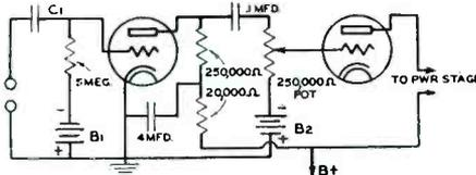
The reason for the tendency toward motor-boating is that all of these tubes unfortunately have a common cathode. That is, each section has its own grid and plate, but there is only one cathode for both. This means, where cathode bias is used, that there is coupling between the first and second plate circuits, regardless of the size of the cathode by-pass condenser.
