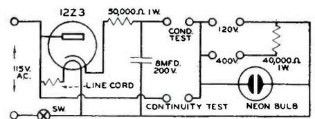
system comprises a 50,000 ohm 1 watt resistor and a 200 volt, 8 mfd. condenser. The neon lamp can be either the  $\frac{1}{2}$  or 1 watt size. When testing the condition of condensers a pair of test prods should be plugged into the jacks marked "condenser test." For testing resistors or other parts for continuity the test prods should be plugged into the jacks marked "continuity test" as shown in the diagram.
