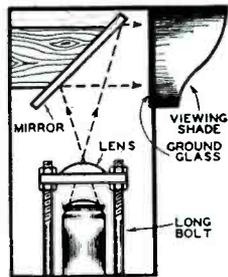
The mirror is mounted on the wall of the cabinet by a wedge-shaped piece of wood. This mirror should be placed at a 45 degree angle and it is mounted approximately 4" above the tube. Place the groundglass screen 4" to 5" from the mirror and over the 3"
