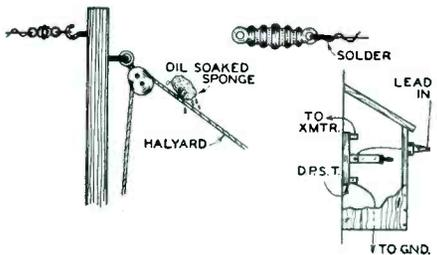
Before reeving in any new halyard it will be wise to weatherproof it as follows. Fill a bucket with boiled linseed oil and coil the rope into the bucket. Leave it there overnight. Then stretch it between posts and wipe off all extra oil, catching this in a bucket as you work along. Such treatment makes the rope pliable and just about doubles its life.
