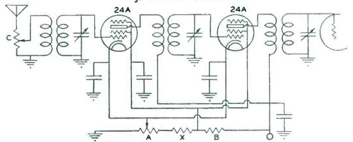
A is old volume control. B is old screen resistor.
