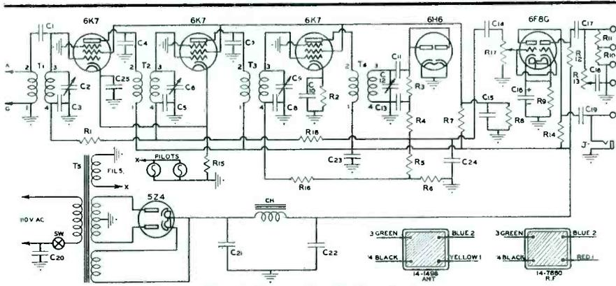
Circuit diagram for the P.A. Tuner.
