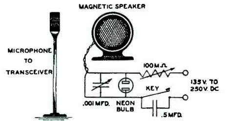
Connect the output to an old magnetic speaker, turn on the power and press the key. The neon bulb will oscillate and produce a tone in the speaker. Its strength can be controlled by the variable resistance while the pitch can be varied from a low note of only a few cycles to one of the highest audible frequency by means of the tuning condenser. The note can be transferred to the transceiver by placing the mike close to the speaker and will not interfere with voice unless the key is depressed.
