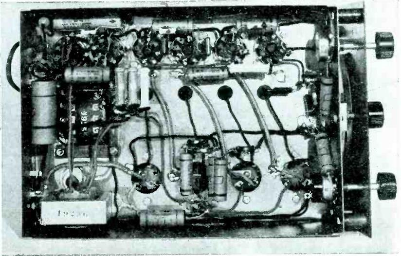
Simplicity of control, including a phone jack, make this P.A. Tuner the ideal for use by the serviceman. The parts connected to each tube are grouped around that socket to give the best reception afforded by short leads and feed-back free operation on local signals.
