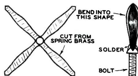
length of the intended plug. Spot the center and draw a line to each corner. Then draw in the legs approximately the shape suggested. Cut out the cross with a pair of tin shears.
