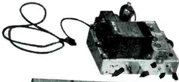
The complete Video Section hooked up ready to transmit a picture. The radio frequency section is not shown.
