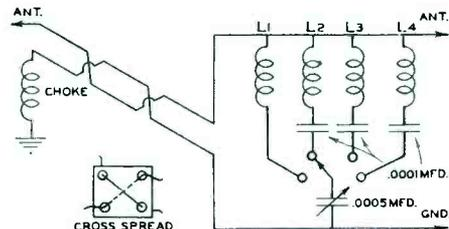
more upon boosting the desired signal than suppressing lead-in pickup. This is accomplished by tuning the antenna circuit to the desired wave-length. No impedance-matching transformers are needed. The antenna proper may be anything from 25 to 75 feet long. The lead-in, doubled upon itself, is made practically non-inductive, and its capacity minimized, by the spacing, 1½ inches. Transpose every four feet with 2 inch square spacers, which can be threaded on and worked along to position.
