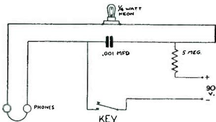
Pressing the key completes the circuit between lamp, phones and resistor and causes the lamp to oscillate. For normal use set the resistor at about  $1\frac{1}{2}$  megohms. Lowering or raising the resistance will alter the pitch of the signal.
