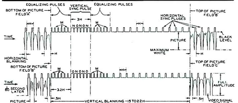
Figure 5. A diagrammatic breakdown of a television signal.
