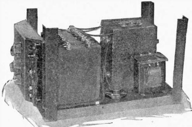
FIG. D. The "B" power section of the double-deck unit illustrated opposite.
