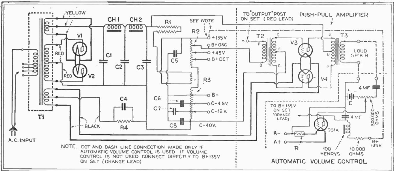
FIG. 4. THE SCHEMATIC DIAGRAM OF THE POWER UNIT, THE AMPLIFIER AND THE AUTOMATIC VOLUME CONTROL THAT THE AUTHOR SUGGESTED IN HIS NOTES ARE SHOWN HERE
