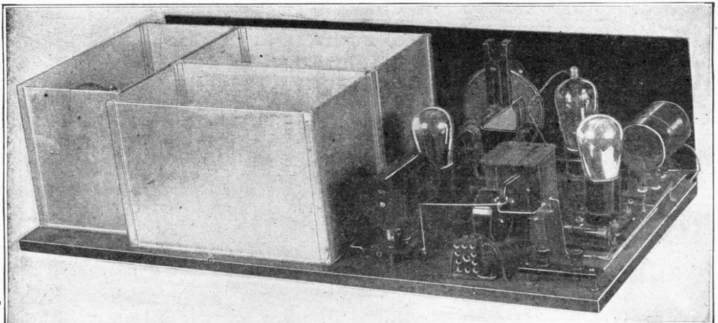
The modulator tube, between its tuning condenser and coil, is in need of no shielding; neither are the second detector and first audio-stages, here shown at the rear right. The shielded oscillator is in the forward can; the intermediates in the other two.
