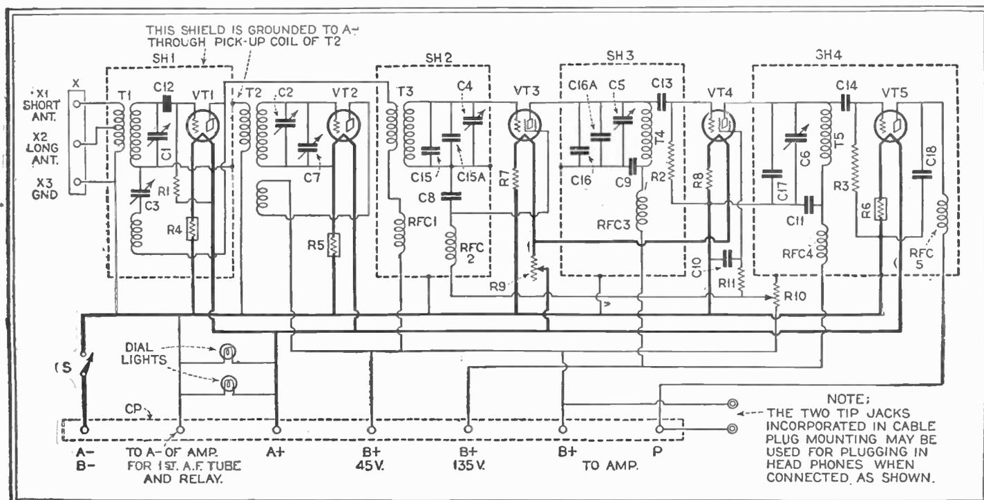
In the "Band-Isolator" circuit, it will be seen, a large number of condensers are used; these, however, are in parallel, to facilitate exact adjustment of the
