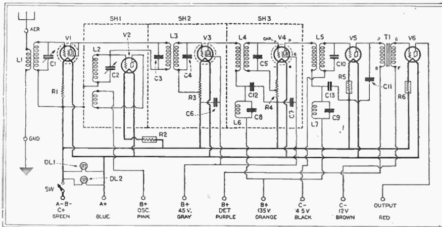
FIG. 7. The schematic diagram is shown here. The screen-grid tubes will be seen in the modulator and the intermediate frequency circuits.
