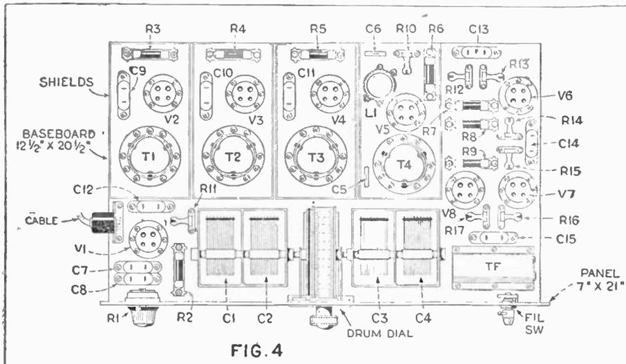
The layout diagram above, when compared with the list of components on page 1139, and the photographic illustrations, will clearly identify each part.
