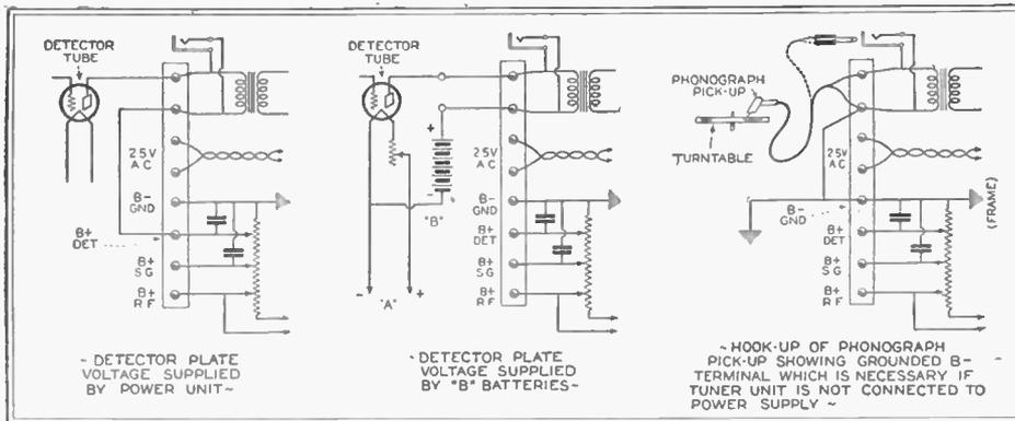
FIG. 2. The "Velvetone" is connected to an A.C. tuning unit externally, as at the left; to a D.C. tuner as in the center diagram; while the connection at the right gives phonograph reproduction of a high quality with volume of any desired amount. It will operate three or more loud speakers.
