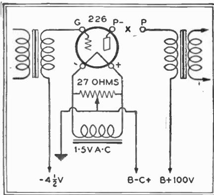
FIGS. 3 AND 4, ABOVE AND AT THE RIGHT, SHOW THE CONNECTIONS TO THE TEST SET WHEN TESTING, RESPECTIVELY, A D.C. AND AN A.C. AMPLIFIER STAGE
