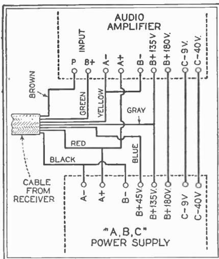
Connections for the cable from the tuning unit to audio amplifier and power unit
