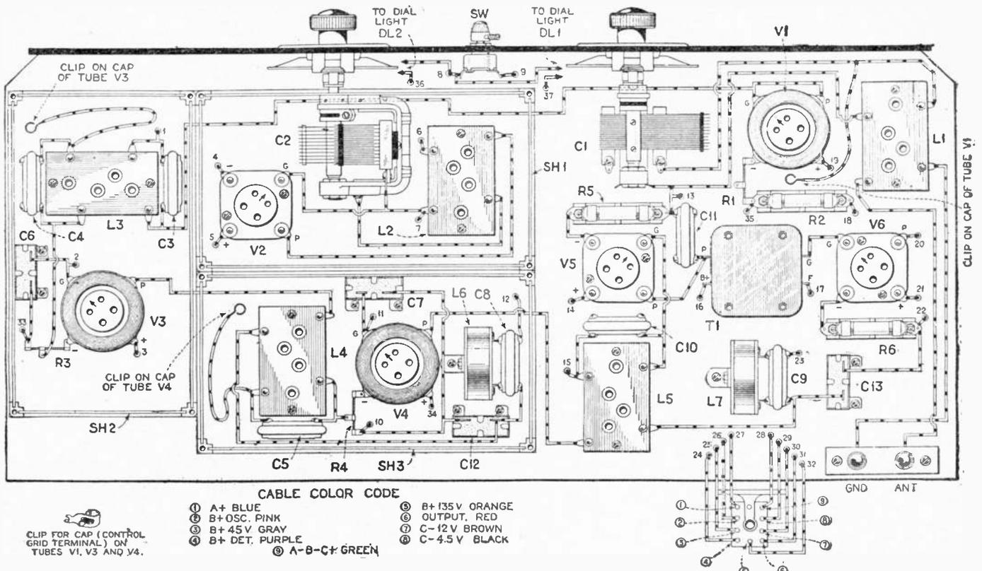
FIG. 2. THE POSITIONS OF ALL THE APPARATUS IN THE SET ARE SHOWN IN THIS ILLUSTRATION. FIGS. 1 AND 2 CAN BE USED FOR WIRING THE SET, AFTER THE APPARATUS HAS ALL BEEN MOUNTED
