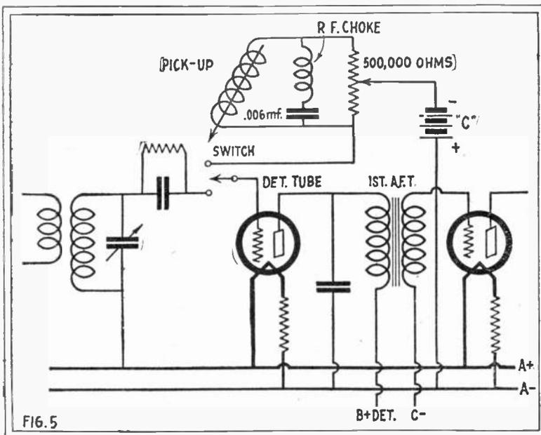
In the electric phonograph pick-up, a permanent magnet is also used, a coil, or several coils, is placed near the magnet and a thin
