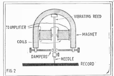
The electric pick-up vibrates more freely than the older unit; but its output may be amplified to any volume desired.
