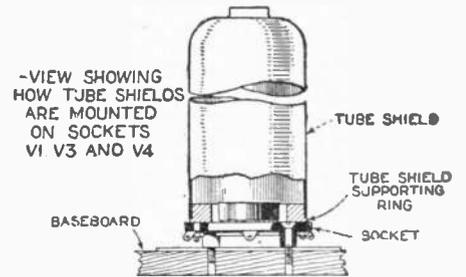
to use a flat-head machine screw. Then remove the thumbscrews and nuts which are holding the floating part of the socket. Once the screws are removed, be careful not to turn the center part of the socket, since each blade must remain in its original position.
