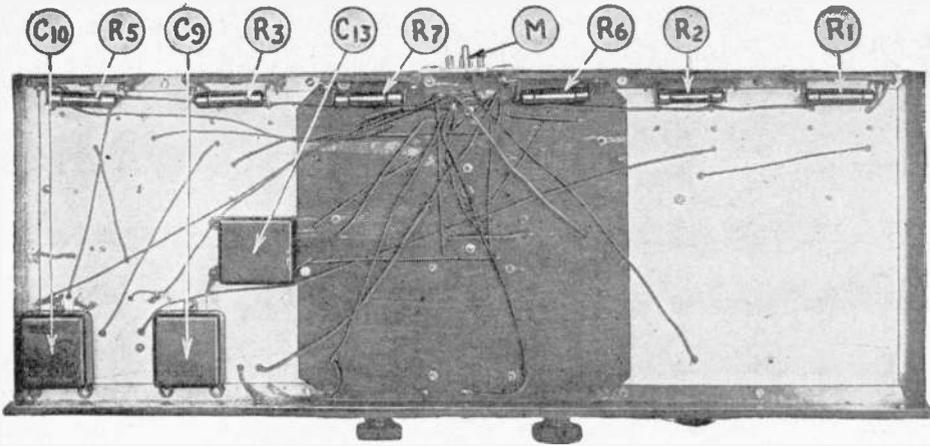
The central sub-panel, of insulating material, and the bottoms of the shield cans on either side, carry the limited apparatus shown on the under side. The wiring which comes through should be carried direct from point to point, and be well insulated.
