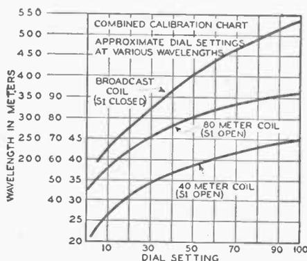
FIG. 2. A calibration chart of the plug-in coils.
