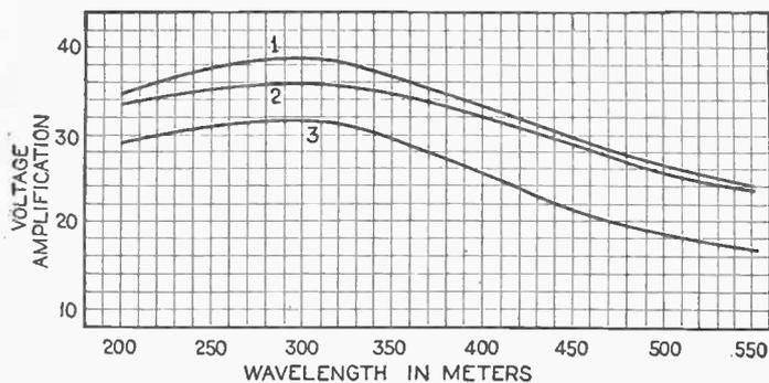
FIG. 5. These curves are plotted to show the change of voltage amplification of the 1 1/4" coil, inside and outside of shield cans
