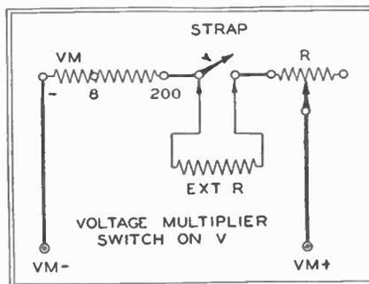
FIGS. 5, 6 AND 7, SHOWING CONNECTIONS FOR THE RHEOSTAT (R), SERIES-PARALLEL SWITCH; ALSO VOLTMETER PIN-JACKS AND BINDING POSTS FOR CUTTING IN EXTRA RESISTANCE
