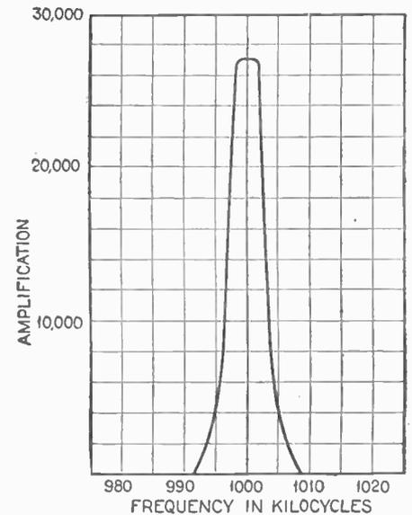
FIG. 3. Here the tuning has been slightly staggered to obtain a flatter peak—hence less side-band cutting
