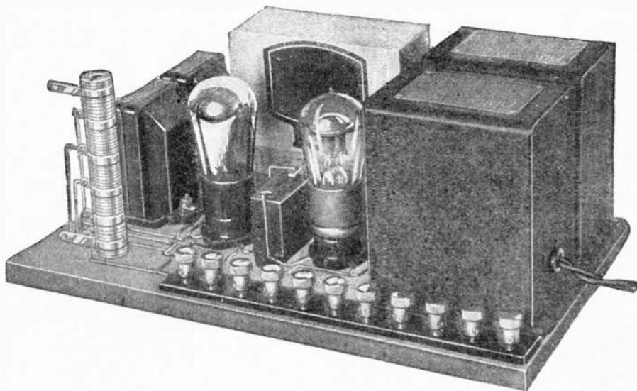
THE COMPLETED COMBINATION AMPLIFIER-POWER SUPPLY UNIT. IT SHOULD BE COMPARED WITH THE LAYOUT OF PARTS ON PAGE 64
