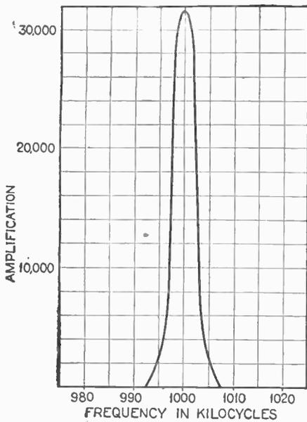
FIG. 2. This curve shows the selectivity effect of four tuned stages, each stage tuned alike
