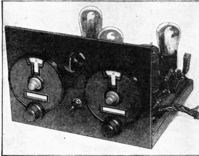
incl. forms. The secondary of each coupler contains 86 turns of No. 28 S.S.C. wire. The turns should be space-wound, by placing a piece of silk sewing-thread beside the wire. The primary of each coupler contains 15 turns and the tickler (on the detector coupler) 20 turns.
