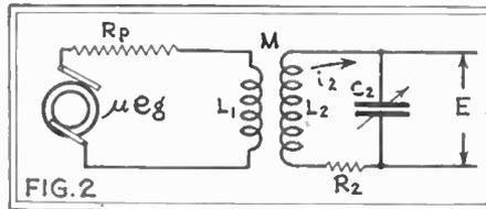
The virtual circuit of Fig. 1, showing the "mu" of the tube as a factor of the input, and its plate resistance at Rp.
