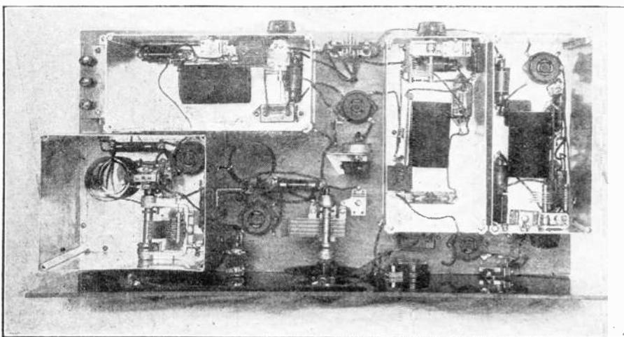
Looking down on the completed band isolator receiver, with shield removed to show the various parts
