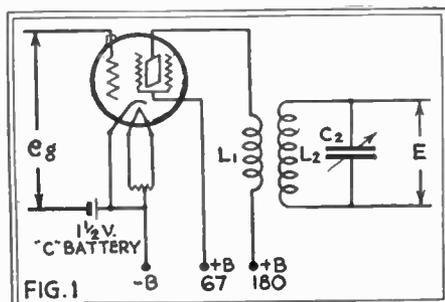
The schematic circuit of a screen-grid stage of R.F. amplification, indicating both input and output voltages.
