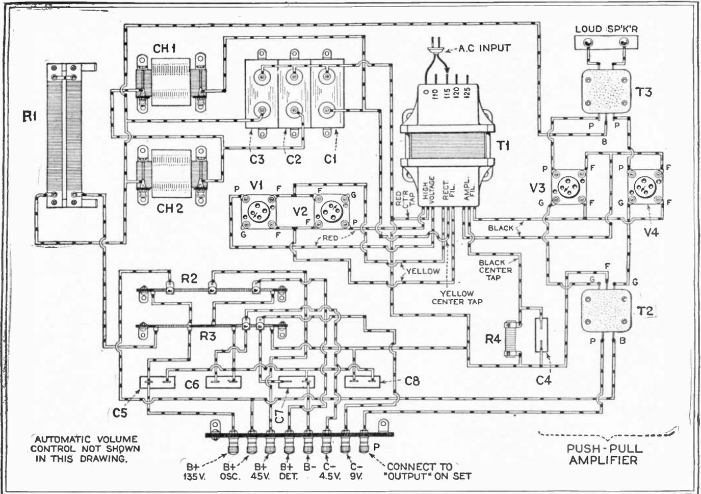
FIG. 6. THE LAYOUT OF THE PARTS IN THE POWER UNIT AND AMPLIFIER FACILITATES THE CONSTRUCTION AND WIRING OF THE UNIT. SOCKETS V1 AND V2 ARE FOR THE UX281 RECTIFIERS; V3 AND V4 ARE THE AMPLIFIER SOCKETS
