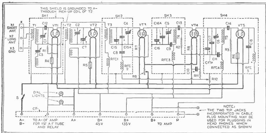
This circuit diagram of the band isolator receiver embodies a correction which should be noted. The original diagram on page 61 failed to include condenser C17A, in shield can SH4
