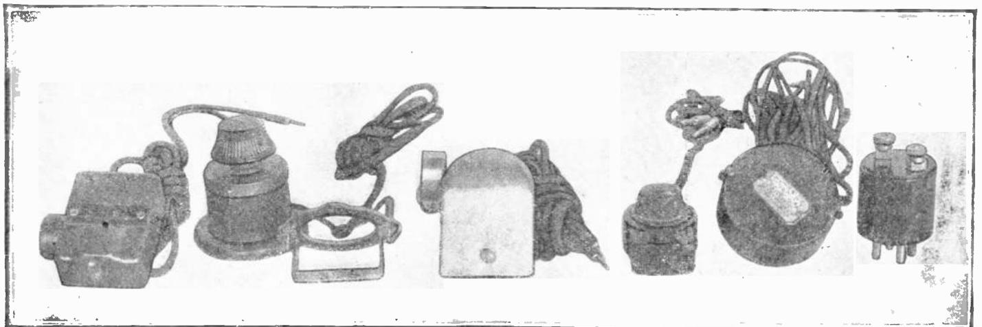
Commercial apparatus for converting a receiver to phonograph use. Left to right, a pick-up with control, an adapter making a detector the first A.F. stage, a pick-up, a remote-control device, a
