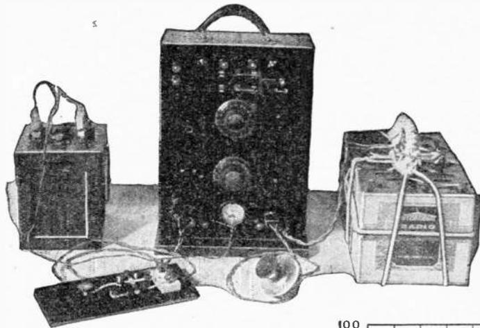
THE 80 METER TRANSMITTER WITH COMPLETE ACCESSORIES. ITS SIMPLICITY AND COMPACTNESS ARE APPARENT
