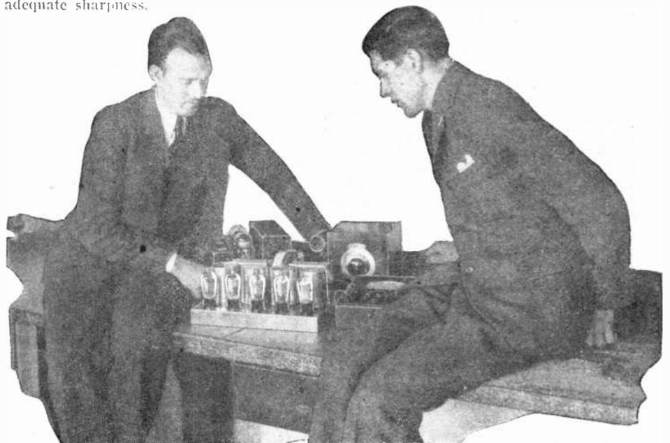
Dr. Browning (left) is well known to our readers as co-inventor of the Browning-Drake circuit. He is exhibiting here a tuning unit with four R.F. stages, using the transformer constants calculated here, and detector. It is designed to feed into the "Velvetone" amplifier seen behind it, and described on page 1099 by James Millen (right).
