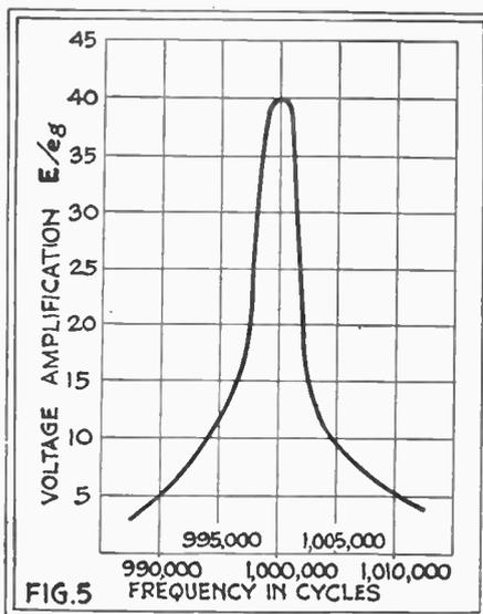
FIG. 5 Above the curve of a transformer designed as described here. In the complete tuner, for of these are used, their peaks staggered to give a band-pass effect.
