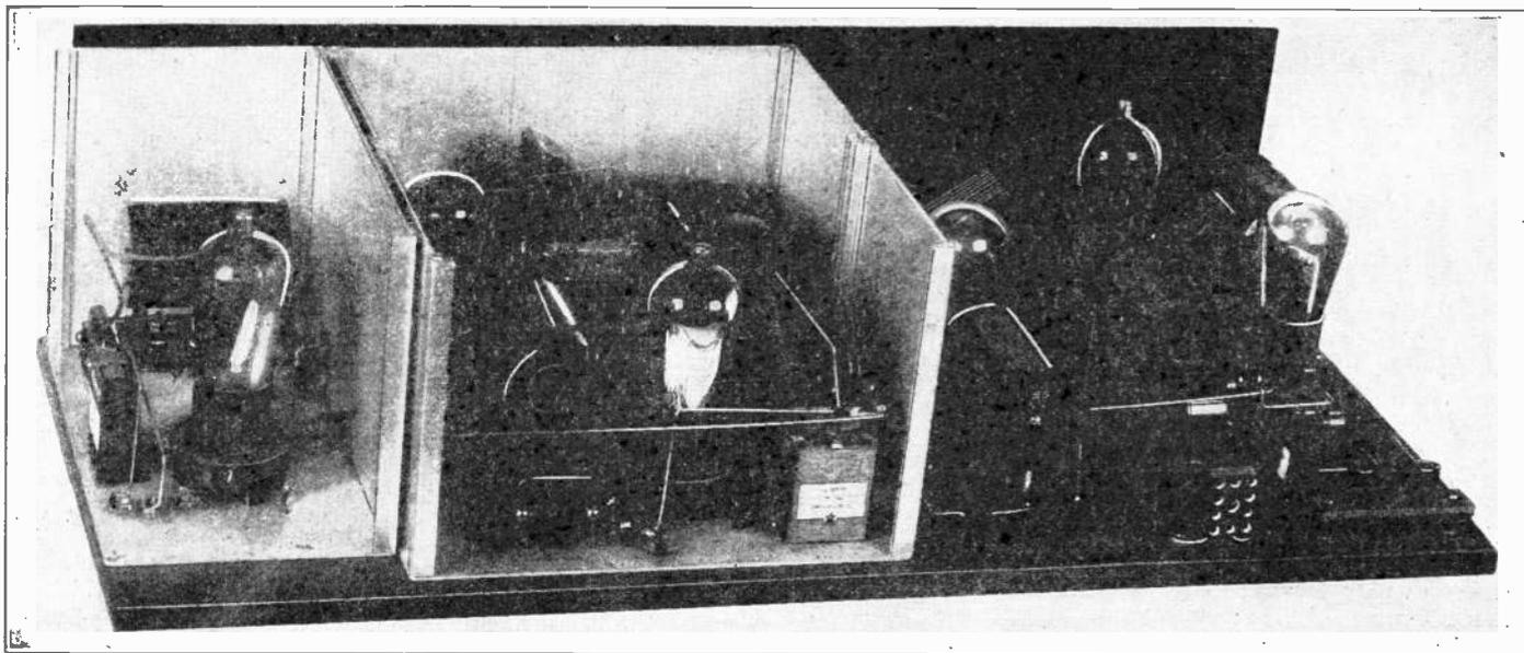
The "RE 29" is shown here with its rear and partition shields removed. The wiring is run with the utmost directness. The first or modulating tube, which in this system is not a "detector," employs its screen-grid and plate as a single element, of high effectiveness.
