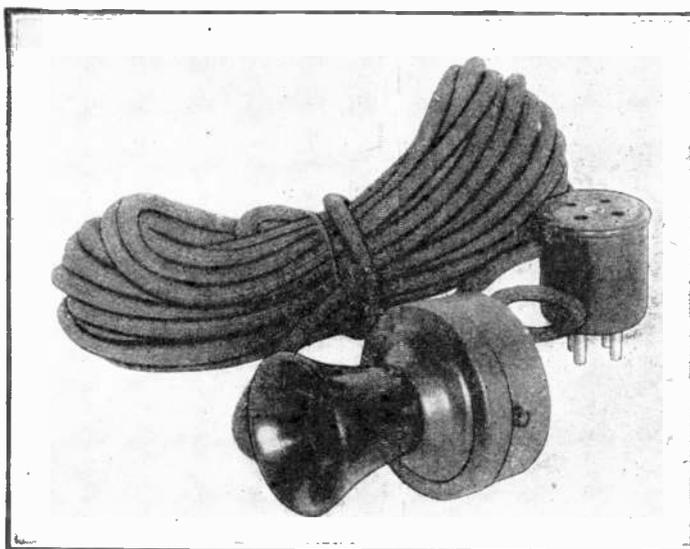
With a small microphone connected to the detector socket by a plug, speech is clearly reproduced through the A.F. amplifier of a receiver.
