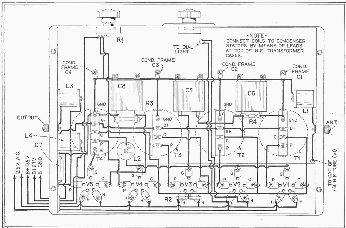
As this picture wiring diagram shows, all the wiring, with the exception of the leads to the caps of the screen-grid tubes, is made underneath the base
