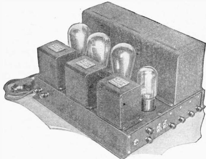
FIG. A. A front view of the "Velvetone" amplifier assembled. The power transformer, filter chokes and large Mershon condenser are in the rear cases; the three audio transformers in front. The terminals at the side are connected to other apparatus as shown in FIG. 2.
