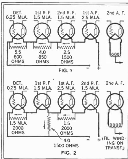
Series filament wiring with 60-milliamperes tubes requires some compensating resistors. Fig. 1 is a usual, and Fig. 2 an improved circuit.
