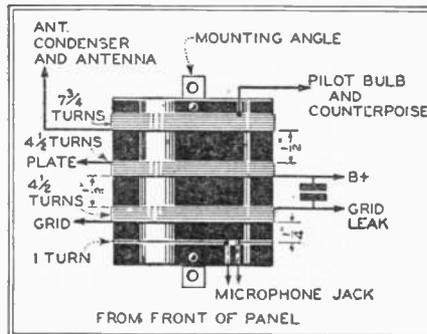
FIG. 5—DETAILS OF THE COIL CONSTRUCTION
