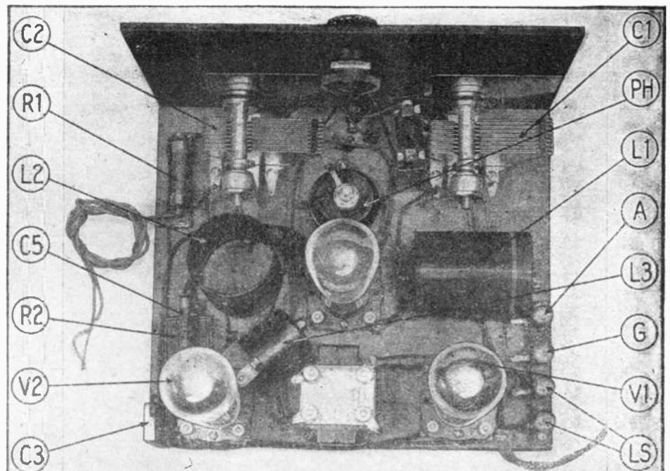
*The layout of parts in the "Beginner's Three" is shown so well above that a diagram is hardly needed but the wiring may be traced with the aid of Fig. 2. The leads at the right are for the "B" and "C"; those at the left for the "A." The arrangement is convenient.*
