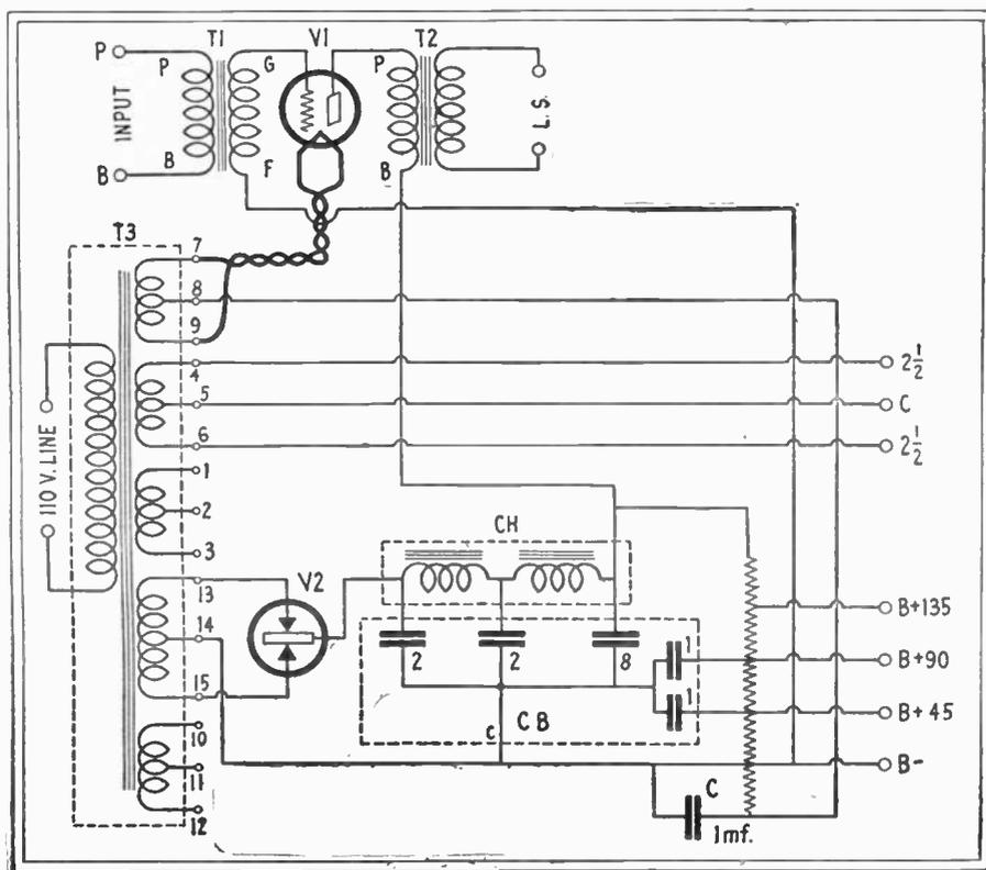
manufacture as the transformer and is designed to operate in conjunction with this power transformer. The condenser block has a sufficiently high working voltage so that no trouble will be encountered from breakdown. The voltage divider has a number of output taps which are used to supply the required "B" voltage to the three tubes of the original receiver.
