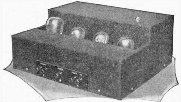
FIG. C. Another of the commercial amplifiers and power units now being placed on the market for the new "intermediate" 245 tube. This is of Ferranti make.
