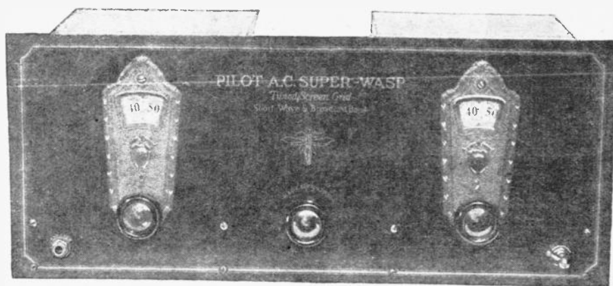
The front panel view of the A.C. Super-Wasp. Tuning is accomplished by the two main tuning dials, while the center knob controls regeneration
