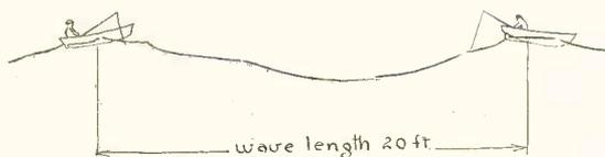
Figure 1. When Both Boats Rise and Fall Together the Wave Length is the Distance Between Them, Here 20 Feet.
