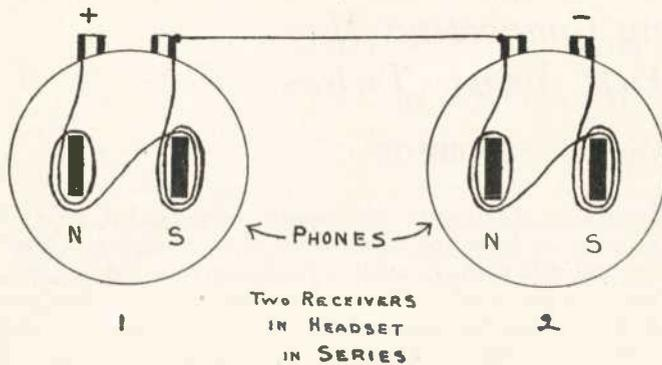
Fig. 4. This Polarity Strengthens Magnets
