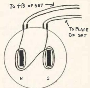
Fig. 3 Polarity of Receiver
