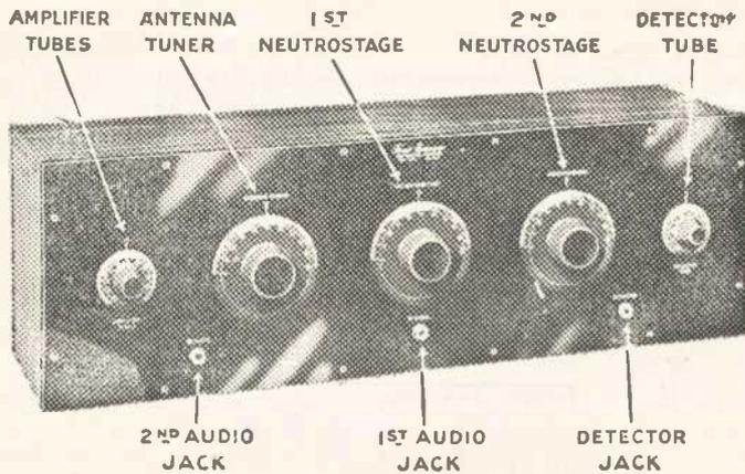
Fig. 2. Names of Neutrodyne Controls
