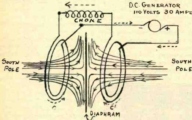
Fig. 3. How Coils Affect Diaphragm
