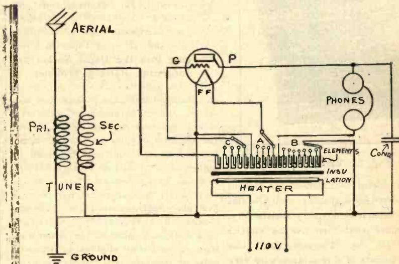
Fig. 6. Hook-up of Thermoformer
