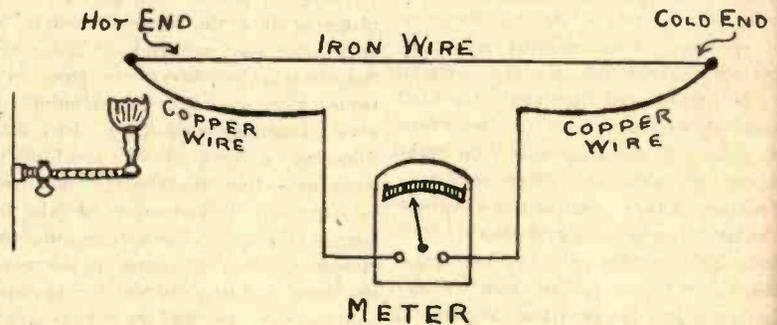
Fig. 4. This is Principle of Thermo-Couple
