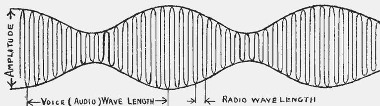
Fig. 1. Carrier Wave Modulated by Audio Frequency
