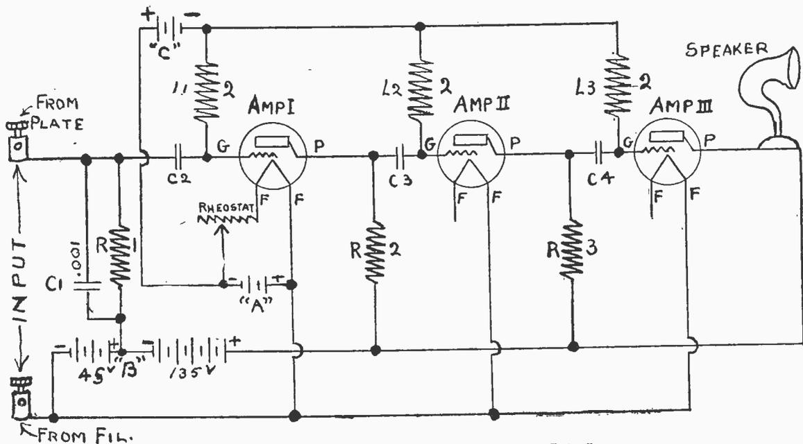
Fig. 1. Three-Step Resistance Amplifier Using Grid Leaks
