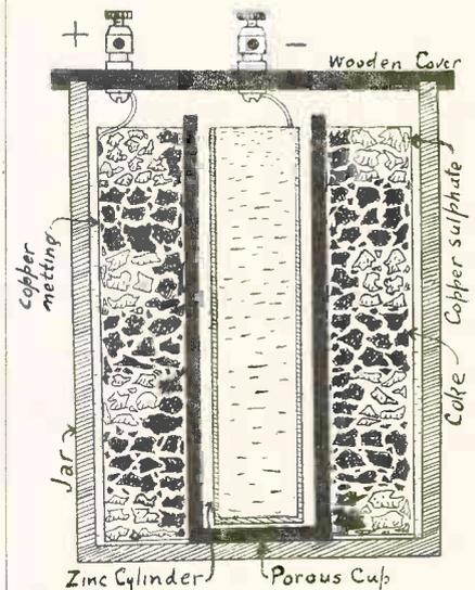
Fig. 4. Details of New Cell
