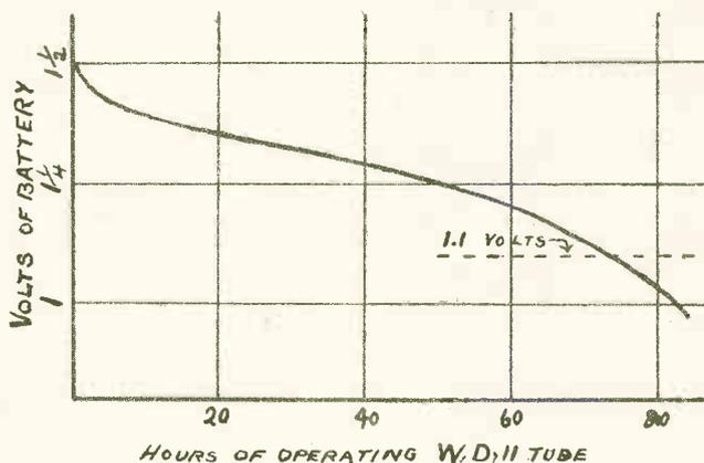
Fig. 1. How Dry Cell Lasts with WD Tube
