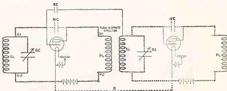
Fig. 1. Neutralizing Circuits of a Neutrodyne
