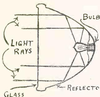
Fig. 2. How Headlight Focuses
