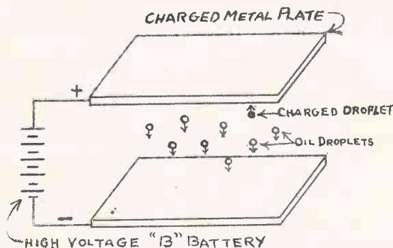
Fig. 1. How Electron Makes Oil Drop Dance
