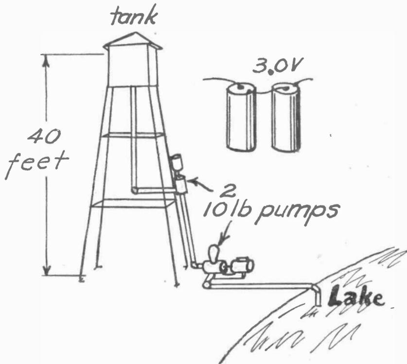
Fig. 3. Pumps in Series, Double Pressure
