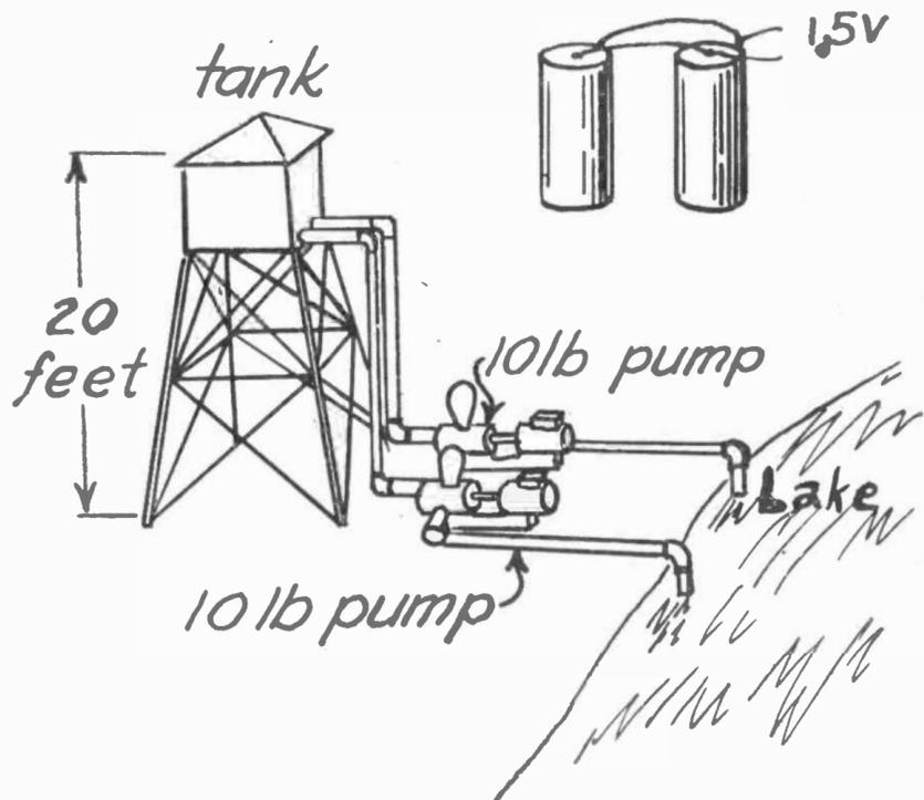
Fig. 4. Pumps in Parallel, Double Current
