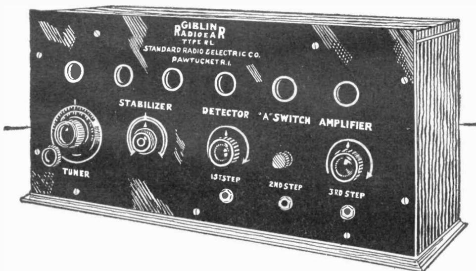
The set comprises two stages of radio frequency amplification, a detector and three stages of audio frequency amplification. The parts are mounted on a sub-base to which a Bakelite panel is attached. It is enclosed in a handsome solid mahogany cabinet.
