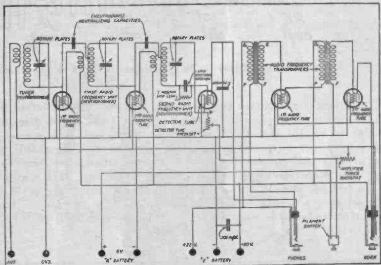
Fig. 4. Neutralized R. F. Amplification in a Neurodyne
