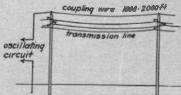
Fig. 3. Broadcasting to the Electric Light Wires
