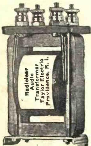
This transformer has  $3\frac{1}{2}$  to 1 ratio, which gives greatest increase of loudness possible without introducing distortion. One reason for its clear music is the generous amount of iron in the circuit. Such special transformer iron is expensive, but results justify its use. The large number of turns of wire is what makes the program so loud.
