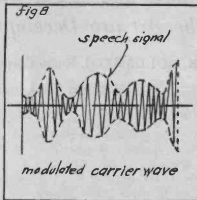
Fig. 3. The Varying Loudness Shows Wave Is Modulated
