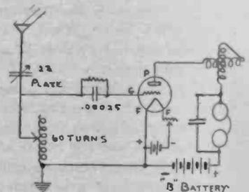
Fig. 3. Regeneration from a Variometer
