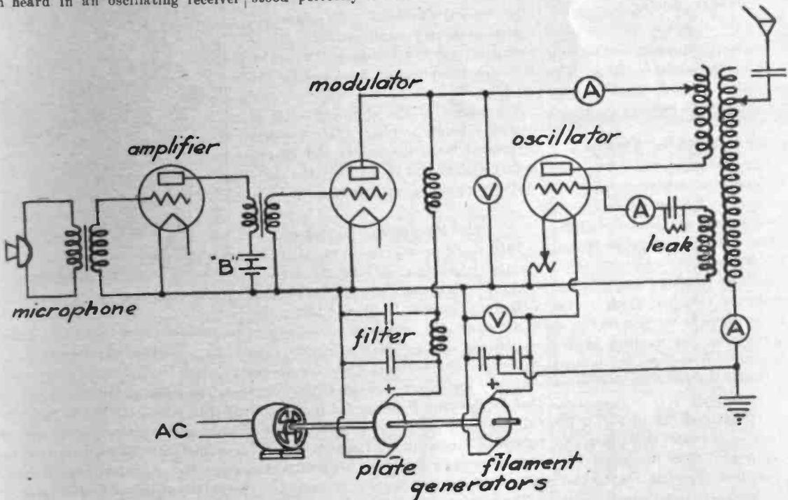
Fig. 6. Complete System. This Combines the Oscillator of Fig. 2 with the Modulator of Fig. 4
