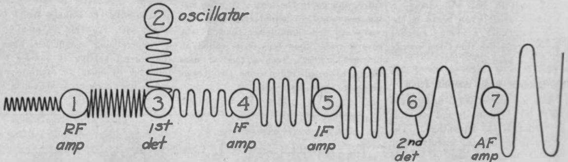
Fig. 5. What the Tubes Do in a Superhet. R. F., A. F., Detector, and Oscillator Tubes Are Needed
