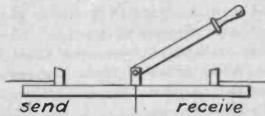
Fig. 1. Old Scheme—Listener Must Throw Switch
