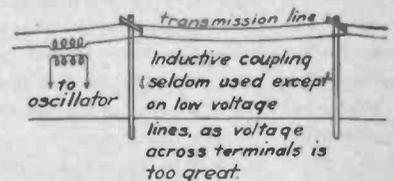
Fig. 2. Coupling for Small Stations
