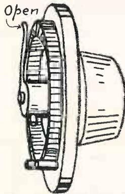
Fig. 3. This Explains a Frequent Cause of "Static"
