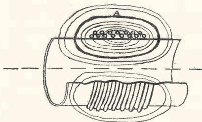
Fig. 1. A Honeycomb Coil is Like a Banked Winding Developed
