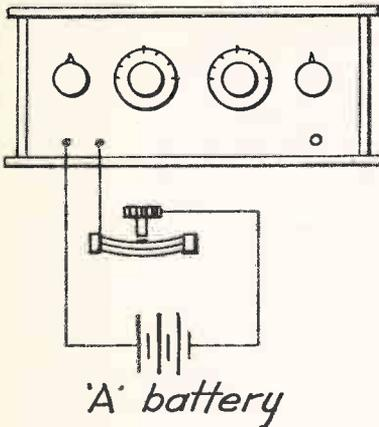
Fig. 5. Hook-up in Set for Radio Alarm
