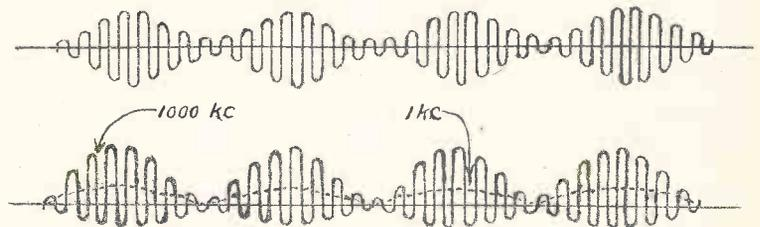
Fig. 5. How the Detector Treats the Amplified Waves of Fig. 4. Notice the Shape is Changed
