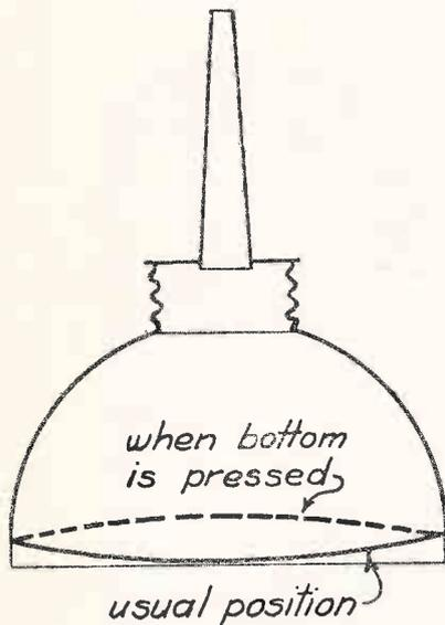
Fig. 3. Snap Action is Like Bottom of Oil Can
