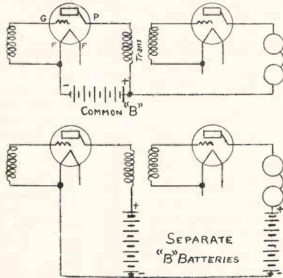
Fig. 2. This Invention Saves a Lot of "B" Batteries
