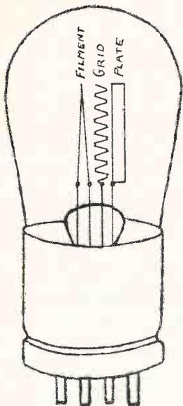
Fig. 6. The Necessary Parts Inside a Tube—Three Elements
