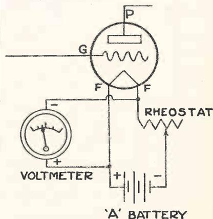
Fig. 1. Proper Way to Use Meter in Adjusting Filament
