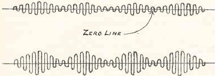
Fig. 4. What an Amplifier Does to Incoming Radio Waves. Shape is the Same
