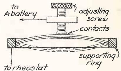
Fig. 4. How Contact is Made by New Thermostat
