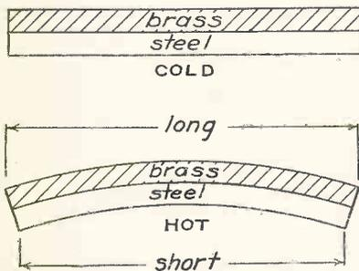
Fig. 1. Brass Expands with Heat and Bends Steel
