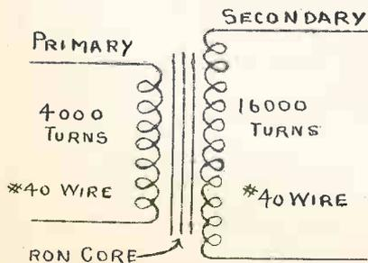
Fig. 1. Shows Principle of Iron-Cored Transformer
