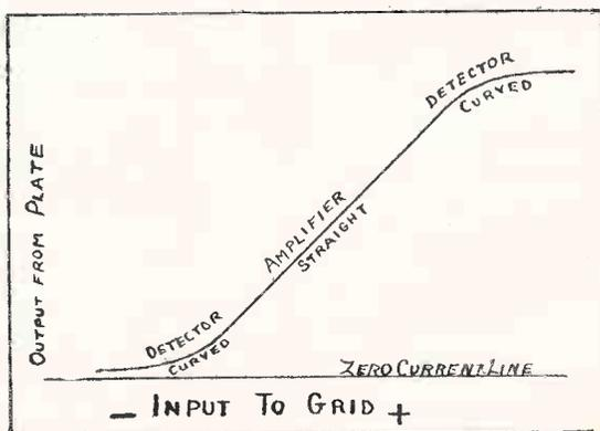
Fig. 7. This is the Curve Which Shows How a Tube Acts
