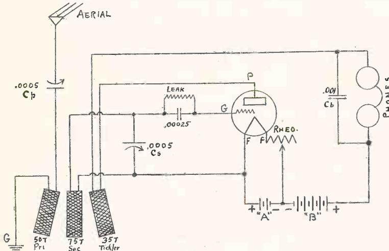
Fig. 2. Connections for Honeycomb Set. Selective Because of Loose Coupling
