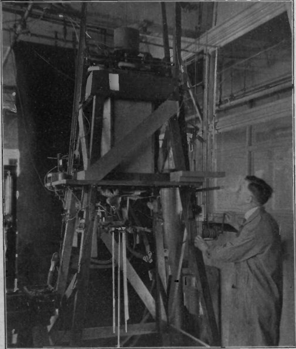
Fig. 3. Here is the Special Vacuum Furnace in Which the Quartz is Melted. A Carbon Resistance is Used in Generating the Tremendous Heat
