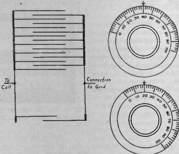
Fig. 2. Although Main Dial is Unchanged, the Vernier has Shifted, Which Throws Set Out of Tune
