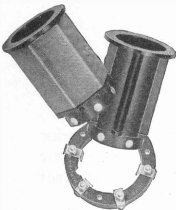
S-M interchangeable inductances are the last word in low loss coil design. They are wound with enameled wire on the threaded bakelite forms. This method of space winding brings these inductances to the highest point of efficiency. It also assures a uniformity of approximately one-quarter of one per cent, making S-M coils ideal for gang condenser tuning—their uniformity is permanent. Made in five wavelength ranges fitting type 515 coil sockets. Suited to all standard circuits.
