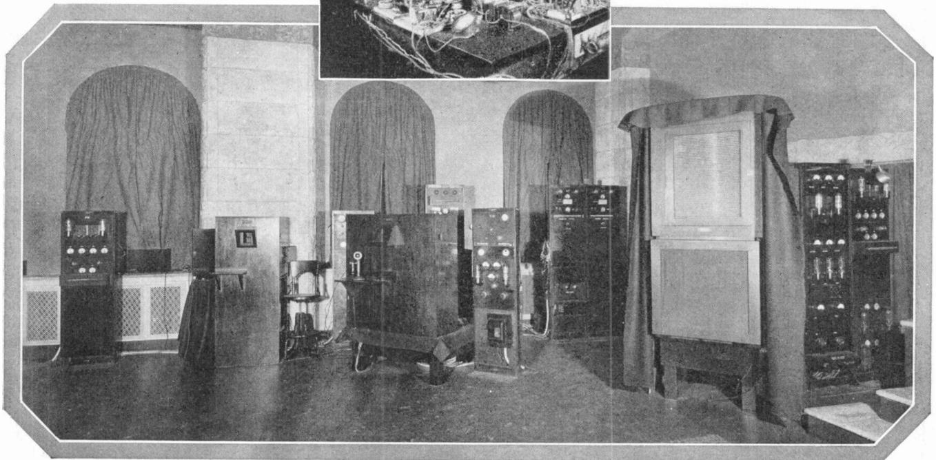
That television is, in its present state, a complicated and expensive function is shown by this photo of the apparatus developed by the American Telephone and Telegraph Company. Left to right: 1, Control panel for monitor board; 2, Monitor board for operator; 3,
