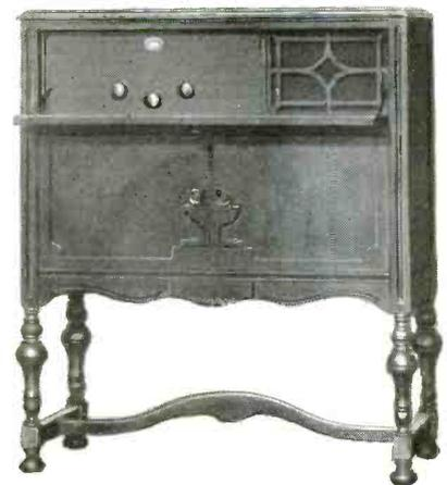
A six tube tuned radio frequency console model. Single dial station selector with separate vernier adjustment, stabilized circuit, two stages radio frequency, detector, three stages audio. Attractive blended cabinet with built-in speaker and space for batteries, etc.
