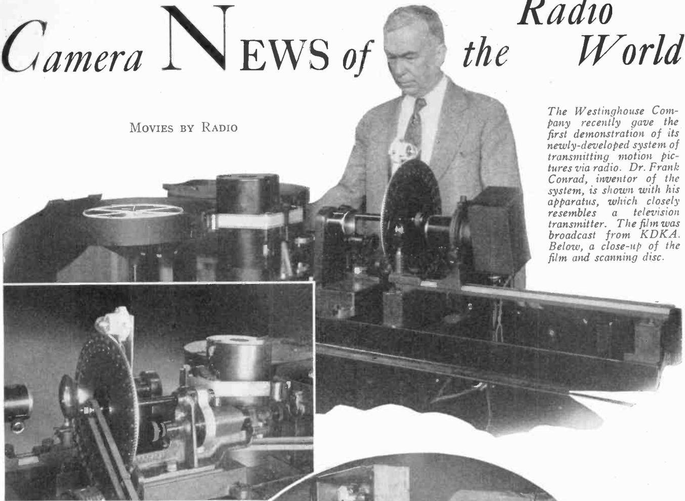
The Westinghouse Company recently gave the first demonstration of its newly-developed system of transmitting motion pictures via radio. Dr. Frank Conrad, inventor of the system, is shown with his apparatus, which closely resembles a television transmitter. The film was broadcast from KDKA. Below, a close-up of the film and scanning disc.
