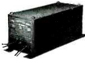
Here's permanent B-Power for auto radios, giving full volume, undiminished by time or usage. Completely replaces dry "B" batteries. Transforms 6 or 12 volt current from storage battery into 135 or 180 volt "B" current. Furnished complete with voltage divider for tapping off "C" current.
