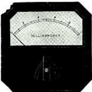
Bakelite case measures 3 1/2" square, mounts through 2 5/16" panel hole. Long arc scale with knife edge pointer. Rugged movement of 2% accuracy—sensitivity 50 MV in the 0/1 MA range.
