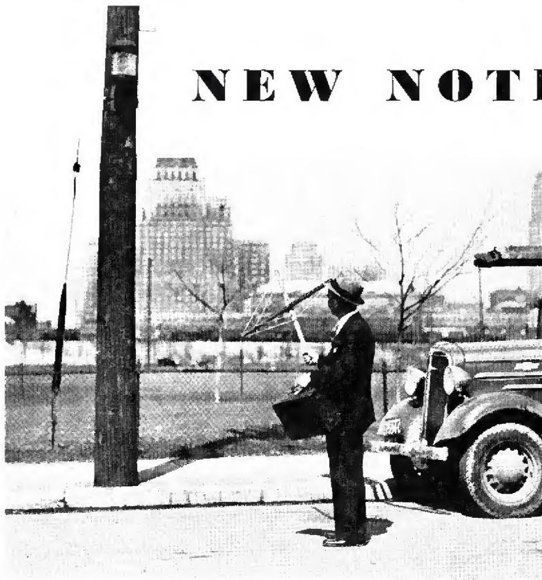
**CHECK-UP**—The author runs down noise with a portable receiver and a loop
